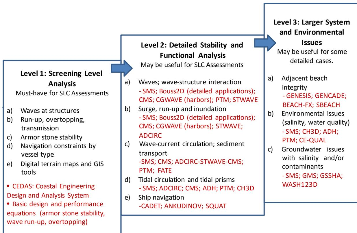
Figure C-12. Graduated levels of USACE analysis tools and modeling techniques.
