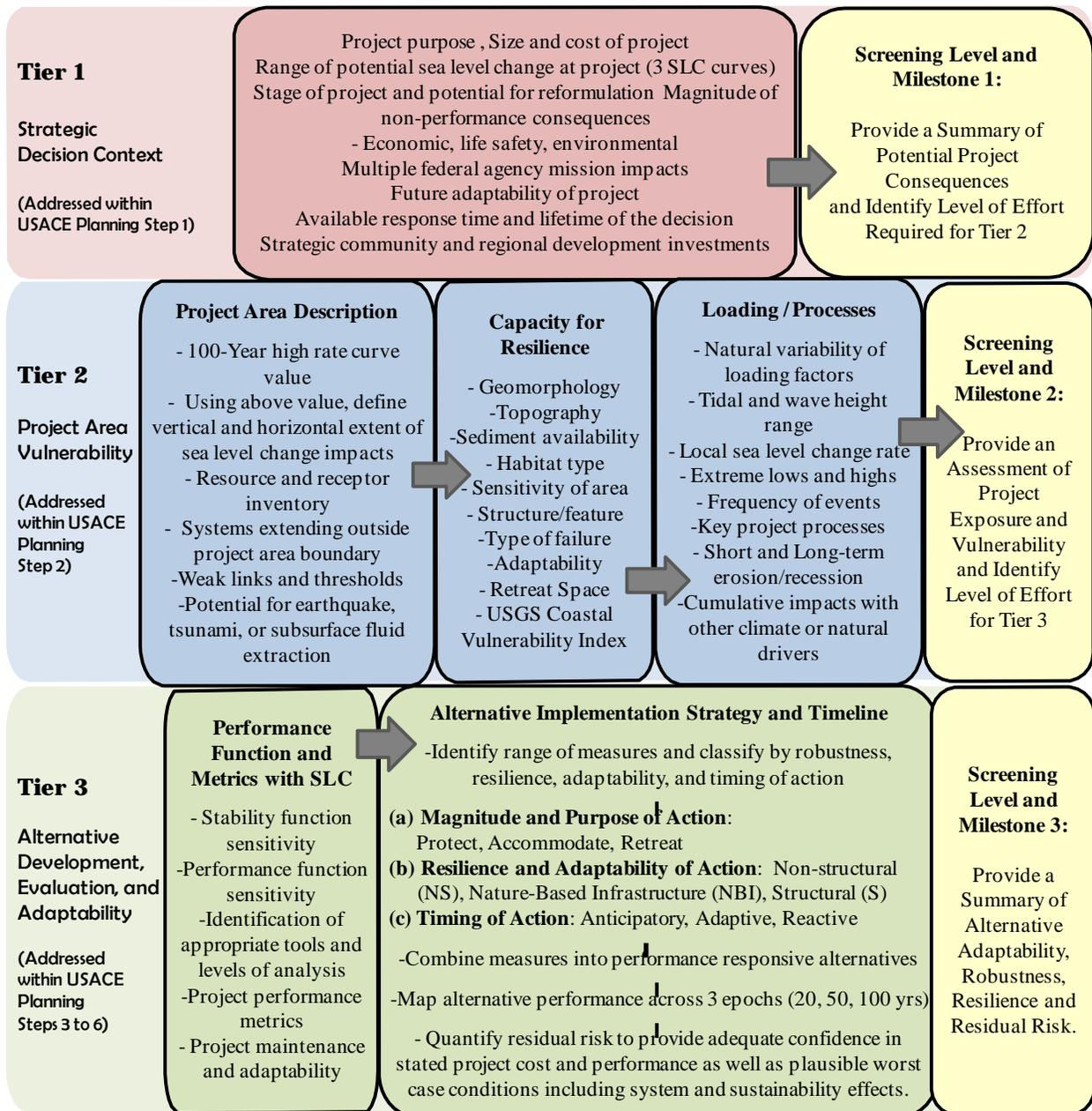
Figure 9. Screening process flowchart for analyzing and incorporating SLC throughout the project life cycle.
