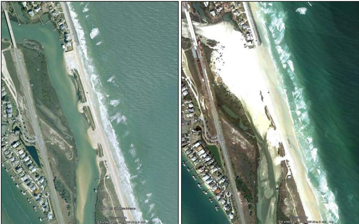
Figure D-10. Example of low-upland barrier island overwash at Summer Haven, Florida. The left panel depicts initial overwash fans; the right panel depicts barrier island roll-over and breaching resulting from storm waves and surge.
