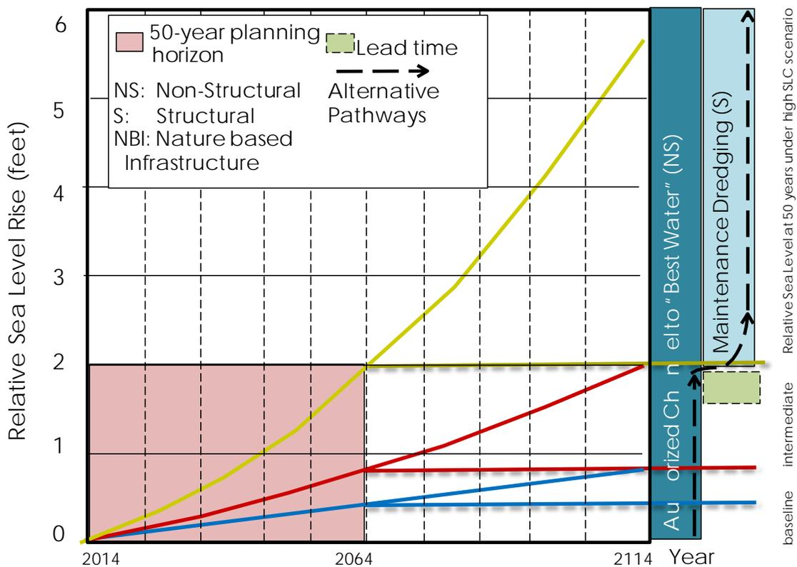
Figure C-11. Transition of a project feature over the life cycle from “best water” to maintenance dredging for the three USACE SLC planning curves (blue is low, red is intermediate, and yellow is high-rate curve).
