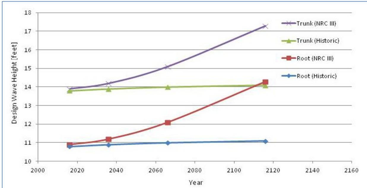
Figure C-15. Depth-limited breaking wave heights (with SLC).
