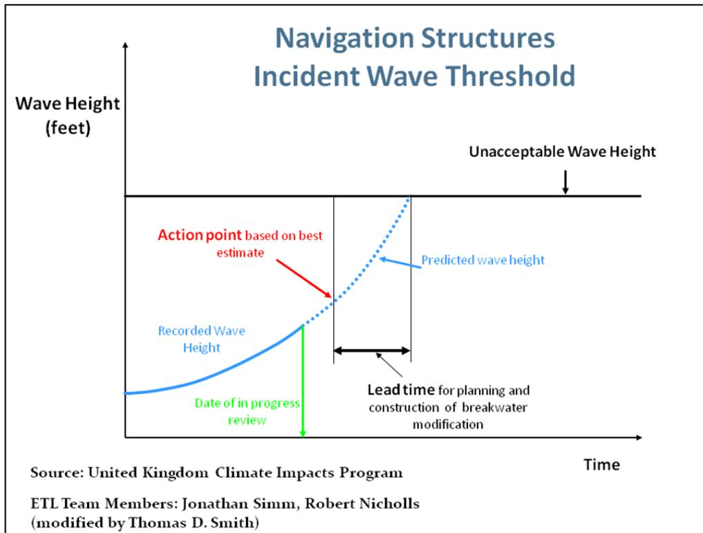
Figure C-2. Activities required under an adaptive strategy to prevent reaching a tipping point at which wave height becomes unacceptable.
