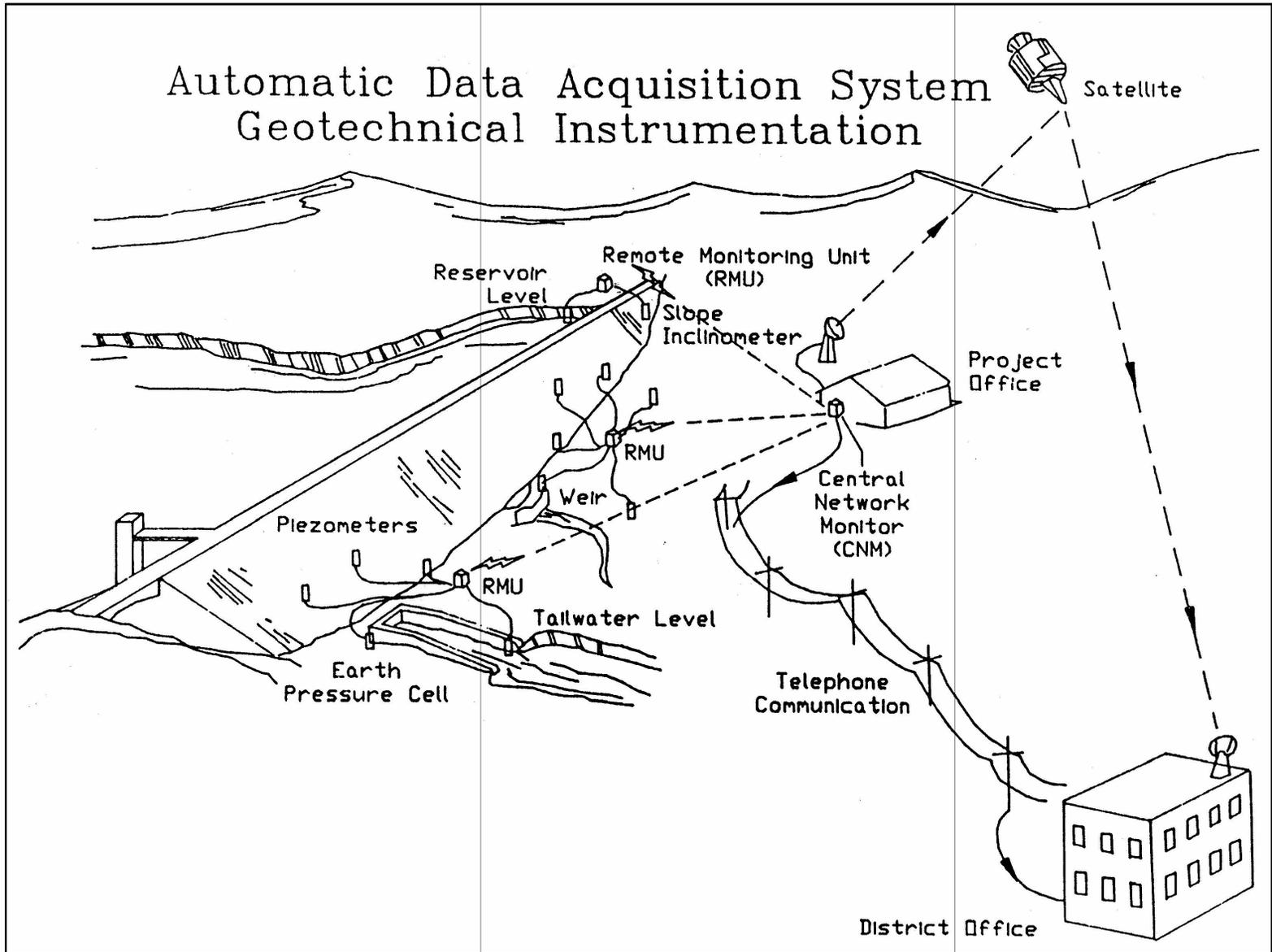
Figure D-1. Typical project automation plan
