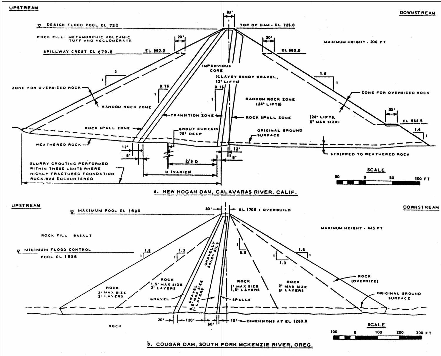
Figure 7-3. Embankment sections, rock-fill dams (New Hogan and Cougar Dams)
