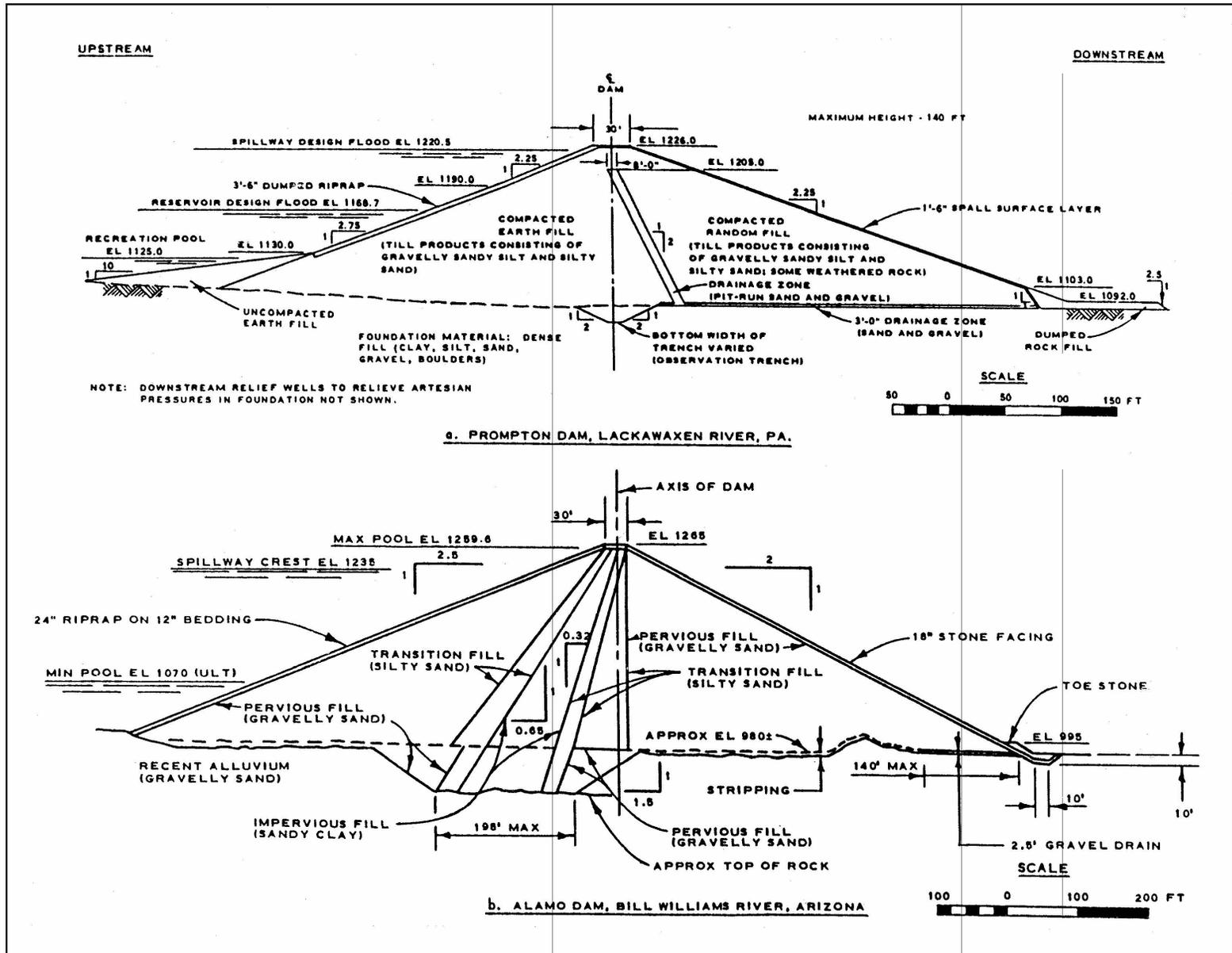
Figure 7-1. Typical embankment sections, earth dams (Prompton and Alamo Dams)
