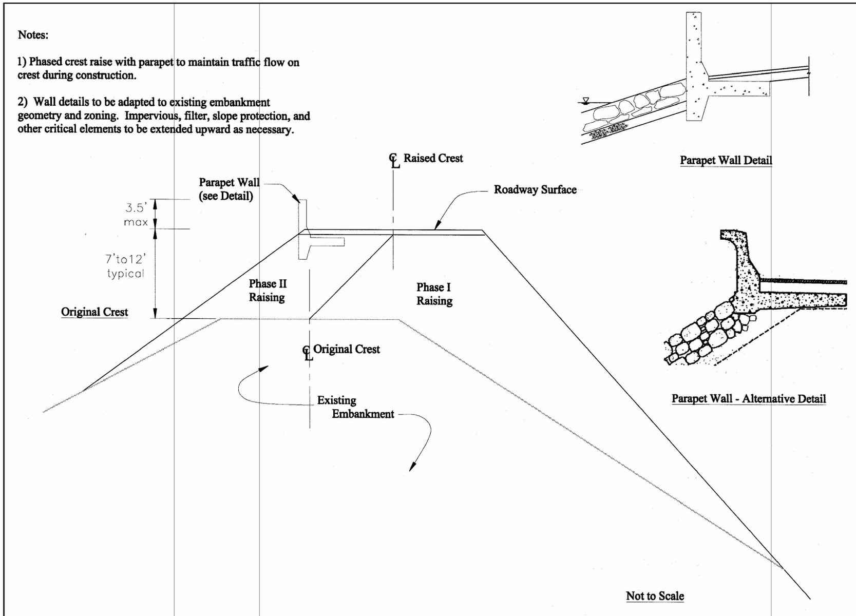
Figure F-4. Embankment raising with parapet wall
