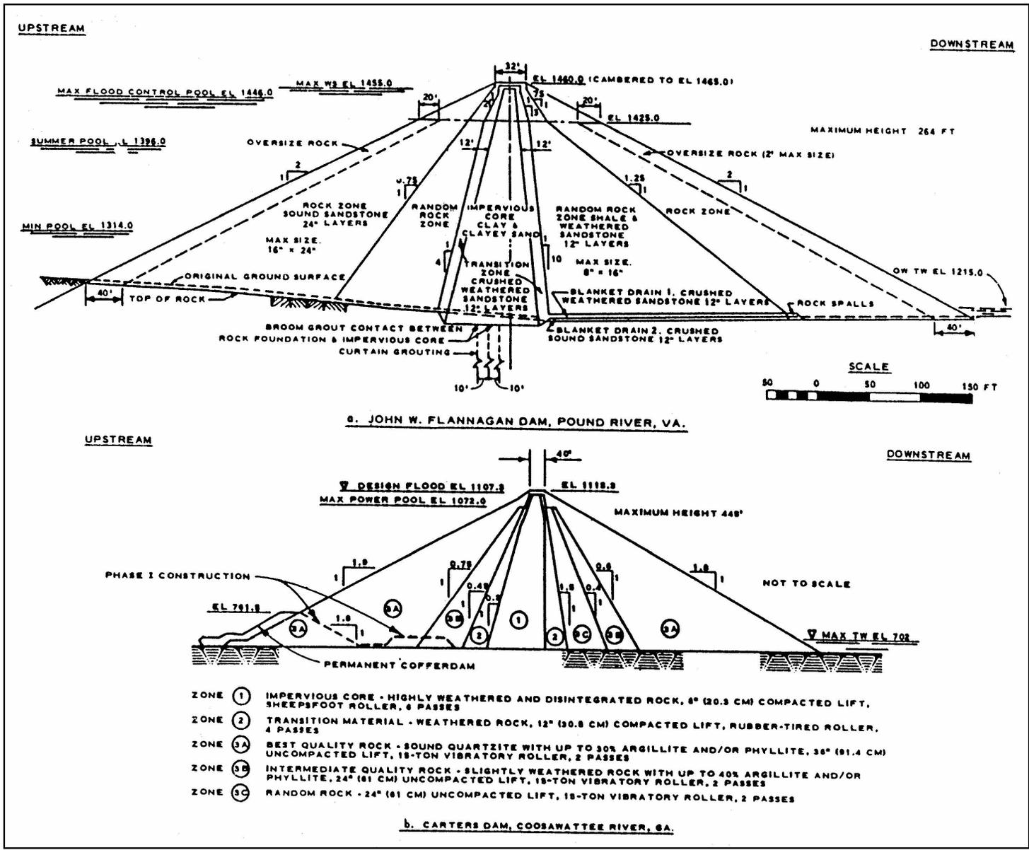
Figure 7-4. Embankment sections, rock-fill dams (John W. Flannagan and Carters Dams)
