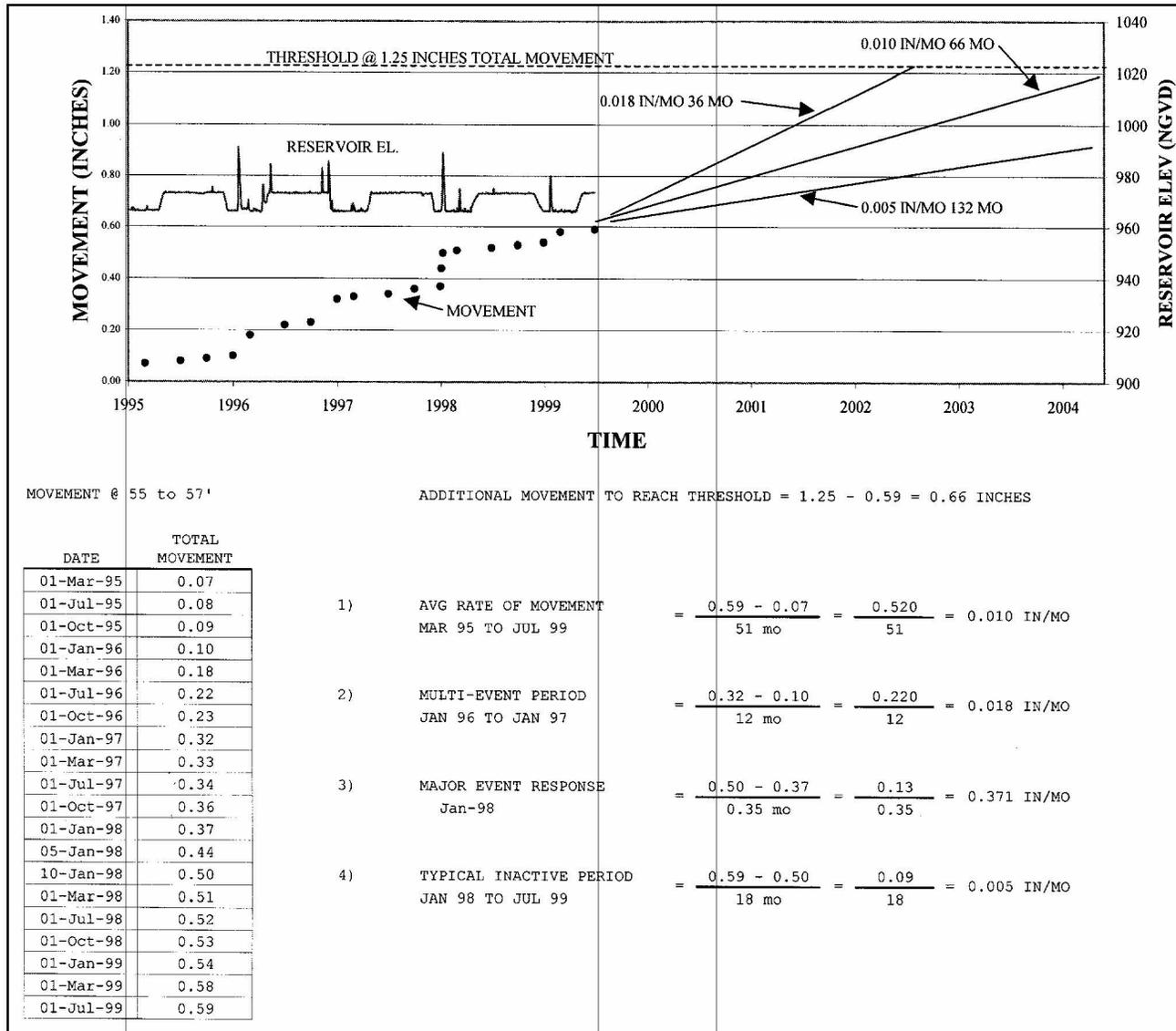
Figure E-4. Deflection/threshold movement
