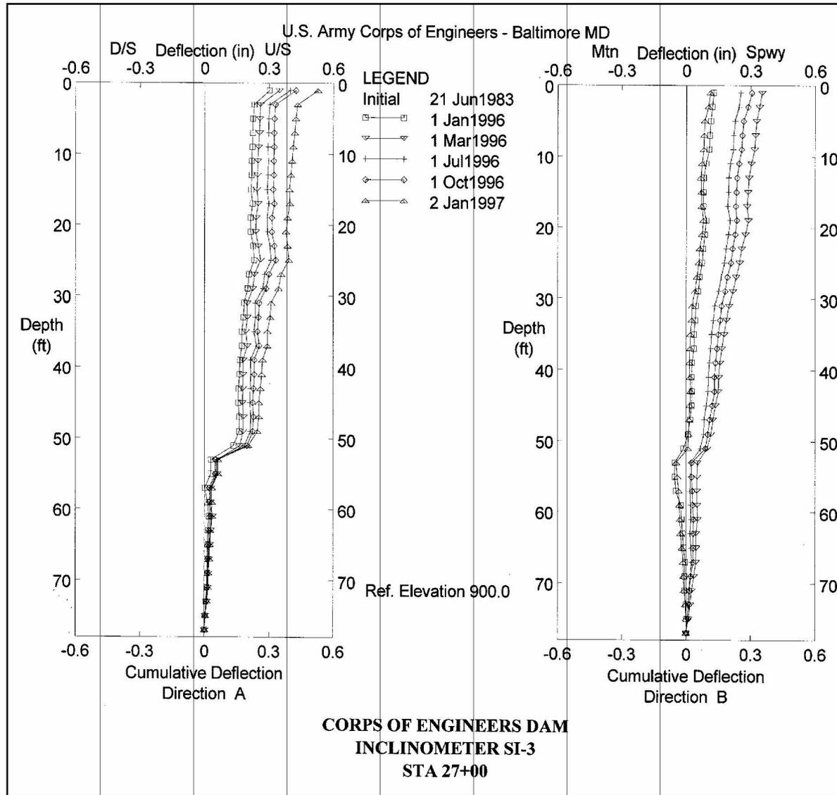
Figure E-5. Typical inclinometer plot
