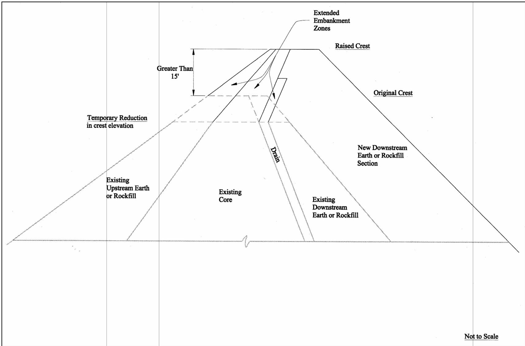
Figure F-8. Downstream raising of embankment dam
