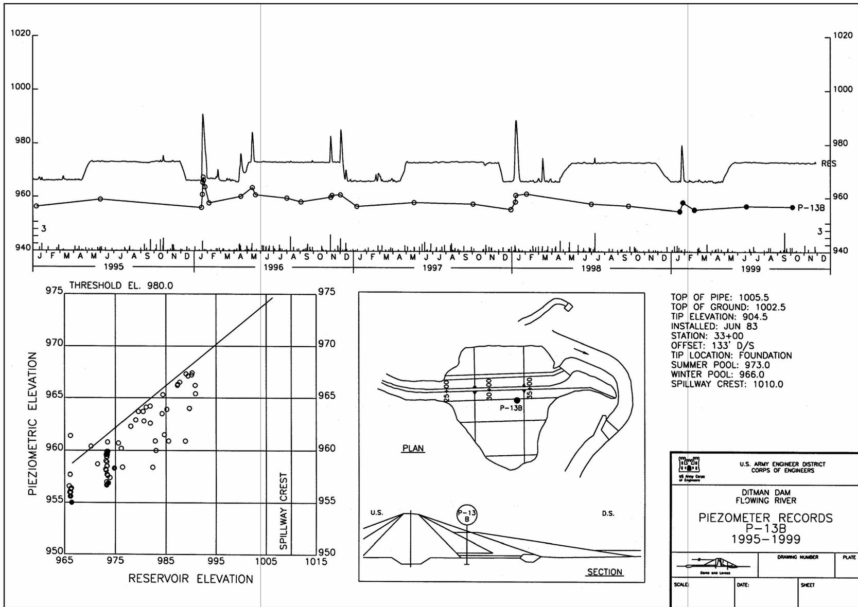
Figure E-2. Typical piezometer plot
