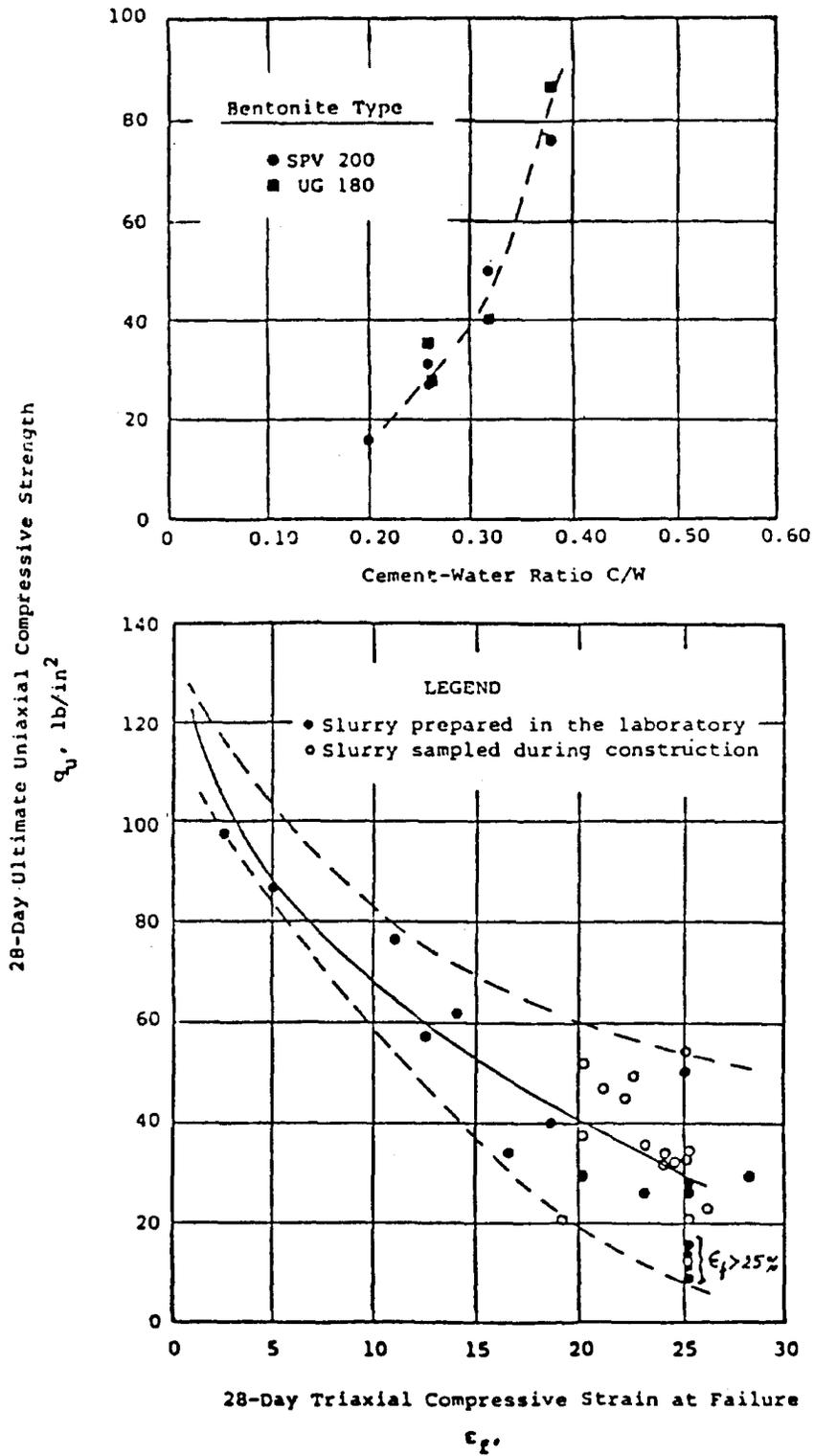
Figure 9-12. Strength and deformation characteristics of cement-bentonite slurries (courtesy of American Society of Engineers<sup>223</sup>)
