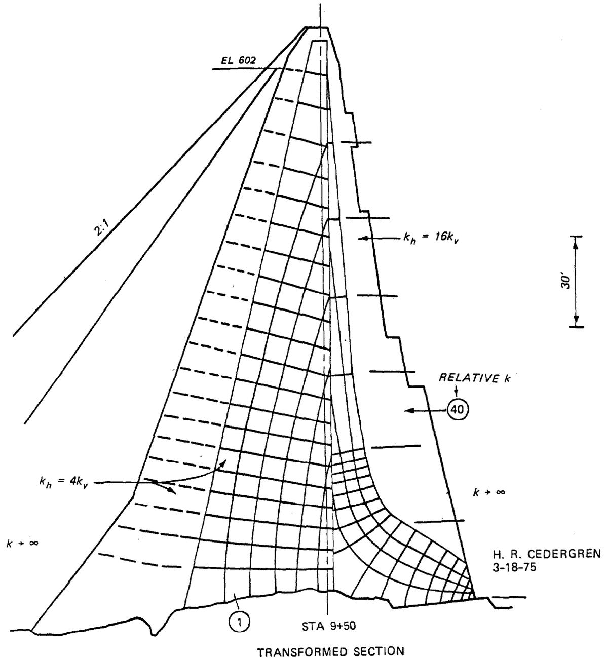
Figure 6-17. Buchanan Dam flow net studies full reservoir- Sta 9+50 D/S transition fill -  $k_h = 16 k_v$  transformed section (from Cedergren<sup>25</sup> and U. S. Army Engineer District, Sacramento 1977)
