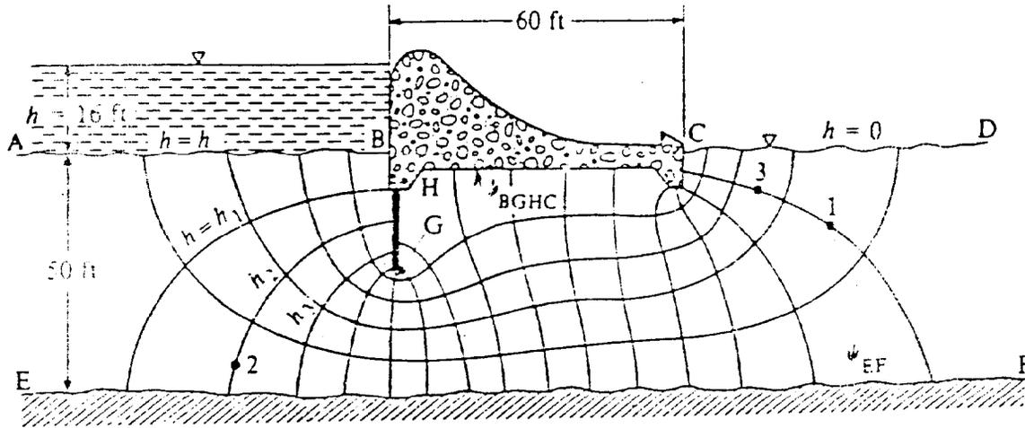
Figure 5-2. Gravity dam on pervious foundation of finite depth
