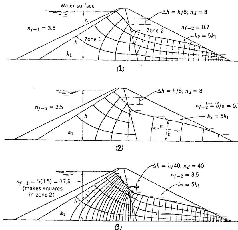
Figure 6-16. Three forms of one flow net (courtesy of John Wiley and Sons<sup>155</sup>)
