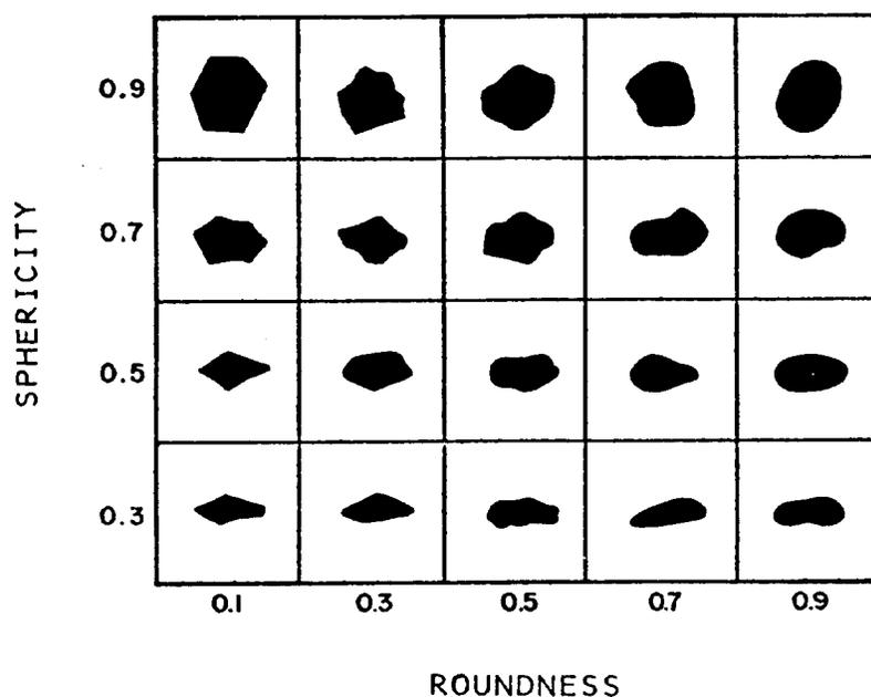
Figure 2-10. Krumbein and Sloss standard chart for visual estimation of sphericity and roundness of cohesionless soils (courtesy of W. H. Freeman and Company<sup>198</sup>)
