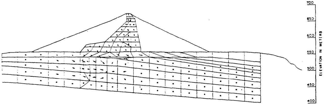
Figure B-22. Finite element study results (courtesy of International Commission on Large Dams<sup>269</sup>)
