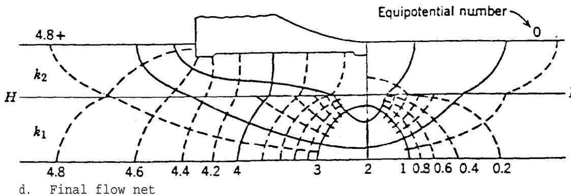
Figure 4-12. Flow net construction for a composite section (courtesy of John Wiley and Sons<sup>155</sup>)
