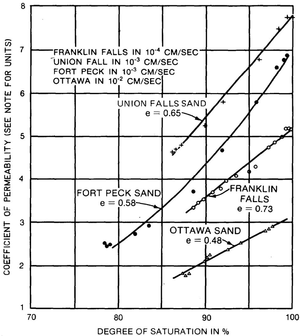
Figure 2-7. Permeability versus degree of saturation for various sands (courtesy of John Wiley & Sons, Inc. <sup>200</sup>)
