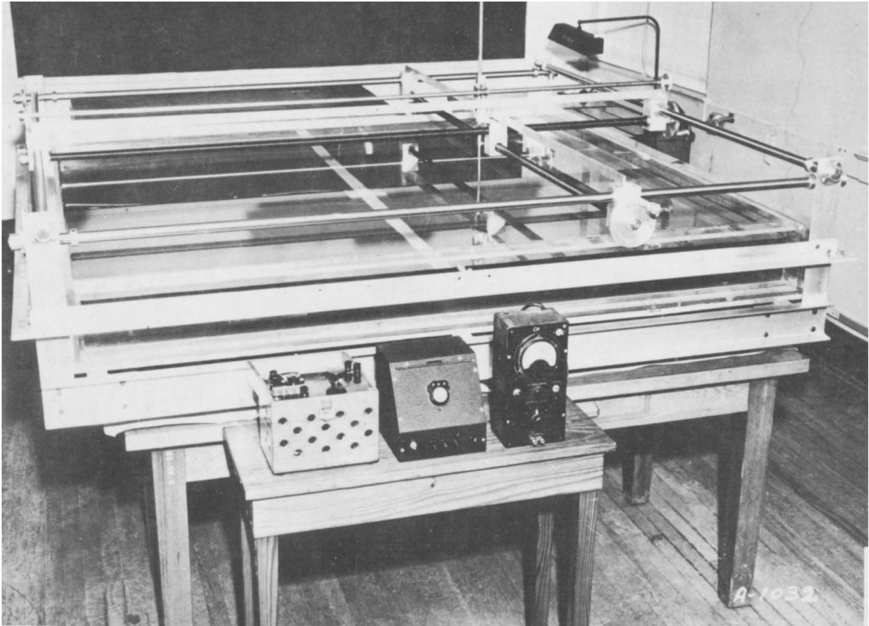
Figure B-1. Three-dimensional electrical analogy apparatus (after Duncan<sup>36</sup>)
