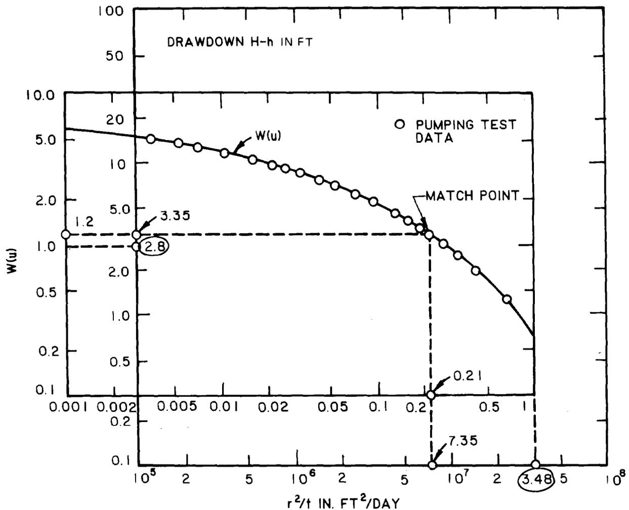
Figure 7-9. Use of type curve for analysis of nonsteady state flow (courtesy of John Wiley and Sons<sup>164</sup>)
