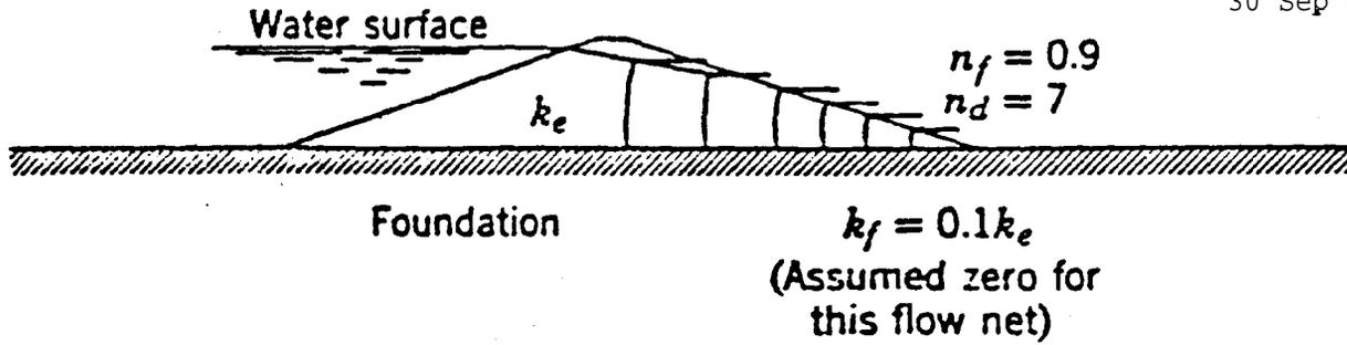
a. Construct flow net assuming an impermeable foundation.
