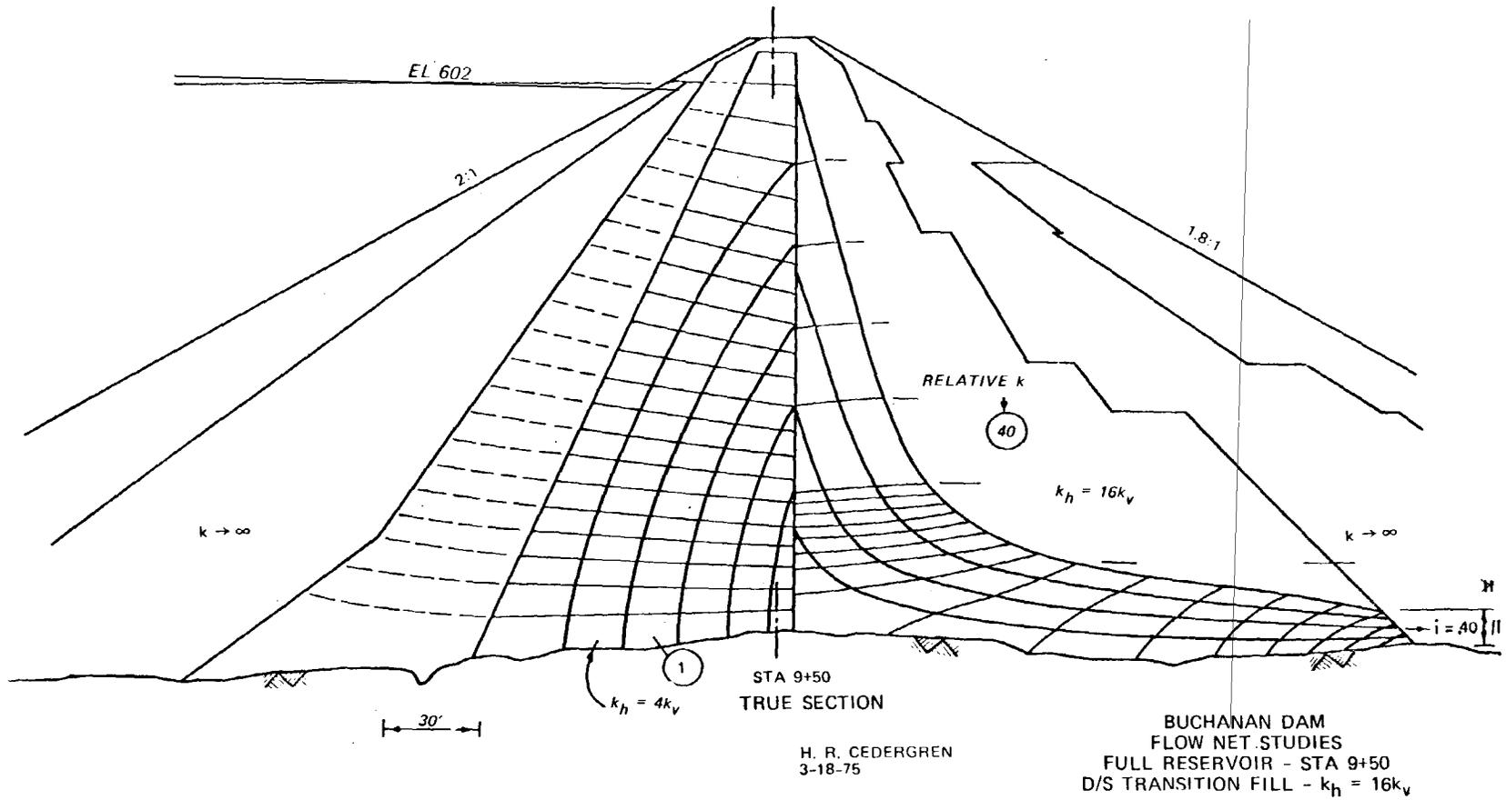
Figure 6-18. Buchanan Dam flow net studies full reservoir - Sta 9+50 D/S transition fill -  $k_h = 16 k_v$  true section (from Cedergren<sup>25</sup> and U. S. Army Engineer District, Sacramento 1977)
