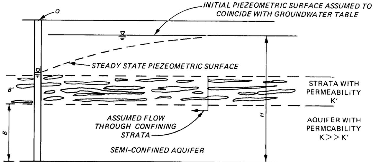
Figure 7-8. Flow to well with significant vertical flow through confining layer (courtesy of John Wiley and Sons<sup>164</sup>)
