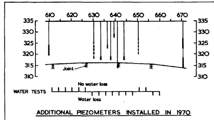
Figure 13-6. Layout of Baldershead Dam piezometer installation in upstream shale fill (courtesy of British Geotechnical Society<sup>212</sup>)
