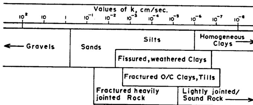
Figure 2-5. Approximate range in coefficient of permeability of soils and rocks (from Milligan<sup>224</sup>)
