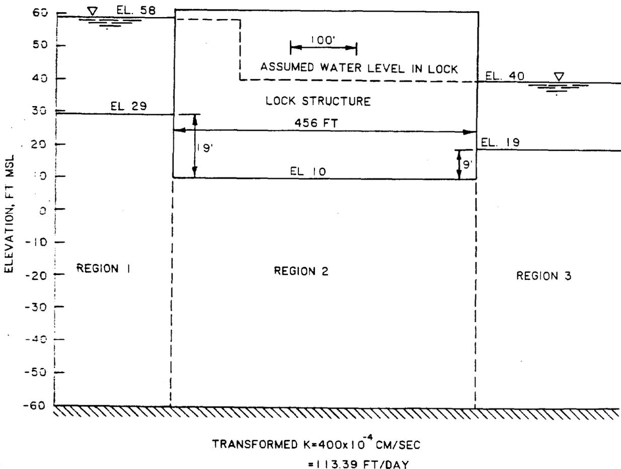
Figure B-16. Transformed section of John H. Overton Lock simplified to one soil layer (from U. S. Army Engineer District, St. Louis<sup>112</sup>)
