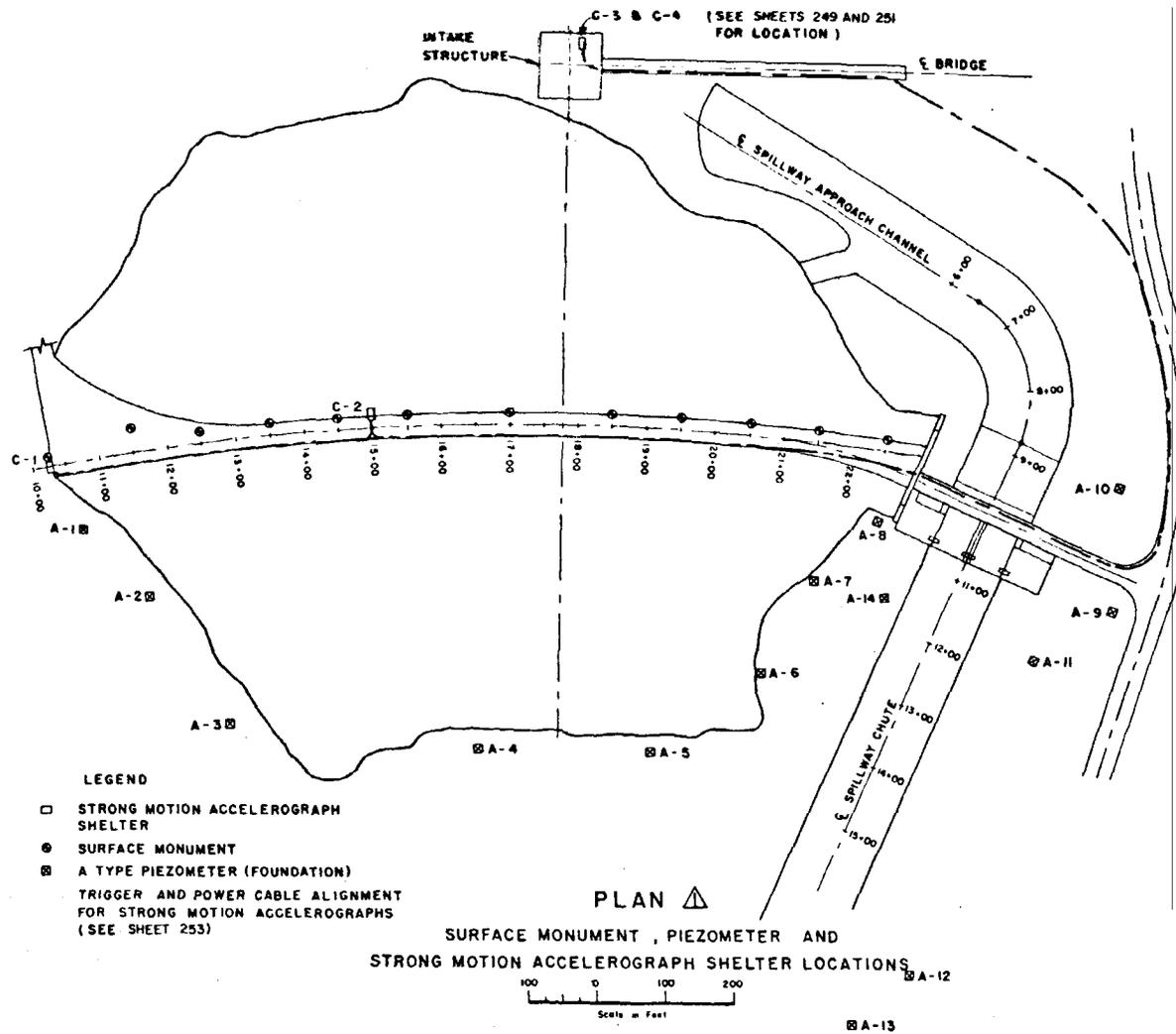
Figure 13-4. Piezometer installation for dam abutments having grout curtains or cut-slope drains, Applegate Lake Dam (from U. S. Army Engineer District, Portland<sup>104</sup>)
