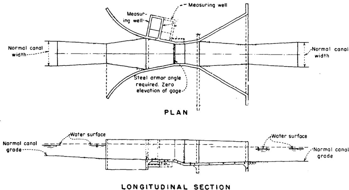
Figure 13-14. Modified Parshall flumes of 6- to 65-second-foot capacity (after Bureau of Reclamation<sup>24</sup>)
