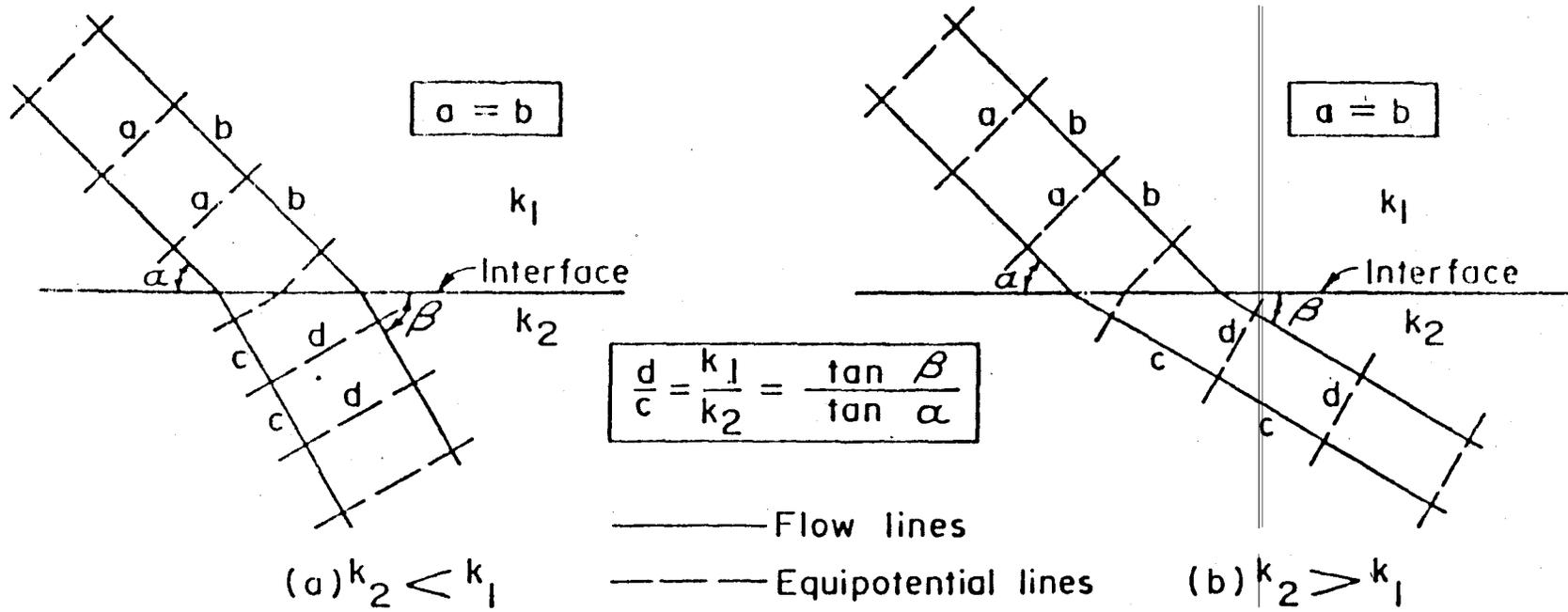
Figure 4-11. Deflections of flow lines at interfaces of soils having different permeabilities (courtesy of New England Waterworks Association<sup>151</sup>)
