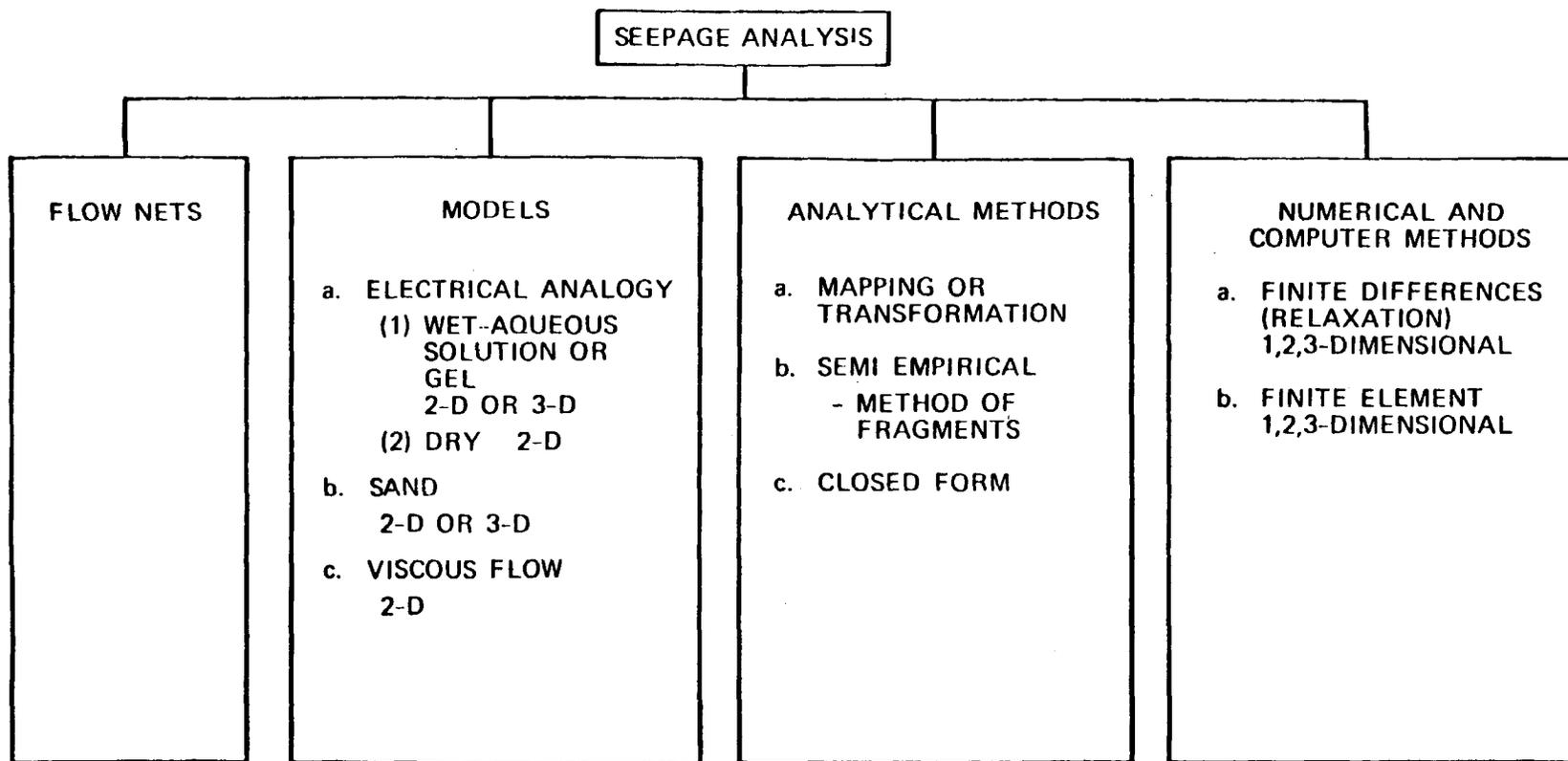
Figure 4-3. Seepage analysis methods (from Radhakrishnan<sup>66</sup>)
