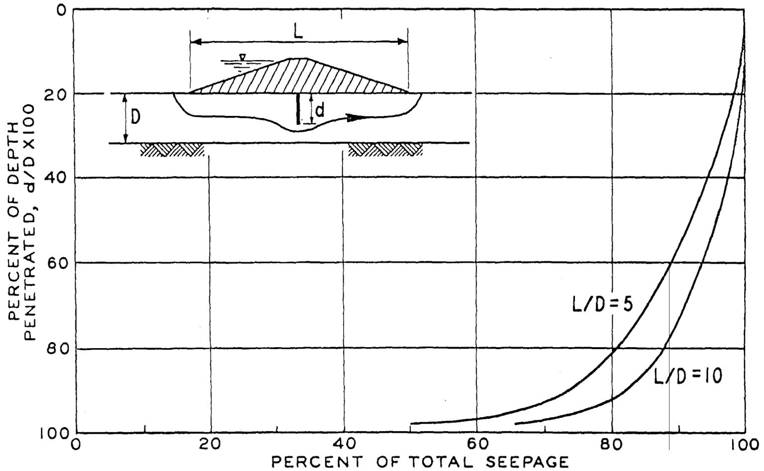
Figure 9-2. Effect of depth of penetration of partial cutoff on seepage reduction for a homogeneous isotropic foundation (prepared by WES)
