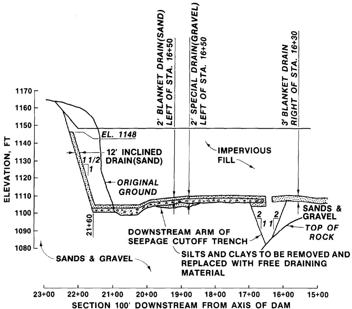
Figure 10-2. Seepage control of left pervious abutment at North Branch of Kokosing Dam, Ohio (from U.S. Army Engineer District, Huntington<sup>87</sup>)
