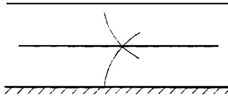
The flow line and equipotential line nearest an angle should intersect on the bisector of the angle.
