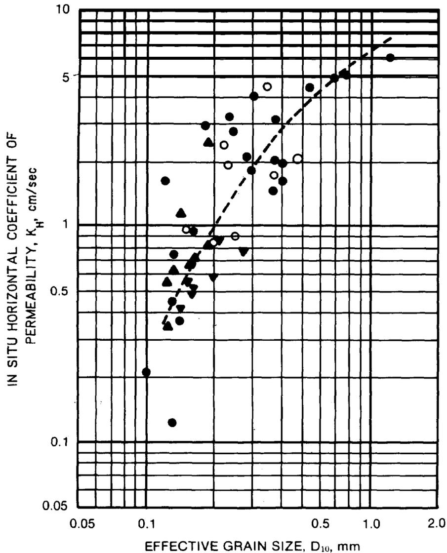
Figure 2-15. Relationship between in situ horizontal permeability and effective size (prepared by WES<sup>120</sup>)
