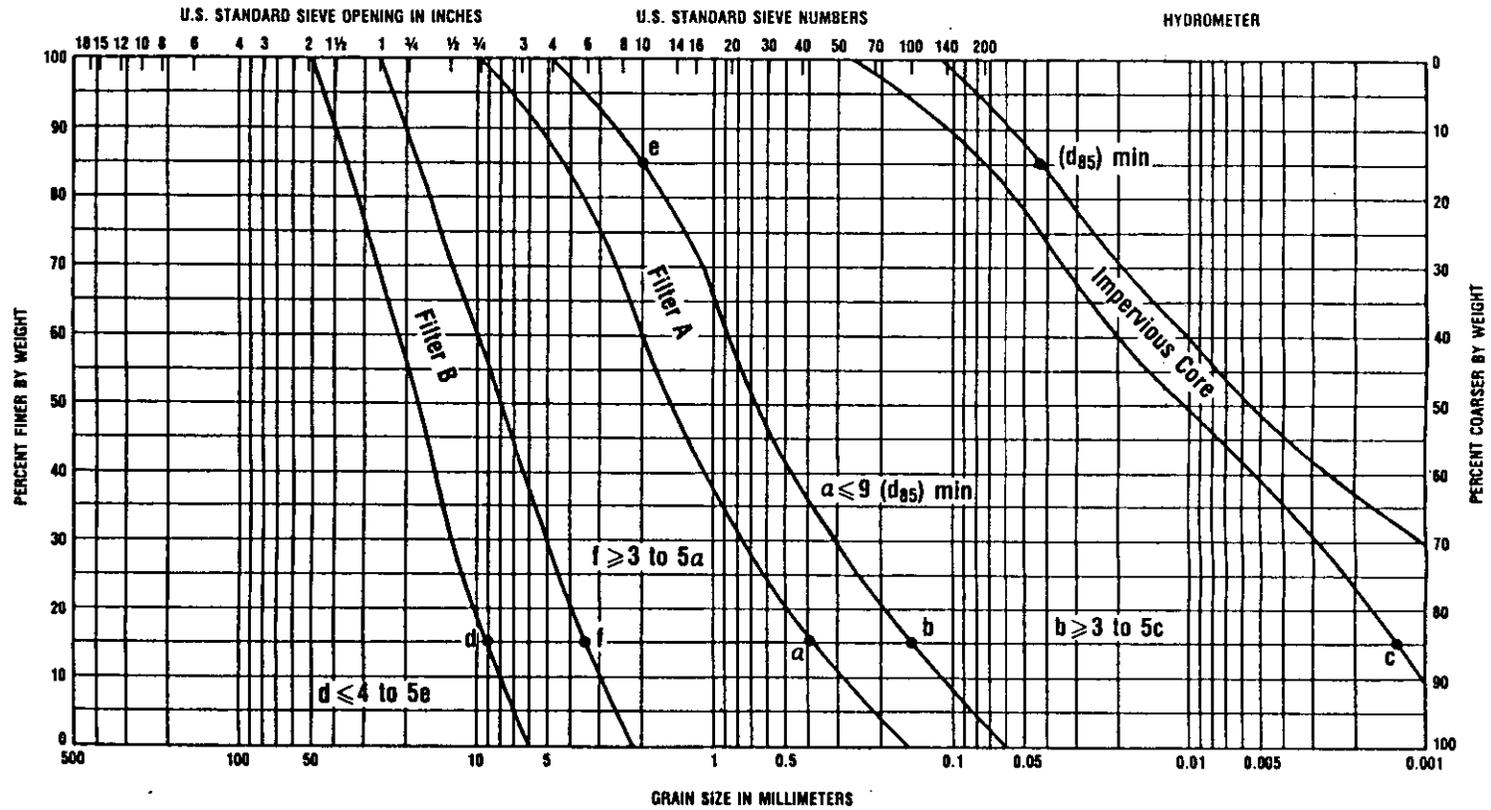
Figure D-2. Illustration of the design of a graded filter
