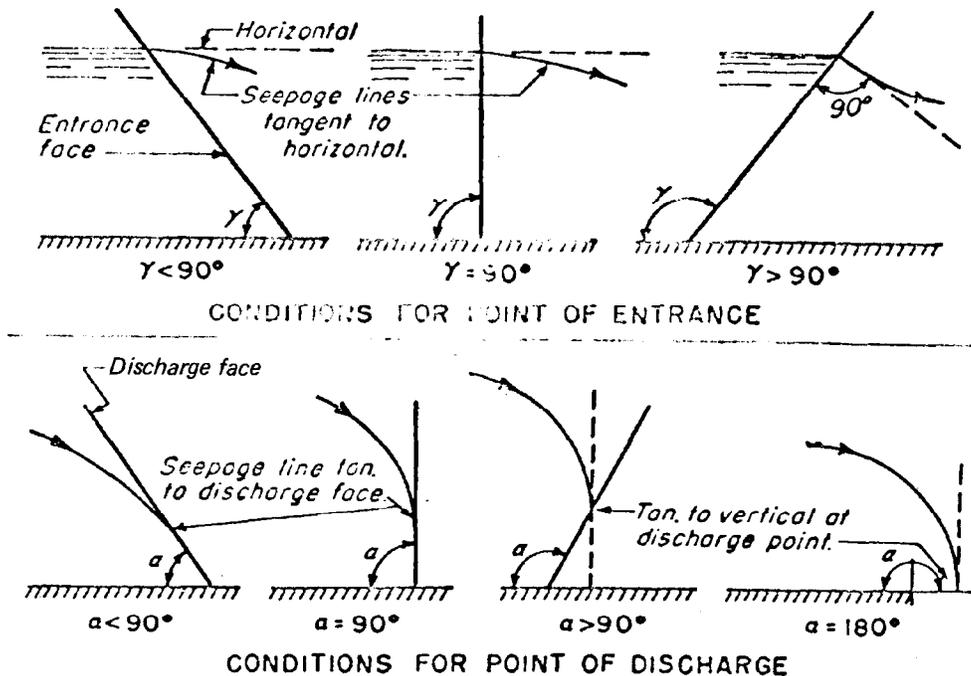
Figure 4-7. Entrance and discharge (exit) conditions for a line of seepage (courtesy of New England Waterworks Association <sup>151</sup>)
