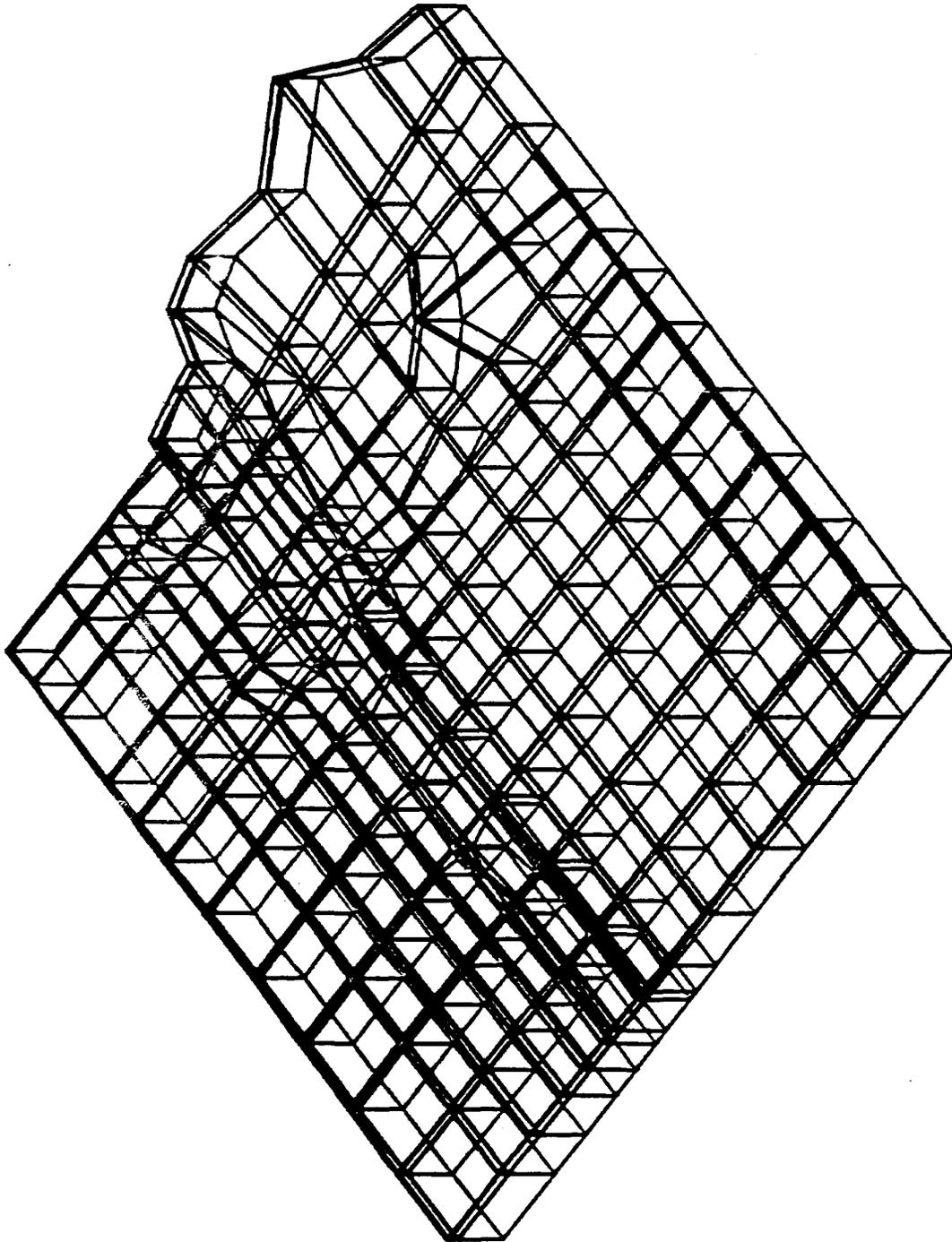
Figure B-26. Grid for three-dimensional finite element model study of Calamus Dam, Nebraska (courtesy of American Society of Civil Engineers<sup>217</sup>)
