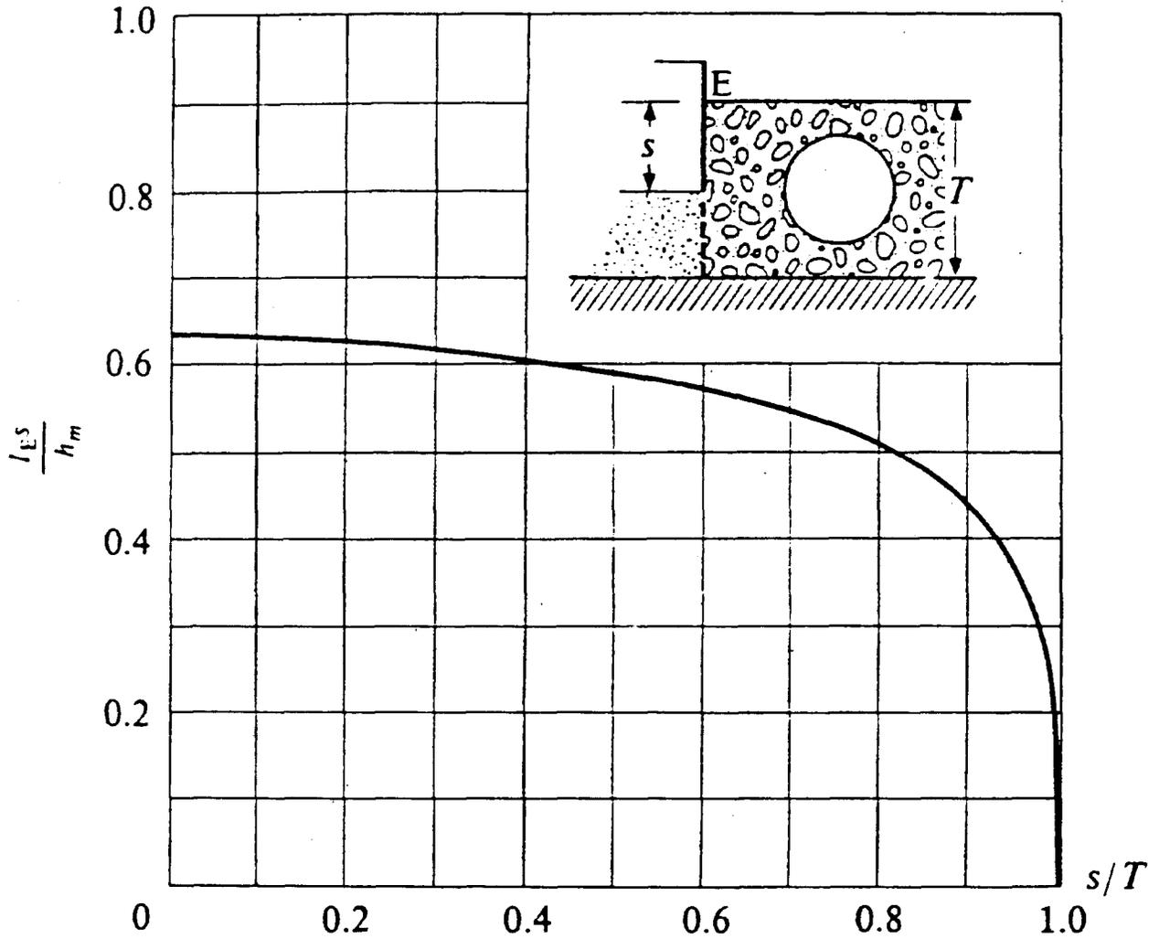
Figure B-15. Relationship for determining the exit gradient as a function of the head loss in the fragment and geometry for a Type II fragment (courtesy of McGraw-Hill Book Company<sup>181</sup>)
