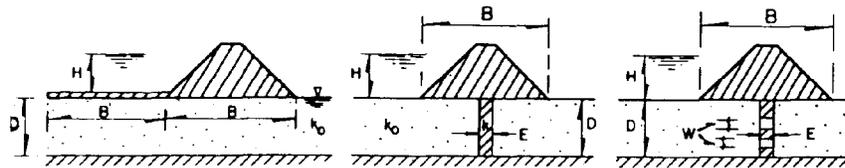
Impervious upstream blanket      Compacted backfill trench      Concrete wall or slurry trench
