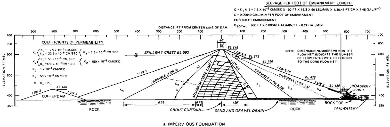
Figure 6-19. Seepage analysis, Blakely Mountain Dam, Arkansas (from U. S. Army Engineer Waterways Experiment Station<sup>121</sup>)
