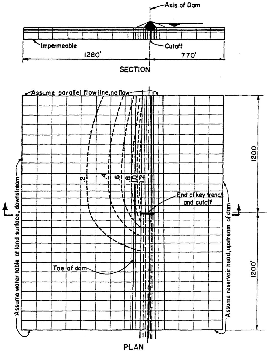
Figure B-24. Contours of exit gradient from three-dimensional finite element model study of Narrows Dam, Colorado (courtesy of American Society of Civil Engineers<sup>217</sup>)
