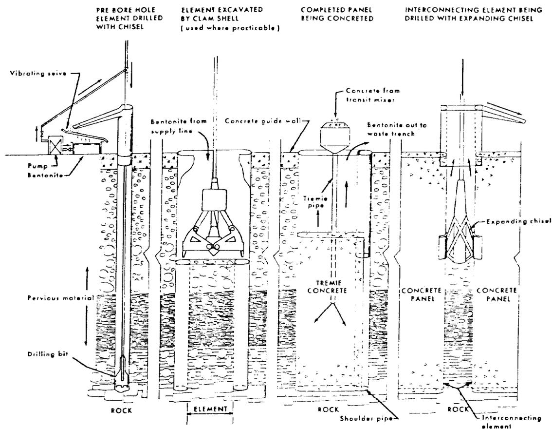
Figure 9-13. Construction procedure for concrete cutoff wall at Kinzua Dam (formerly Allegheny Dam), Pennsylvania (after U. S. Army Engineer District, Pittsburgh<sup>103</sup>)
