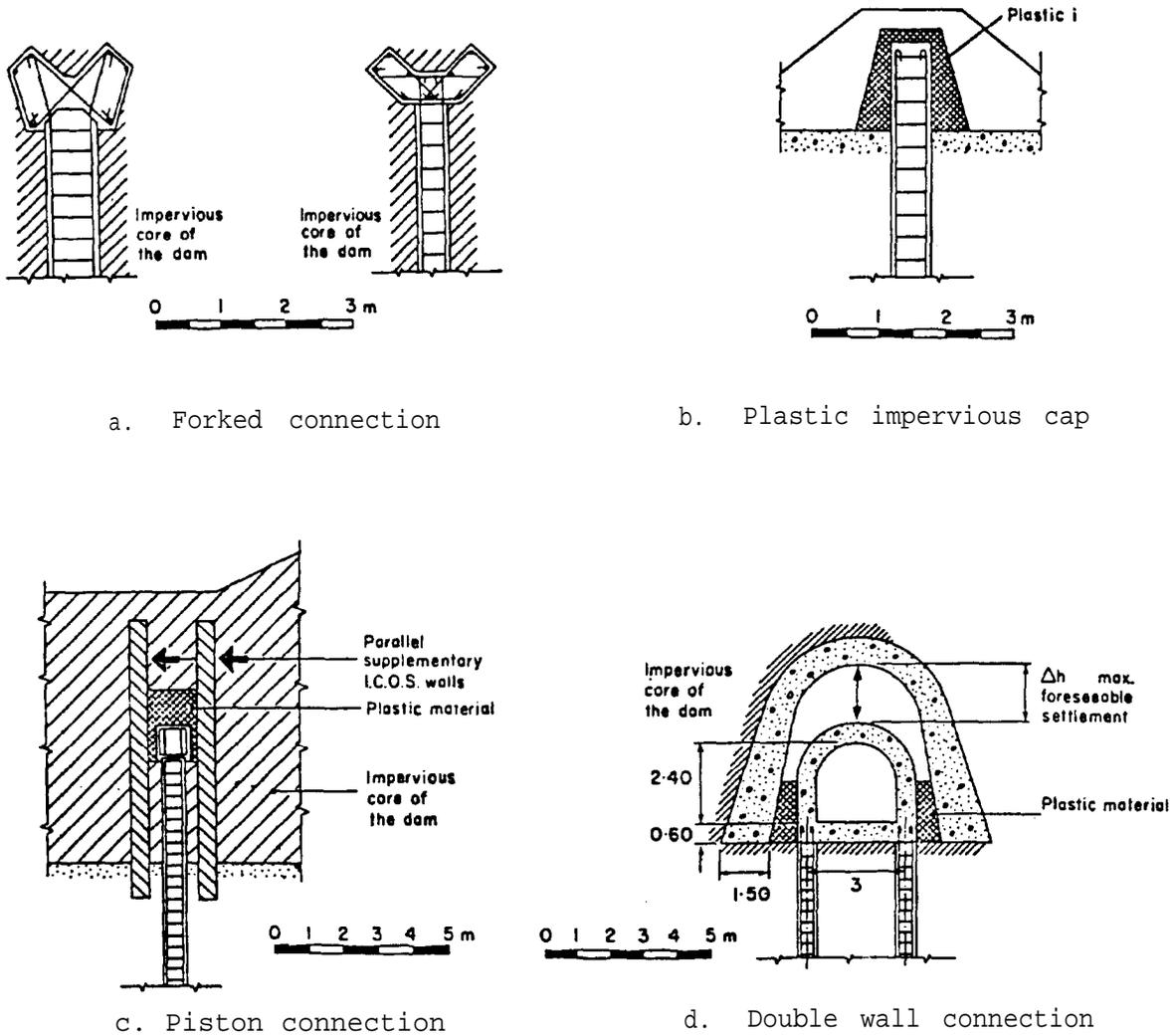
Figure 9-15. Connections between concrete cutoff wall and core of dam (courtesy of ICOS<sup>182</sup>)
