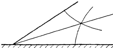
2:1 length ratios to establish shape of the "square" in a pervious foundation at the toe of an impervious fill.
