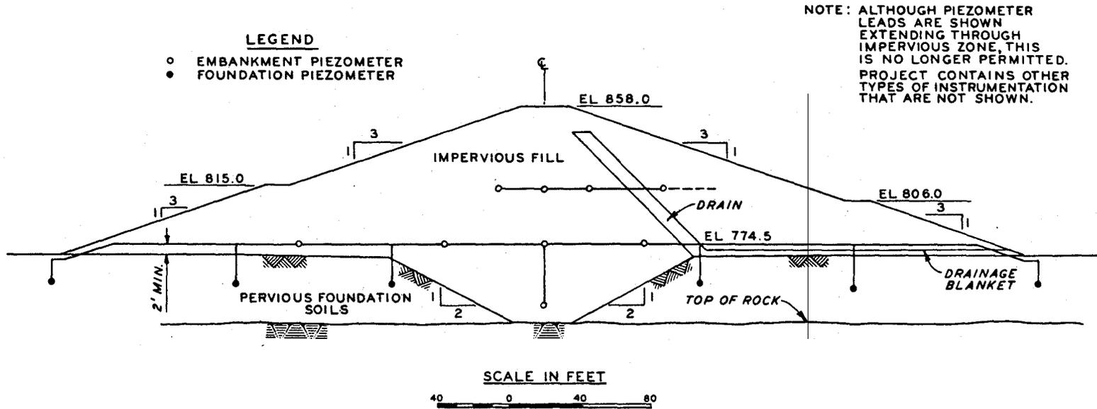
Figure 13-2. Piezometer installation for dams on pervious foundations, Deer Creek Dam (from EM 1110-2-1908)
