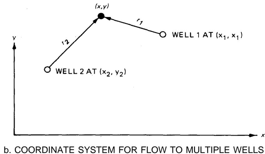
Figure 7-3. Flow to multiple wells (adapted from John Wiley and Sons<sup>164</sup>)
