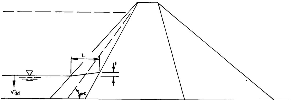
Figure 8-6. Computation of required minimum permeability of the upstream drawdown blanket (courtesy of John Wiley and Sons<sup>155</sup>)
