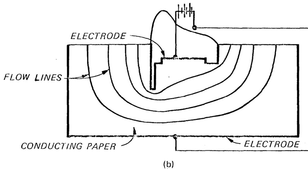
Figure 4-4. Use of two-dimensional conducting paper to find flow lines and equipotential lines (courtesy of John Wiley and Sons<sup>279</sup>)
