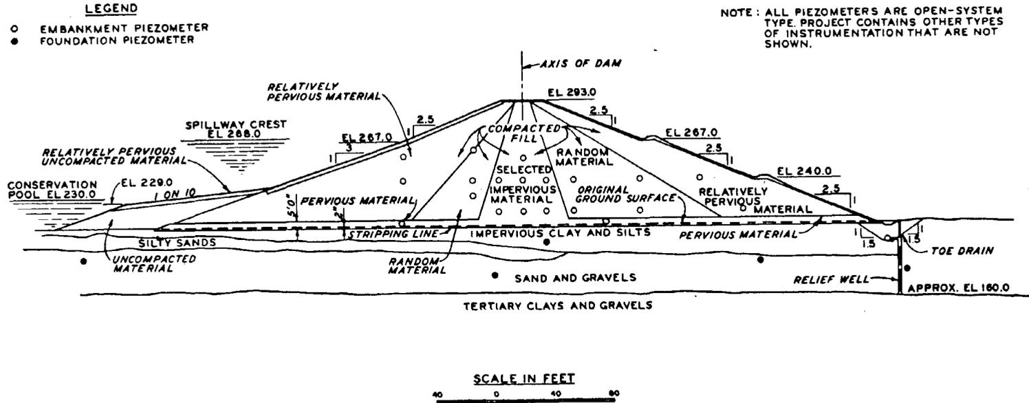
Figure 13-3. Piezometer installation with a thin impervious topstratum and relief well systems, Enid Dam (from EM 1110-2-1908)
