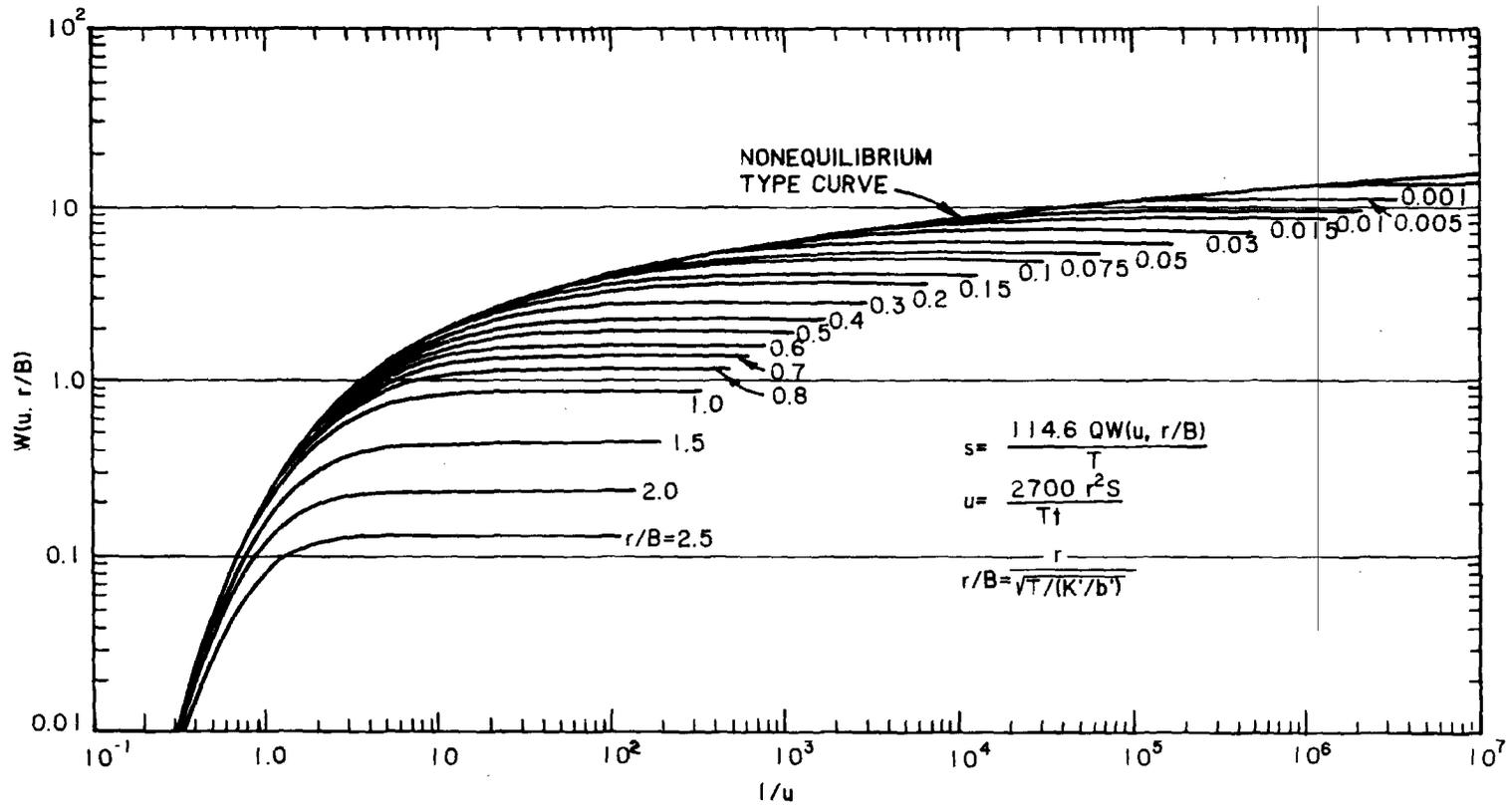
Figure 7-12. Type curve for nonsteady flow in a semiconfined aquifer (courtesy of John Wiley and Sons<sup>164</sup>)
