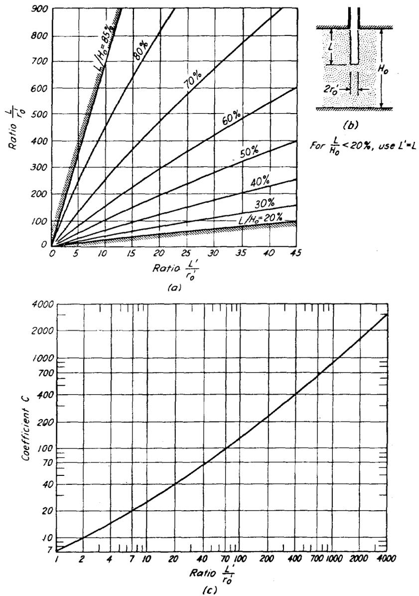
Figure 2-18. Field permeability test in bore hole
