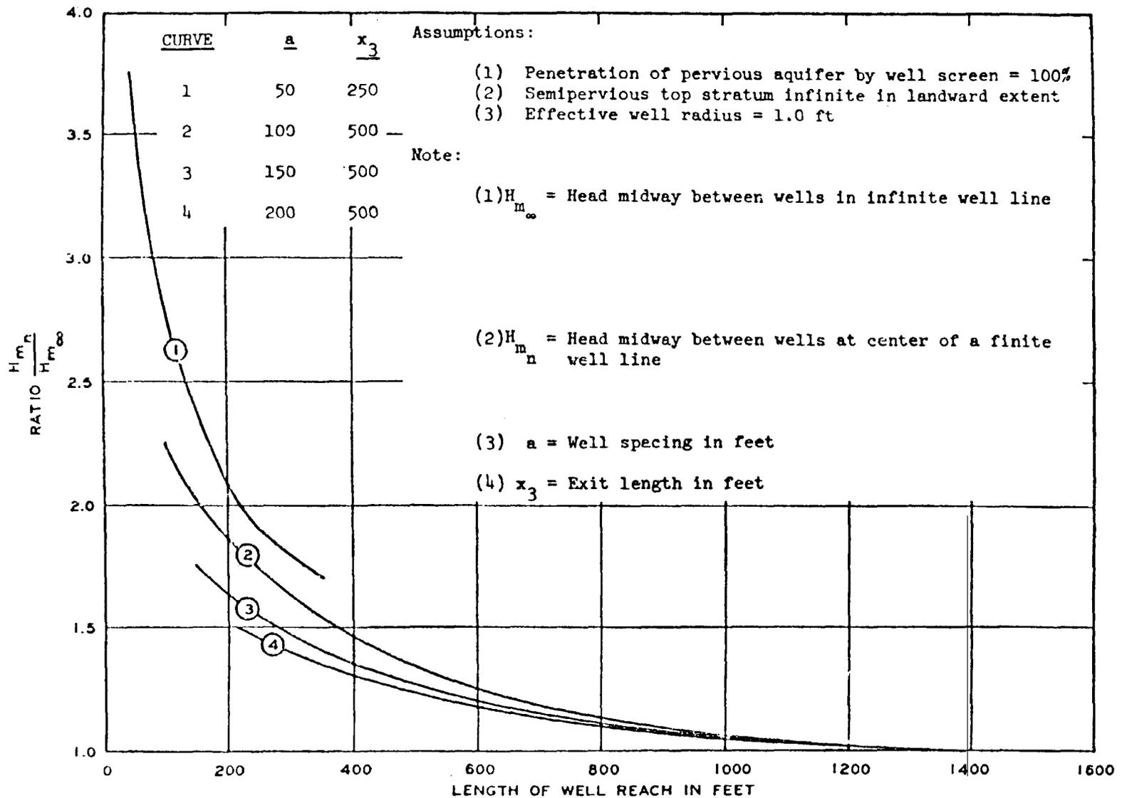
Figure 9-31. Ratio of head midway between relief wells at center of a finite well system to head midway between wells in an infinite system (from U.S. Army Engineer Waterways Experiment Station <sup>120</sup>)
