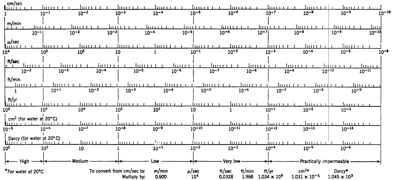
Figure 2-4. Permeability conversion chart (courtesy of John Wiley & Sons, Inc.<sup>201</sup>)
