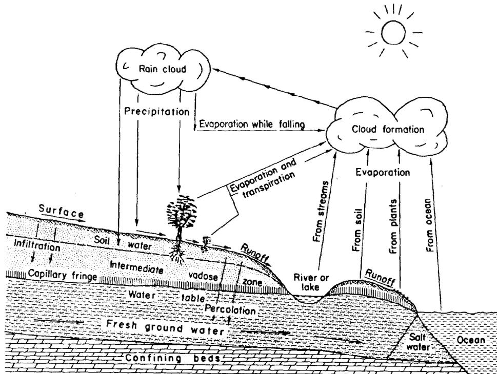
Figure 2-16. Schematic diagram of the hydrologic cycle
