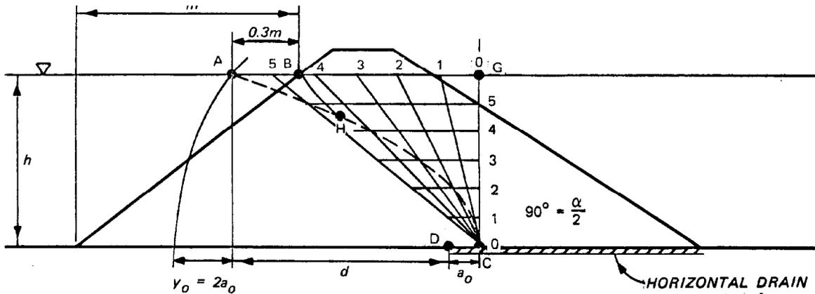
Figure 6-5. Construction of basic parabola and seepage line for  $\alpha = 180^\circ$  Kozeny (courtesy of New England Waterways Association<sup>151</sup>)
