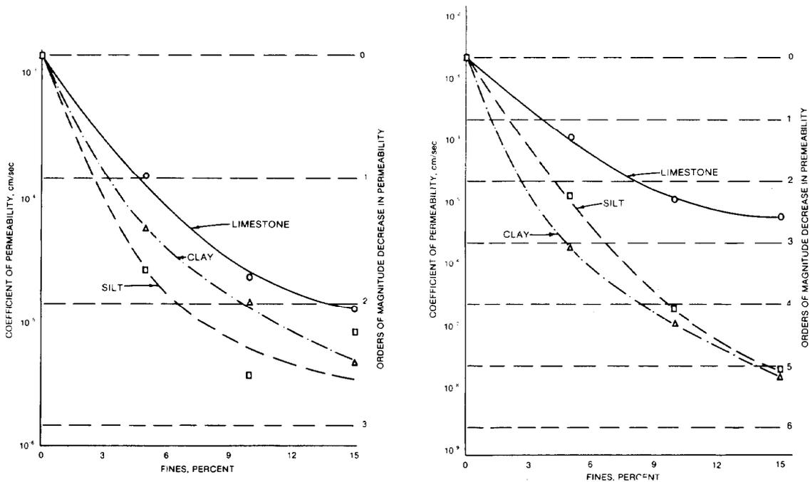
a. Effect of fines on permeability of concrete sand (from Barber and Sawyer<sup>137</sup>)
