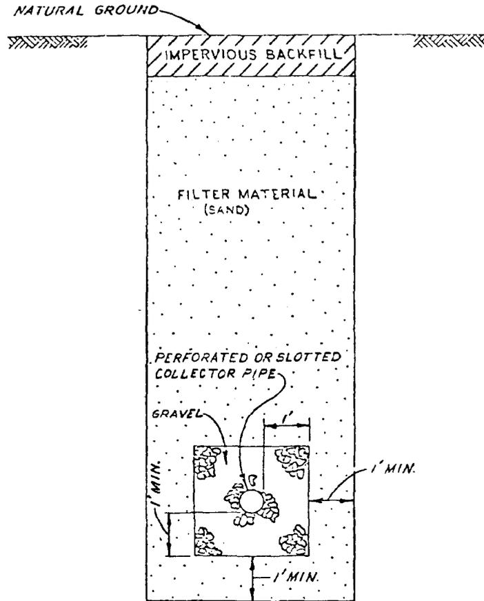
Figure 9-34. Trench drain with collector pipe (from EM 1110-2-1913)
