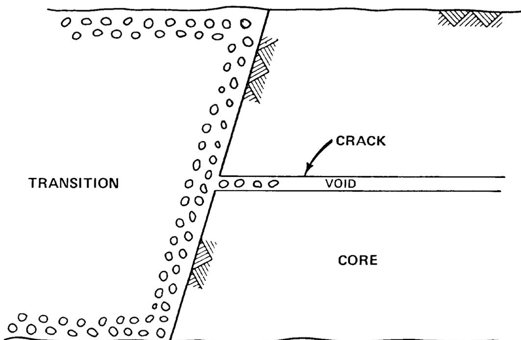
Figure 8-4. Crack stopping transition upstream of a core
