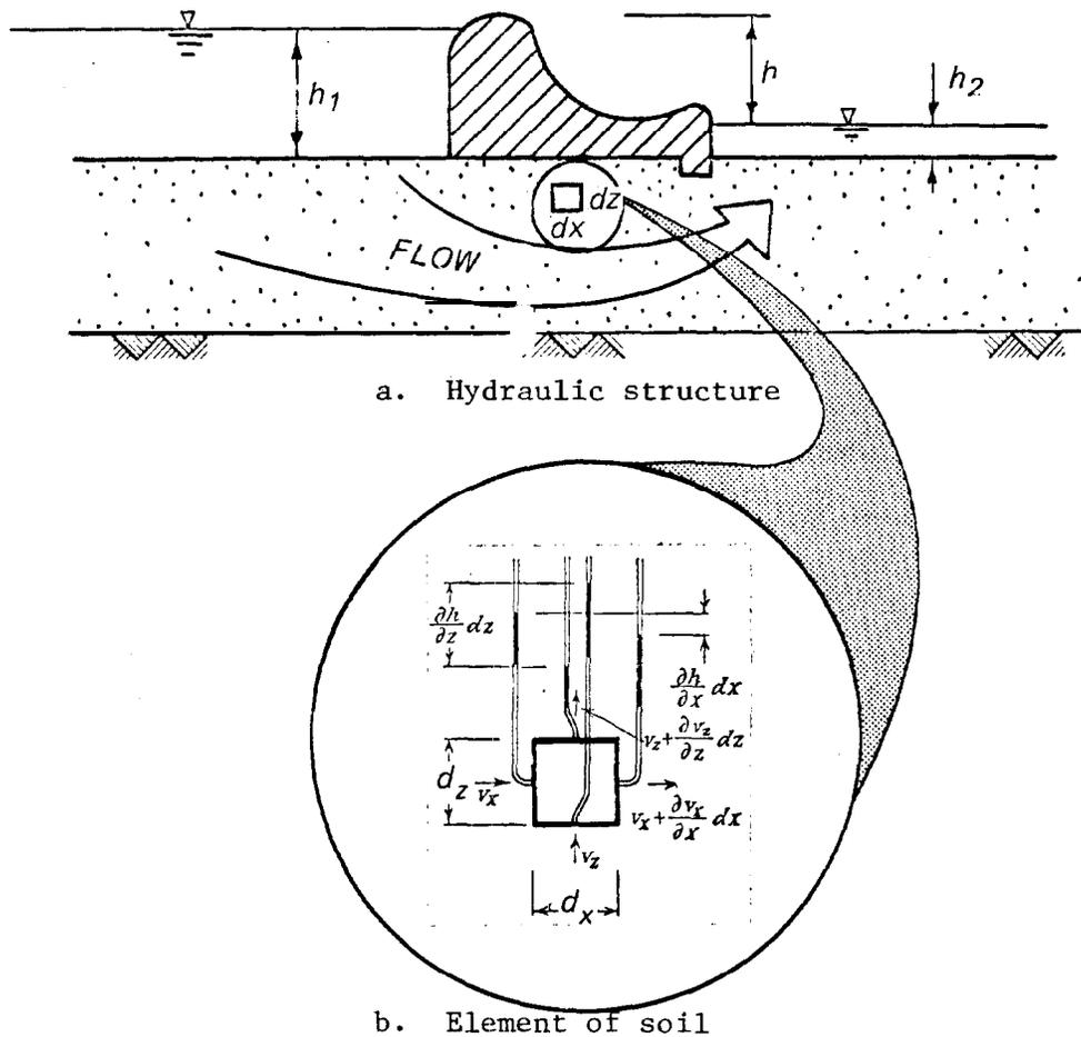
Figure 4-2. Flow of water through saturated pervious soil beneath a hydraulic structure (courtesy of John Wiley and Sons<sup>274</sup>)
