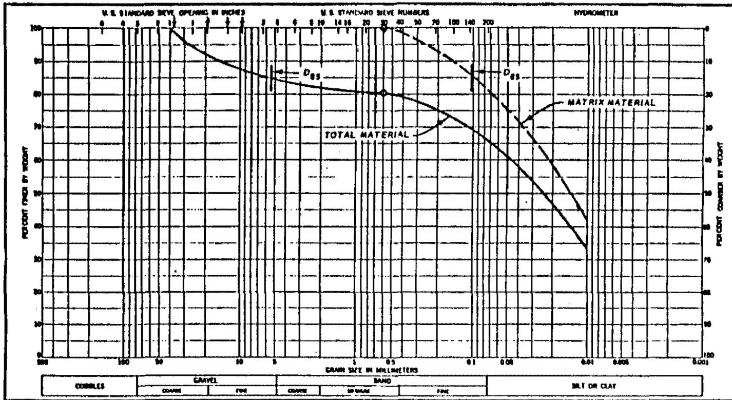
Figure D-1. Analysis of gap-graded material (from EM 1110-2-1913)
