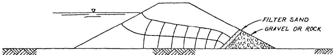
Figure 6-11. Homogeneous embankment on impervious foundation with a toe drain (from EM 1110-2-1913<sup>11</sup>)
