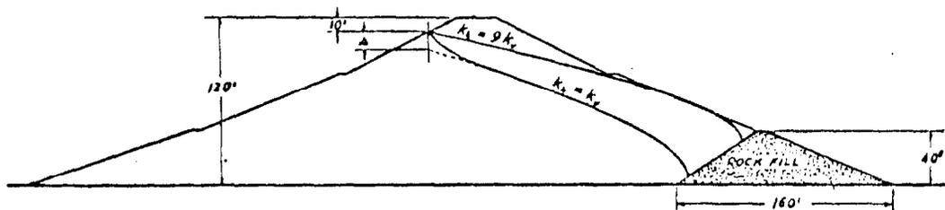
Figure 6-12. Effect of anisotropy for homogeneous embankment on impervious foundation with a toe drain (courtesy of New England Waterworks Association<sup>151</sup>)
