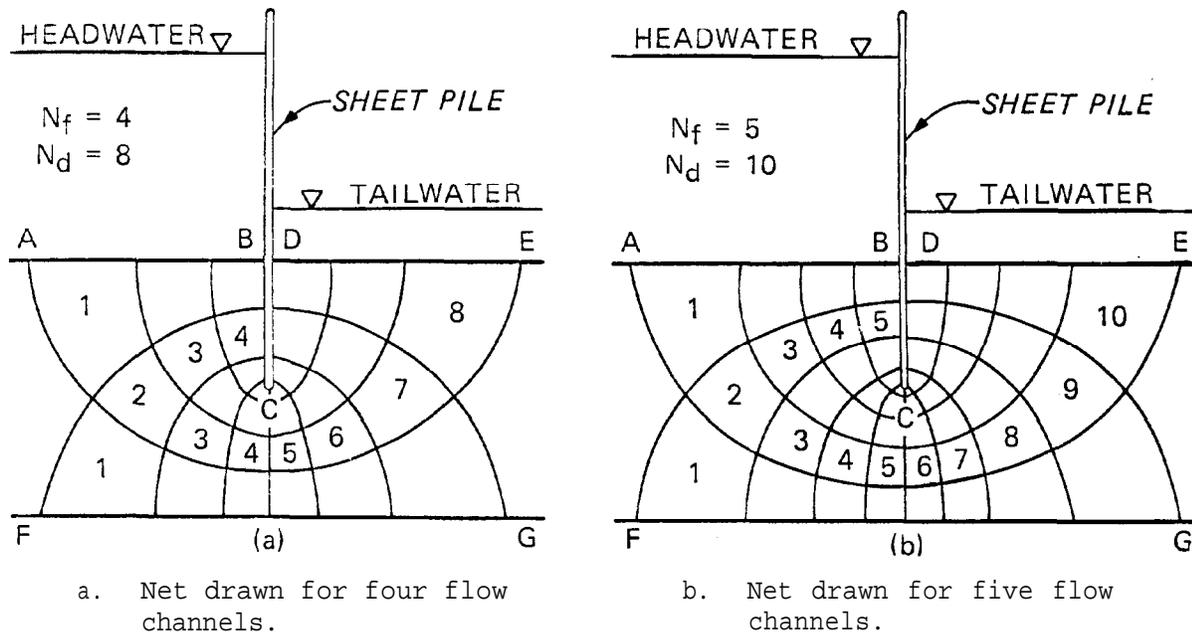
Figure 4-5. Flow net for a sheetpile wall in a permeable foundation (from U. S. Army Engineer District, Little Rock<sup>92</sup>)
