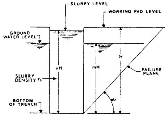
a. Slurry trench typical section
