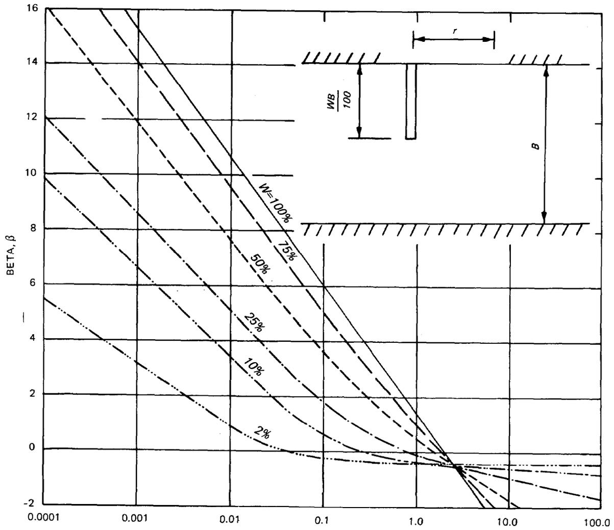
Figure 7-6. Beta function curve (from Warriner and Banks<sup>124</sup>)
