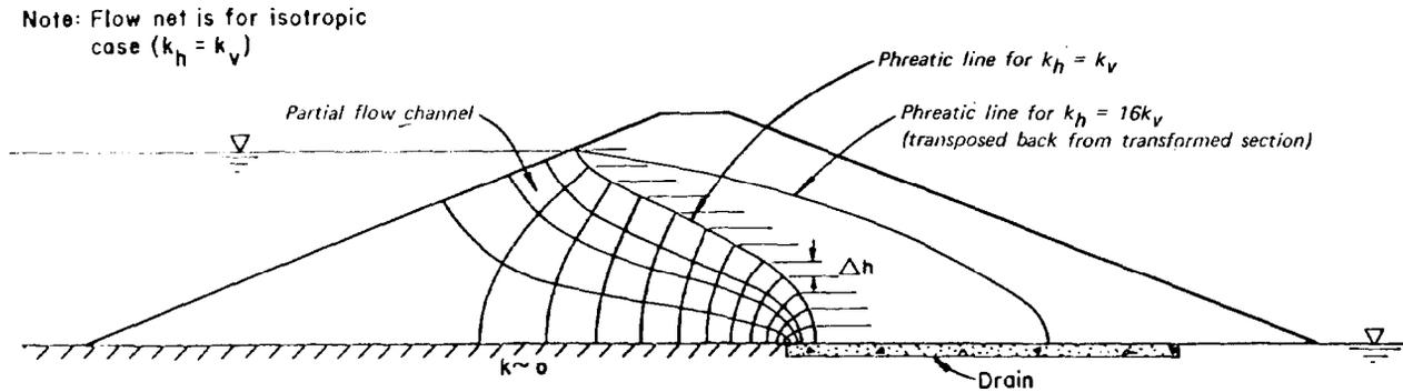
Figure 6-10. Effect of difference in horizontal and vertical permeability (anisotropy) on location of seepage within an embankment with a horizontal drain (after U. S. Department of Agriculture<sup>123</sup>)
