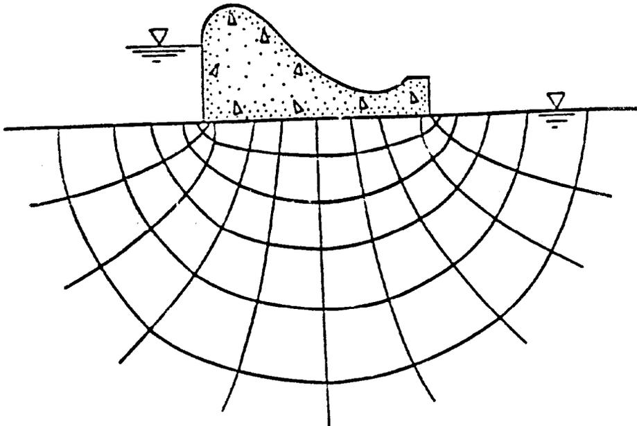
Figure 5-3. Gravity dam on an infinitely deep pervious foundation
