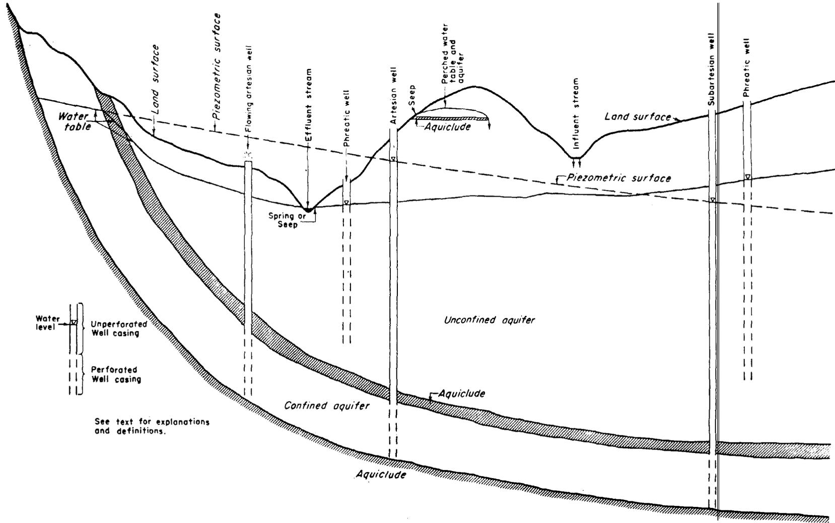
Figure 2-17. Groundwater relationships (courtesy of Soil Conservation Service<sup>68</sup>)
