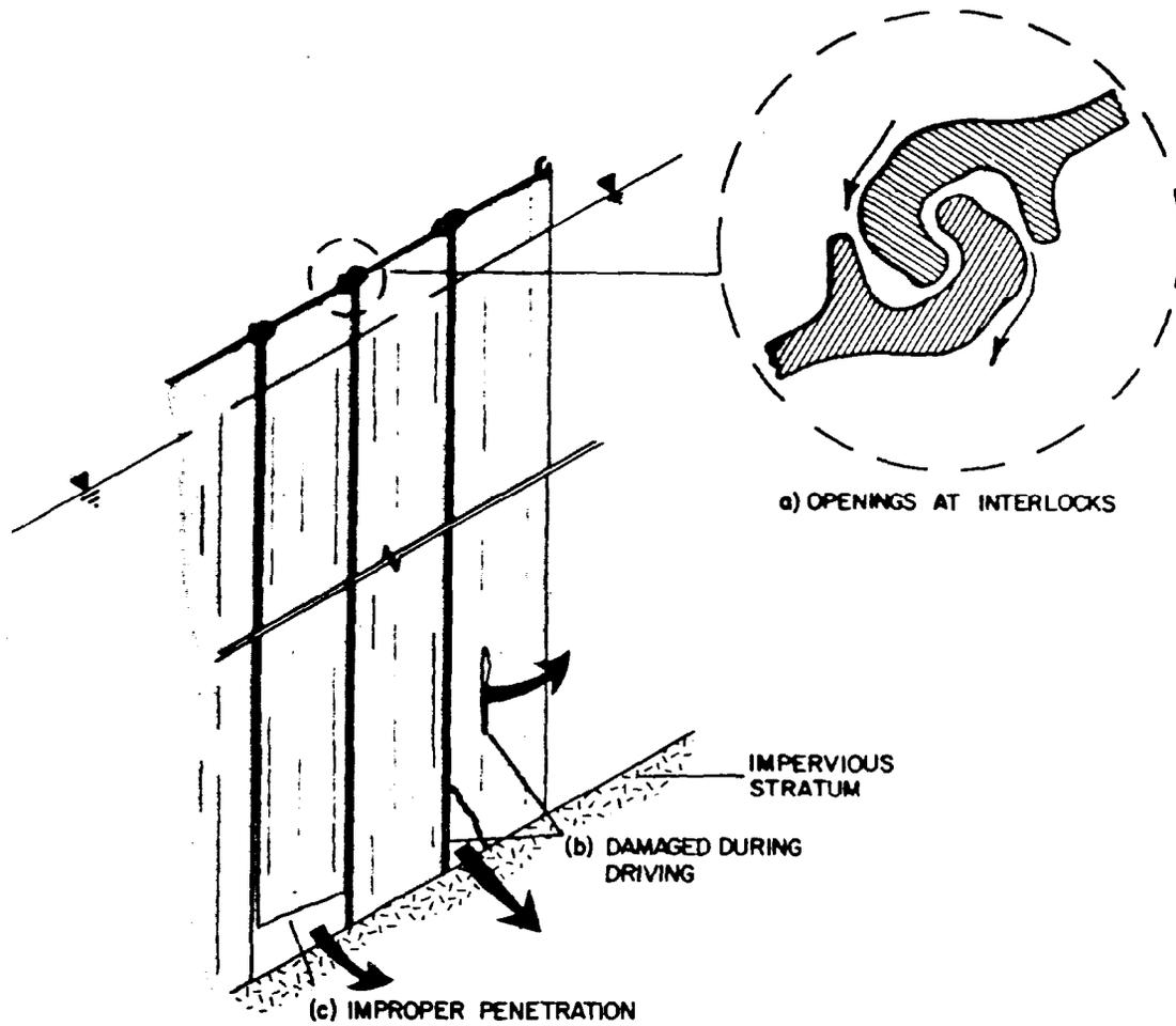
Figure 9-17. Sources of leakage associated with steel sheetpile cutoffs (from U. S. Department of Transportation<sup>41</sup>)
