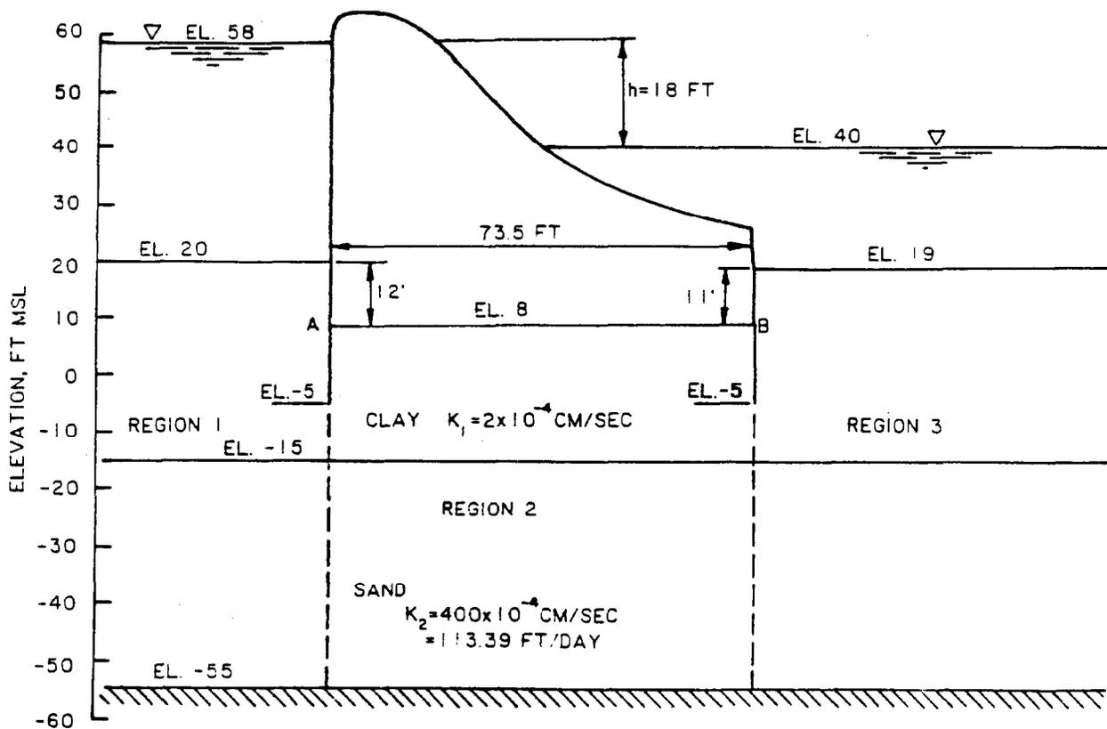
Figure B-19. Transformed section of John B. Overton Dam and stilling basin for one case of sheet pile lengths (from U. S. Army Engineer District, St. Louis<sup>112</sup>)
