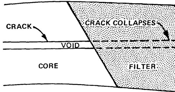
a. Self-healing (by collapse) of filter
