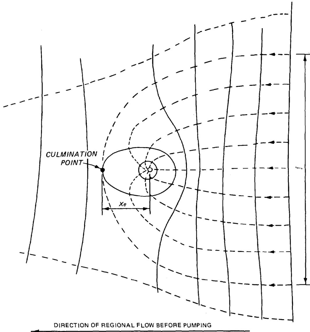
Figure 7-7. Superposition of well drawdown on regional gradient (courtesy of International Institute for Land Reclamation and Improvement<sup>199</sup>)
