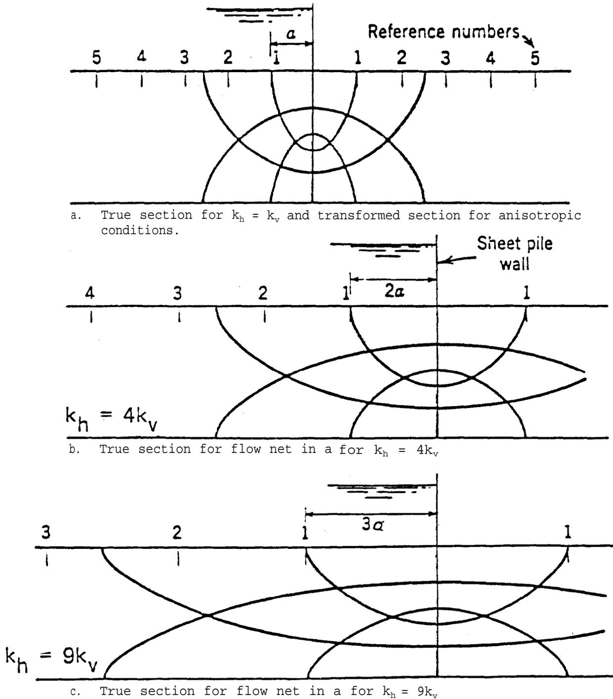
Figure 4-9. Flow nets constructed on transformed section and redrawn on true section (courtesy of John Wiley and Sons<sup>155</sup>)
