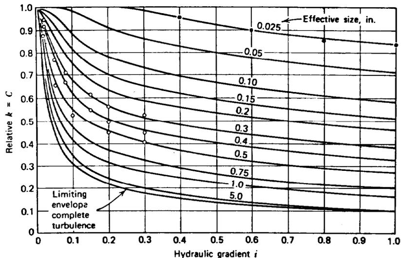
Figure 8-10. Approximation for estimating reduction in permeability of narrow size-range aggregate caused by turbulent flow (courtesy of John Wiley and Sons<sup>155</sup>)
