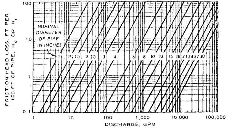
BASED ON HAZEN-WILLIAMS EQUATION WITH C = 100; MULTIPLY LOSSES BY (100/C)<sup>1.85</sup> FOR VALUES OF C OTHER THAN 100
