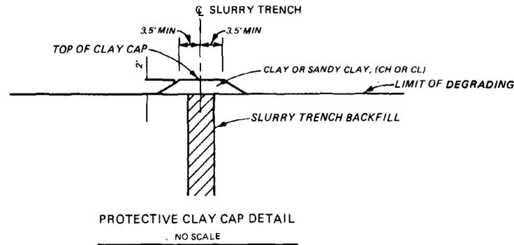
Figure 12-2. Addicks Dams remedial slurry trench for embankment and foundation seepage control (from U.S. Army Engineer District, Galveston<sup>83</sup>)
