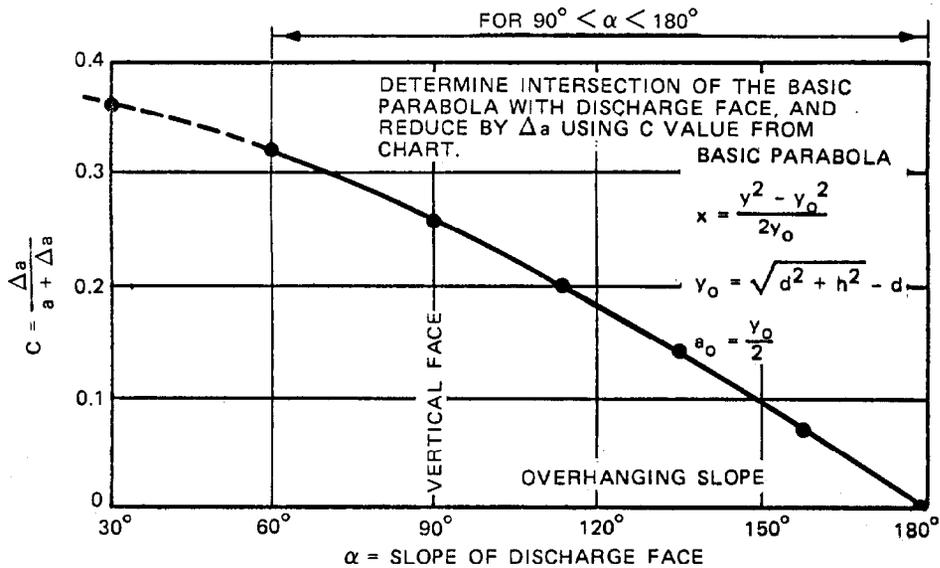
NOTE: POINTS WERE FOUND BY GRAPHICAL DETERMINATION OF FLOW NET.
