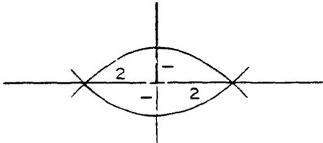
Subdivide to check odd-shaped "squares". Resulting smaller odd-shaped "squares" should have the general shape of the one subdivided.
