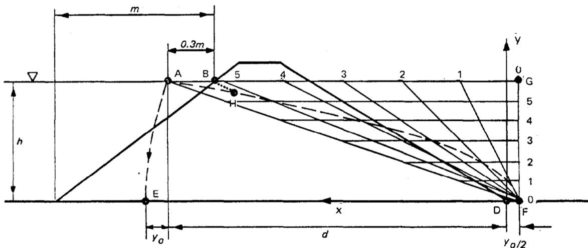
Figure 6-3. Construction of basic parabola (prepared by WES)
