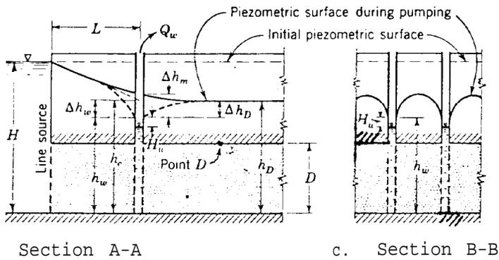
Figure 9-28. Flow to an infinite line of fully penetrating relief wells from an infinite line source of seepage (after Leonards<sup>205</sup>)
