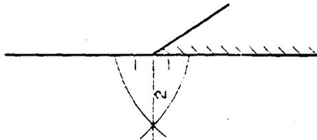
2:1 length ratios used with angle bisectors to shape flow around an imbedded 90-degree angle.
