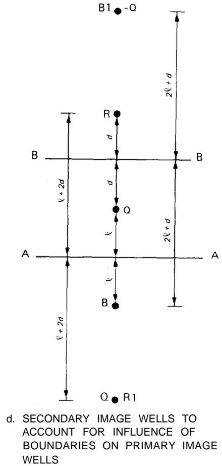
Figure 7-5. Multiple image wells for a two-boundary problem
