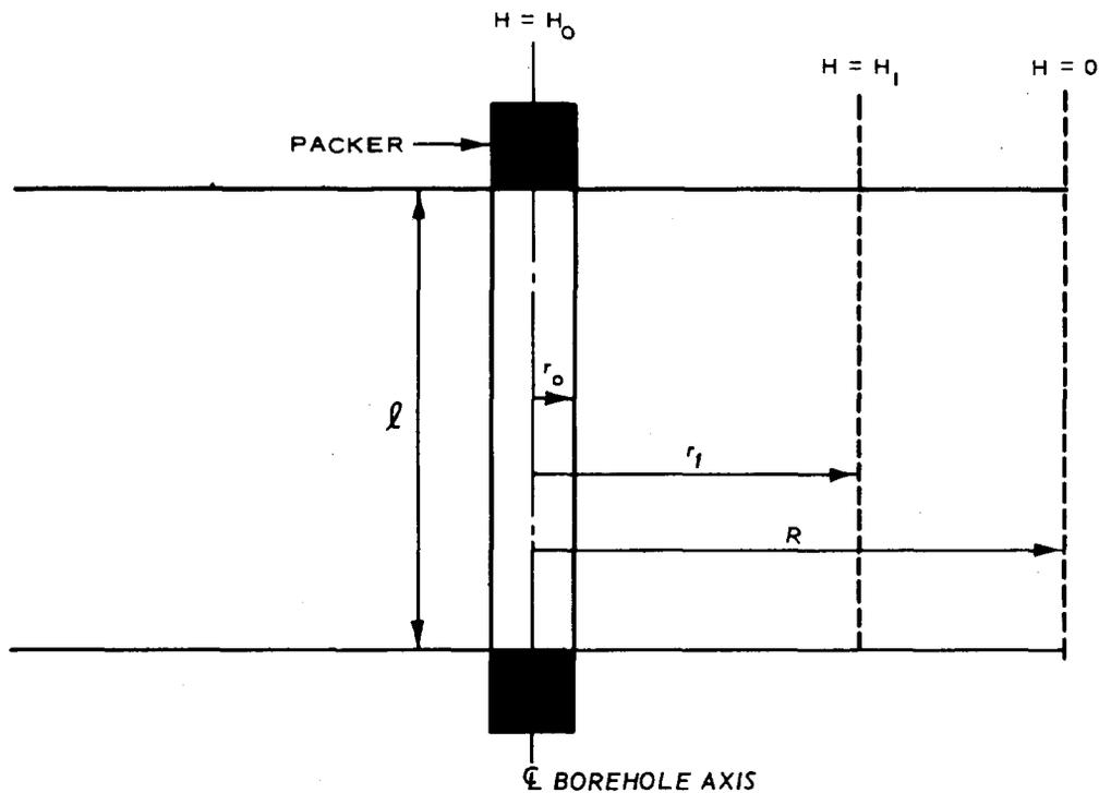
Figure C-2. Homogeneous isotropic material--radial flow
