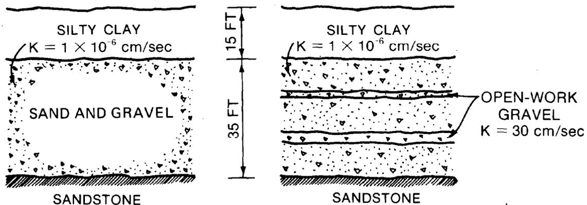
a. Soil profile surmised from drill holes with estimated quantity of seepage under dam equal to 3 cu ft/day
