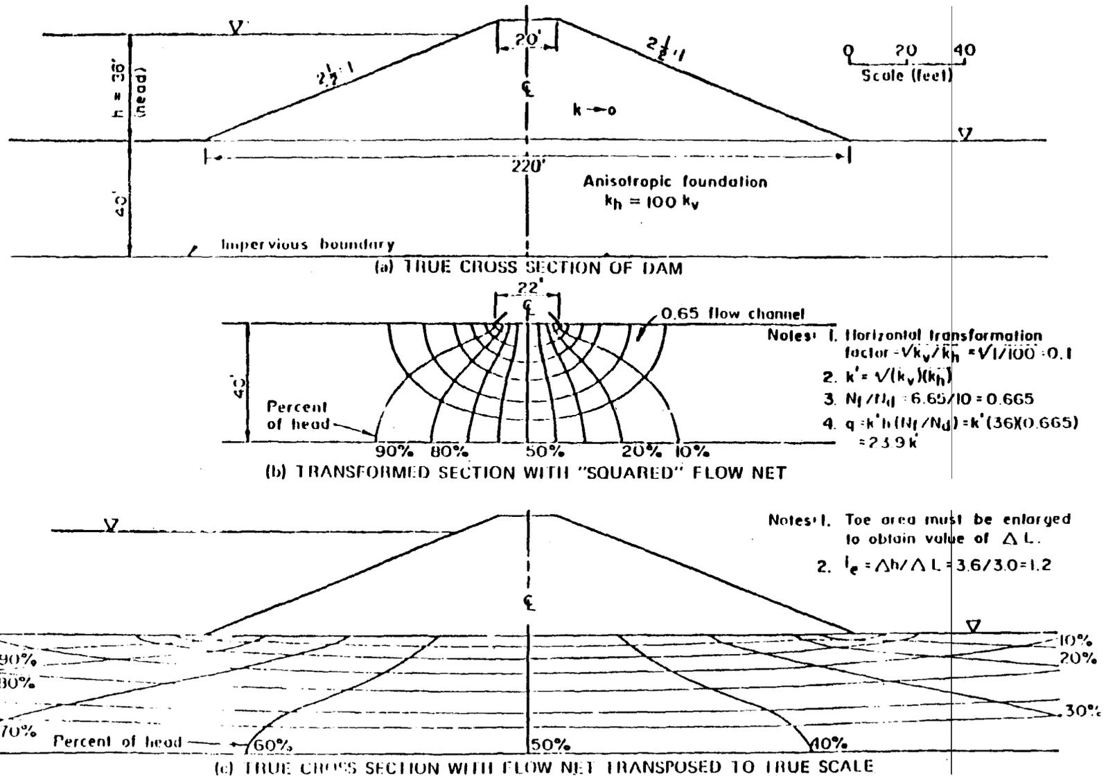
Figure 4-10. Example of technique for developing a flow net for an anisotropic foundation (from U. S. Department of Agriculture<sup>123</sup>)
