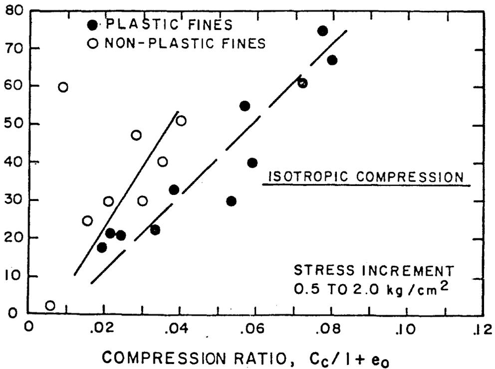
Figure 9-11. Relationship between fines content and compressibility of a soil-bentonite slurry trench backfill (courtesy of American Society of Civil Engineers<sup>163</sup>)
