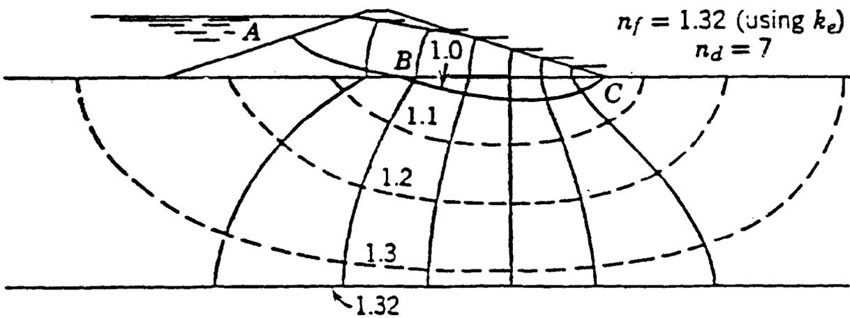
c. Adjust flow net until balanced.
