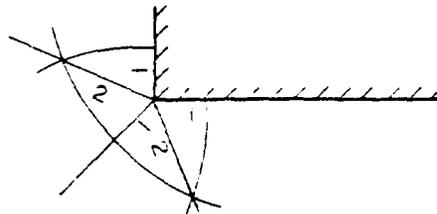
2:1 length ratios to establish flow directions beneath a thin cutoff wall taken to the midpoint of the pervious stratum.
