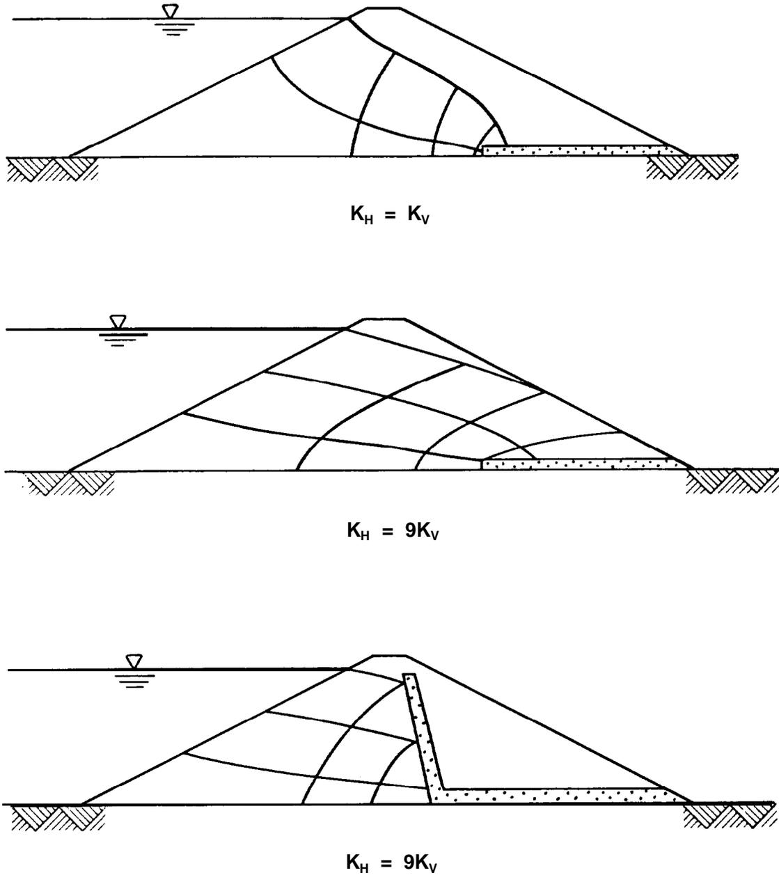
Figure 8-8. Effect of anisotropy of permeability on seepage through earth dam with and without an inclined drain (courtesy of John Wiley and Sons<sup>155</sup>)
