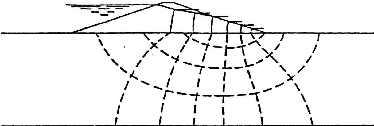
b. External equipotential lines into foundation without adjusting lines of net in dam.
