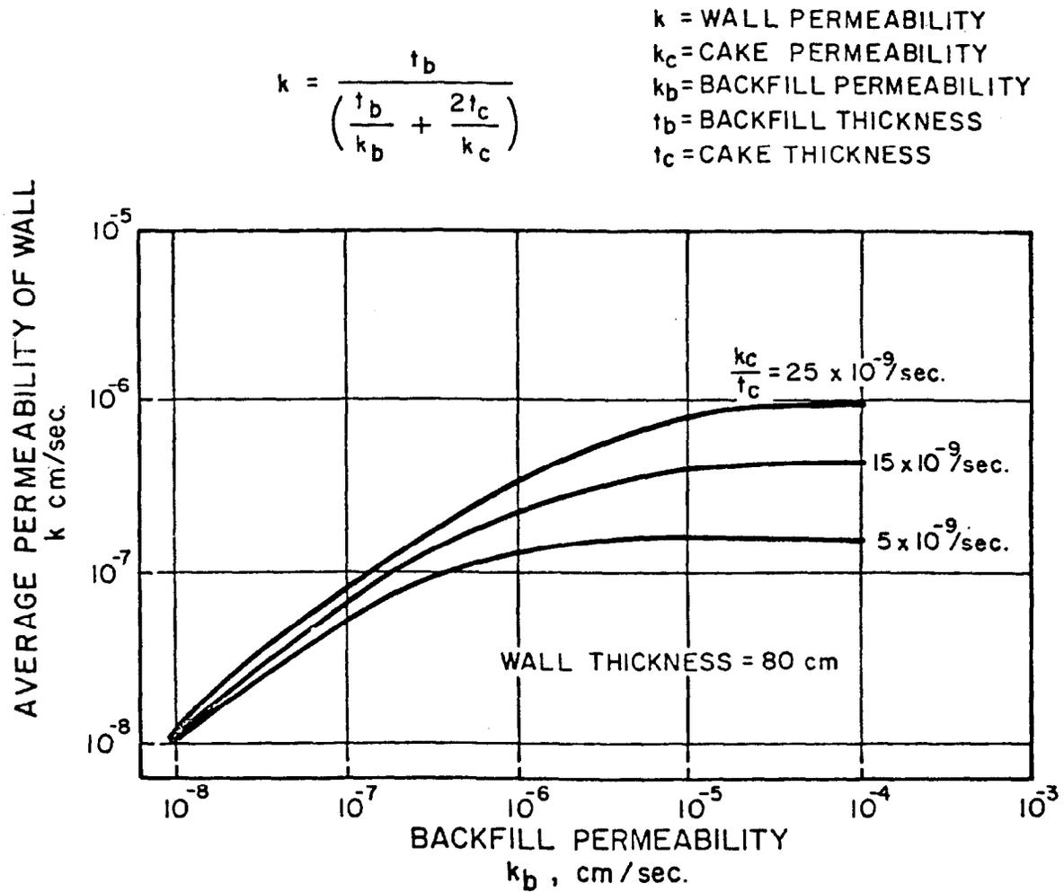
Figure 9-10. Permeability of a soil-bentonite slurry trench cutoff wall 80 cm thick for various values of backfill and filter cake permeability (courtesy of American Society of Civil Engineers<sup>163</sup>)
