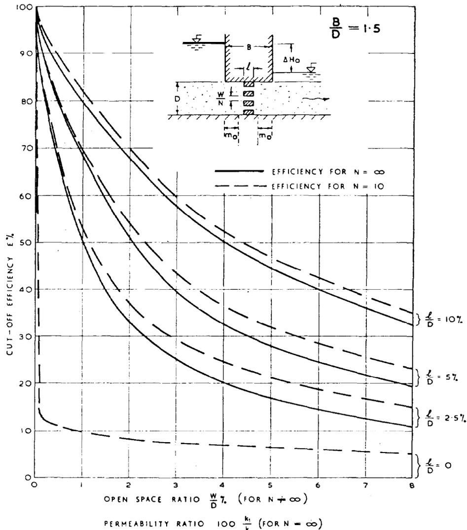
Figure 9-18. Cutoff efficiency versus open space ratio for imperfect cutoffs (courtesy of Butterworths, Inc. <sup>129</sup>)
