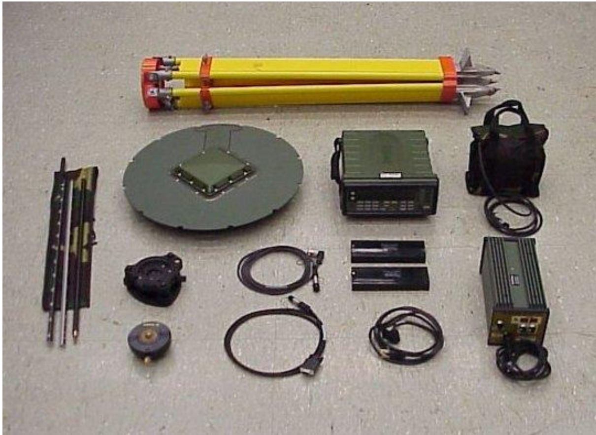
Figure 3-5. Standard GPS equipment for precise surveying. From left to right: graduated rods for antenna height measurement, GPS antenna with ground plane, tribrach, antenna/tribrach adapter, antenna cable, data download cable, surveyors tripod, GPS receiver, camcorder batteries, power cord for support module, 12V battery with attached cable, and support module for data downloading.
