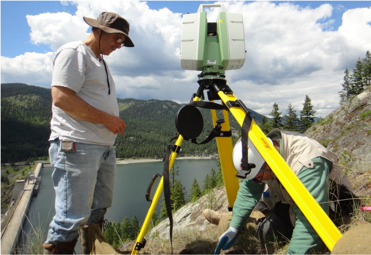
Figure 3-2. Real-time laser scanner being set up to scan Libby Dam. (Army Geospatial Center, Leica Geosystems).
