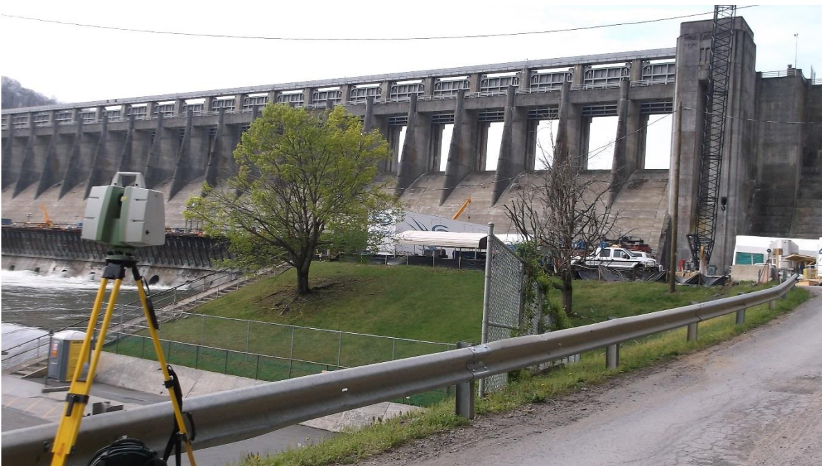
Figure 10-1. A Leica C10 scanner set up for use on a project (USACE Huntington District).
