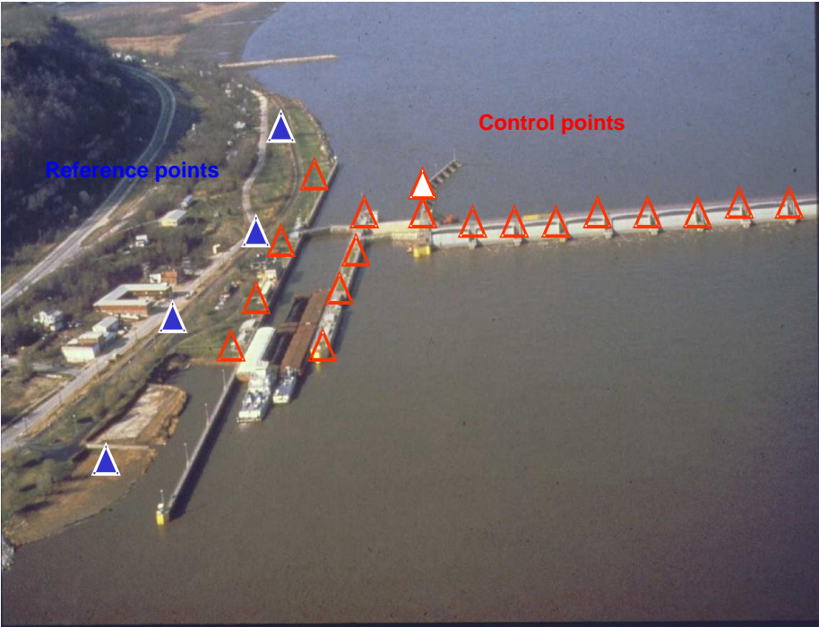
Figure 2-5. Idealized monitoring scheme for controlling target points on the lock and dam.
