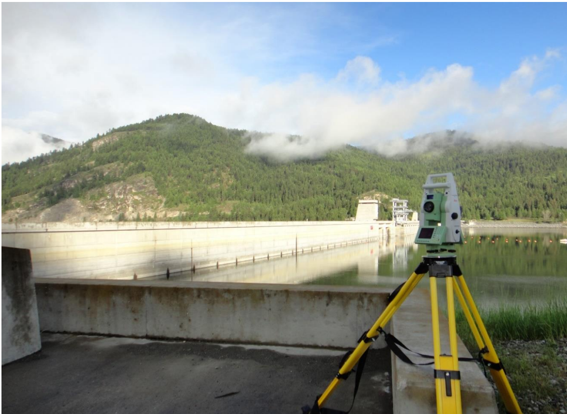
Figure 5-2. EDM observations with a total station at Libby Dam. (from USACE AGC).
