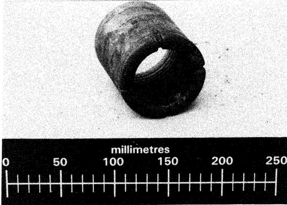
Figure 3-16. Photograph of a typical diamond coring bit
