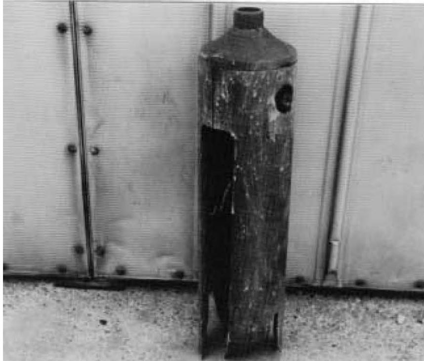
Figure 7-3. Photograph of the McCart split barrel-type auger
