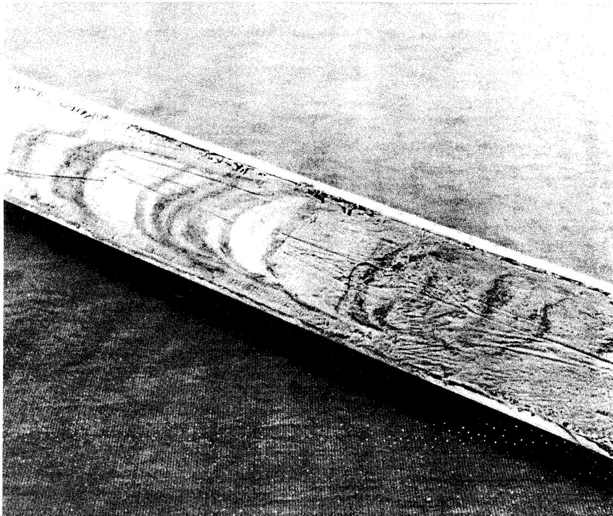
**Figure 10-15. Photograph of a disturbed vibratory core. Note that the thin horizontal layers of dark sediment are curved downward due to sampling disturbance. (Figure provided by the U.S. Naval Facilities Engineering Service Center)**
