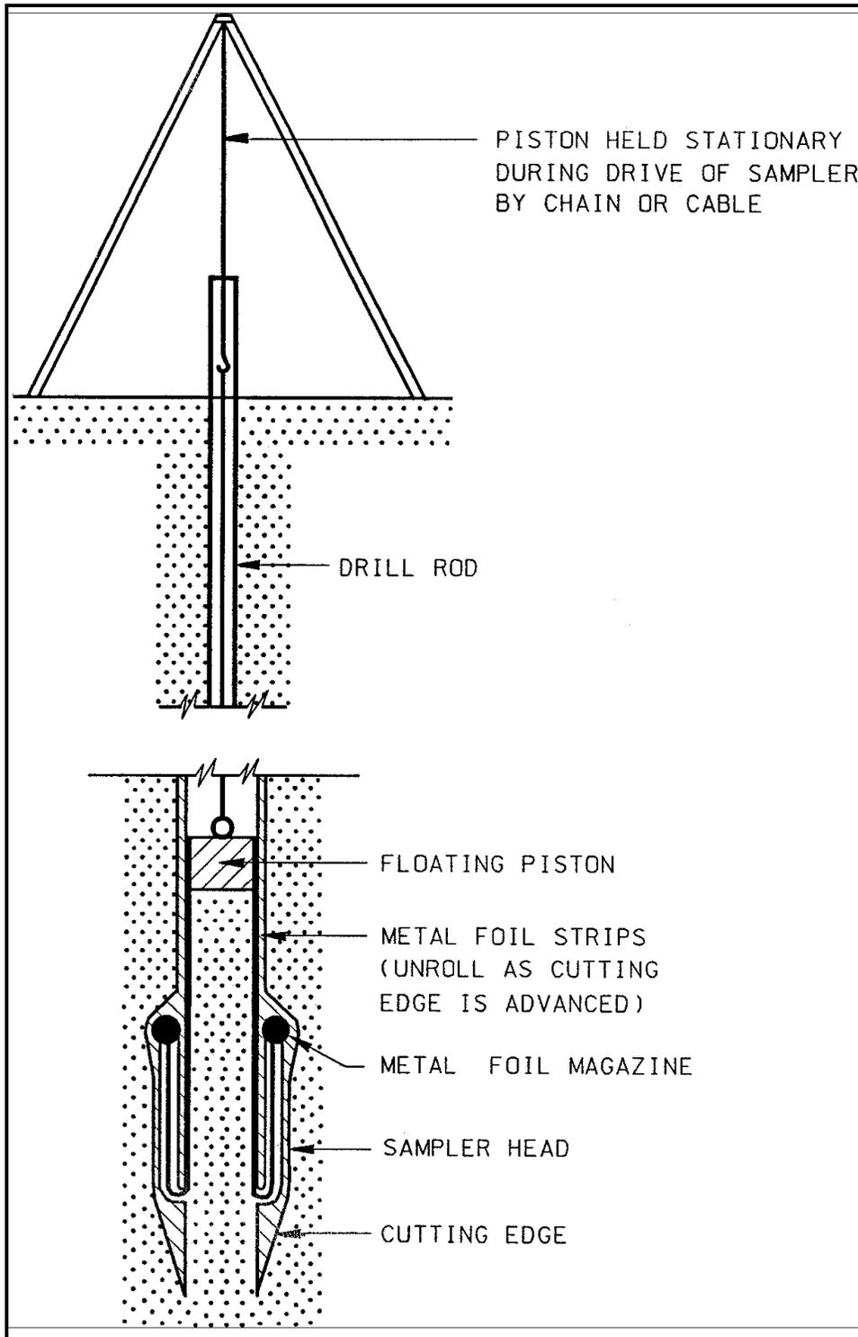
Figure 5-9. Schematic diagram of the Swedish foil sampler
