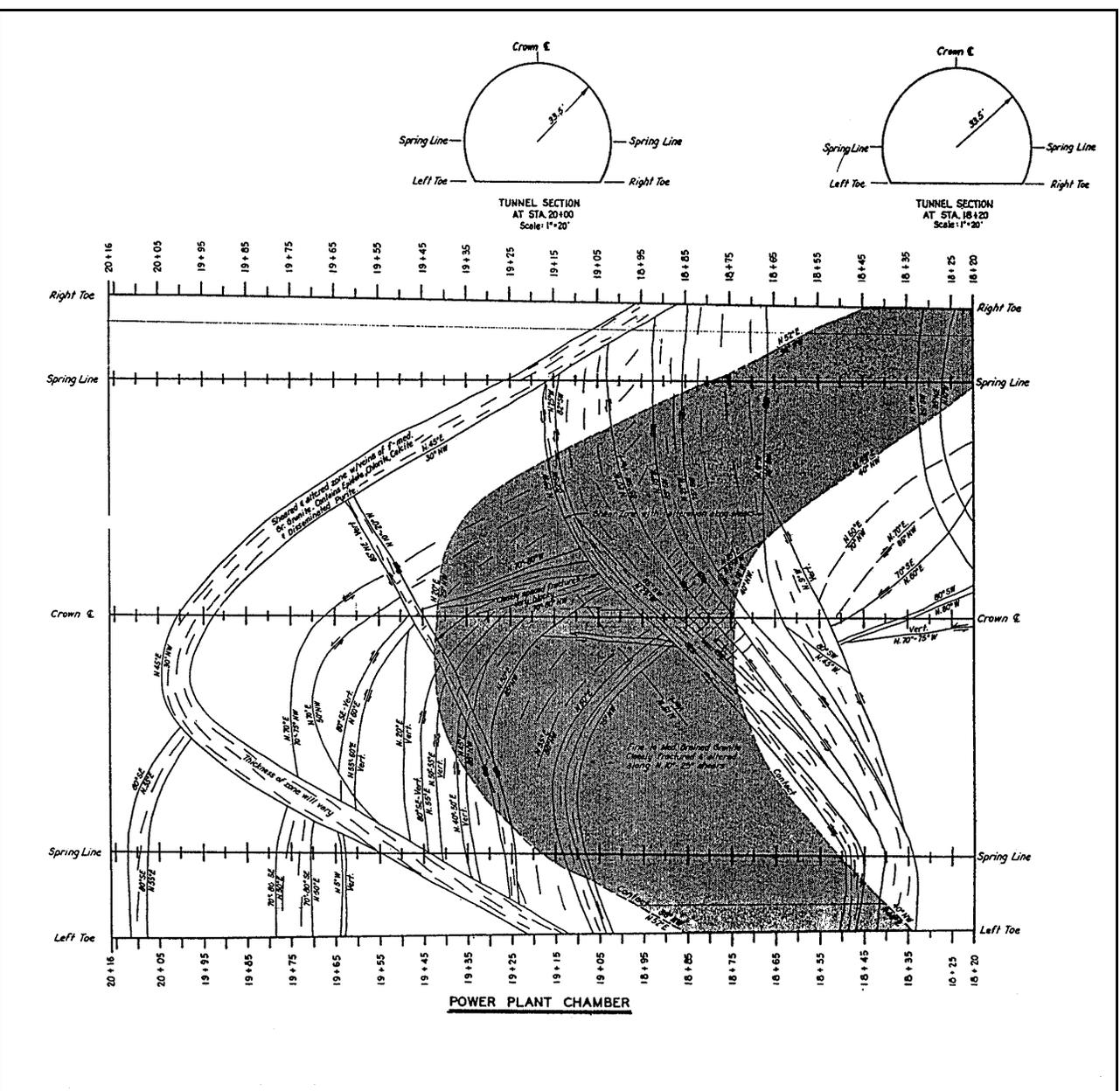
Figure C-9. Developed plan of a horseshoe-shaped large-diameter drift
