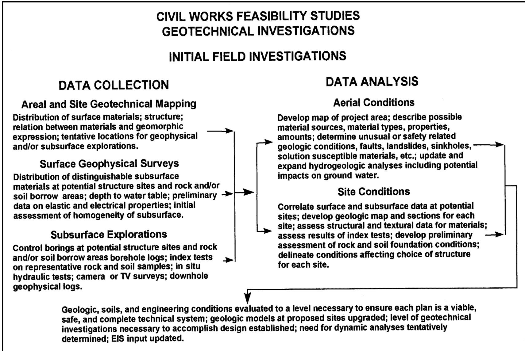
Figure 2-2. Schematic diagram of initial field investigations
