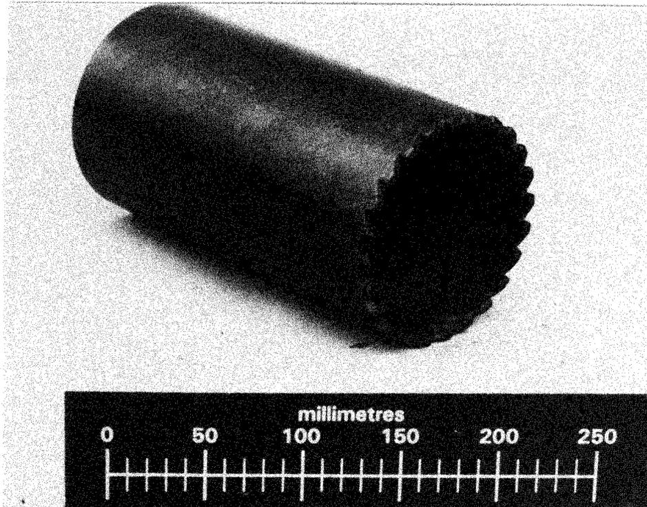
Figure 3-18. Photograph of a sawtooth coring bit
