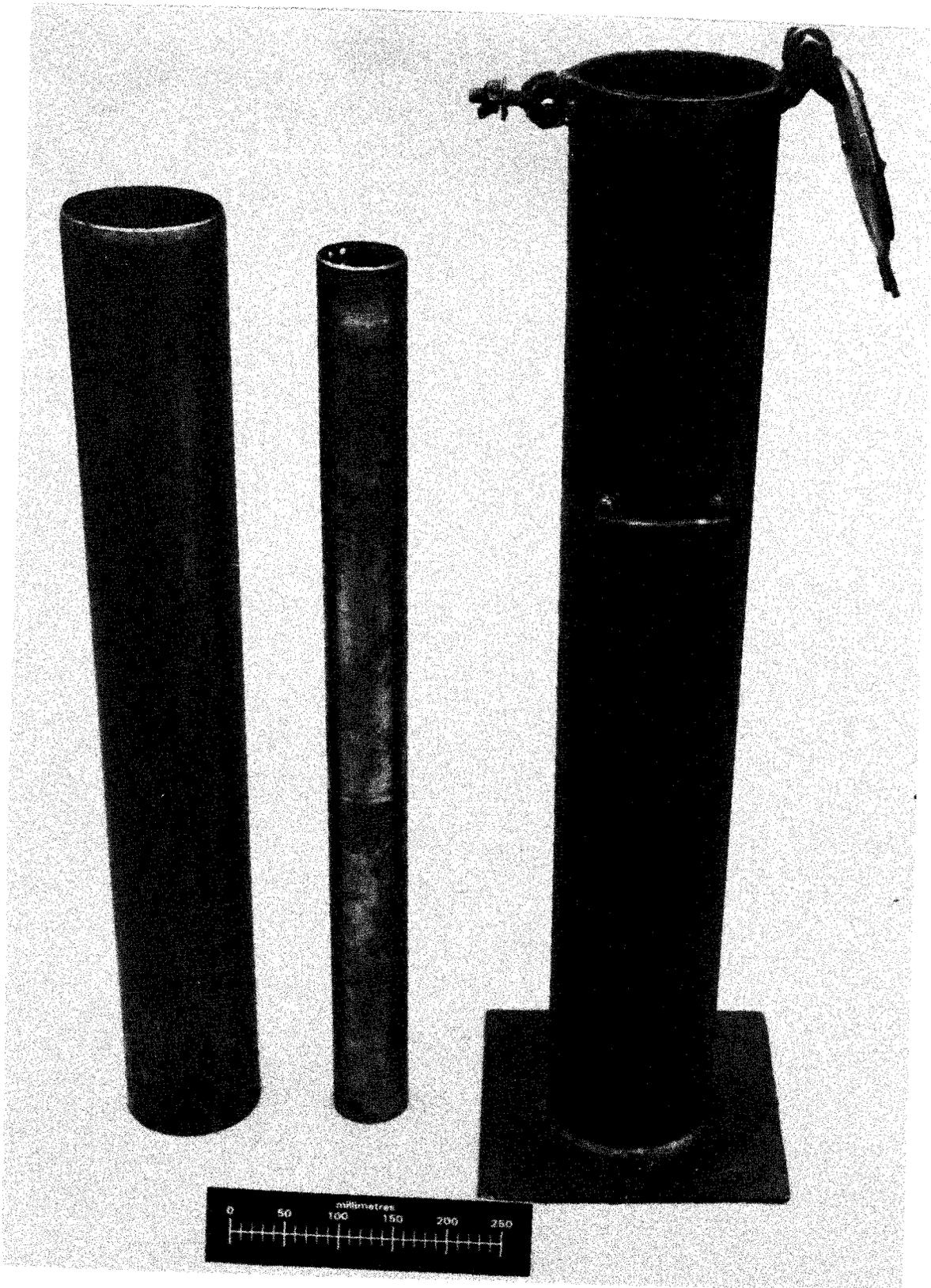
Figure 5-21. Photograph of a dipping tank for coating 75-mm- (3-in.-) and 125-mm- (5-in.-) diam sampling tubes
