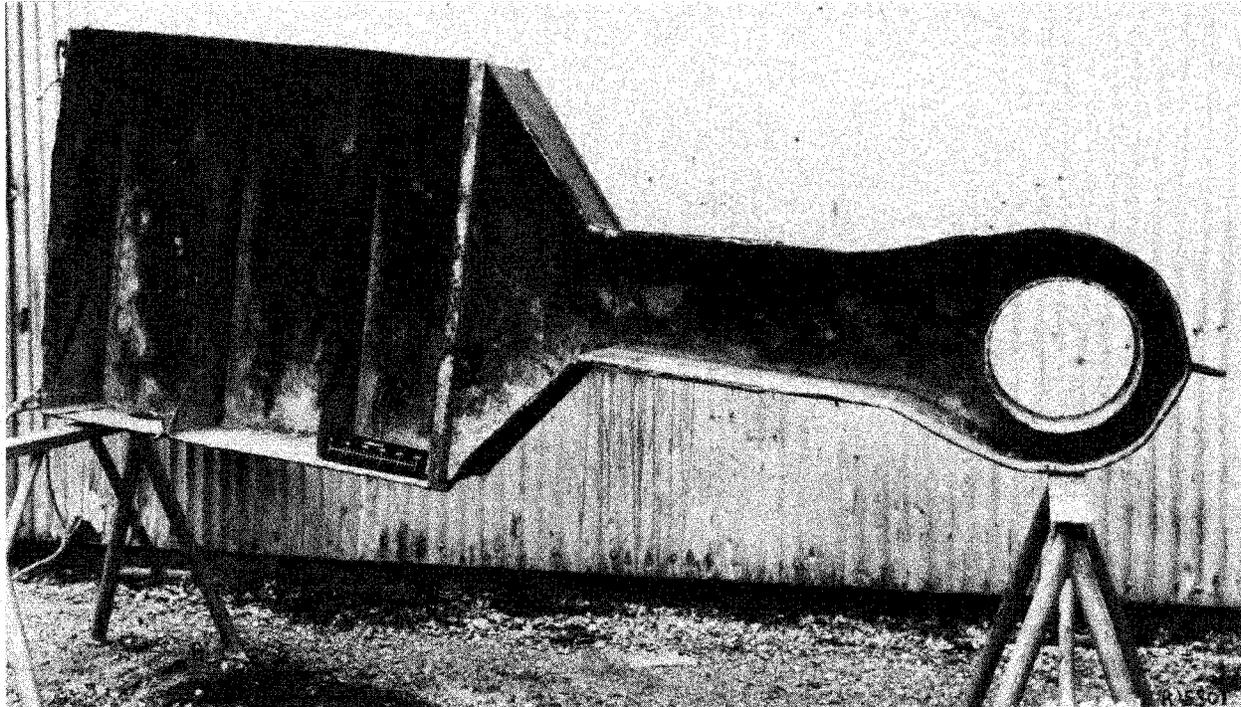
Figure 4-6. Photograph of a portable mud pit
