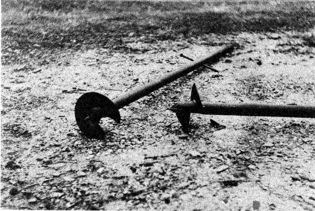
Figure 6-1. Photograph of a screw-type earth anchors
