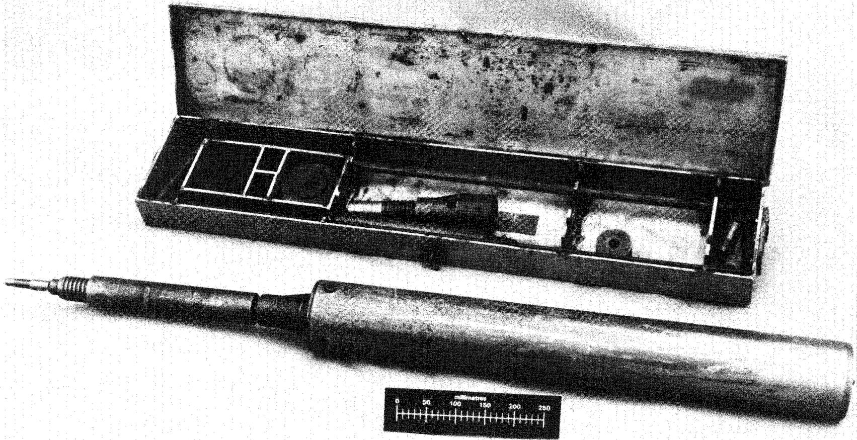
Figure 5-3. Photograph of the Hvorslev fixed-piston sampler
