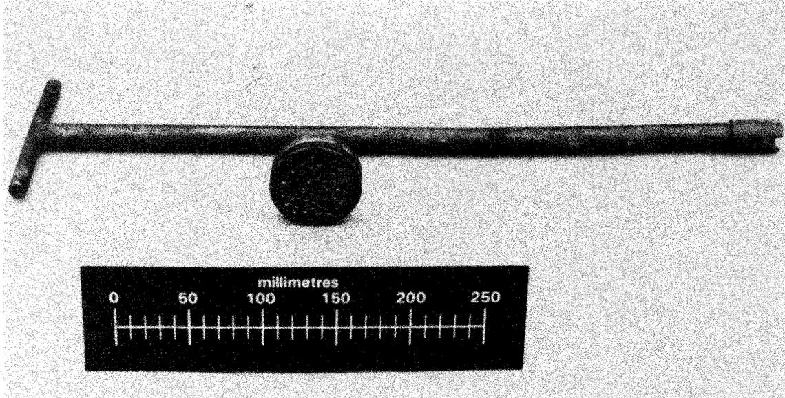
Figure 6-5. Photograph of a perforated, expandable packer
