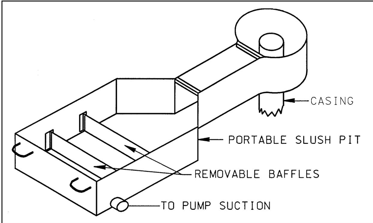
Figure 4-5. Sketch of a portable mud pit
