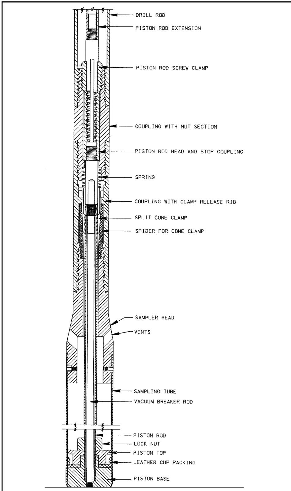
Figure 5-4. Cross-sectional view of the Hvorslev fixed-piston sampler
