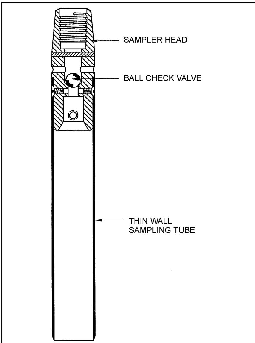
**Figure 5-1. Schematic drawing of an open-tube sampler**
