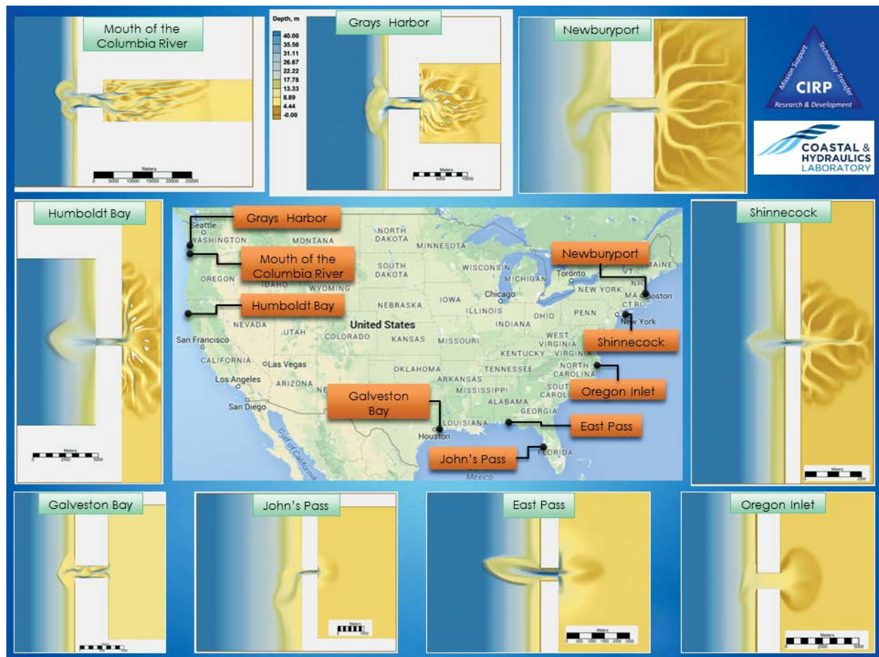
Figure 24. Example of CIRP product illustrating long-term numerical model applications for idealized coastal inlets from the United States' East, West, and Gulf Coasts.
