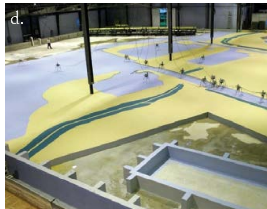
Figure 27. a.) Hurricane Katrina, as a category 5 hurricane (September 2005) bearing down on the Gulf Coast of Louisiana and Mississippi. b.) Storm surge in the New Orleans Inner Harbor Canal and flooding of the 9th Ward. c.) Mapping of flood levels in New Orleans. d.) Physical model study of the 17th St. Canal.
