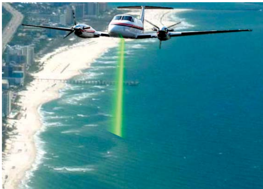
Figure 22. Airborne LIDAR bathymetric mapping system, operated by the JALBTCX, uses topographic and bathymetric lidar and hyperspectral imagery to measure the coastal zone around the U.S.
