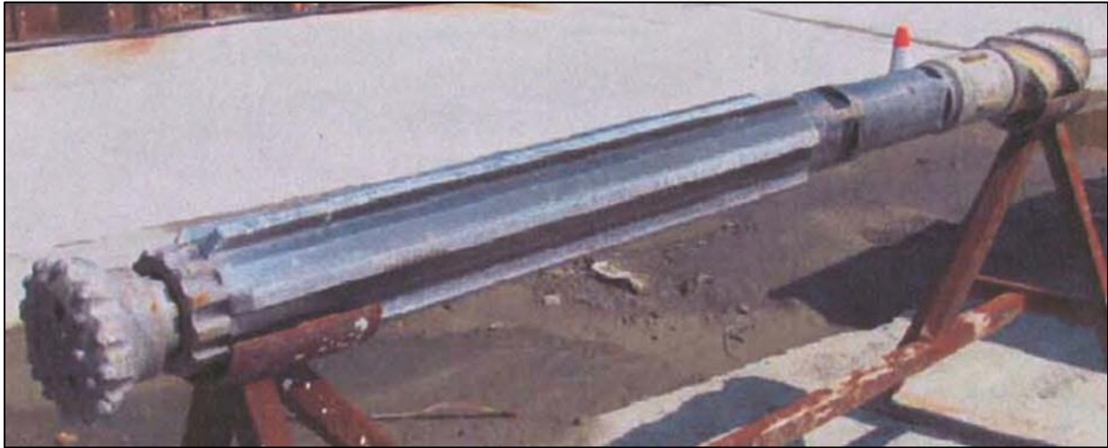
Figure 4-6. Large Water Hammer Down Hole Drill.
