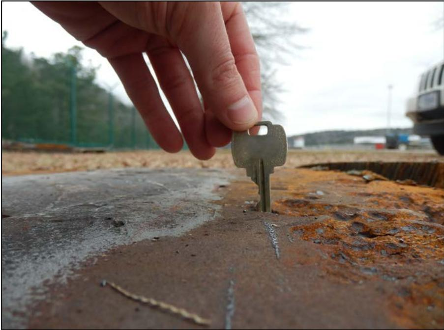
**Figure B-2. Cavitation damage on downstream face of skin plate at Bankhead Lock valve.**
