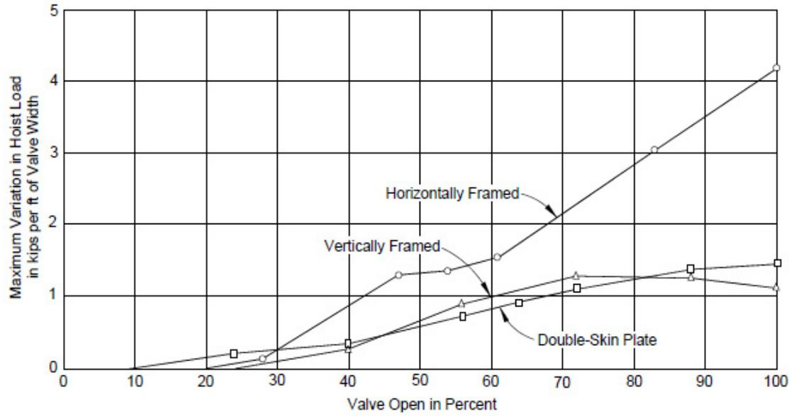
Figure 3-6. Total hoist loads, 60-ft lift.
