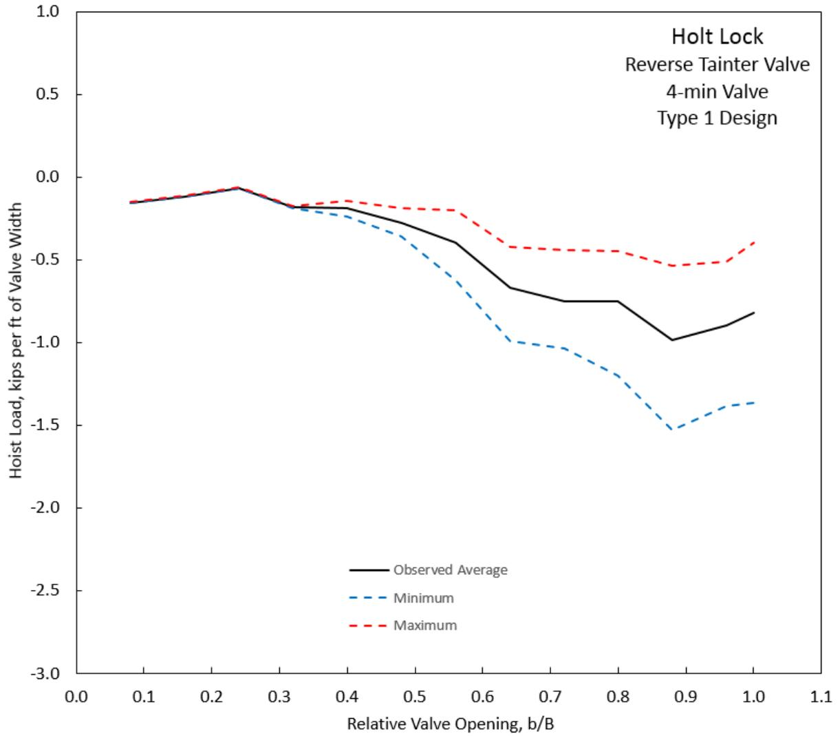
**Figure D-13. Hoist load, Holt Lock, Type 1 Design, 4-min Valve.**
