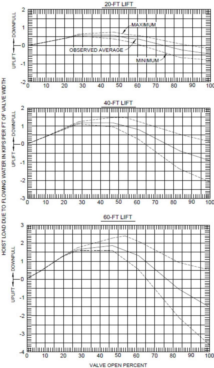
Figure 3-2. Hoist loads in a horizontally framed valve.
