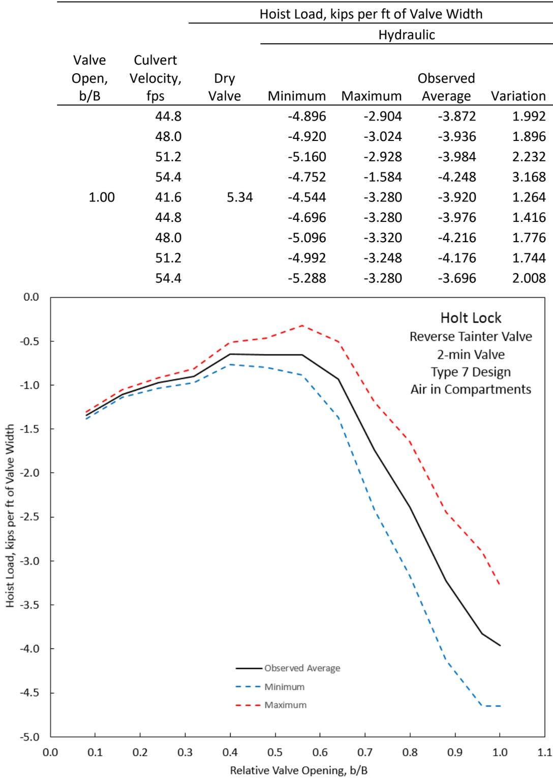
Figure D-26. Hoist load, Holt Lock, Type 7 Design, 2-min Valve, Air in Compartments.
