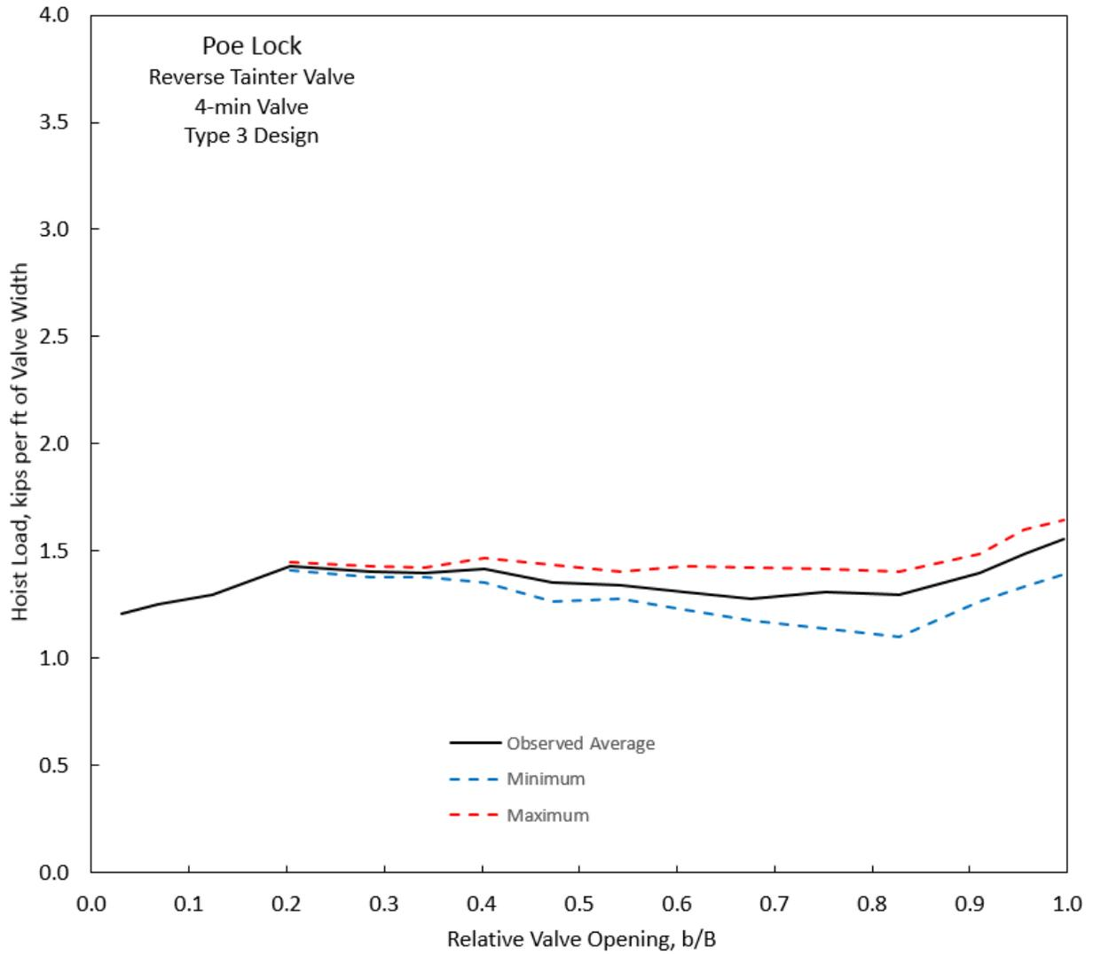
**Figure D-8. Hoist load, Poe Lock, Type 3 Design, 4-min Valve.**
