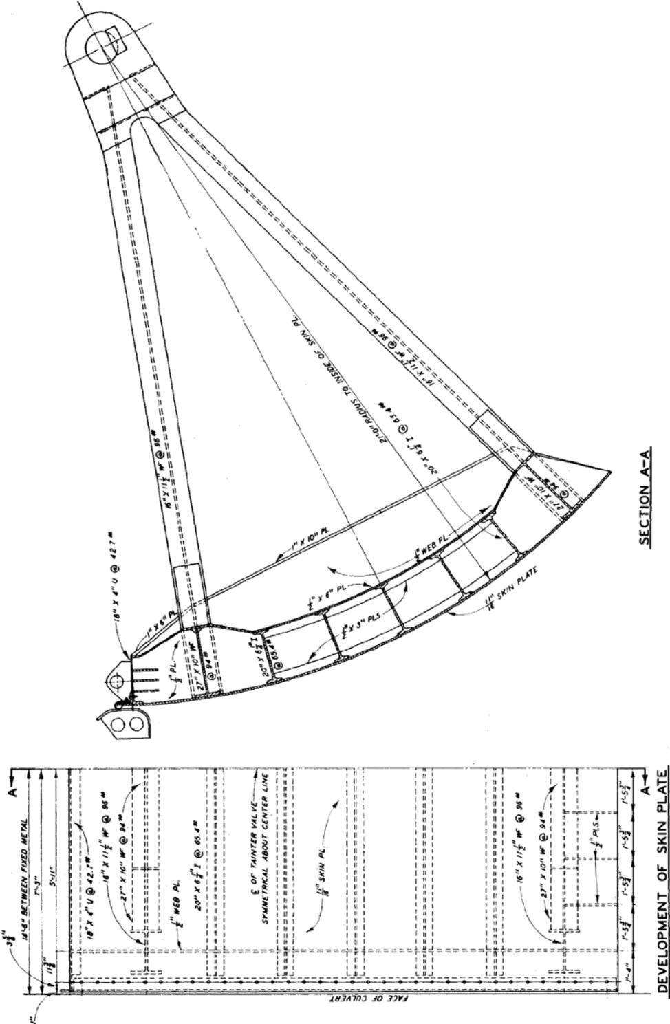
Figure D-1. Tainter Valve, Lock No. 19, Type 1 Design.
