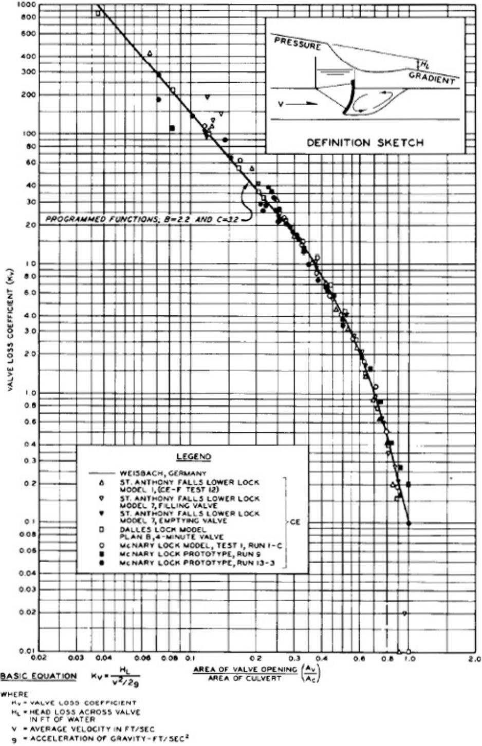
Figure C-3. Loss coefficient, reverse tainter valve.
