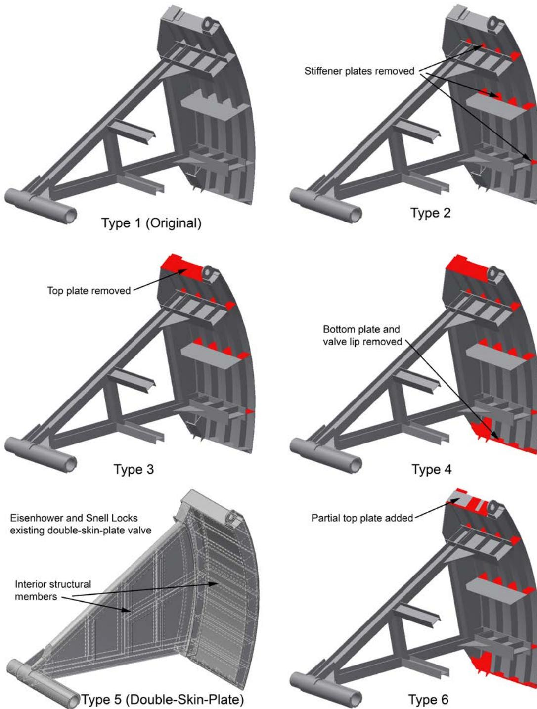
**Figure D-30. Tainter Valves, Snell Lock, Type 1-6 Designs.**
