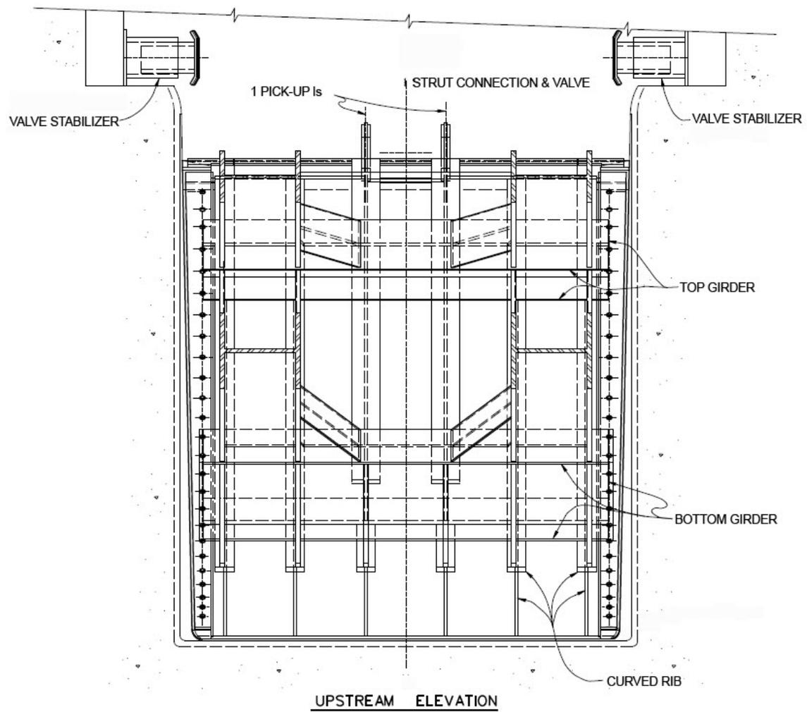
Figure 5-3. Line drawings of dampers installed on valve recess walls, Chickamauga Lock.
