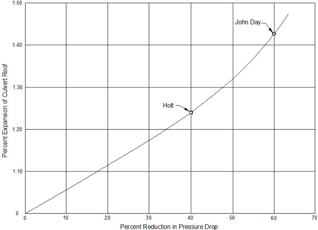
Note: Pressure drop is the difference between the elevation of the lower pool and the minimum pressure gradient at the vena contracta during the valve opening period.
