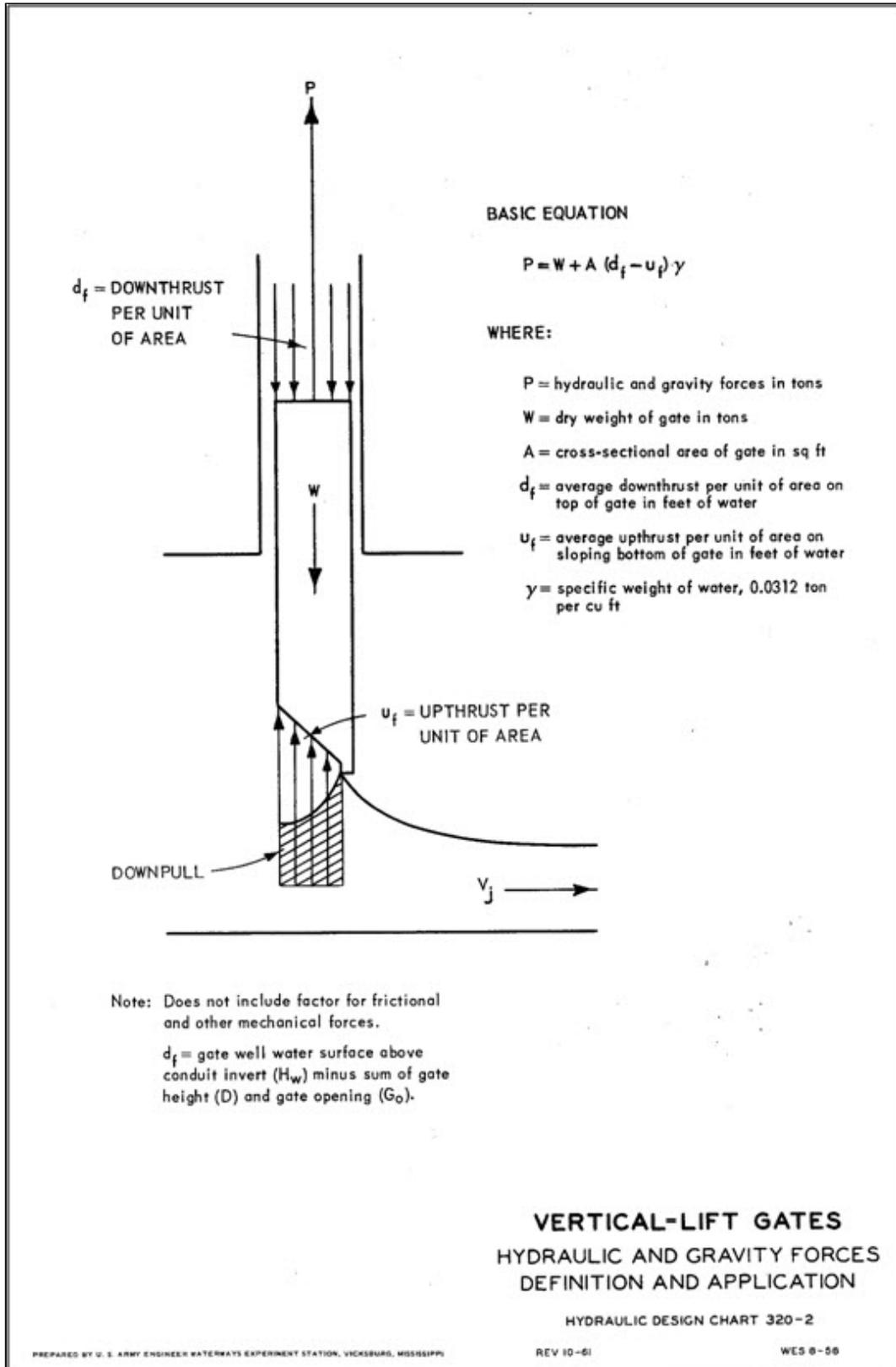
Figure 1-3. Hydraulic and gravity forces on vertical-lift valves.
