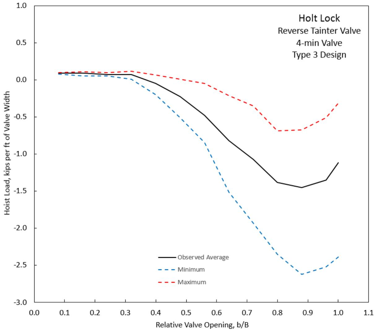
**Figure D-17. Hoist load, Holt Lock, Type 3 Design, 4-min Valve.**
