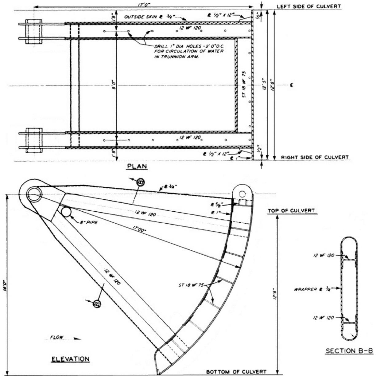
Figure D-25. Tainter Valve, Holt Lock, Type 7 Design.
