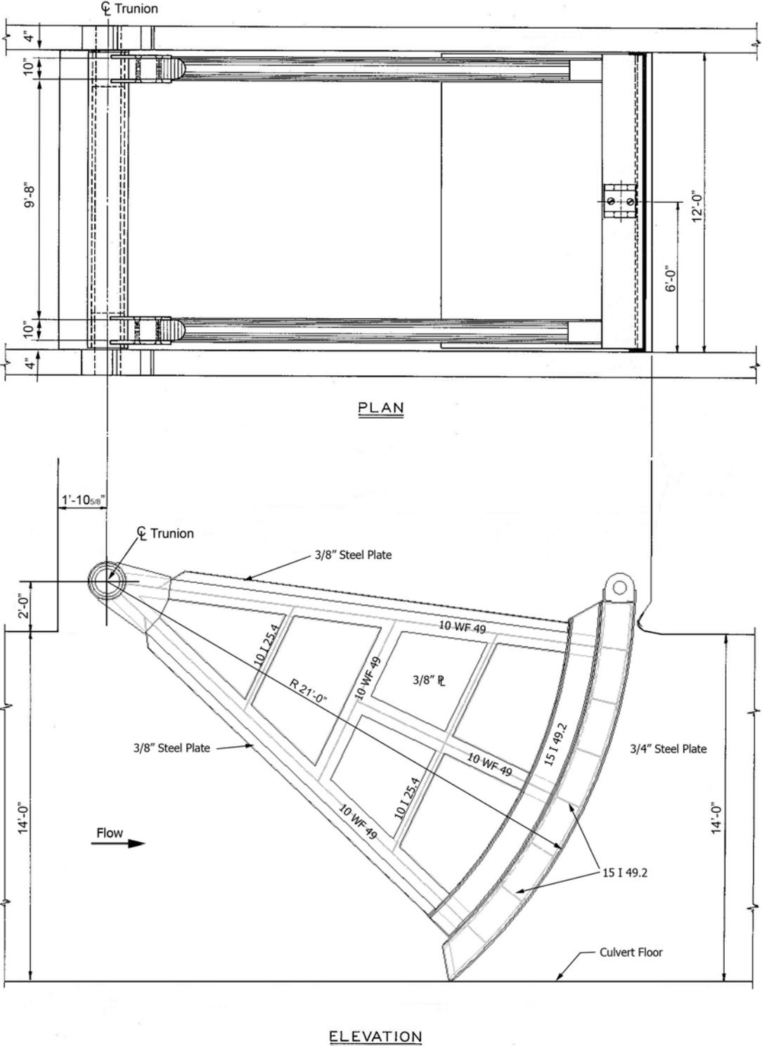
Figure D-34. Tainter Valve, Snell Lock, Type 5 Design.
