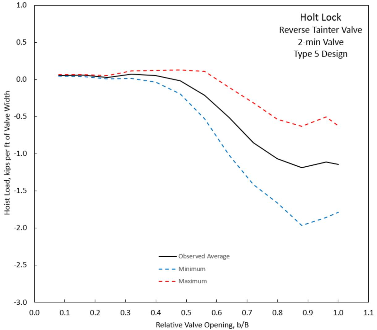
**Figure D-21. Hoist load, Holt Lock, Type 5 Design, 2-min Valve.**
