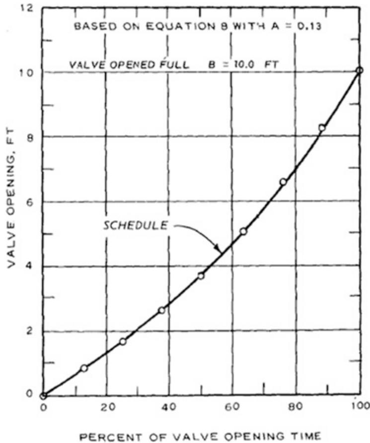
Figure C-2. Valve opening pattern at Millers Ferry Lock.
