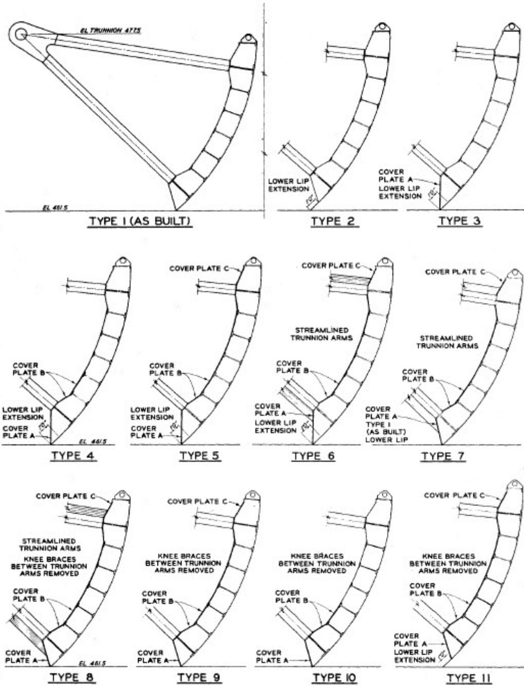
Figure D-4. Tainter Valves, Lock No. 19, Types 1-11 Designs.
