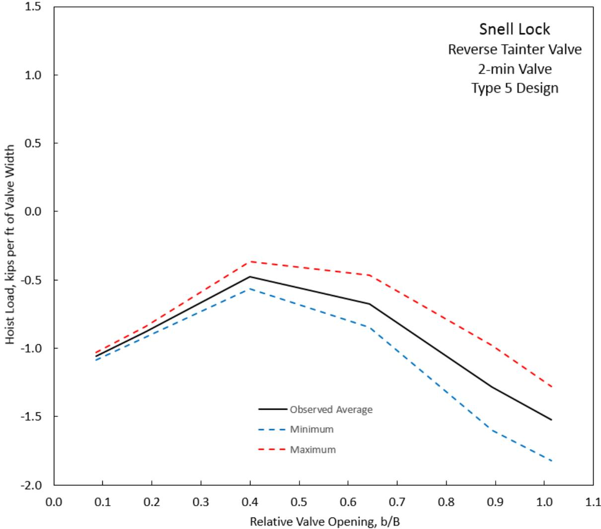
**Figure D-35. Hoist Loads, Snell Lock, Type 5 Design, 2-min Valve.**
