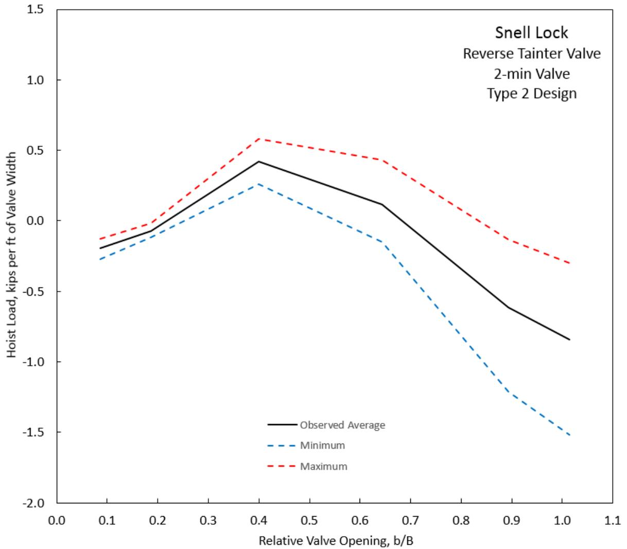
**Figure D-31. Hoist load, Snell Lock, Type 2 Design, 2-min Valve.**
