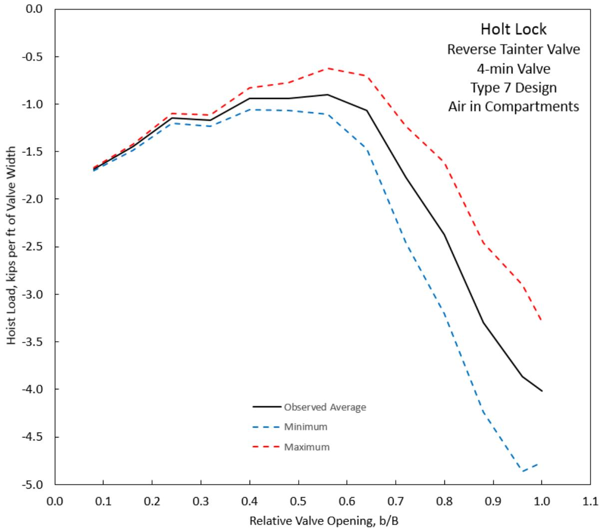
**Figure D-27. Hoist load, Holt Lock, Type 7 Design, 4-min Valve, Air in Compartments.**
