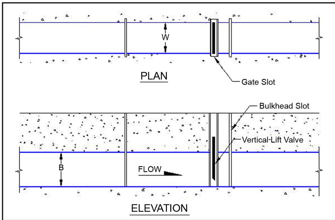
**Figure 1-2. Vertical-lift valve installation.**
