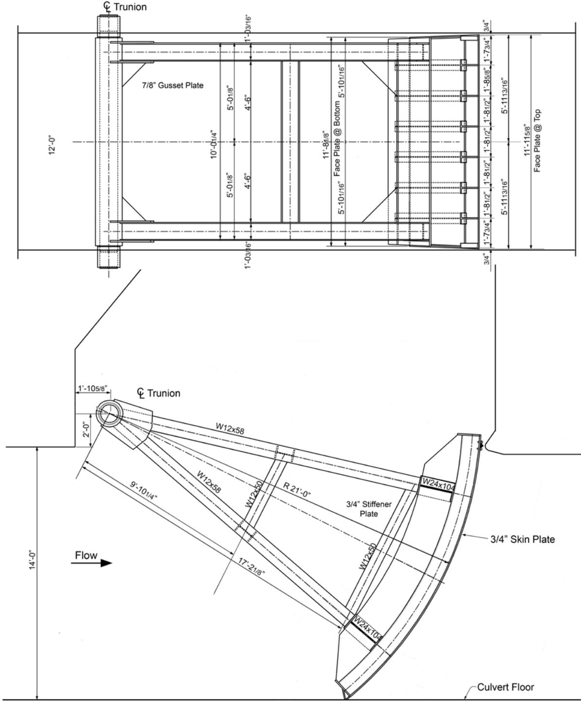
Figure D-28. Tainter Valve, Snell Lock, Type 1 Design.
