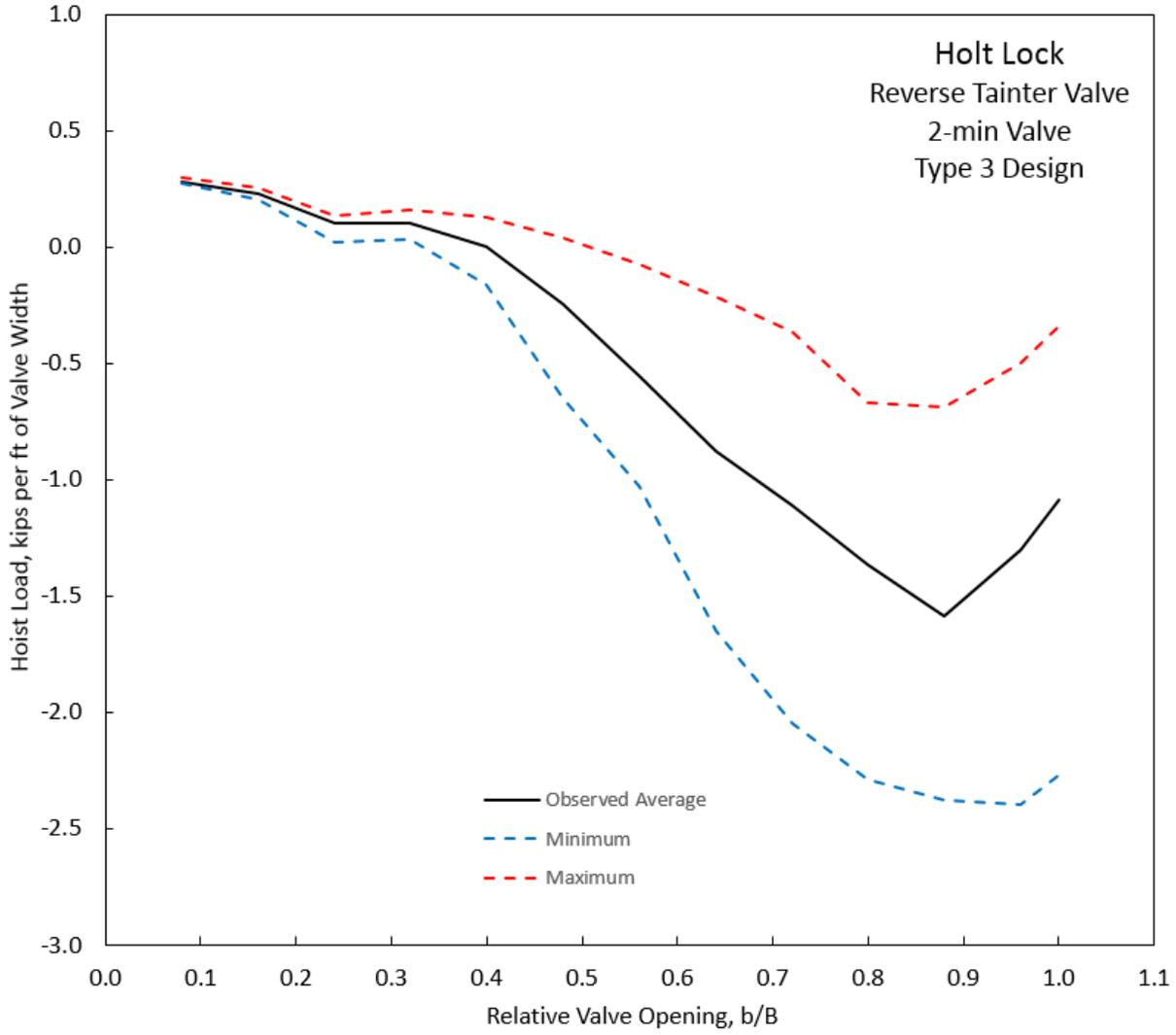
**Figure D-16. Hoist load, Holt Lock, Type 3 Design, 2-min Valve.**
