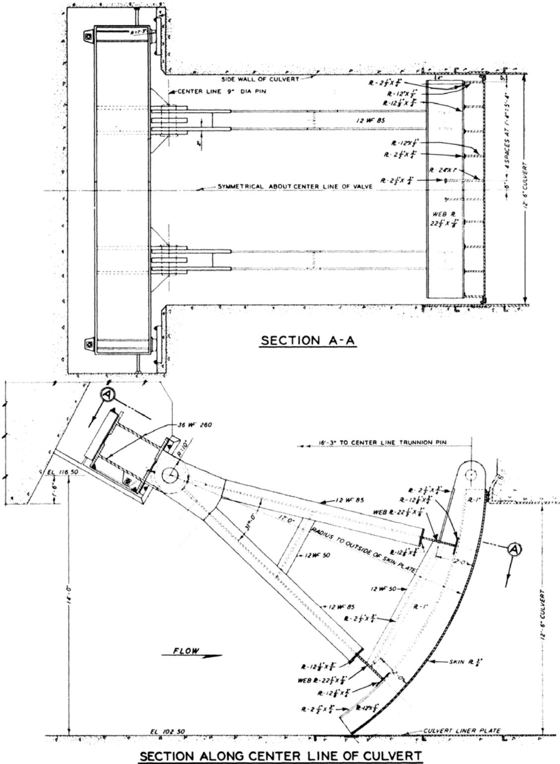
Figure D-20. Tainter Valve, Holt Lock, Type 5 Design.
