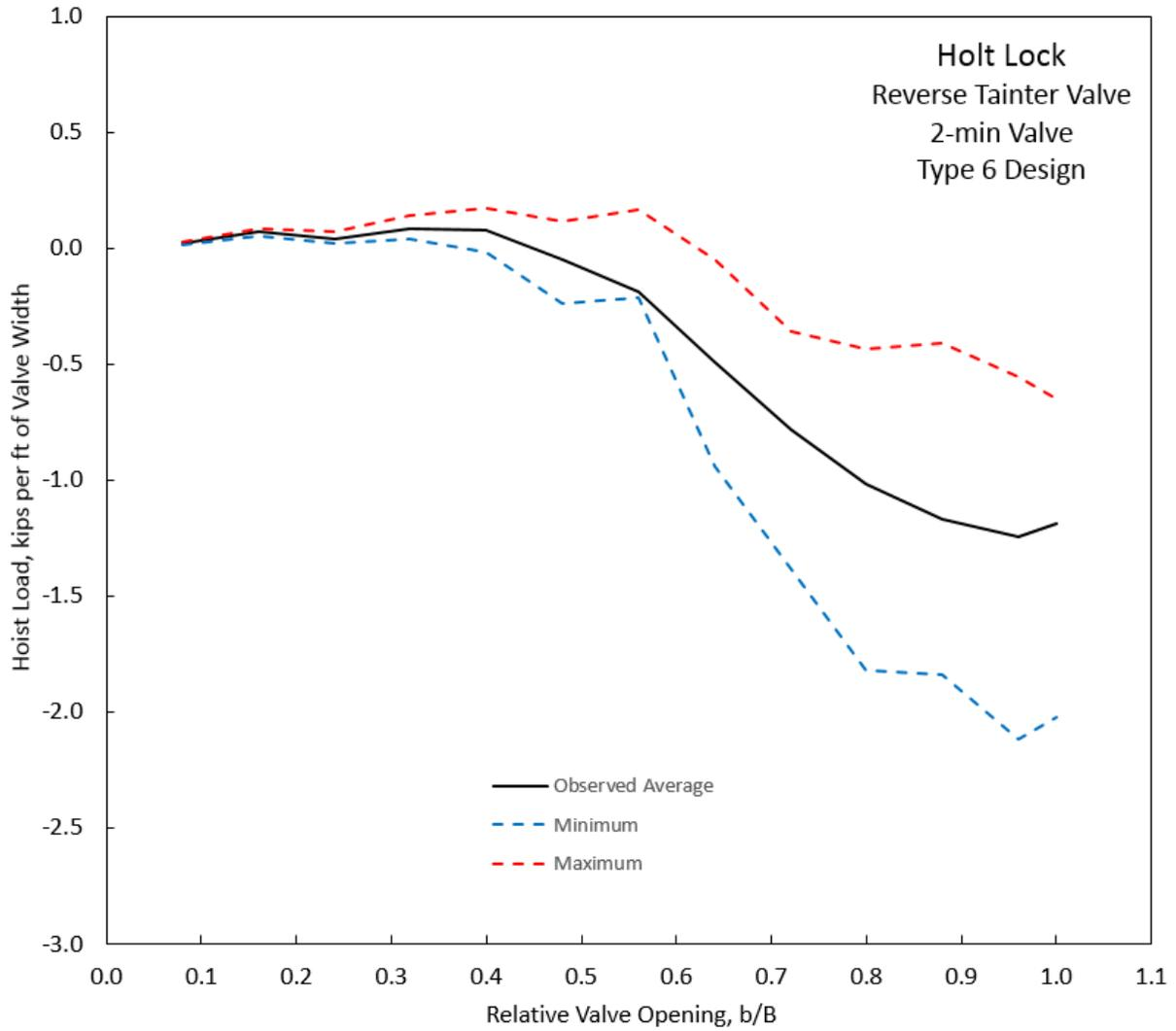
**Figure D-23. Hoist load, Holt Lock, Type 6 Design, 2-min Valve.**
