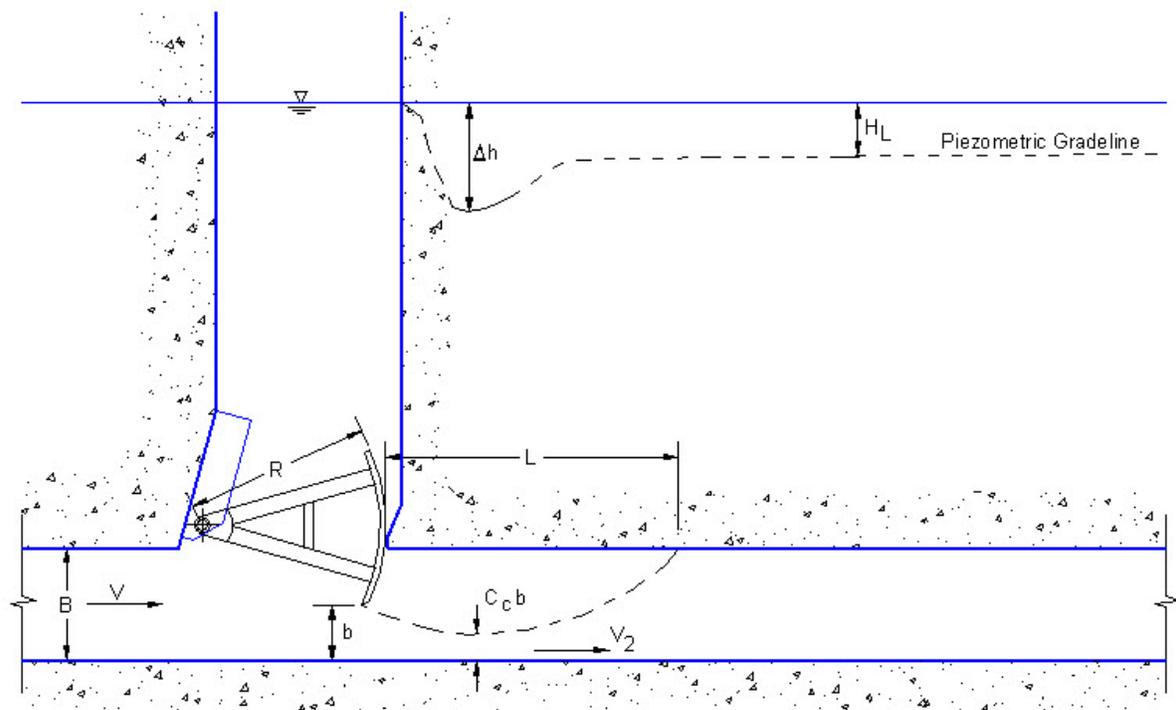
**Figure 1-5. Reverse tainter valve installation.**
