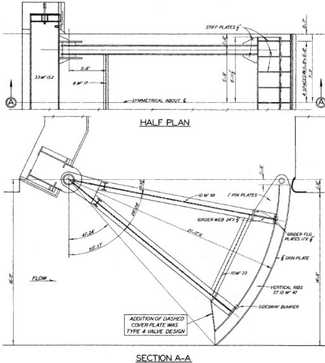
Figure D-9. Tainter Valves, Poe Lock, Types 3 and 4 Designs.
