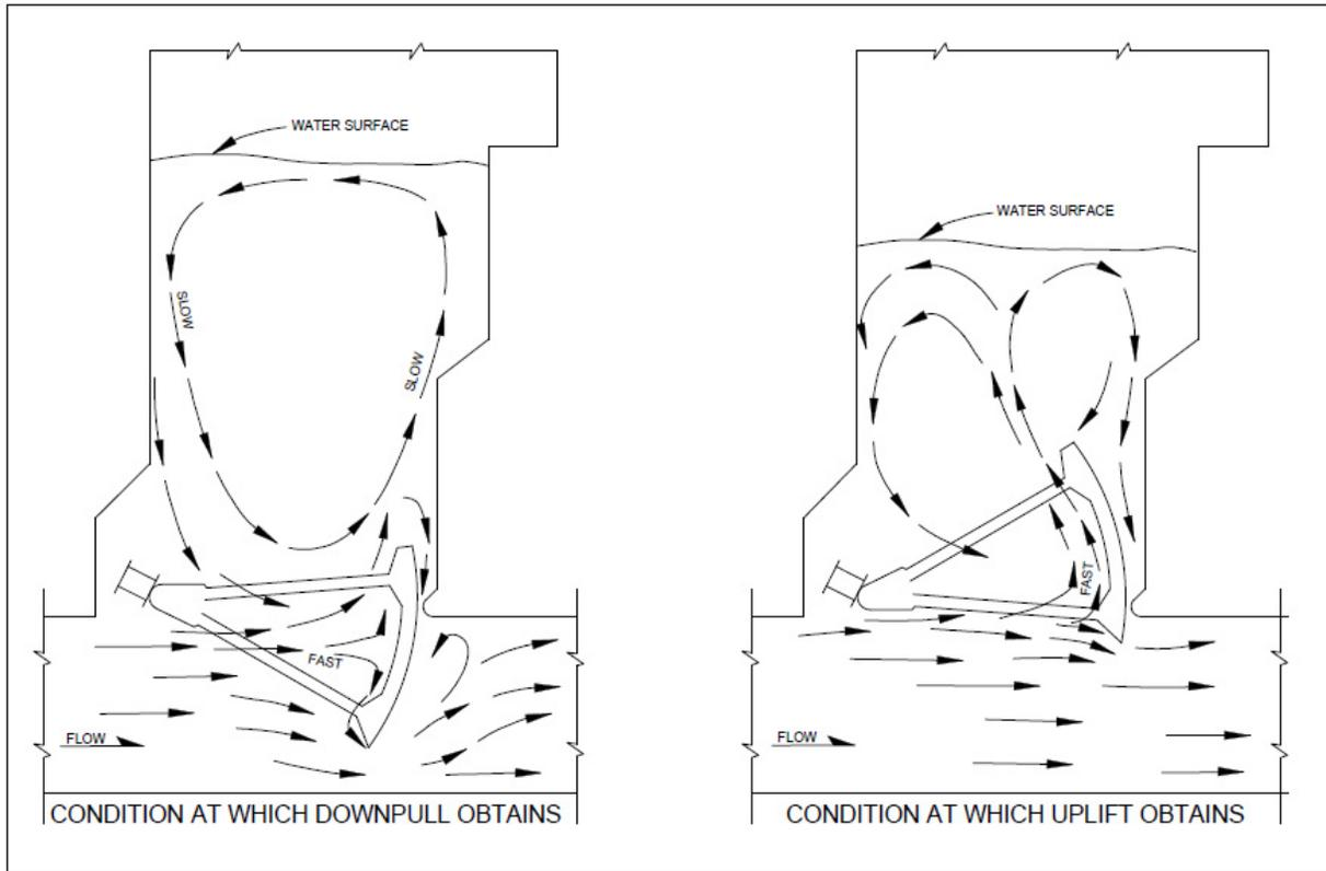
**Figure 3-5. Flow patterns around reverse tainter valves.**
