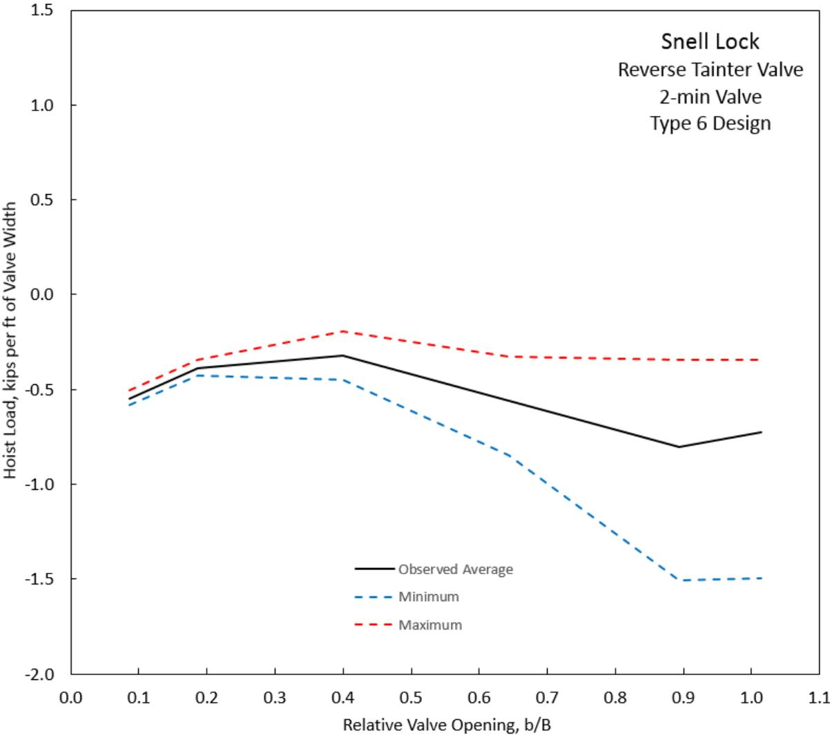
Figure D-36. Hoist load, Snell Lock, Type 6 Design, 2-min Valve.
