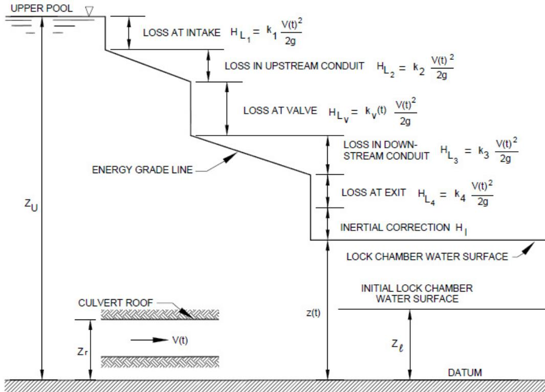
**Figure C-1. Simulated flow conditions at time t.**
