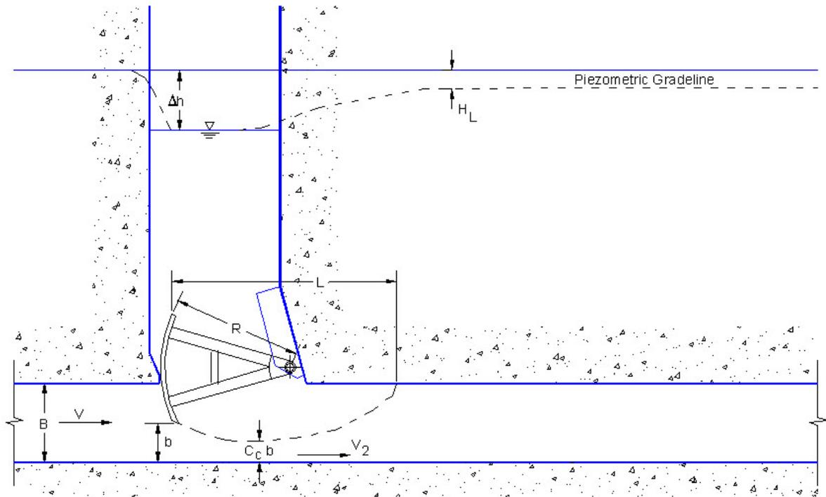
**Figure 1-4. Conventional tainter valve installation.**
