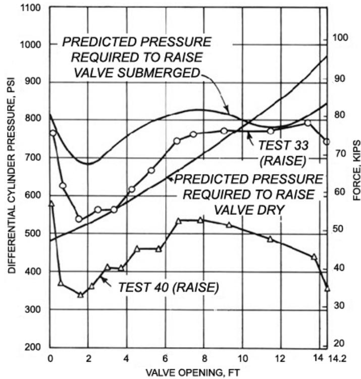
Figure 3-7. Bankhead Lock total hoist loads, design values and those measured in prototype, 1-min (Test 33) and 2-min (Test 40) single-valve operations.
