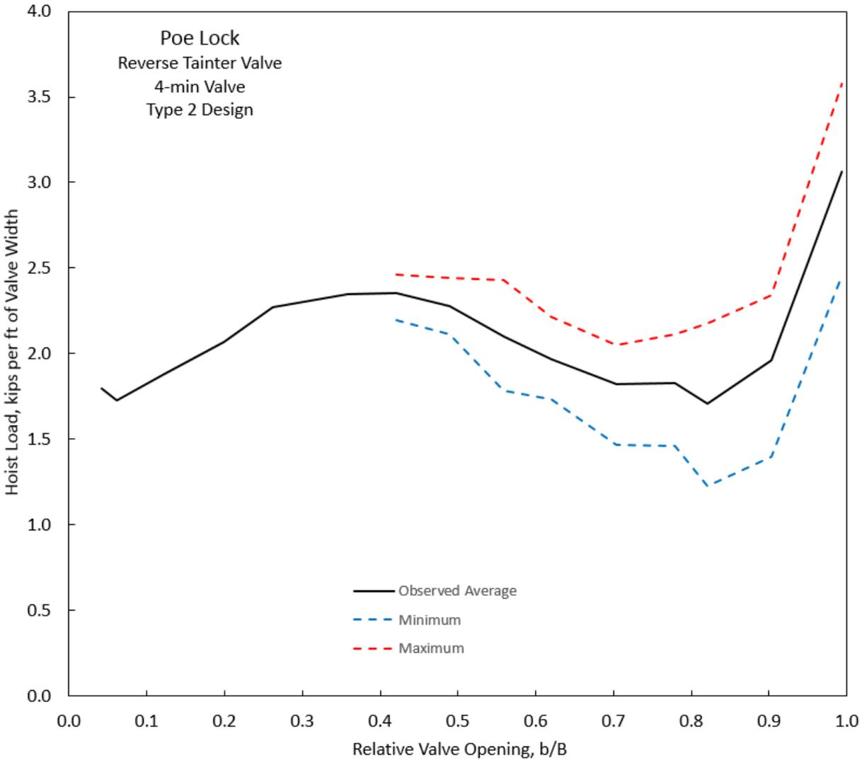
**Figure D-8. Hoist load, Poe Lock, Type 2 Design, 4-min Valve.**
