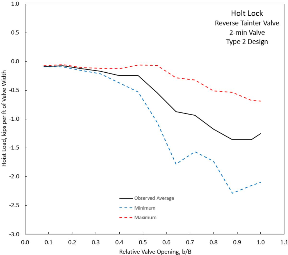
**Figure D-14. Hoist load, Holt Lock, Type 2 Design, 2-min Valve.**
