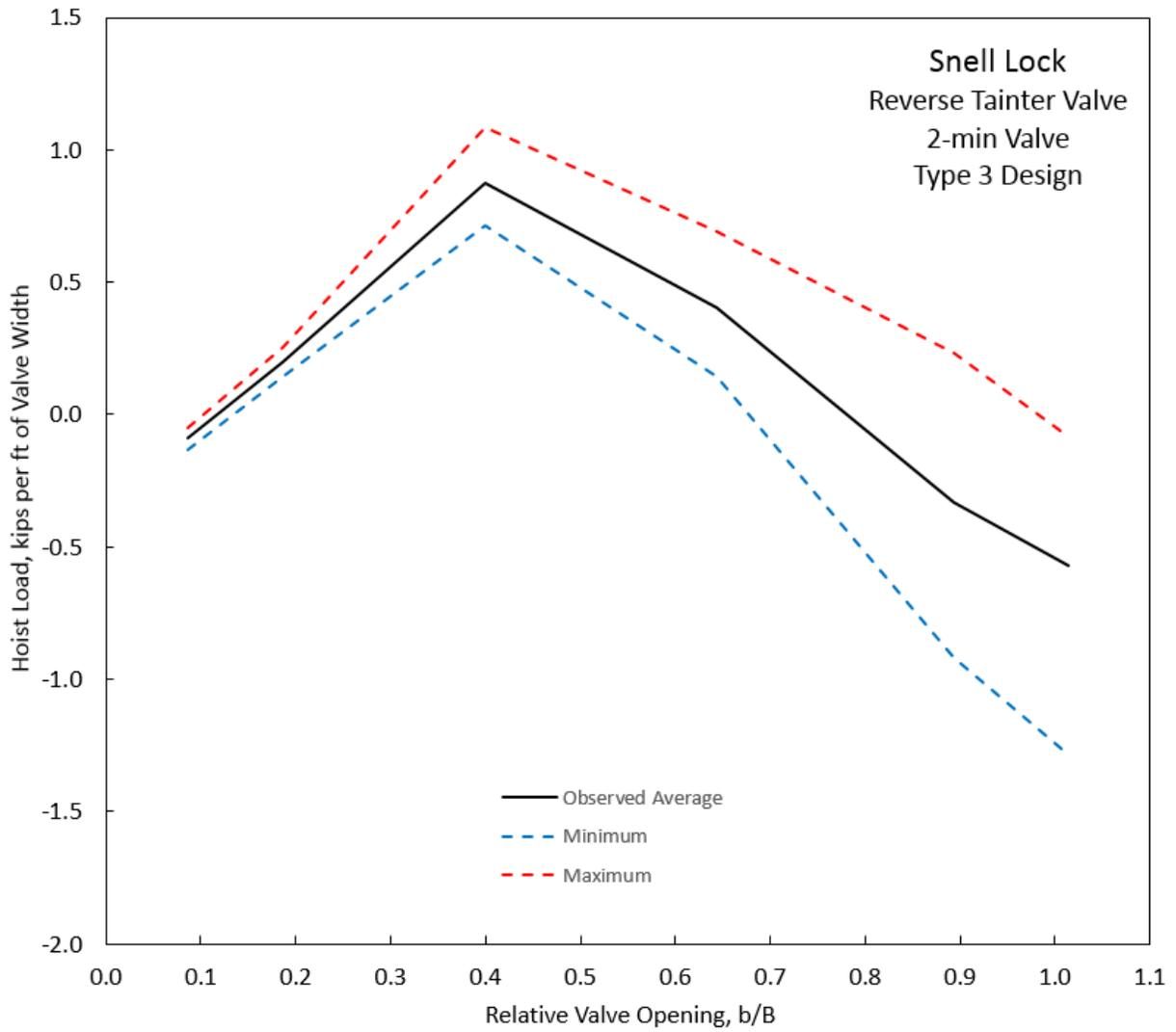
**Figure D-32. Hoist load, Snell Lock, Type 3 Design, 2-min Valve.**
