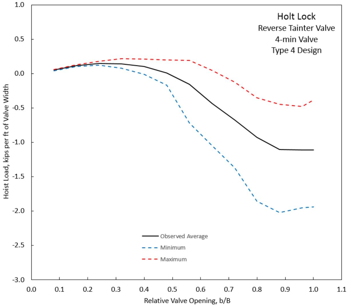
**Figure D-19. Hoist load, Holt Lock, Type 4 Design, 4-min Valve.**
