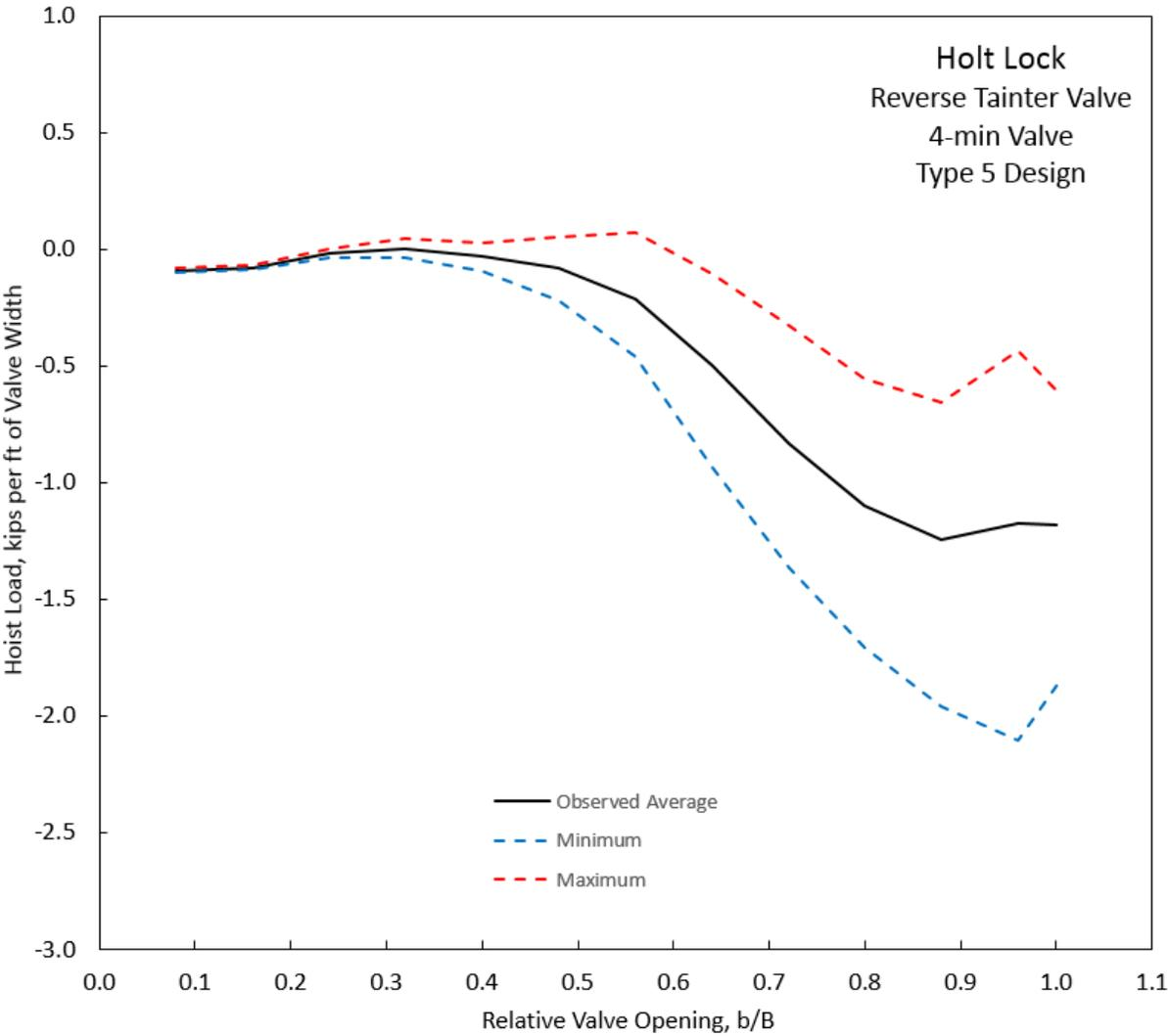
**Figure D-22. Hoist load, Holt Lock, Type 5 Design, 4-min Valve.**
