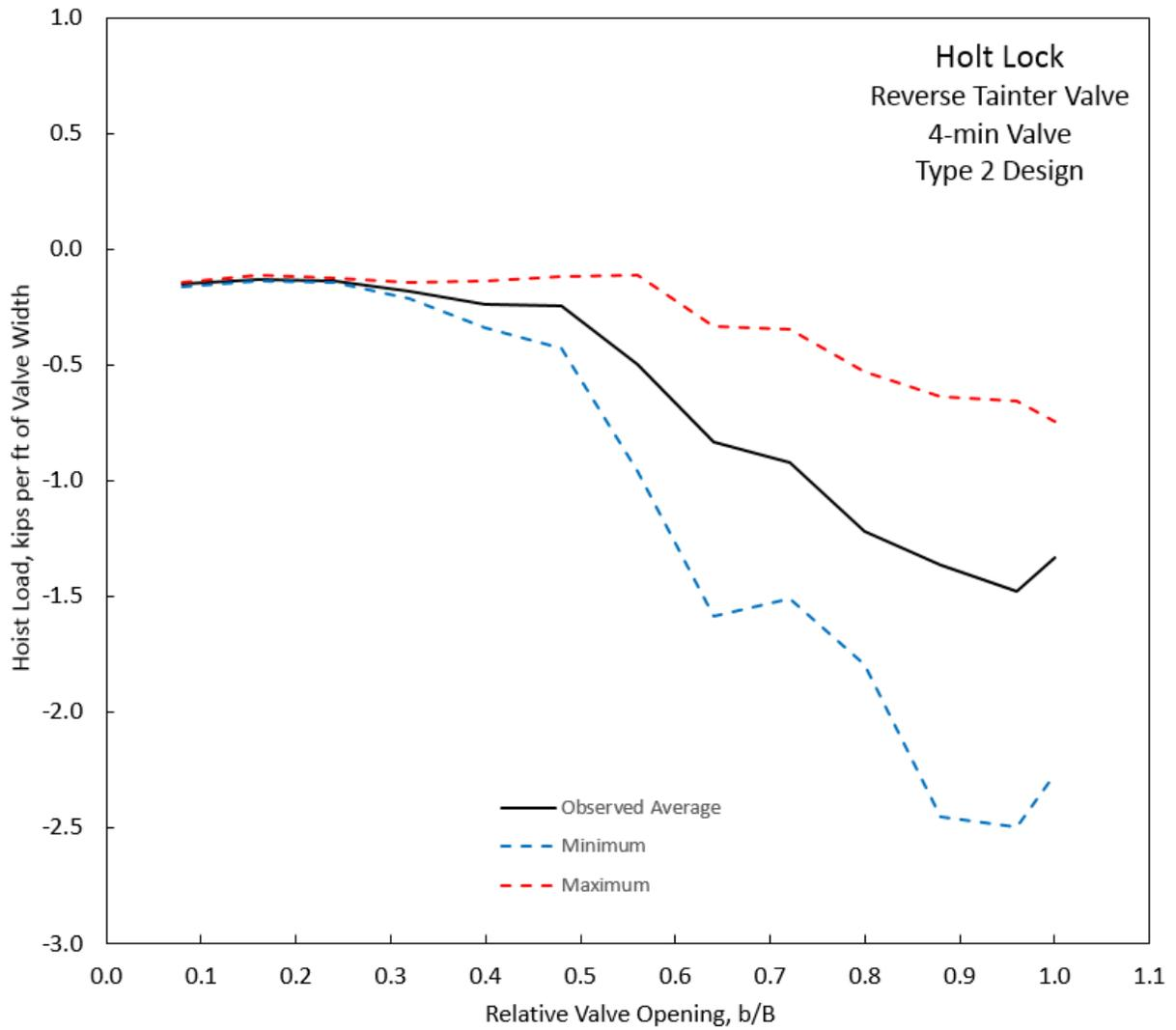
**Figure D-15. Hoist load, Holt Lock, Type 2 Design, 4-min Valve.**
