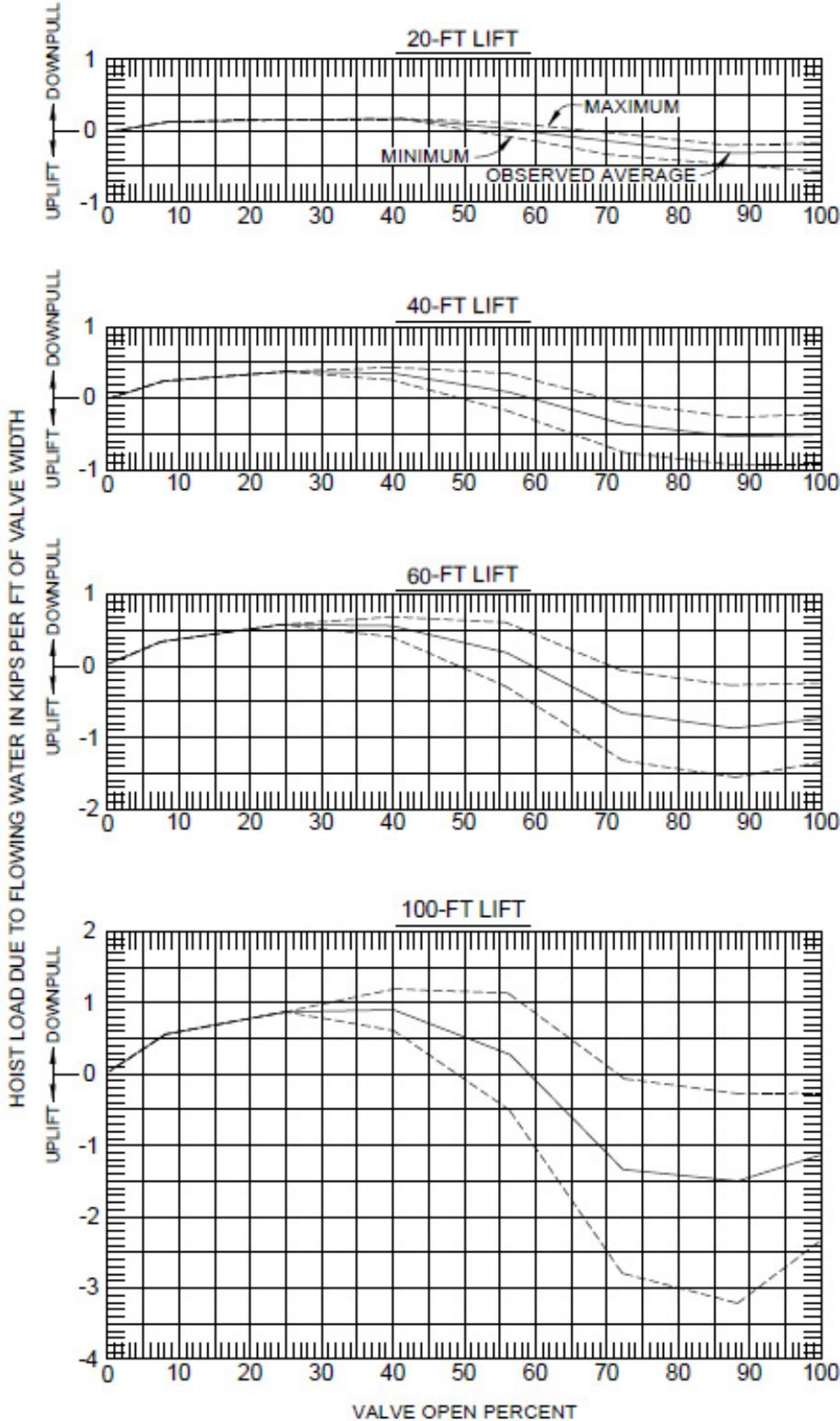
Figure 3-4. Total hoist loads on a vertically framed valve.
