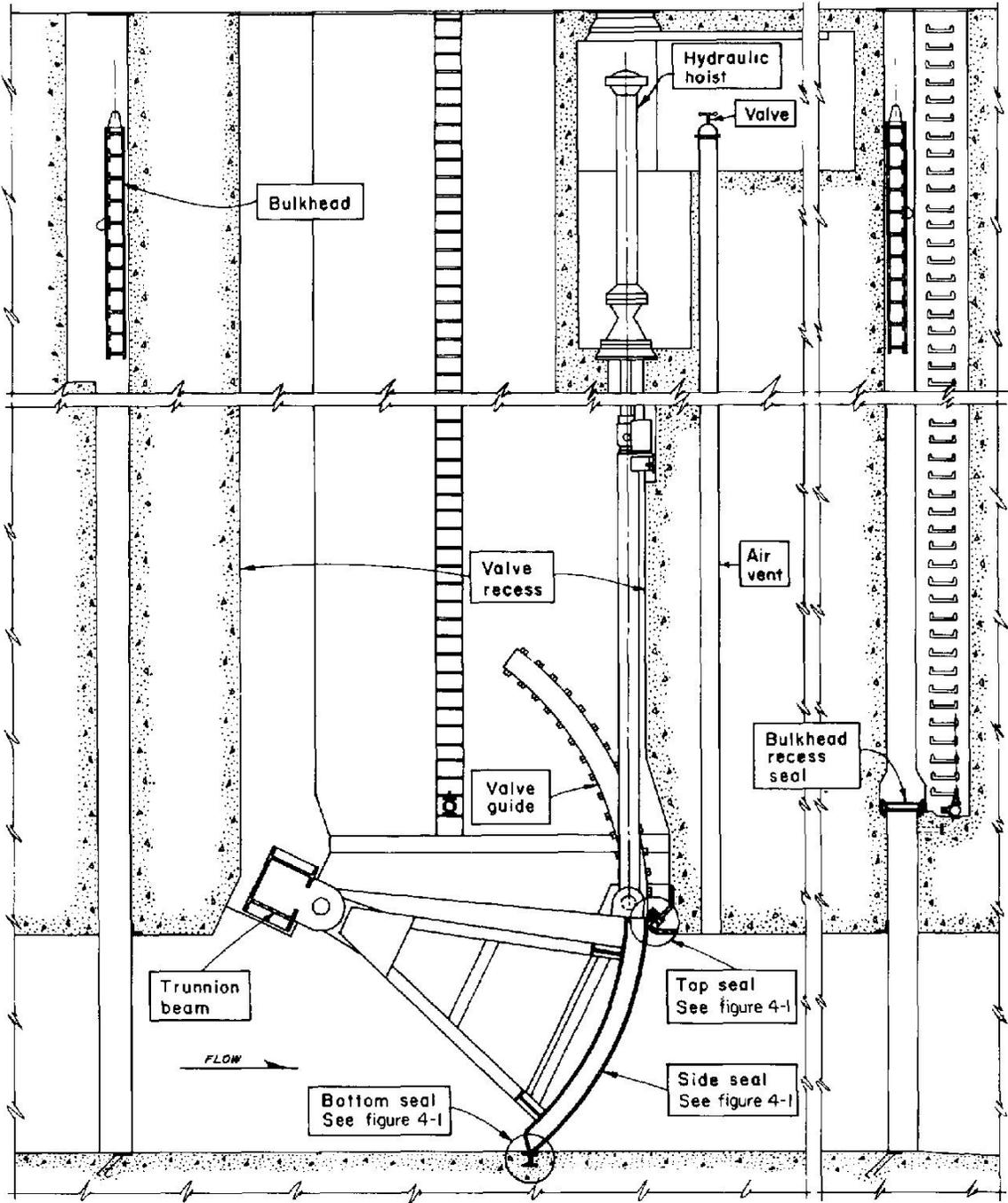
Figure 1-6. Elevation view of typical reverse tainter valve machinery hoist.
