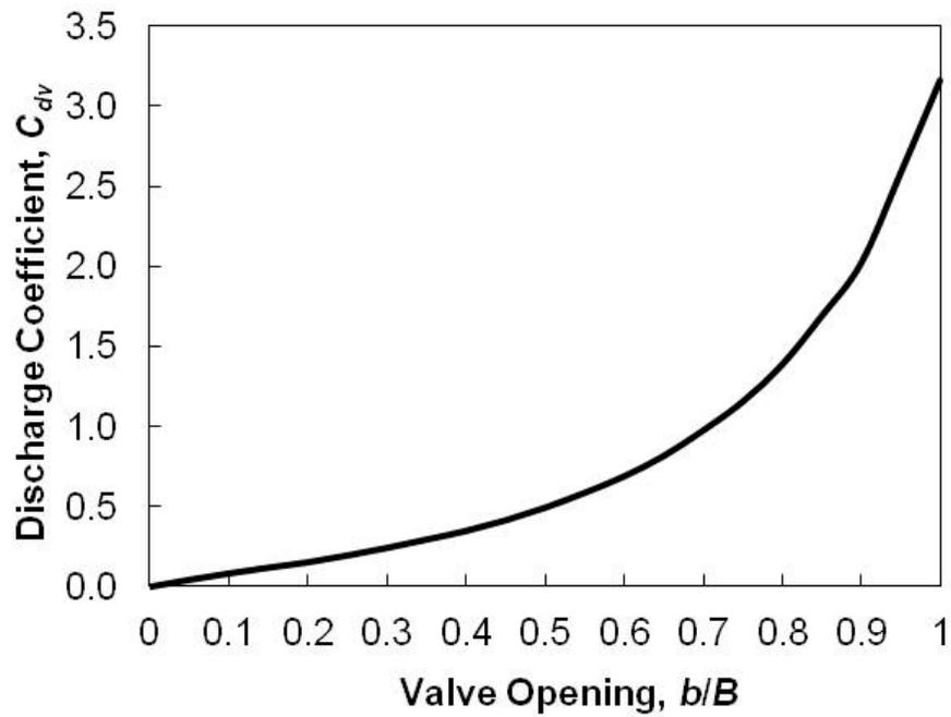
Figure C-6. Discharge coefficient for reverse tainter valve
