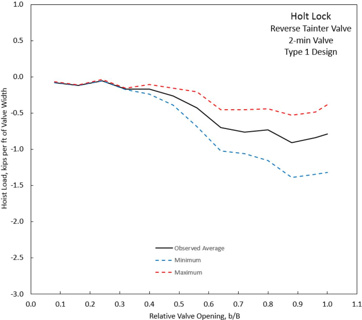
**Figure D-12. Hoist load, Holt Lock, Type 1 Design, 2-min Valve.**
