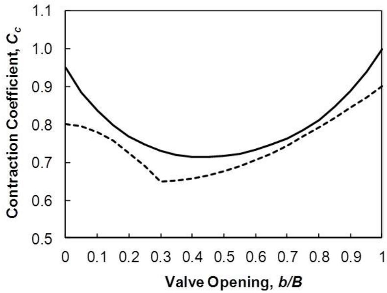
Figure C-5. Contraction coefficient for reverse tainter valve.
