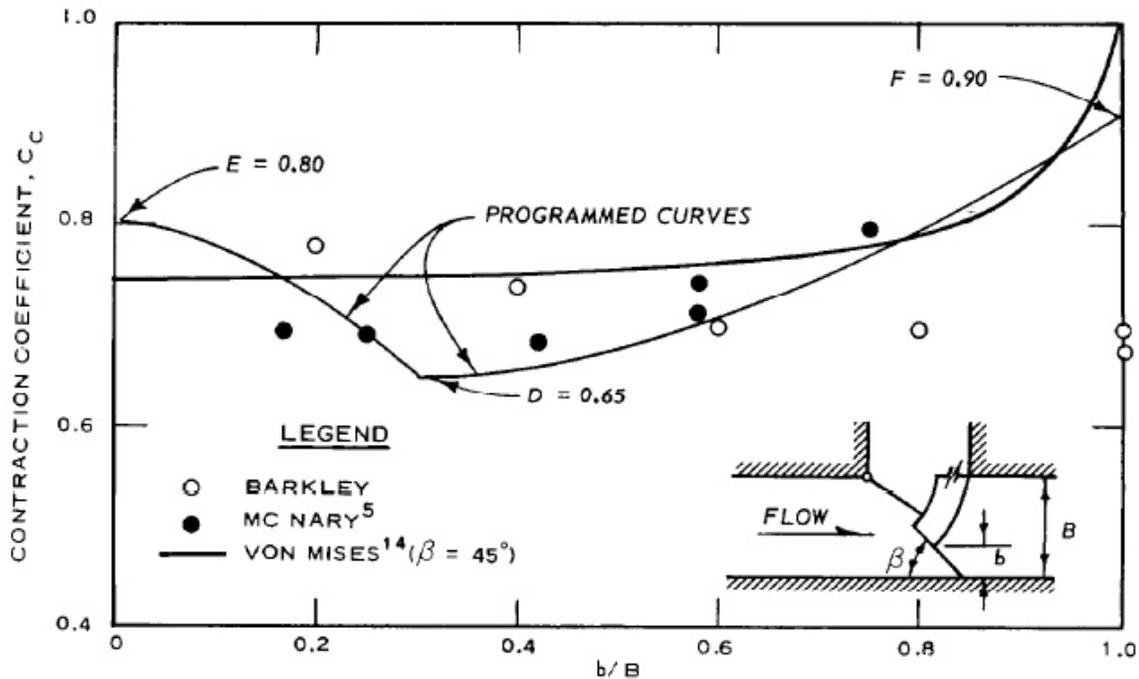
Figure C-4. Reverse tainter valve contraction coefficient.
