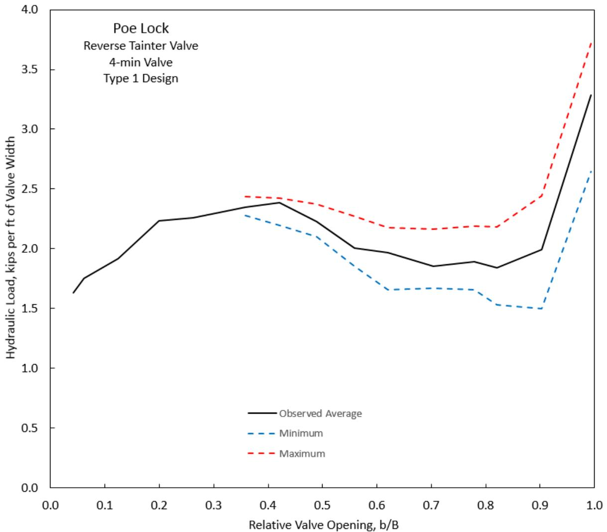
**Figure D-7. Hoist loads, Poe Lock, Type 1 Design, 4-min Valve.**
