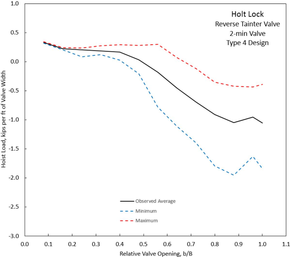
**Figure D-18. Hoist load, Holt Lock, Type 4 Design, 2-min Valve.**
