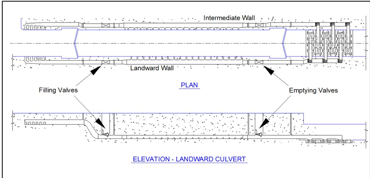
**Figure 1-1. Sidewall port filling and emptying system with reverse tainter valves.**
