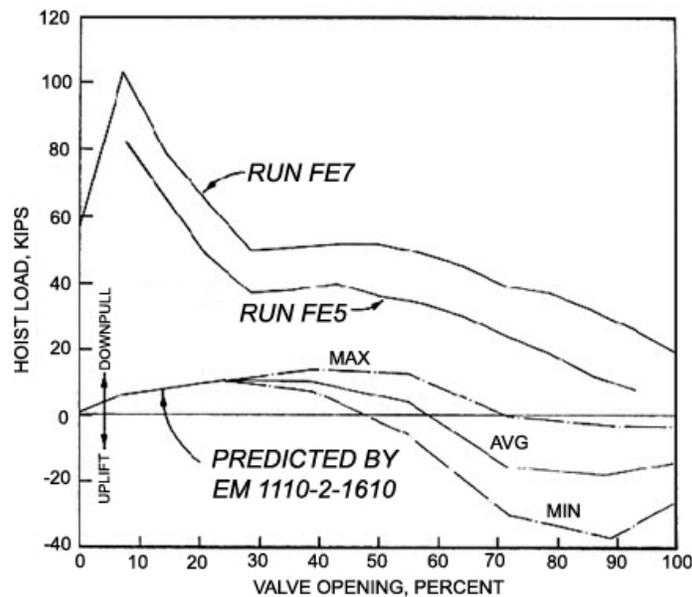
Figure 3-8. Total hoist load on Whitten Lock filling valve hoist load, prototype and design guidance, 1-min (Test FE7) and 4-min (Test FE 5) single-valve operation, 83.1-ft lift.
