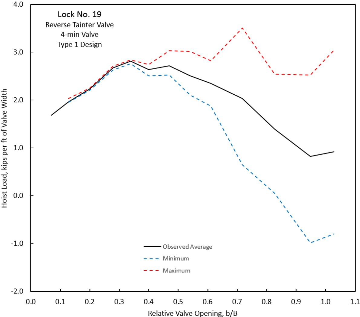
**Figure D-3. Hoist loads, Lock No. 19, Type 1 Design, 4-min Valve.**
