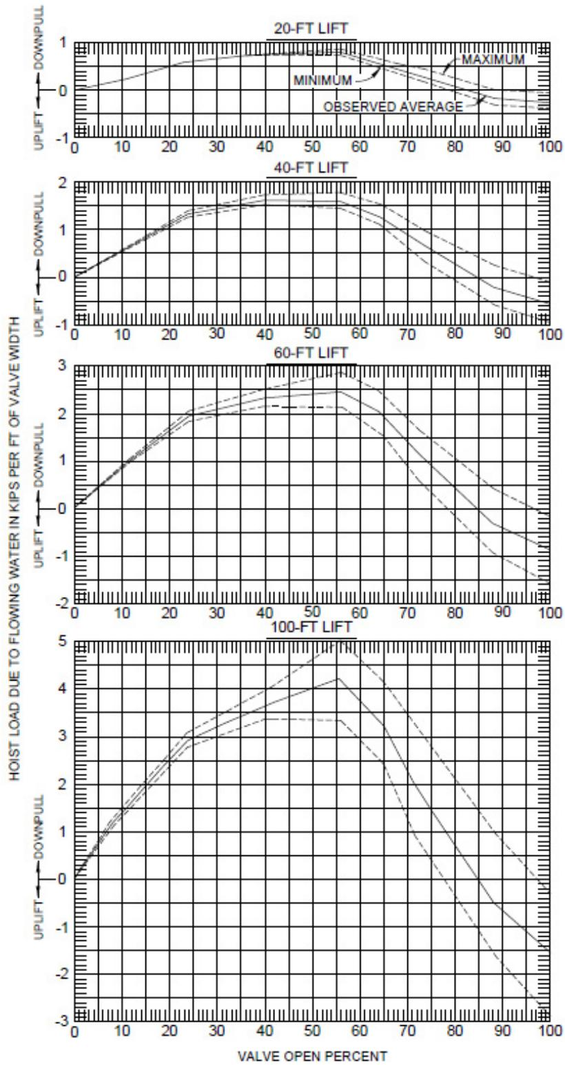
Figure 3-3. Total hoist loads on a double-skin plate valve.
