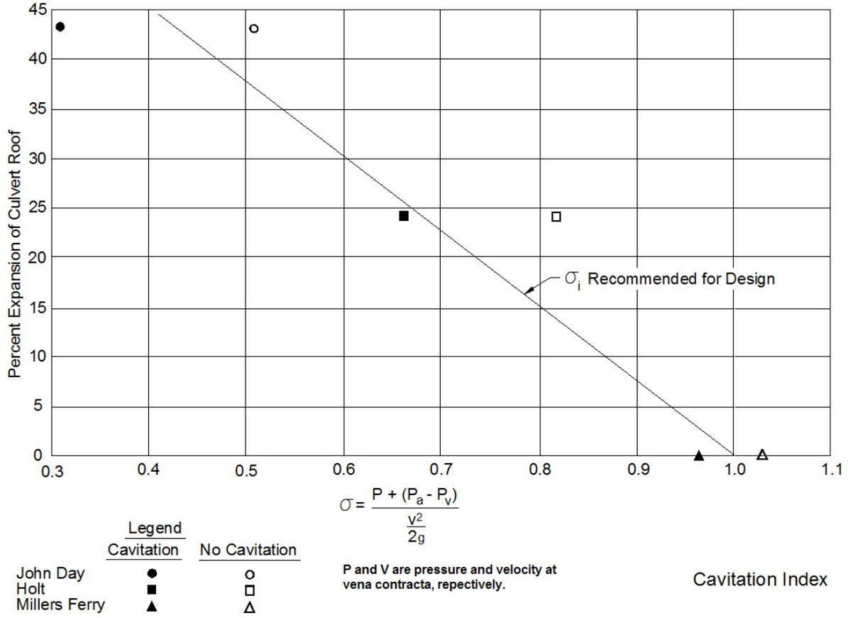
**Figure 2-1. Cavitation index.**
