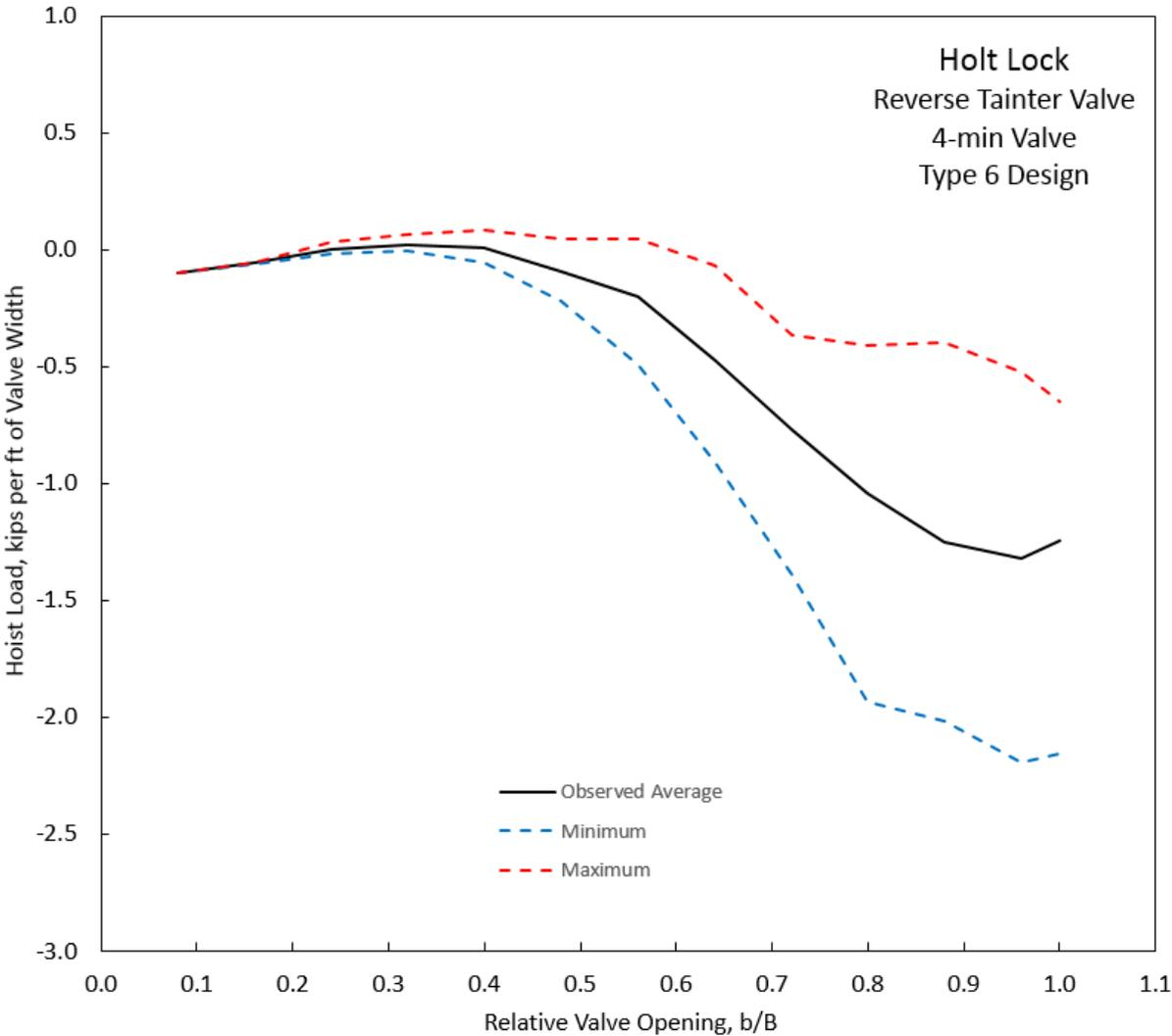
**Figure D-24. Hoist load, Holt Lock, Type 6 Design, 4-min Valve.**
