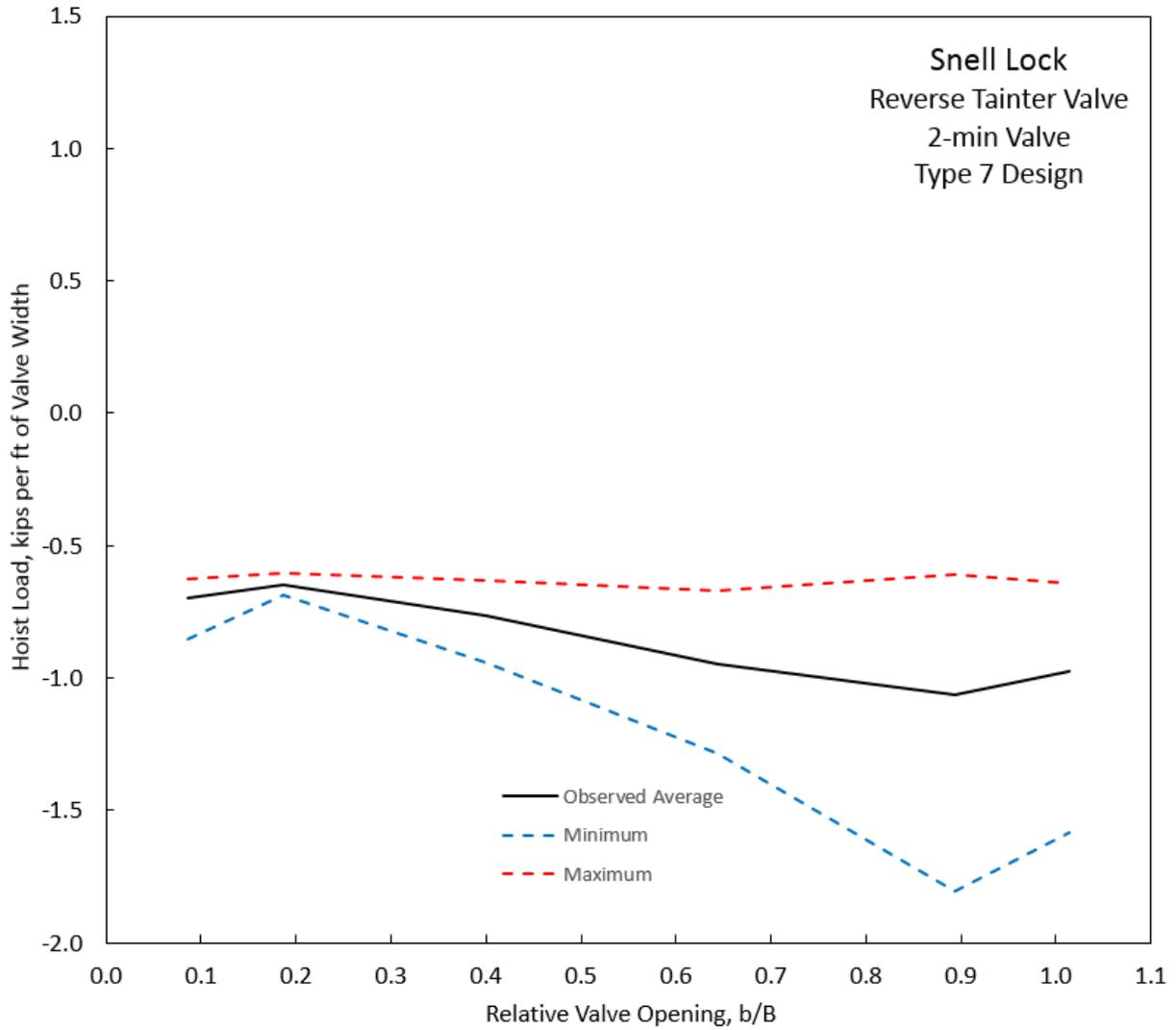
**Figure D-38. Hoist load, Snell Lock, Type 7 Design, 2-min Valve.**
