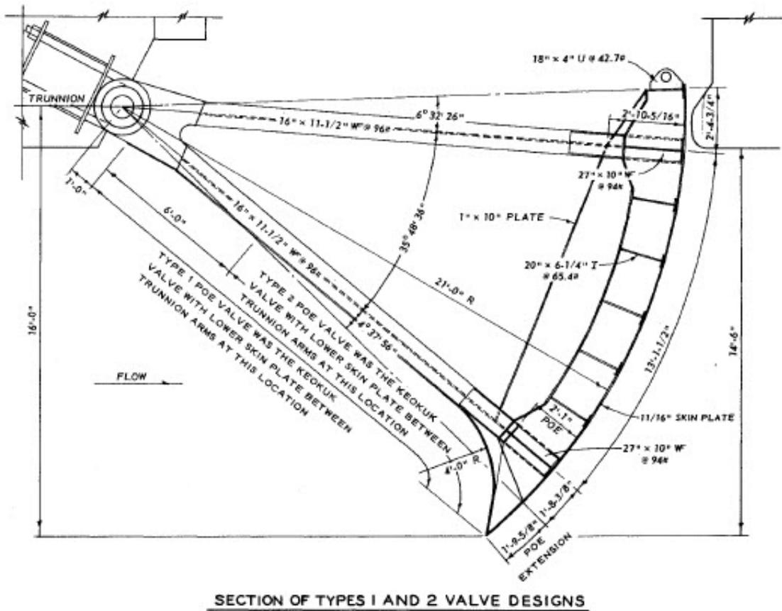
Figure D-6. Tainter Valves, Poe Lock, Types 1 and 2 Designs.
