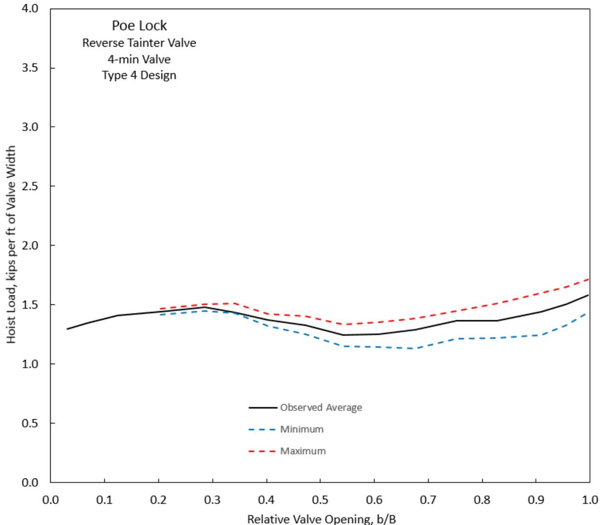
**Figure D-9. Hoist load, Poe Lock, Type 4 Design, 4-min Valve.**
