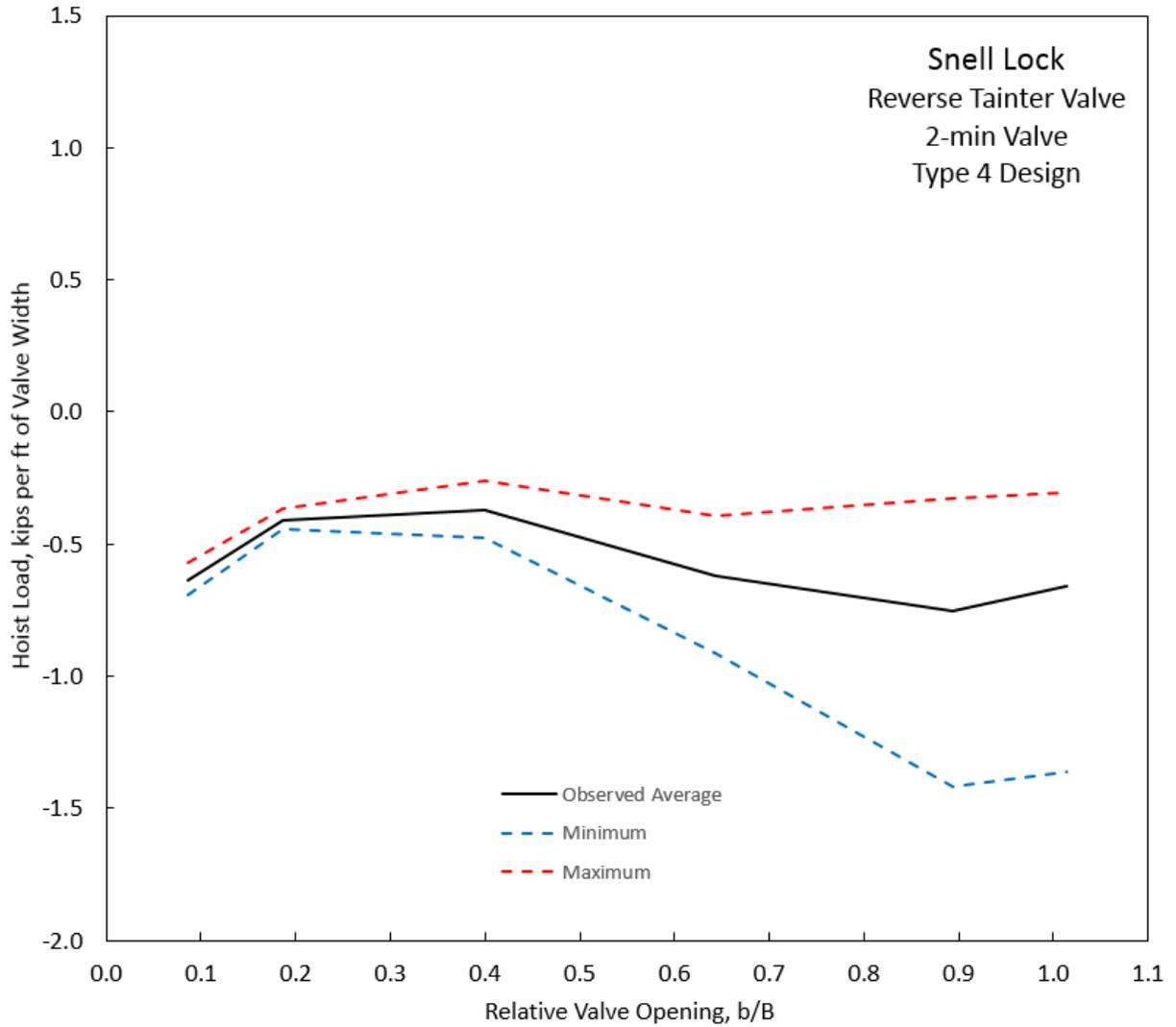
**Figure D-33. Hoist load, Snell Lock, Type 4 Design, 2-min Valve.**
