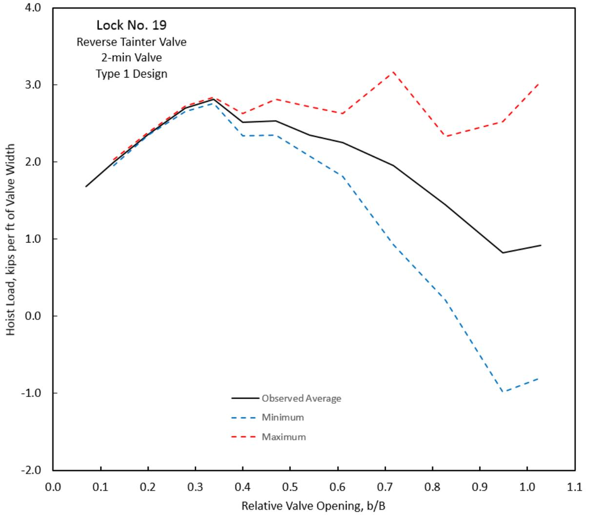
**Figure D-2. Hoist loads, Lock No. 19, Type 1 Design, 2-min Valve.**
