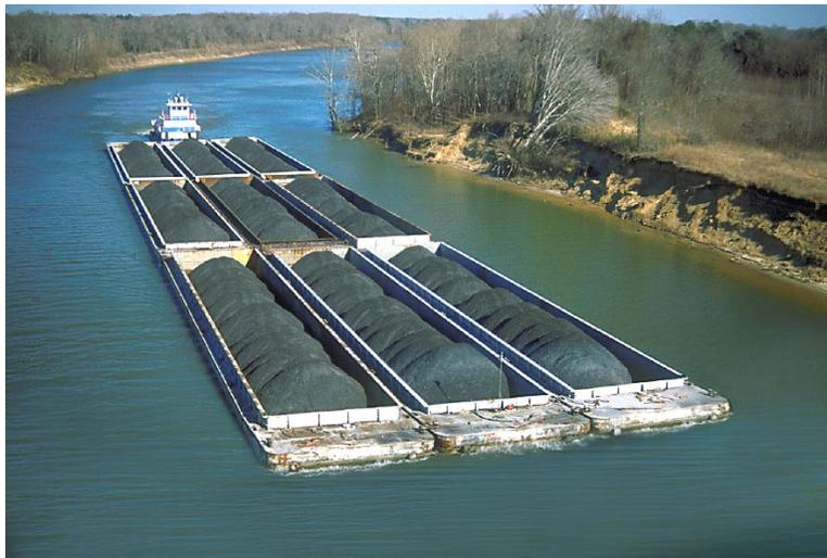
Figure 3.11. Typical Barge Flotilla in Transit
