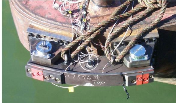
Figure 3.28. Load-Measurement System (Beam, Shear Pins, and Clevis Mounts) Attached to Bow Corner of Barge (Patev 2003)
