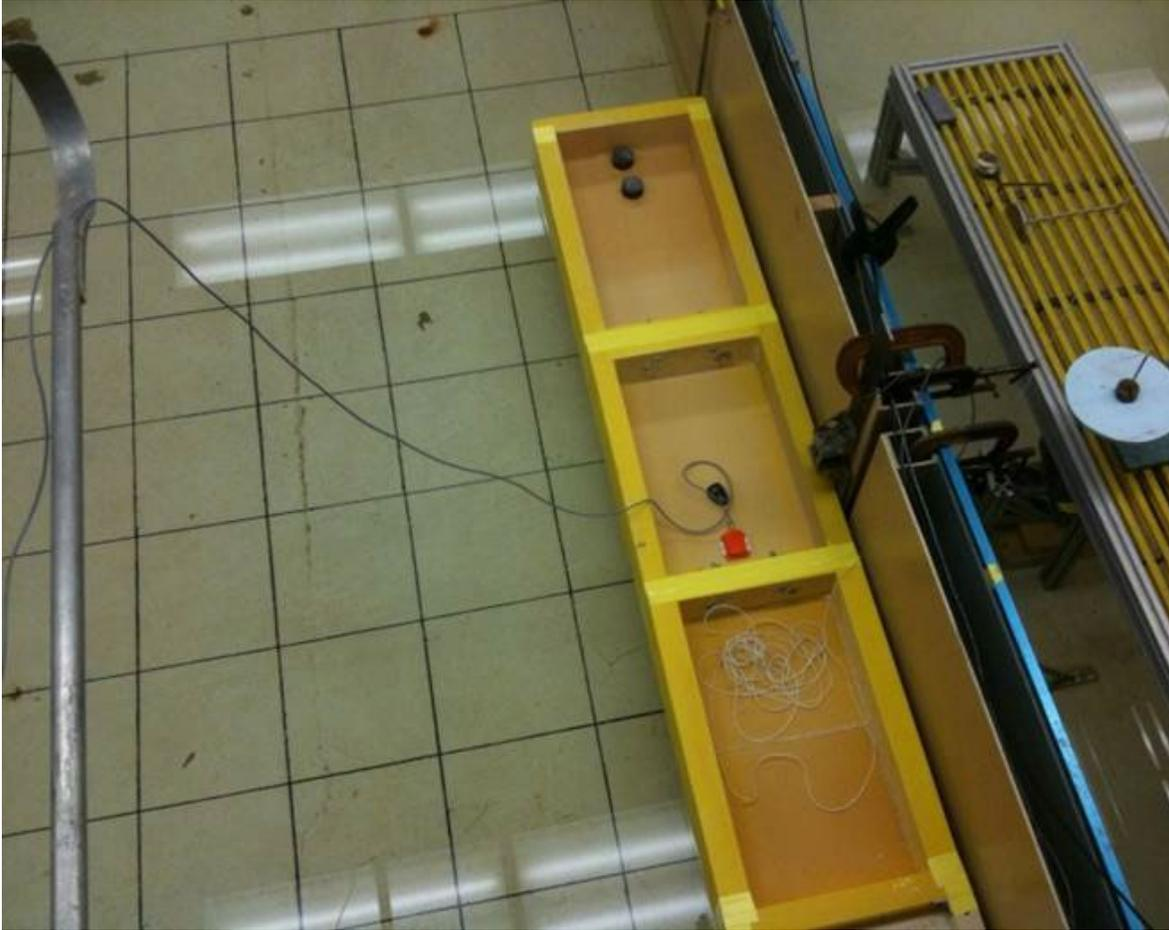
Figure G.9. Barge Model Resting Broadside Against Model Levee Floodwall, and Weight Pan for Constant Force Pulling
