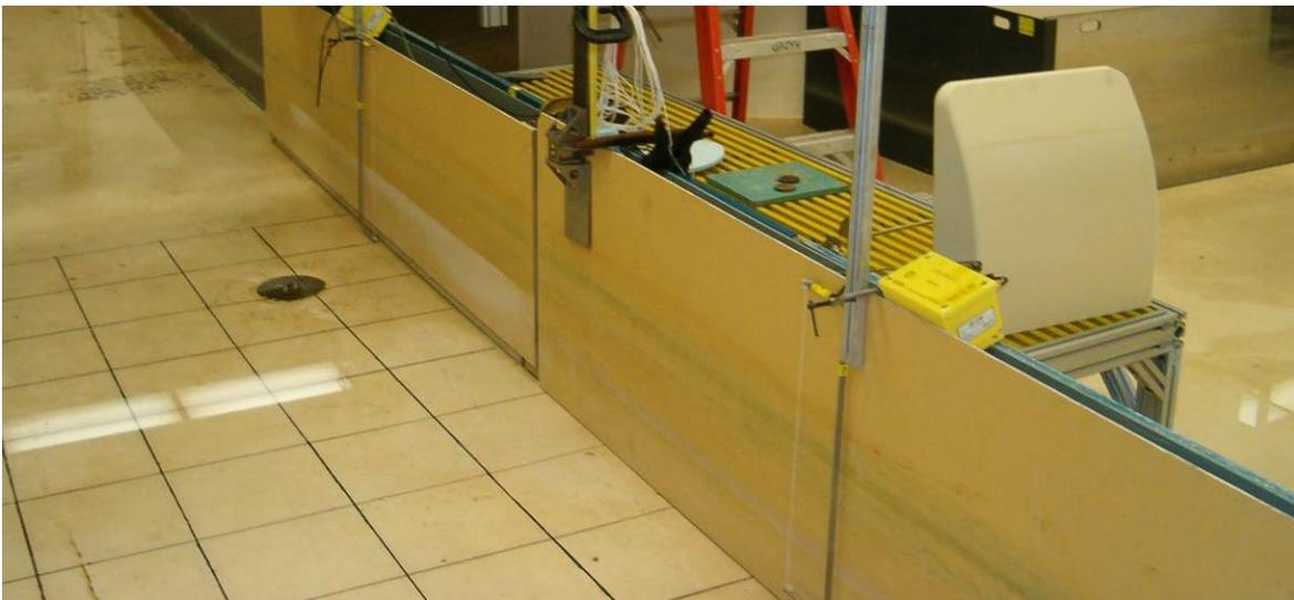
Figure G.8. Experimental Levee Floodwall, Shown with Wave Gauges and Force Gauge in Place and 1-ft by 1-ft Grid on Floor of Coastal Basin
