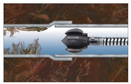
(From General Pipe Cleaners, 2019) Figure 7-3. Root auger within pipe.
