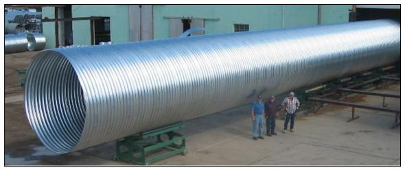
(Courtesy of National Corrugated Steel Pipe Association) Figure 3-3. Large CSP at manufacturing facility.
