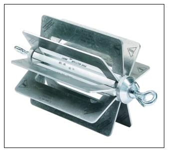
(From Sewer Equipment Company of Florida, 2020) Figure 5-58. New pipe mandrel for small to medium sized pipes.
