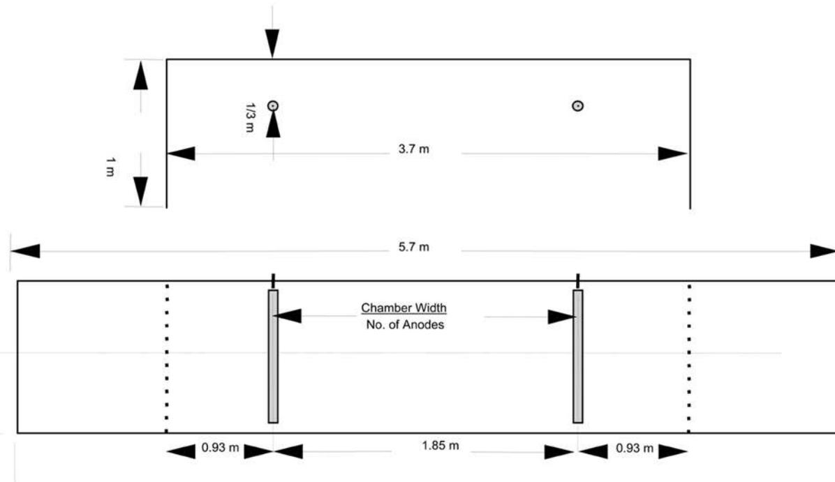
Figure D.6. Rod Galvanic Anode Locations in Largest Downstream Chambers
