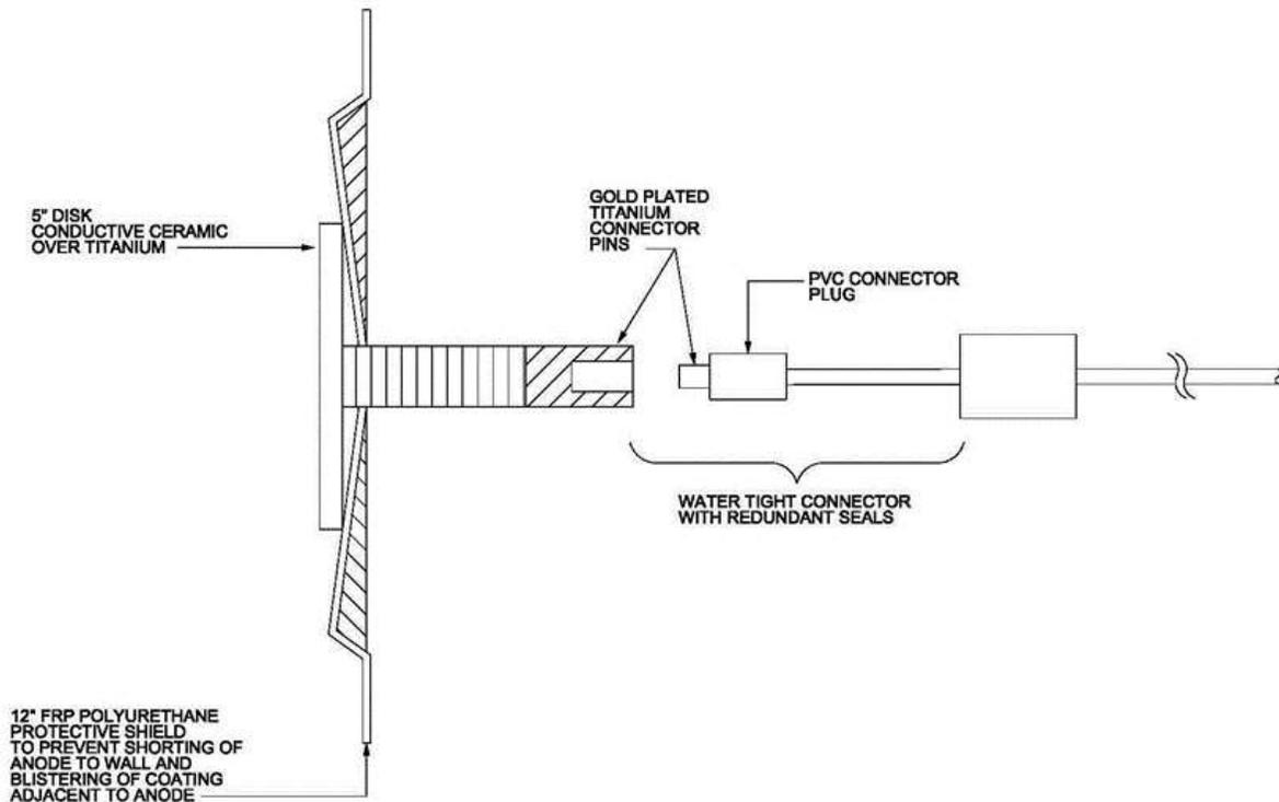
Figure 2.3. Ceramic Coated Flat Disk Anode
