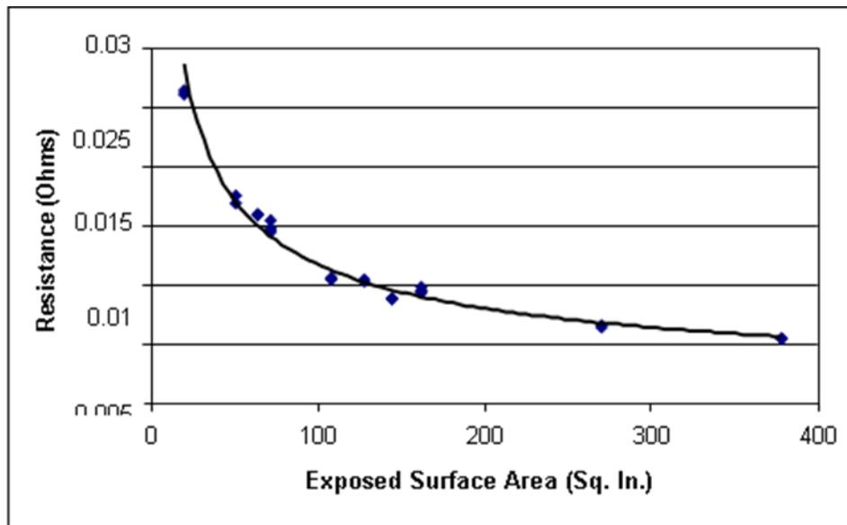
Figure B.1. Resistance vs. Anode Surface Area Normalized for 1 ohm-cm Resistivity Water
