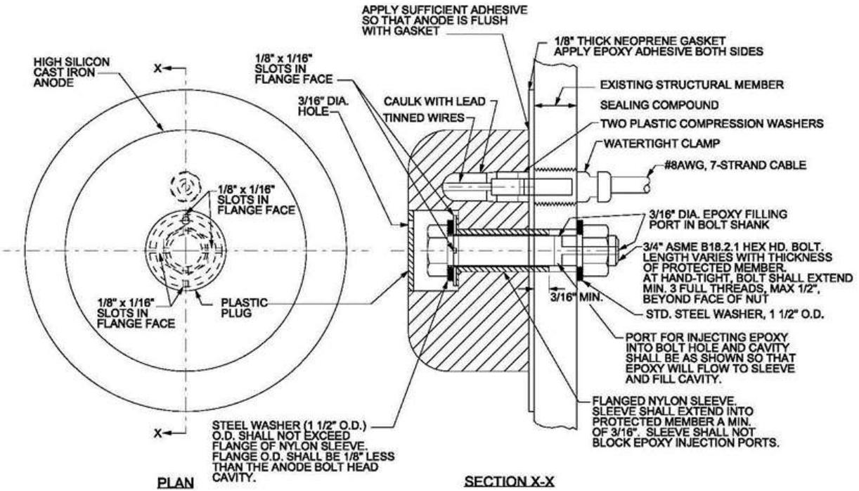
Figure 2.2. High Silicon Cast Iron (HSCI) Button Anode
