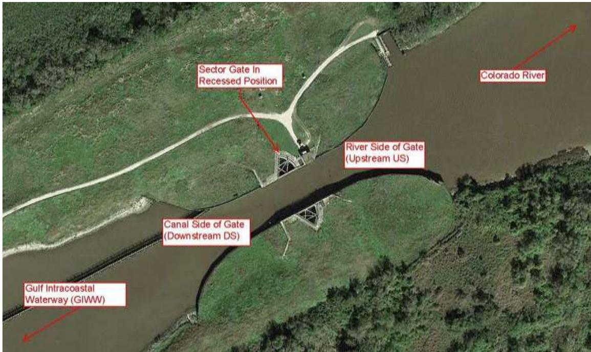
Figure G.2. Enlarged View of Colorado River Lock Sector Gate (Typical of Four)
