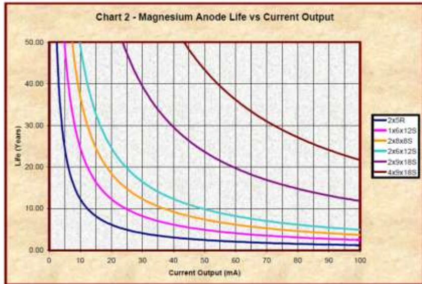
Figure B.2. Magnesium Anode Life vs. Current Output
