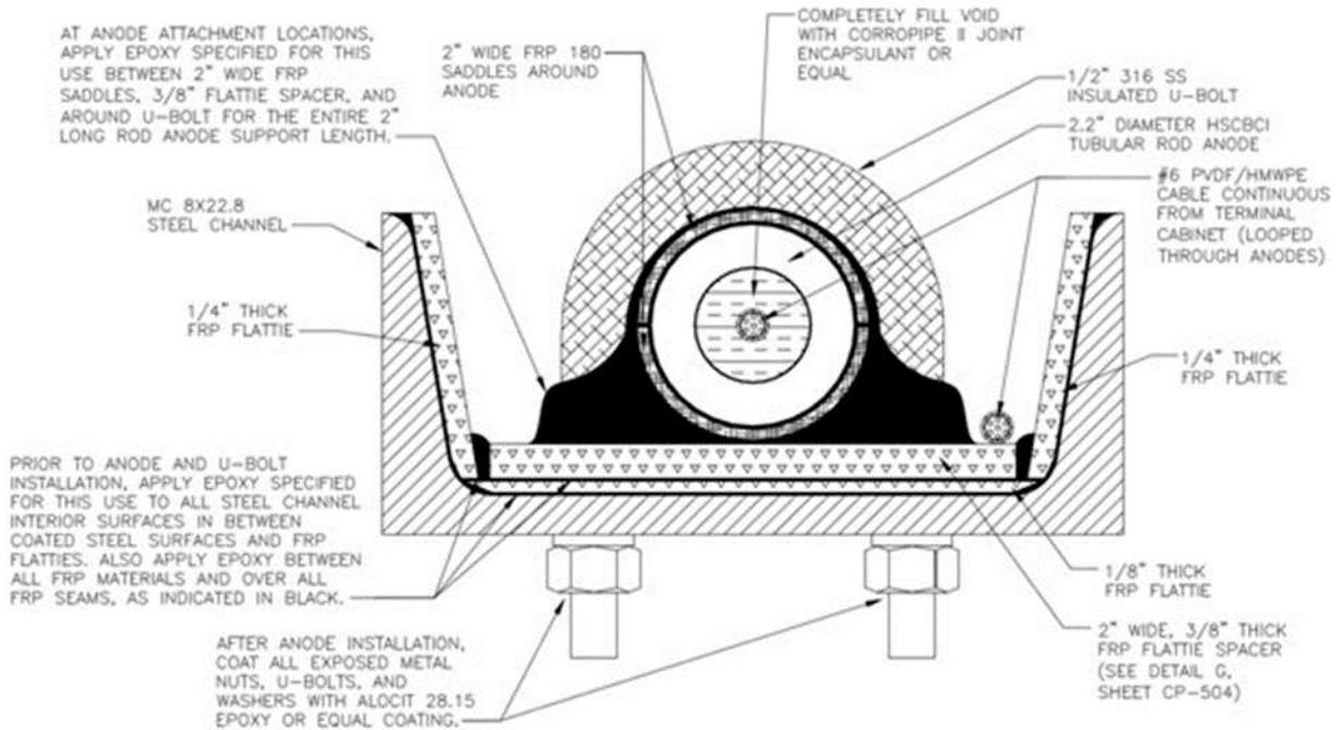
Figure G.7. Cross-Sectional View of Anode Assembly
