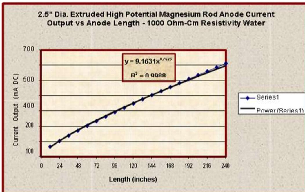
Figure D.3. Current Output vs. Anode Length for 2.5-Inch Diameter High-Potential Magnesium Rod Anodes
