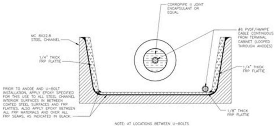
Figure G.8. Cross-Sectional View of Anode Assembly (Locations between U-Bolts)
