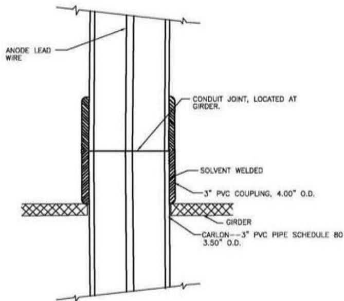
Figure 4.2. Anode Protection Pipe Girder Penetration
