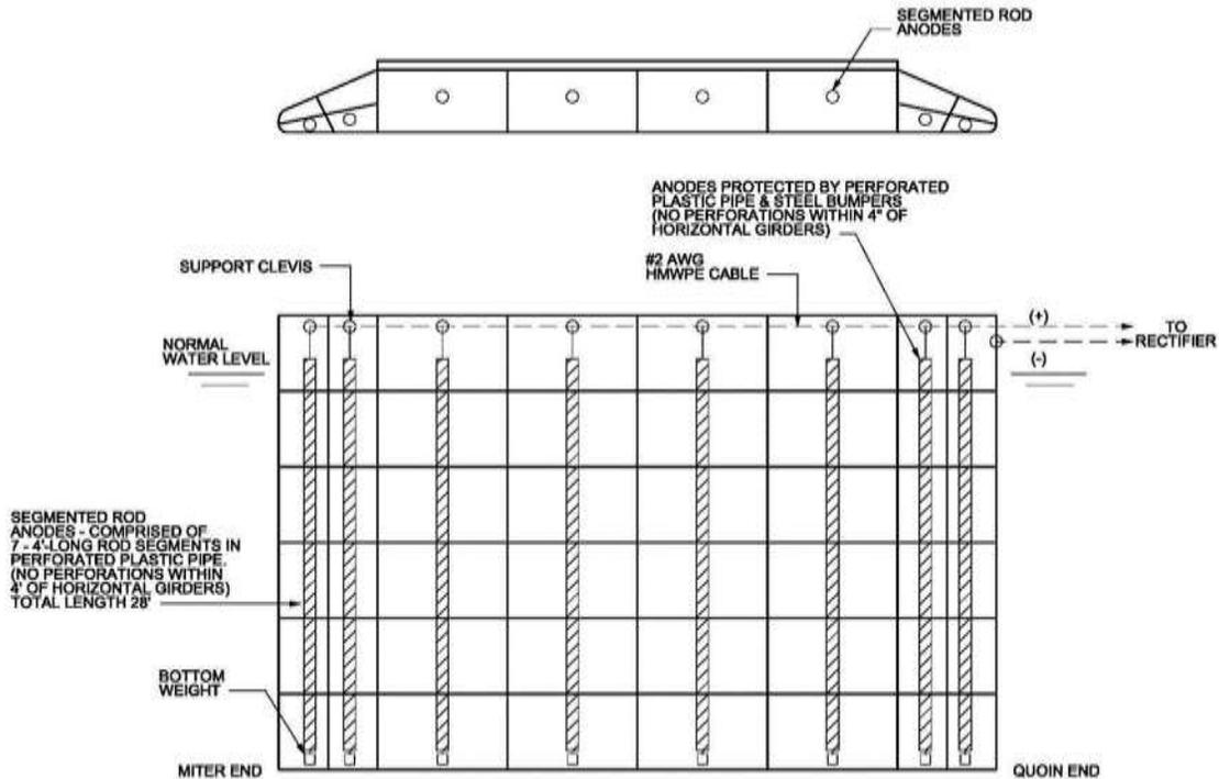
Figure E.3. Auxiliary Lock Miter Gate at Pike Island Showing Rod Anode Placement
