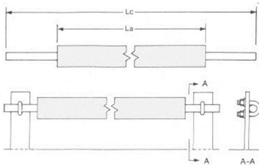
Figure D.5. Connection Schematic for High-Purity Cast Zinc Bar Anodes
