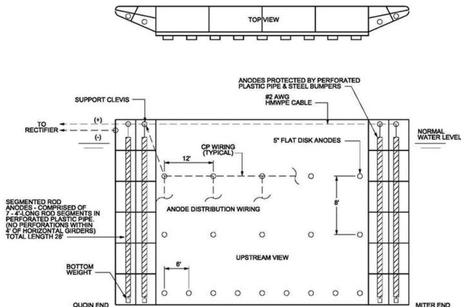
Figure E.2. Auxiliary Lock Miter Gate Design at Pike Island
