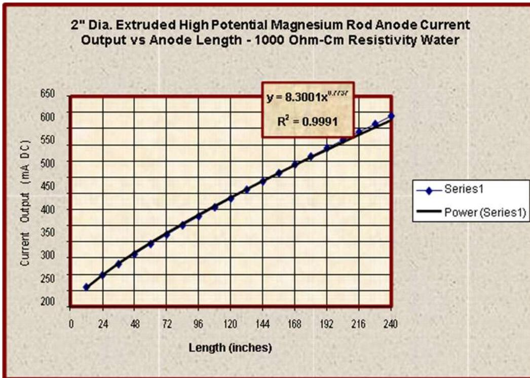
Figure D.2. Current Output vs. Anode Length for 2-Inch Diameter High-Potential Magnesium Rod Anodes
