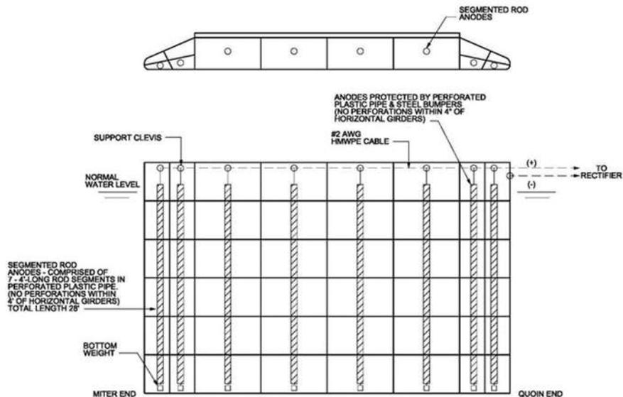
Figure E.1. Pike Island Auxiliary Lock Miter Gate
