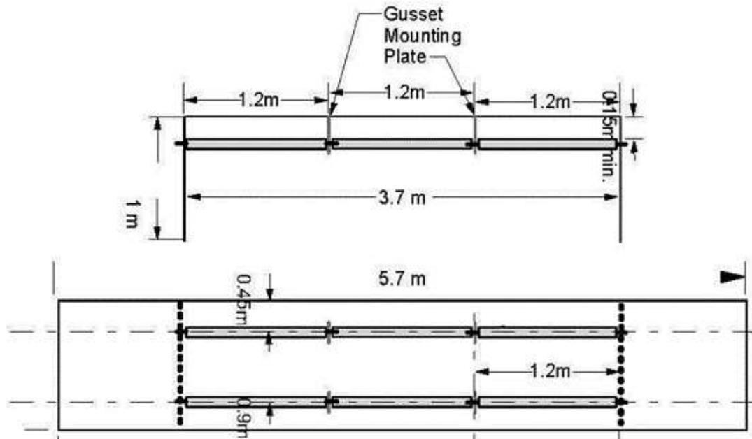
Figure D.7. Zinc Bar Galvanic Anode Locations in Largest Downstream Gate Chambers
