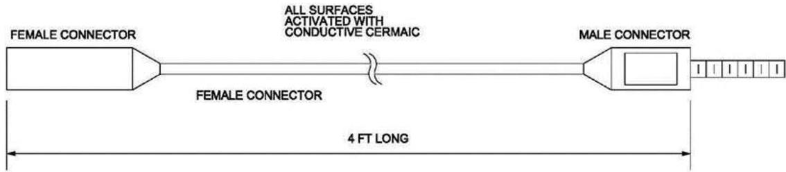
Figure 2.4. Rod Anode Segment
