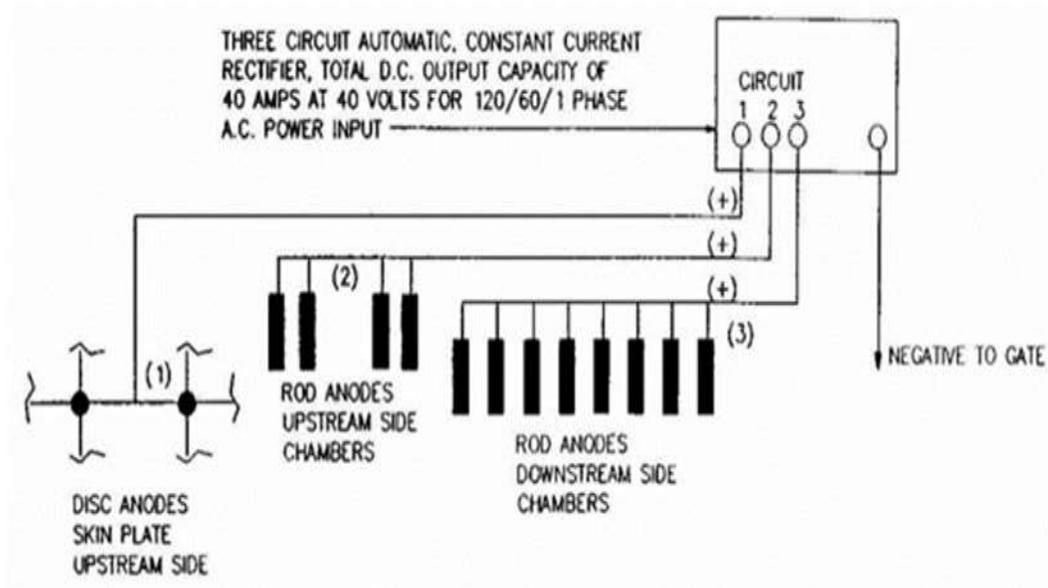
Figure E.4. Circuit Diagram for Lock Miter Gate
