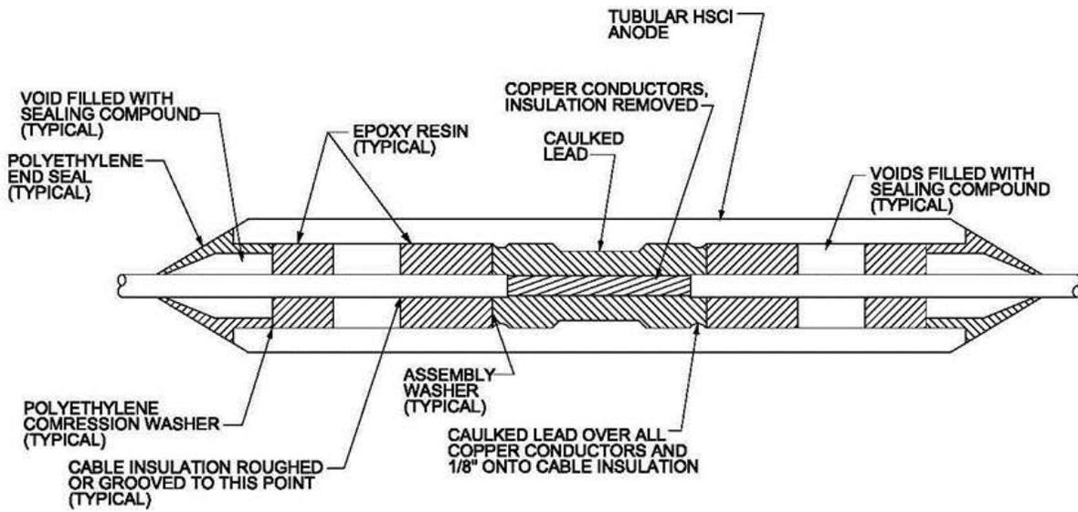
Figure 2.5. High Silicon Cast Iron Sausage or String Anode
