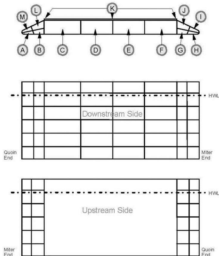
Figure C.1. Lock Gate Vertical, Downstream, and Upstream Structural Layout
