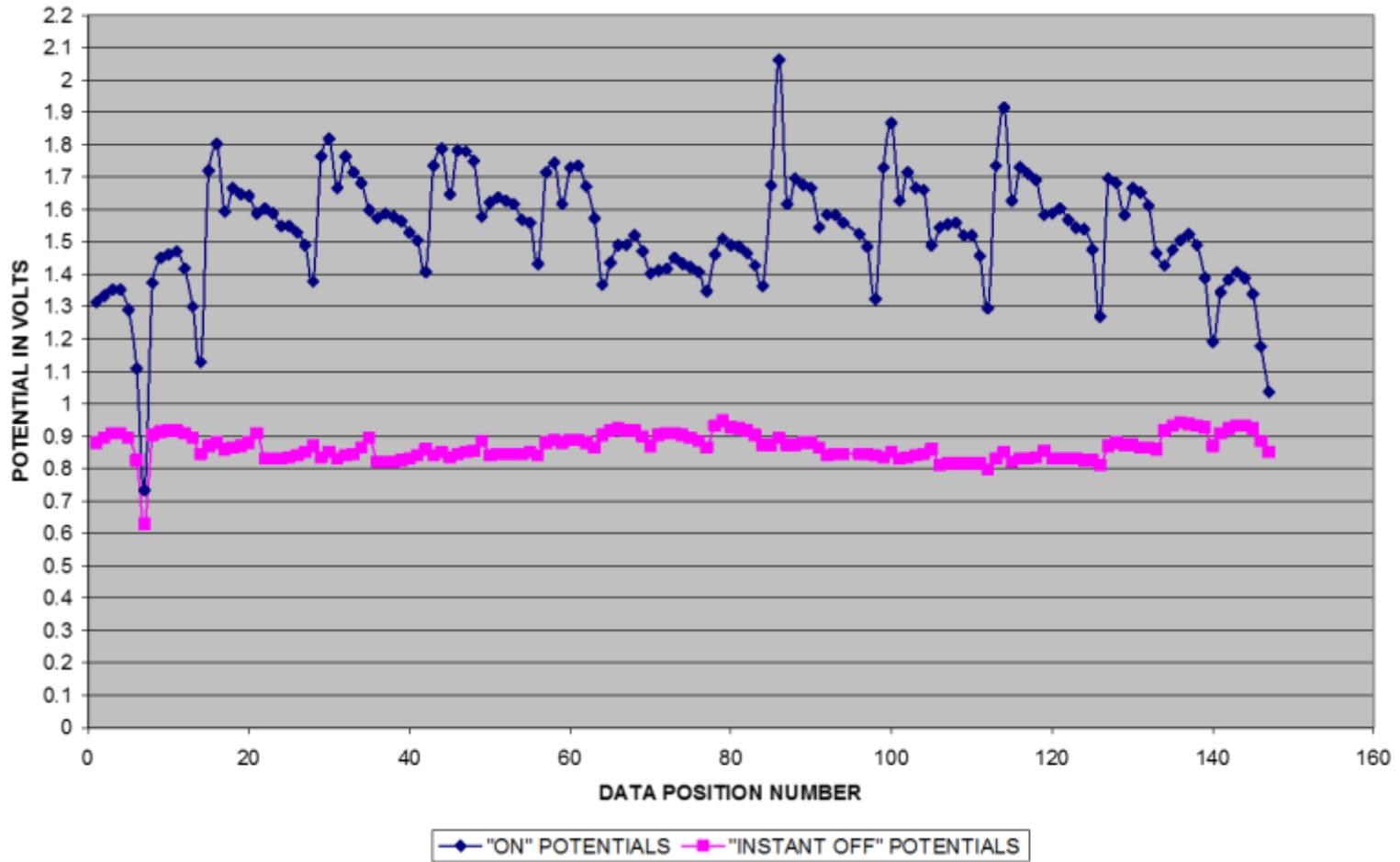
Figure I.1. Oliver Lock Upper Gates Upstream Side, 2007 Data
