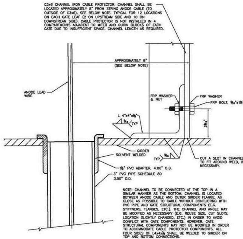
Figure 4.1. Anode Protection Pipe Upper Girder Termination
