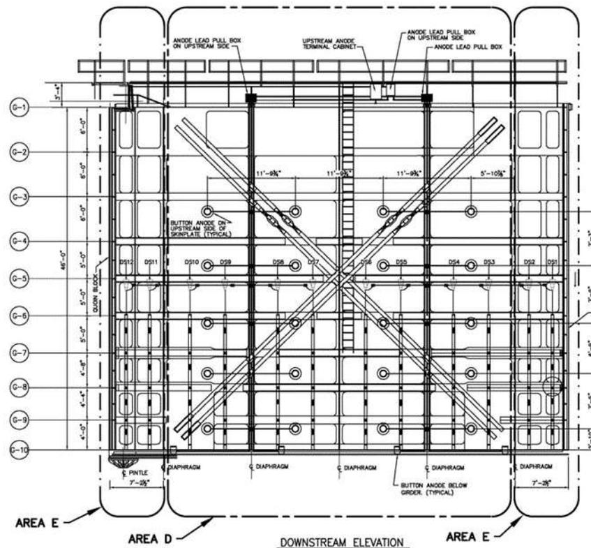
Figure F.1. Downstream Elevation of Selden Lower Lock Gate
