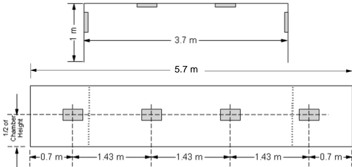
Figure C.2. Galvanic Slab Anode Locations in Largest Downstream Gate Chambers
