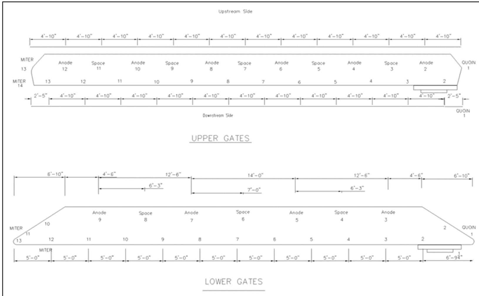
Figure J.10. Schematic View of Demopolis Lock Upper and Lower Gates
