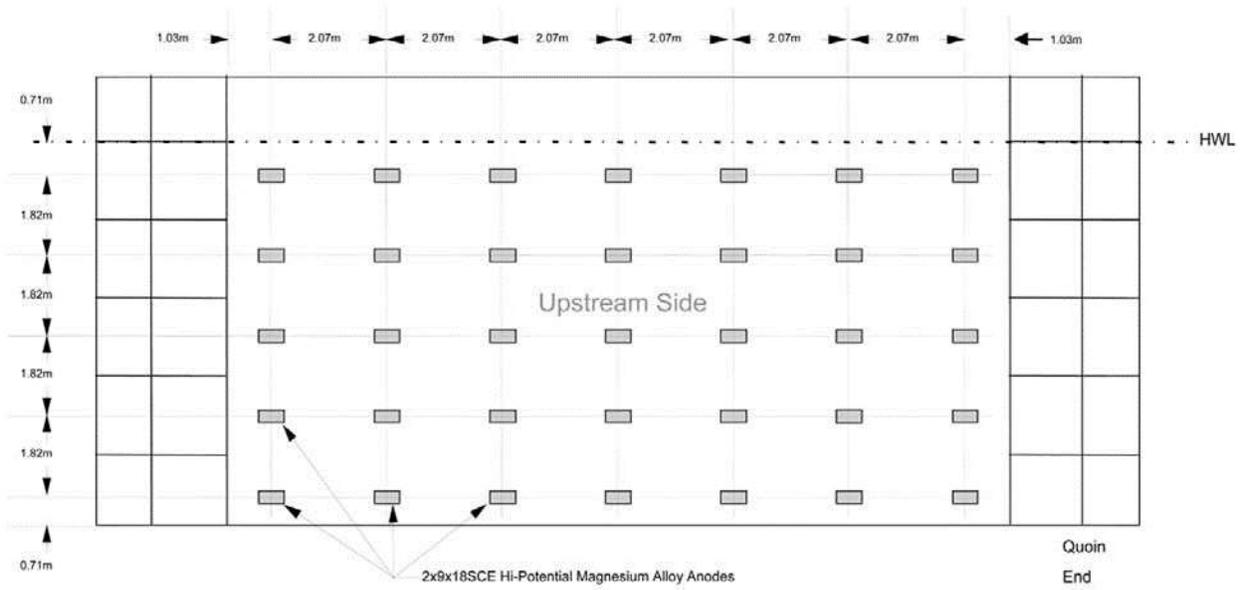
Figure C.3. Example Slab Anode Layout for Upstream Side (Skin Plate)
