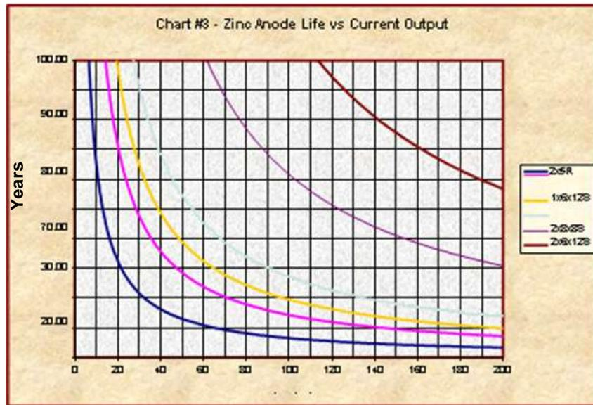
Figure B.3. Zinc Anode Life vs. Current Output
