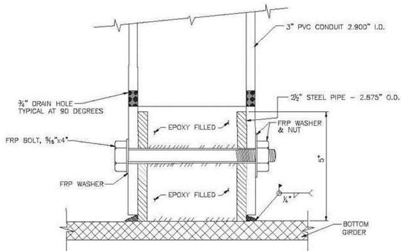
Figure 4.3. Anode Protection Pipe Bottom Girder Termination
