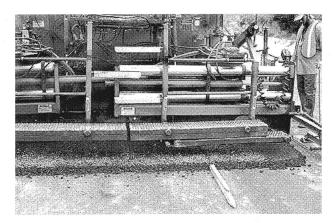
FIGURE 15-21 Hydraulically extendable screed.
