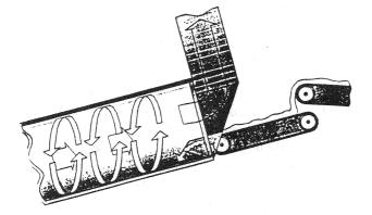
FIGURE 9-2 Typical Slinger conveyors for aggregate delivery.
