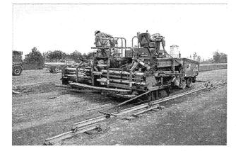
FIGURE 16-6 Floating-beam mobile reference with shoes at ends of beam.
