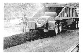
FIGURE 13-2 Typical bottom- or belly-dump truck.
