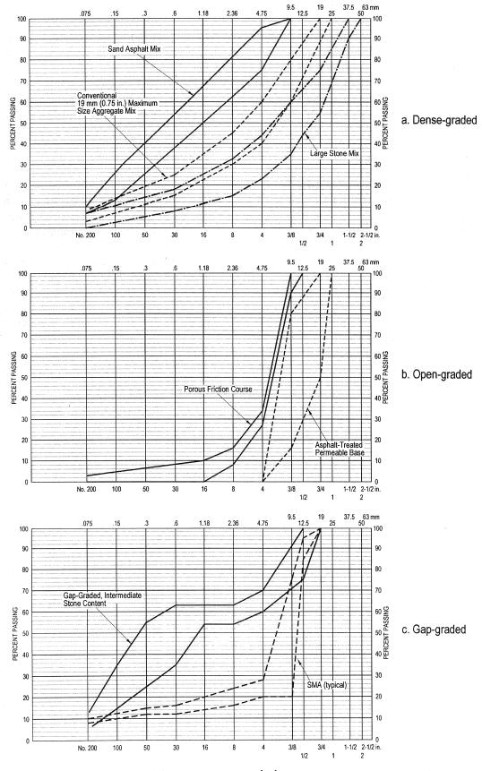
FIGURE 1-1 Representative aggregate gradations.
