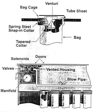
FIGURE 12-9 How bags are mounted to cage, sealed to tube sheet, and installed in baghouse.
