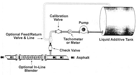
FIGURE 7-4 Typical asphalt additive tank system.
