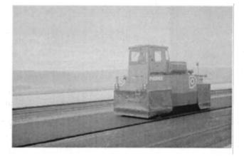
FIGURE 18-5 Pneumatic tire roller with skirts.
