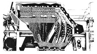
FIGURE 8-3 Cutaway illustration of screening process.
