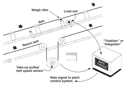
FIGURE 6-10 How a weigh bridge works.
