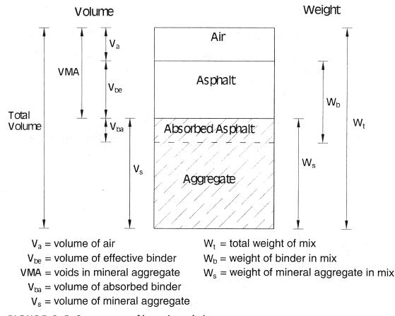
FIGURE 3-5 Components of hot-mix asphalt.
