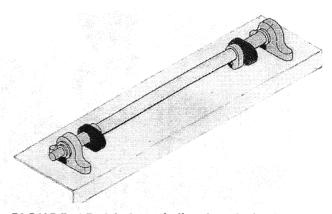
FIGURE 15-16 Screed vibration shaft with weights.
