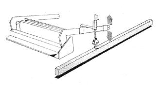
GRADE SENSOR MOUNTING POSITION #1-SIDE ARM MOUNT
