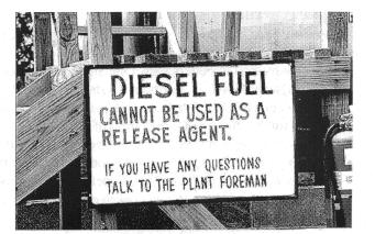
FIGURE 13-6 Diesel fuel is an unacceptable release agent.
