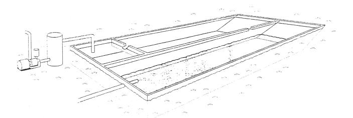
FIGURE 12-6 Typical settling pond.
