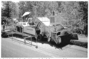
FIGURE 13-3 Material pickup machine.
