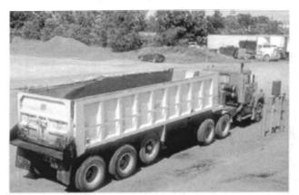
FIGURE 13-1 Typical end-dump truck.
