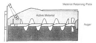
FIGURE 15-9 Schematic of paver auger.
