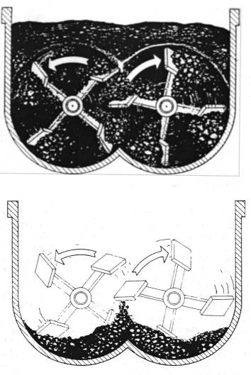
FIGURE 8-5 Overfilled and underfilled pugmills.
