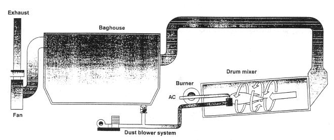
FIGURE 9-8 Pneumatic transfer to mixing area of drum.
