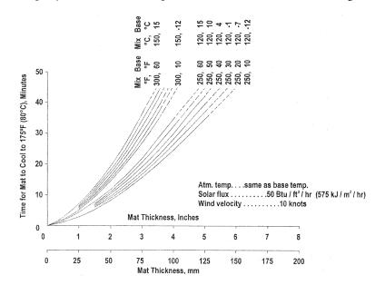
FIGURE 18-1 Time for mat to cool to 80°C (175°F) versus mat thickness for lines of constant mix and base temperatures [121°C (250°F) or 149°C (300°F) behind paver].
