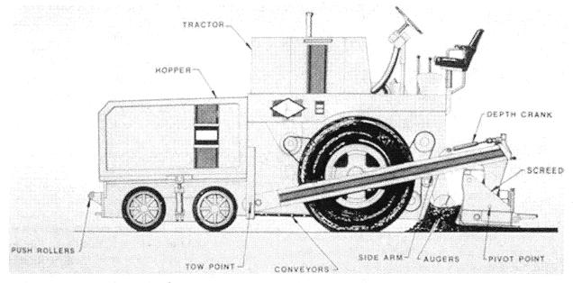
FIGURE 15-1 Schematic of HMA paver.
