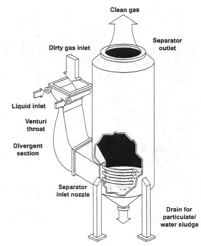
FIGURE 12-5 Flow through typical venturi scrubber.
