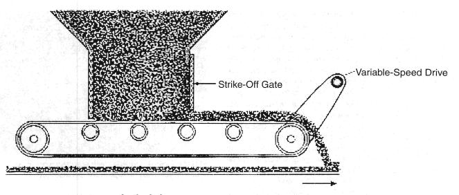
FIGURE 6-5 Continuous feeder belt.
