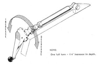
FIGURE 16-1 Thickness control crank.
