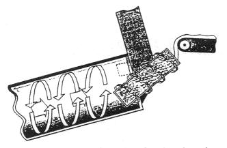
FIGURE 9-1 Typical rotating charging chute for delivery of new aggregate.
