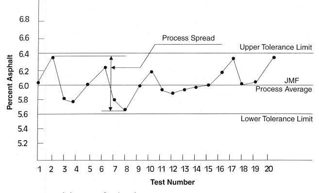
FIGURE 4-2 Asphalt content of paving mixture.
