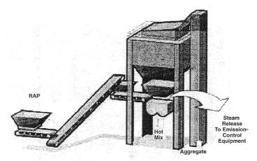
FIGURE 8-6 Weigh-box method of batch plant recycling.
