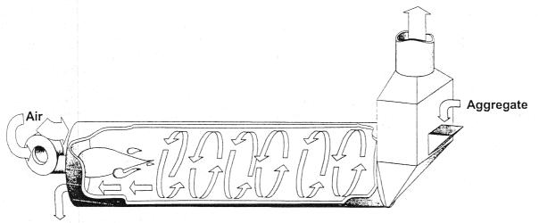
Aggregate FIGURE 8-1 Typical counter-flow dryer.
