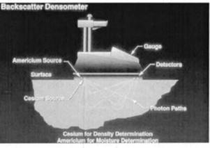
FIGURE 18-8 Schematic of nuclear gauge.
