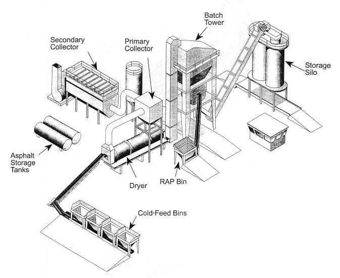
FIGURE 5-2 Major components of a batch plant.
