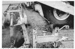
FIGURE 15-8 Paver auger.
