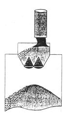
FIGURE 11-6 Segregation caused by feeding batcher off center.
