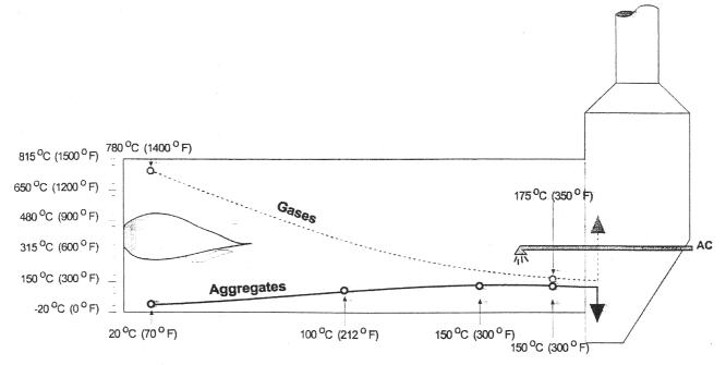
FIGURE 9-5 Temperature profile for parallel-flow drum drying aggregate.
