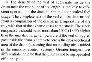
The presence of light-brown, uncoated fine aggregate on one side of the mix in the discharge chute is also an indication that the veil of aggregate is incomplete across the drum circumference.
