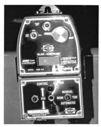
FIGURE 16-10 Slope-control device.
