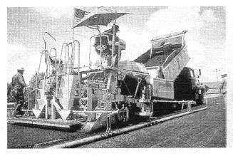
FIGURE 16-4 Paver with mobile reference employing rigid pipe.
