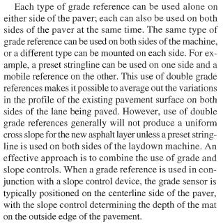
The grade sensor or wand is in contact with the reference in all but sonic systems. As the grade of the reference changes, the wand senses that change and sends an electrical signal to the control panel on the paver. A signal is then sent, in turn, to the tow points on either side of the paver, and their elevation is changed relative to the change sensed by the grade sensor.
