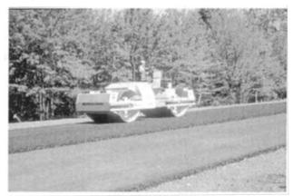
FIGURE 18-6 Vibratory steel wheel roller.
