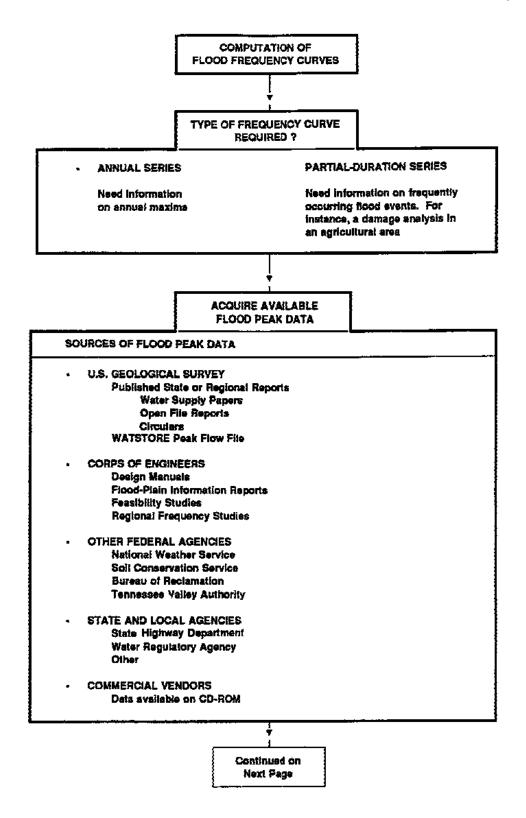
Figure 1. Flood frequency analysis flowchart (Continued)
