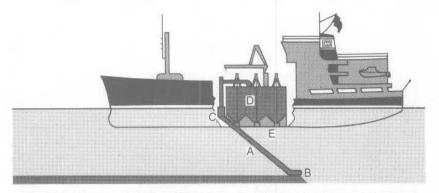
**Typical Hopper Dredge Components:** Hopper dredges are seagoing vessels designed to dredge and transport dredged material to open-water disposal areas. The working of a hopper dredge is similar to that of a home vacuum cleaner.
