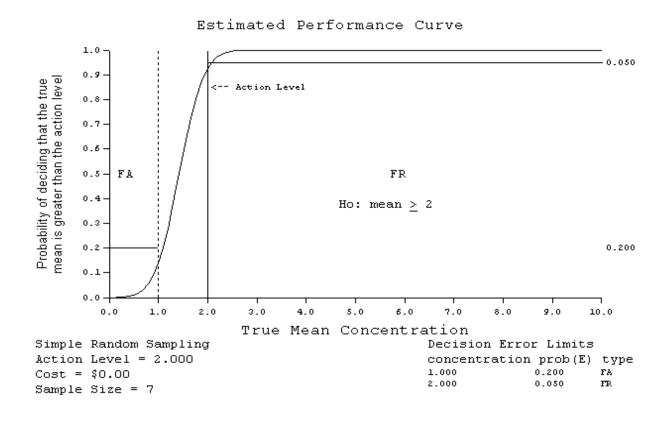
Figure L-2. Power Curve for the One-sample t-Test for Simple Random Sampling.
