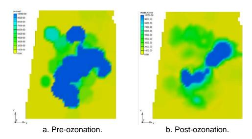
Figure R-2. Comparison of Krige-Interpolated Benzo(a)pyrene Concentrations before and after Treatment by In Situ Ozonation.
