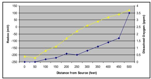
Figure 4-8. Geotechnical Parameters Versus Distance From Source. (yellow triangle-redox; blue diamond-dissolved oxygen.
