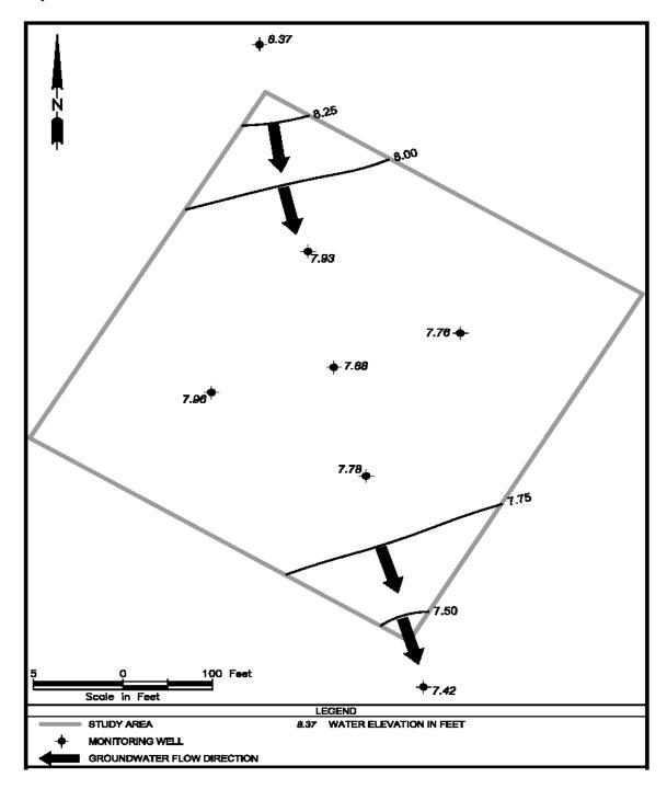
Figure J-24. Contour Plot Drawn by Modeling Software Using IDW.
