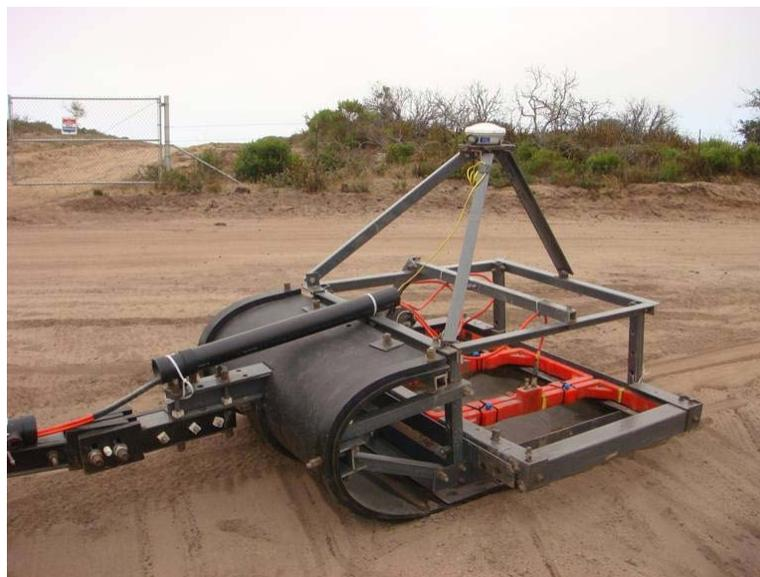
Figure 6-5: Example of a Towed TDEMI Array
