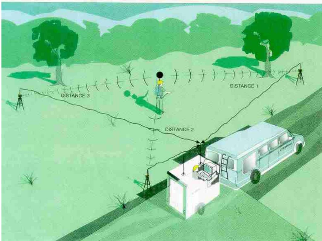
Figure 6-25: Example of an Acoustic Positioning System
