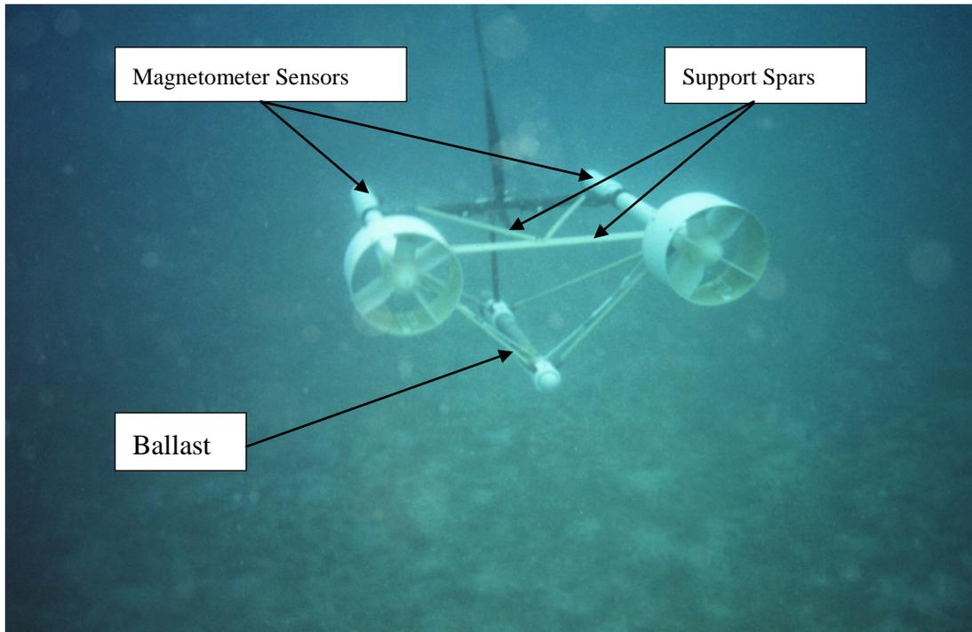
Figure 6-29: Example of an Underwater Geophysical System
