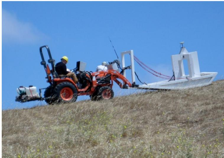
Figure 6-6: Geometrics MetalMapper™ Advanced EMI Sensor
