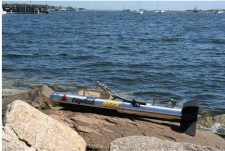
Figure 6-15: Example of an SSS Sensor
