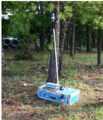
Figure 6-2: Geometrics G-856 Proton Precession Magnetometer
