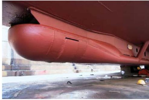
Figure 6-14: Example of an MBES Sensor
