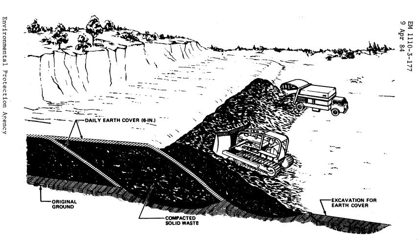
SOLID WASTES ARE SPREAD AND COMPACTED ON A SLOPE. THE DAILY CELL MAY BE COVERED WITH EARTH SCRAPED FROM THE BASE OF THE RAMP. THIS VARIATION IS USED WITH EITHER THE AREA OR TRENCH METHOD.
