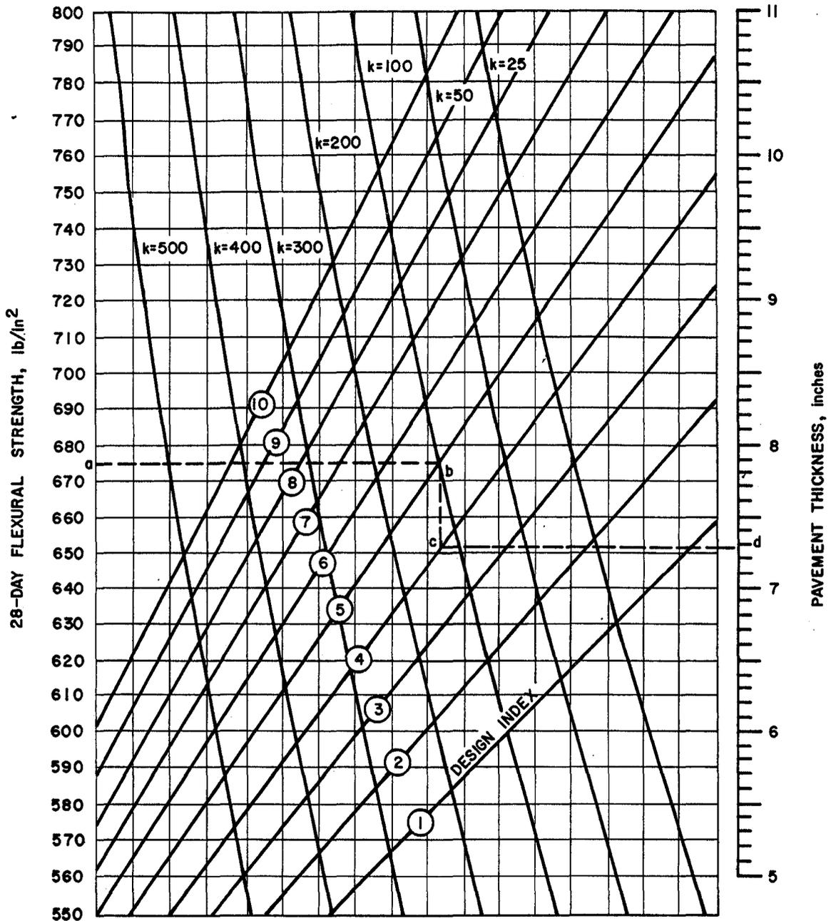
NOTE: Minimum allowable thickness of nonreinforced rigid pavement is 6 inches.
