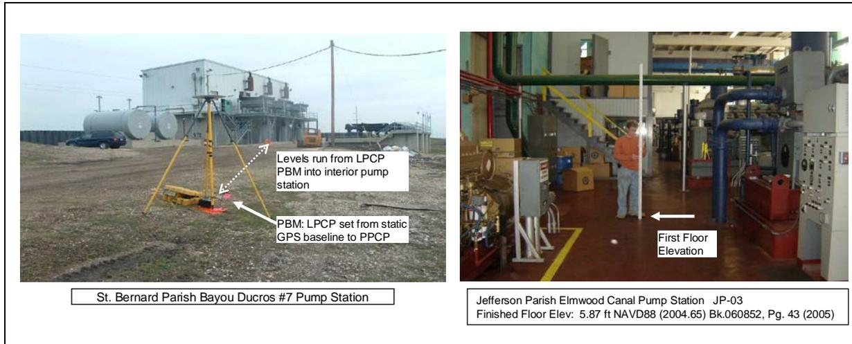
Figure 5-7. Referencing pump station elevations to NAVD88.
