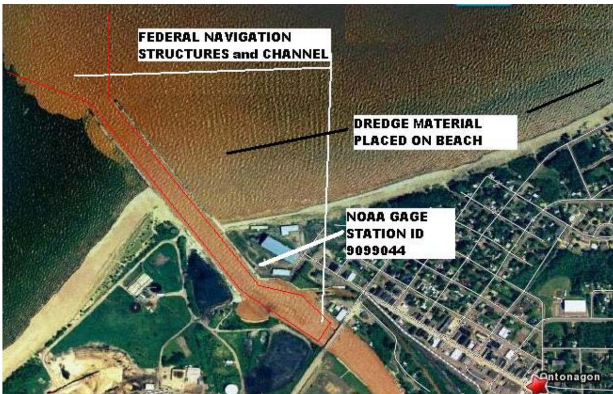
Figure K-2. Ontonagon Harbor Michigan – Structure and federal navigation channel.
