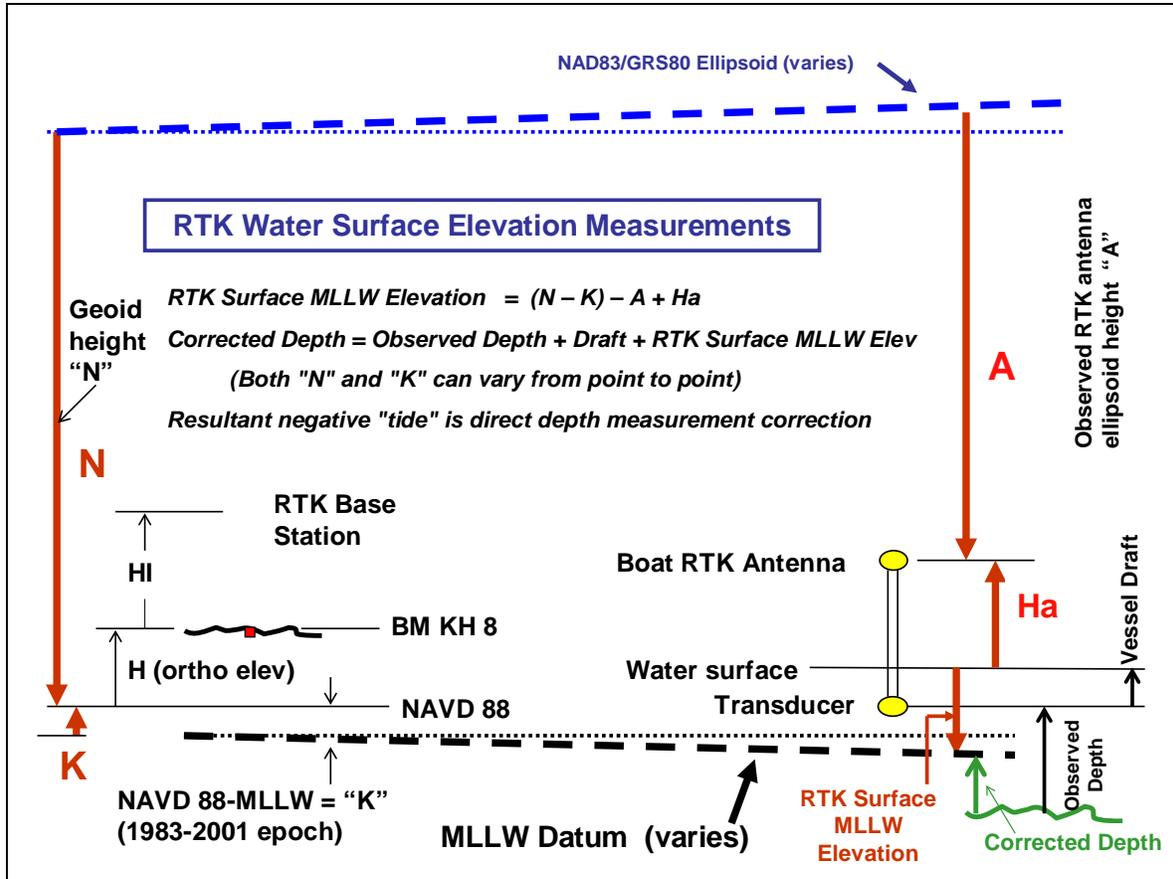
Figure 4-12. RTK Ellipsoid-Tidal-Geoid parameters for water surface elevation measurements.
