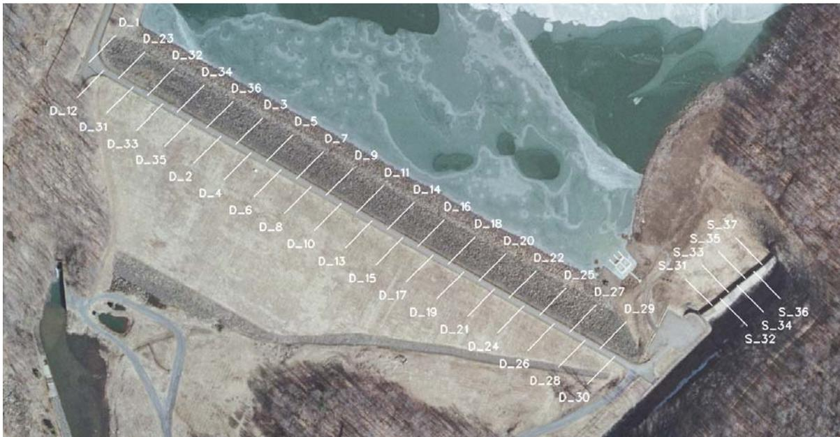
Figure H-7. Dam and Spillway Profile Stations displayed with 2006 PaMAP Ortho Imagery.
