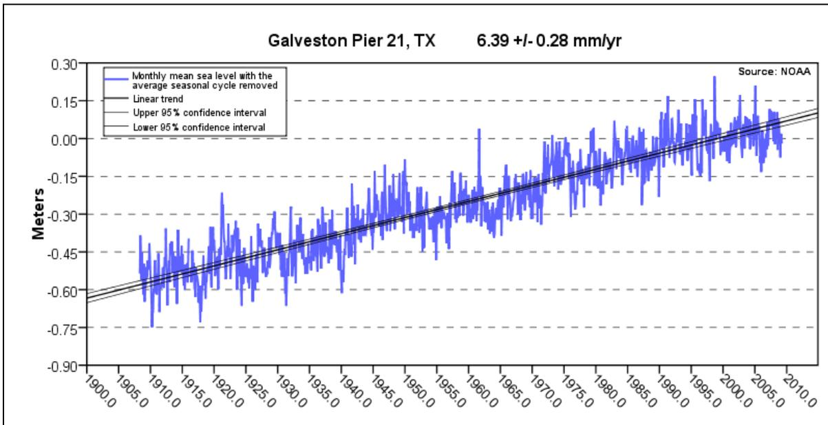
Figure M-6. The mean sea level trend for Galveston, Texas is 6.39 millimeters/year with a 95% confidence interval of +/- 0.28 mm/yr based on monthly mean sea level data from 1908 to 2006, which is equivalent to a change of 2.10 feet in 100 years.
