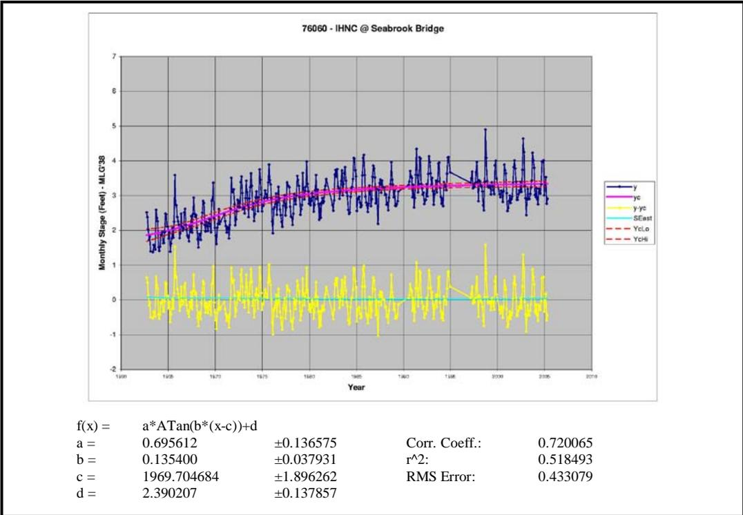
Figure L-17. Arctangent function fit to the monthly means Gage 76060 IHNC @ Seabrook Bridge.
