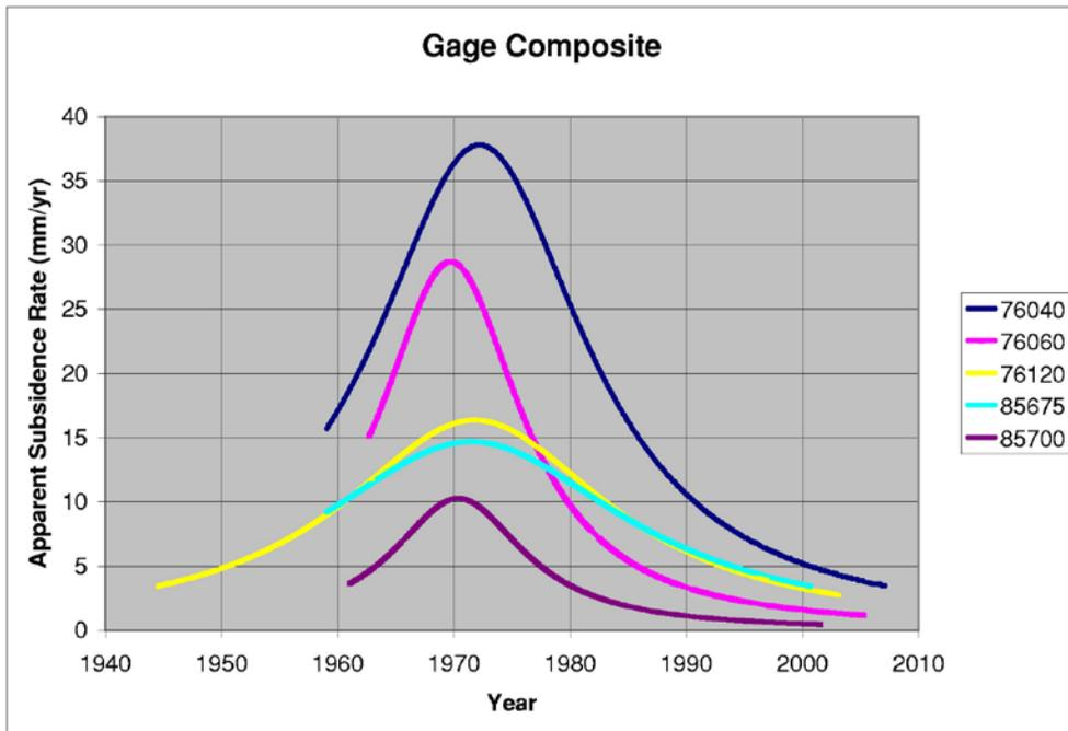
Figure L-26. Composite graph of estimated instantaneous rate of apparent subsidence for all gages.
