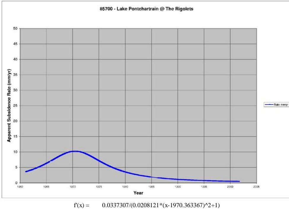
Figure L-25. Estimated instantaneous rate of apparent subsidence for Gage 85700 Lake Pontchartrain @ The Rigolets.
