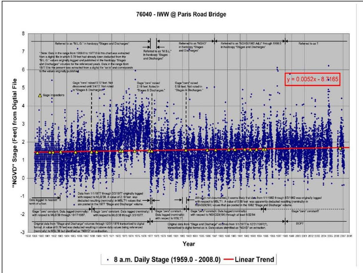
Figure L-4. Gage readings for gage 76040 – IWW @ Paris Road.
