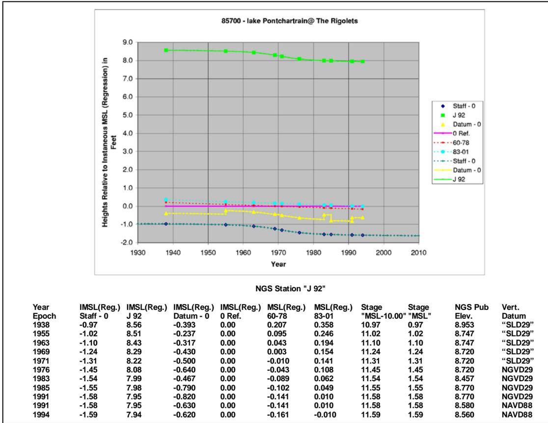
Figure L-30. Estimates of the relationships among the geodetic and tidal datum epochs at Gage 85700 Lake Pontchartrain @ The Rigolets.
