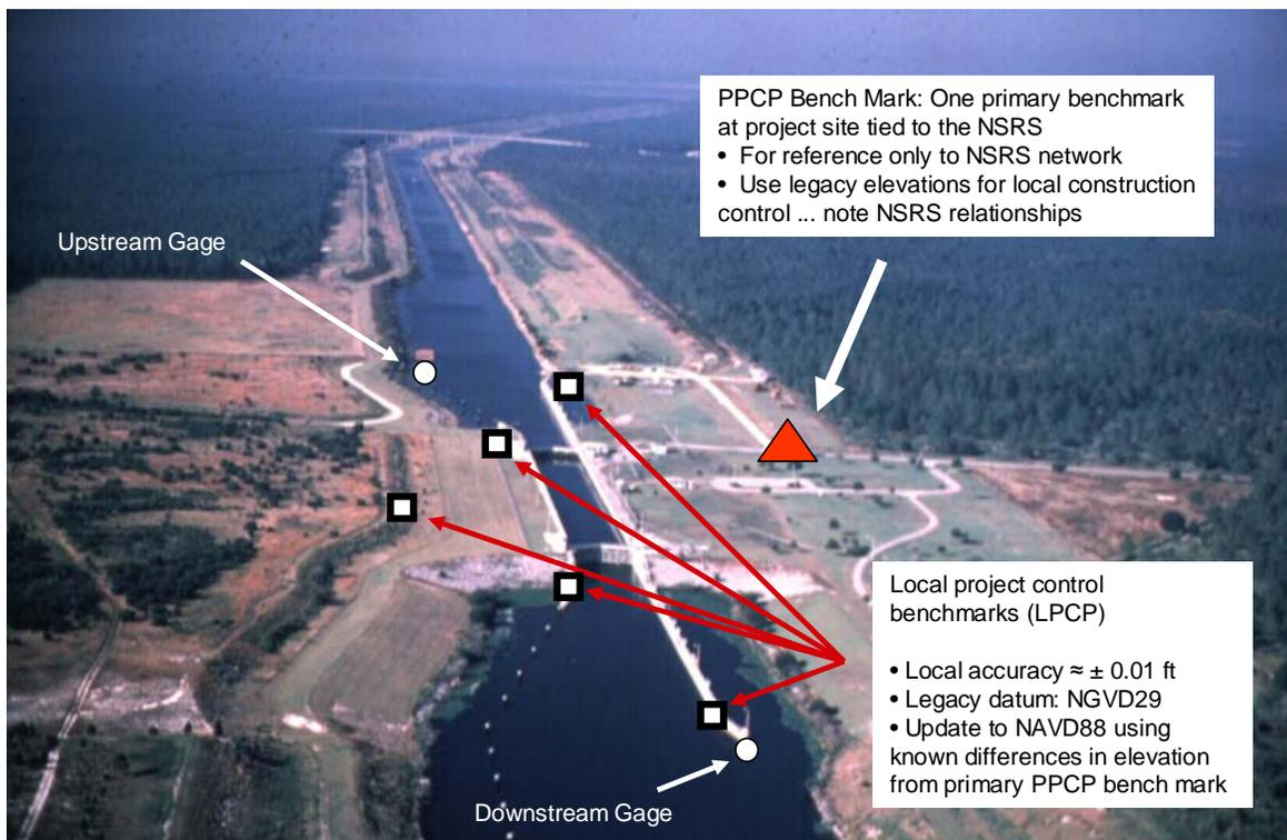
Figure 6-5. NSRS connections at an inland lock project.
