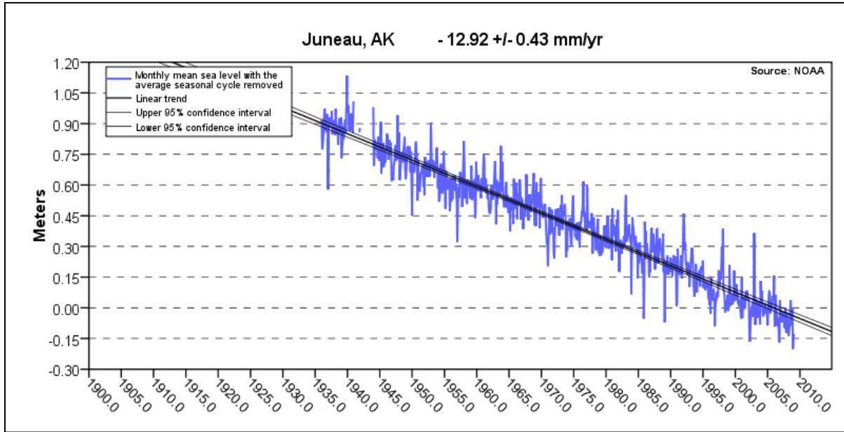
Figure M-5. The mean sea level trend for Juneau, Alaska is -12.92 millimeters/year with a 95% confidence interval of +/- 0.43 mm/yr based on monthly mean sea level data from 1936 to 2006, which is equivalent to a change of -4.24 feet in 100 years.
