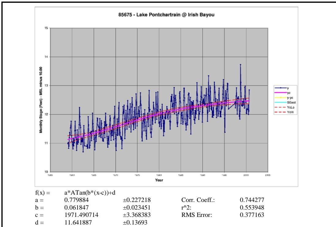
Figure L-19. Arctangent function fit to the monthly means for Gage 85675 Lake Pontchartrain @ Irish Bayou.
