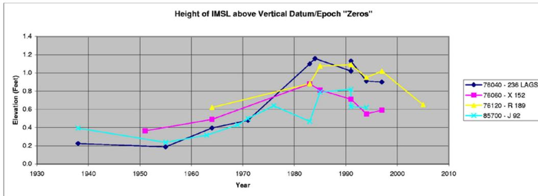
Figure L-31. Elevation of local instantaneous mean sea level with respect to geodetic datum zero as defined by referenced control monuments and associated elevations for given datum and epoch identified in Tables L-2 though L-5.
