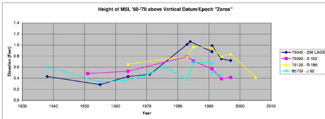
Figure L-32. Elevation of local mean sea level (NTDE 60-78) with respect to geodetic datum zero as defined by referenced control monuments and associated elevations for given datum and epoch identified in Tables L-2 though L-5.
