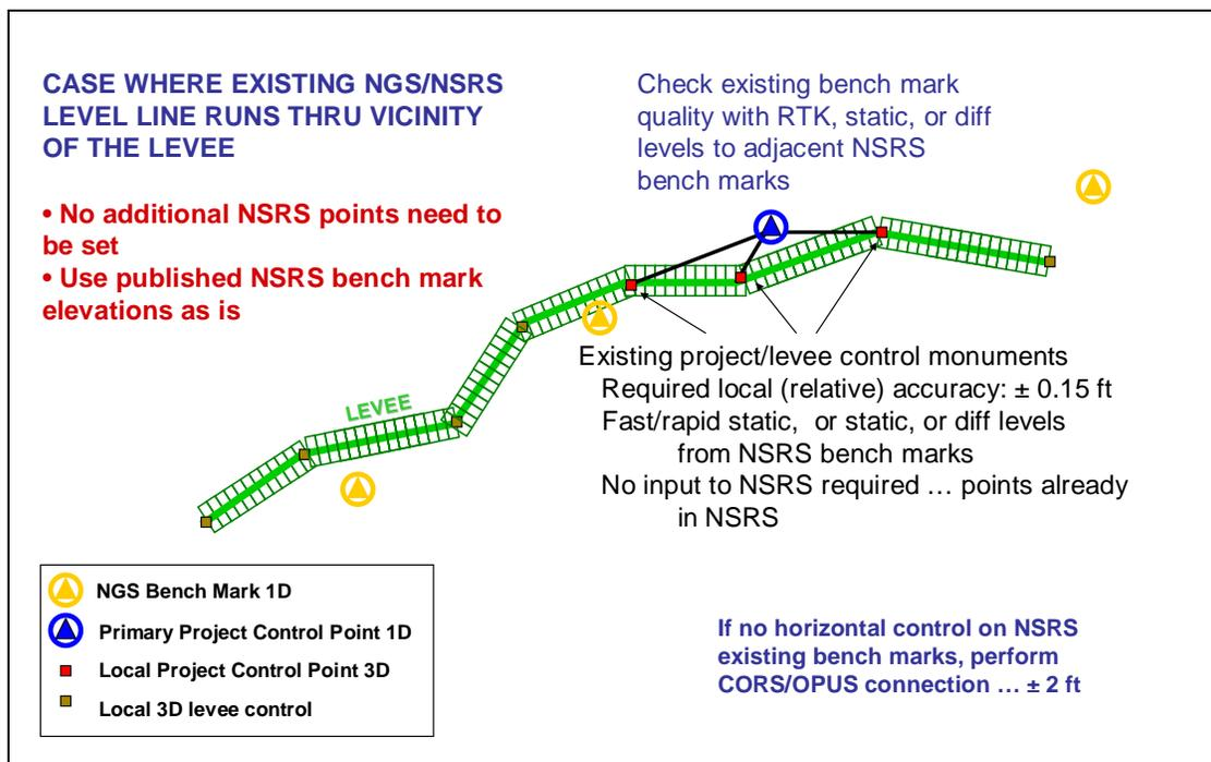
Figure 3-2. Published NSRS control within a levee project.
