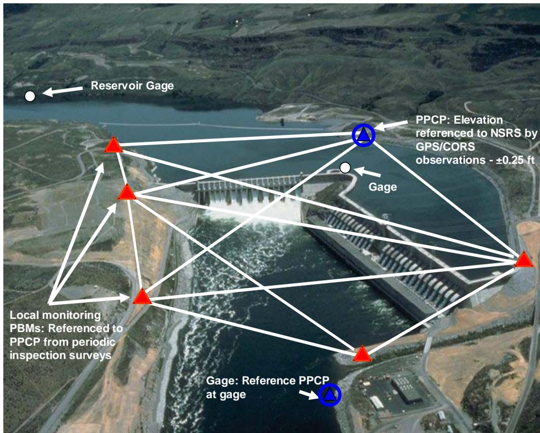
Figure 6-4. NSRS connections at a multipurpose hydropower project.
