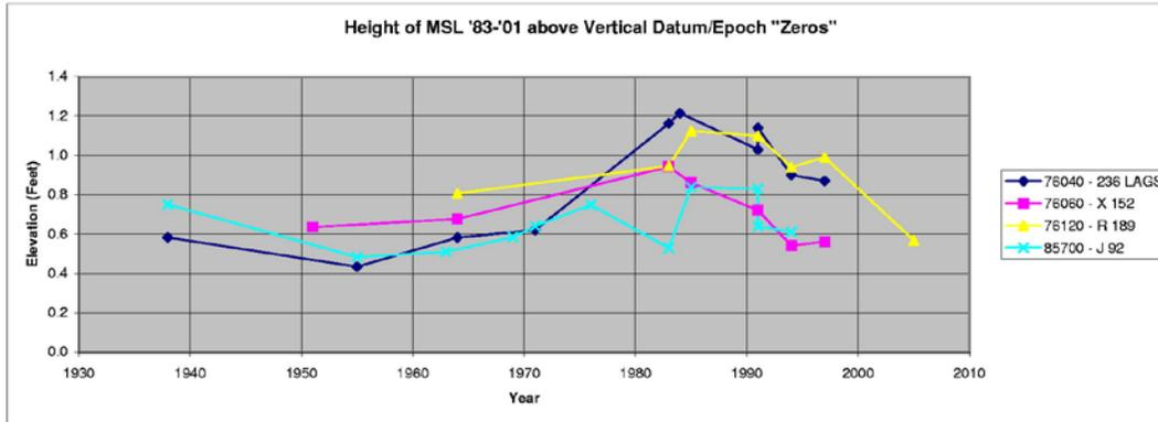
Figure L-33. Elevation of local mean sea level (NTDE 83-01) with respect to geodetic datum zero as defined by referenced control monuments and associated elevations for given datum and epoch identified in Tables L-2 though L-5.
