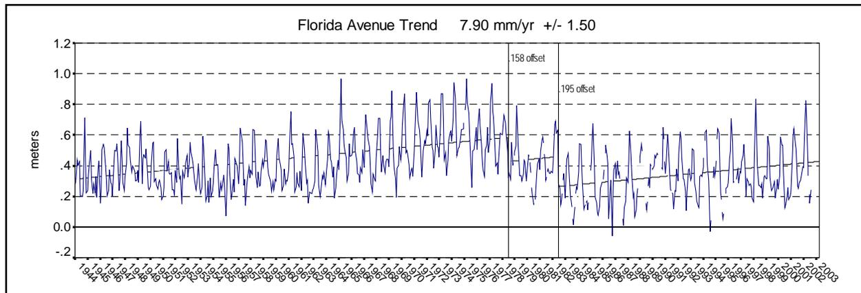
Figure 8-8. Apparent sea level rise at Corps IHNC Florida Ave. gage from 1944 to 2003. Gage zero adjustments were estimated. (IPET 2007)
