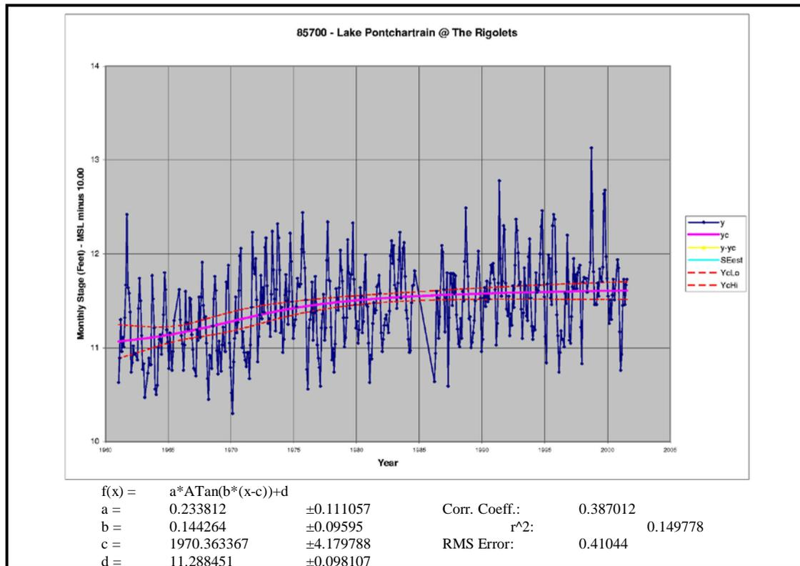
Figure L-20. Arctangent function fit to the monthly means for Gage 85700 Lake Pontchartrain @ The Rigolets.
