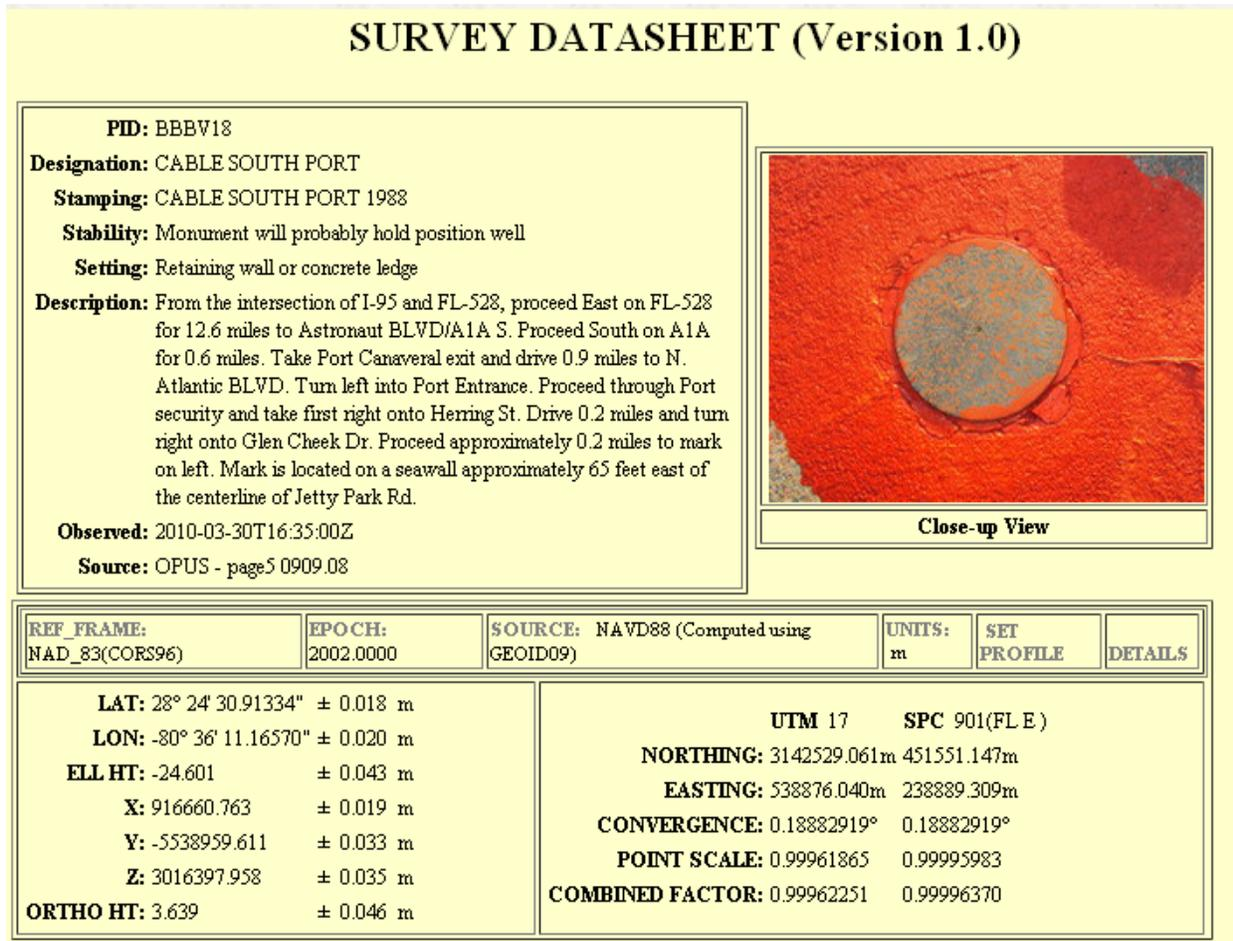
Figure F-13. Portion of NSRS Datasheet for USACE PPCP "CABLE SOUTH PORT."
