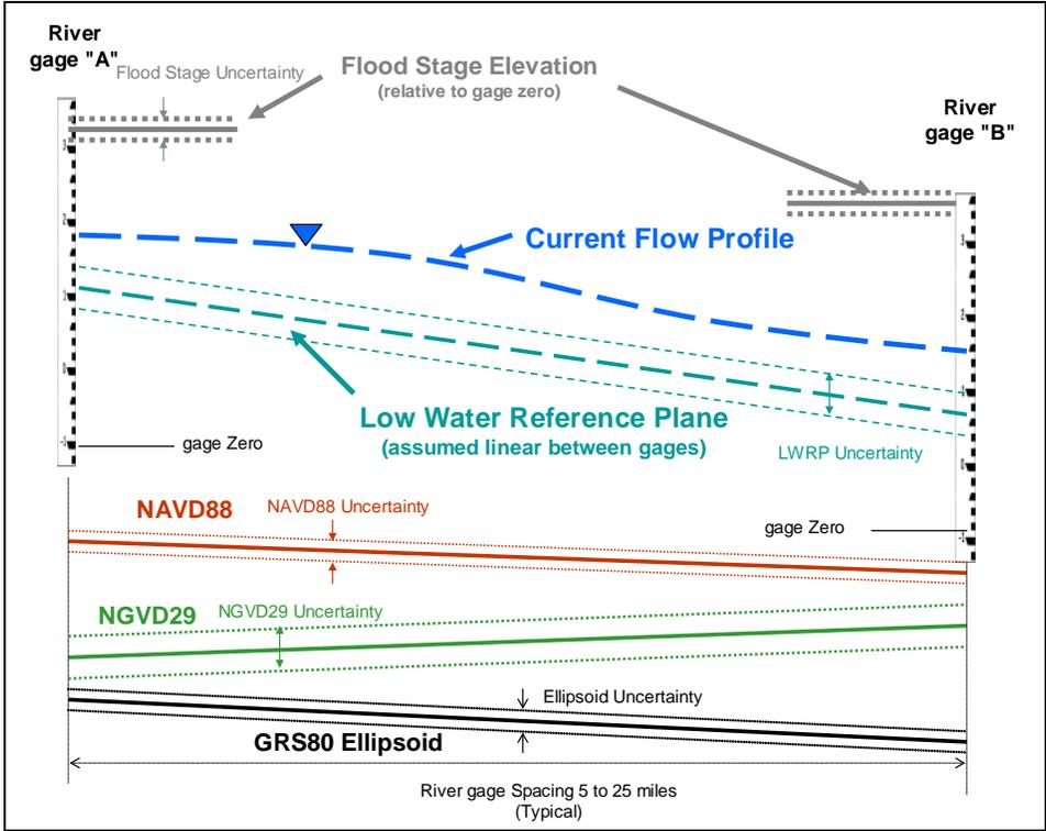
Figure 1-2. Design and protection height considerations and uncertainties due to vertical reference datum variations at gages on an inland river system. (Not to scale)
