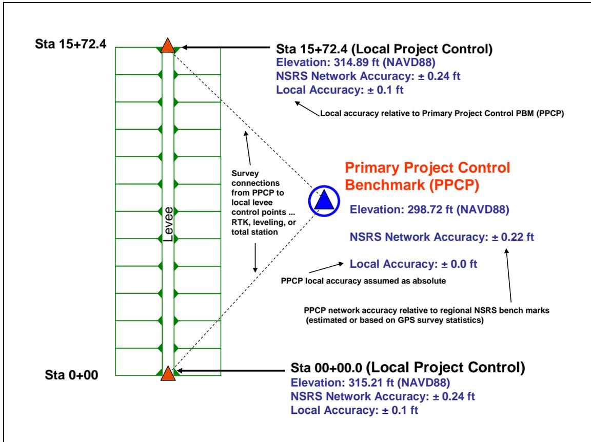
Figure 3-1. Distinction between Primary Project Control and Local Project Control points on a simple levee segment-- Network and Local Accuracies.
