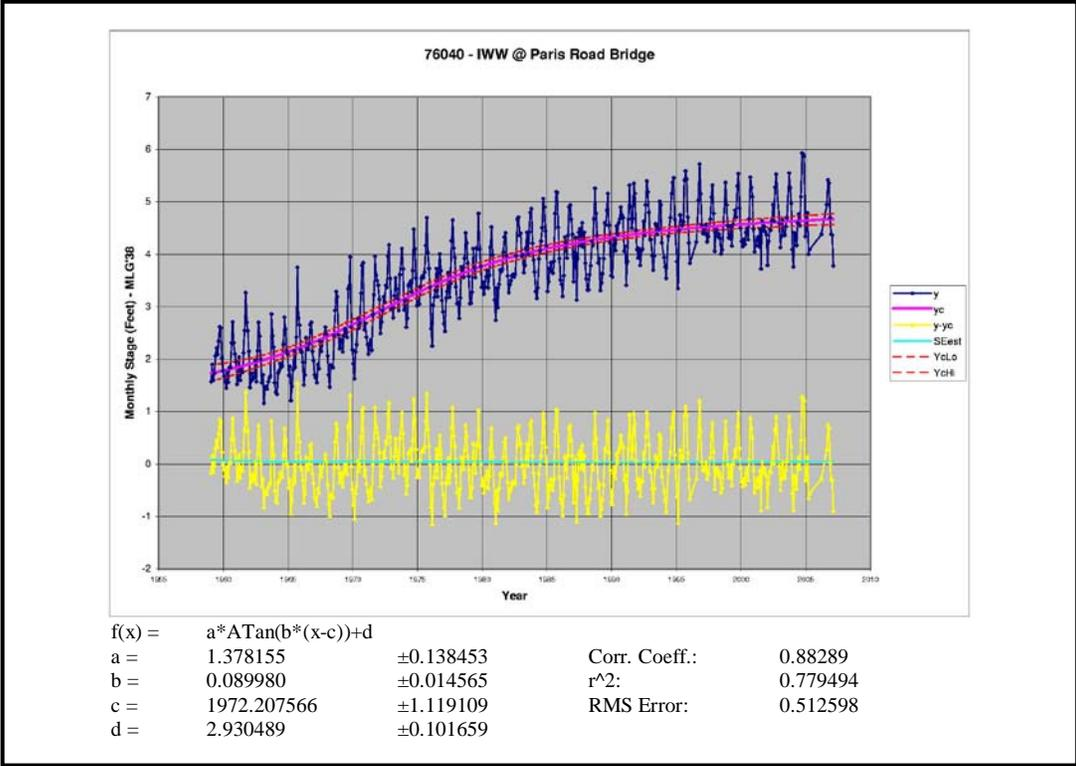
Figure L-16. Arctangent function fit to the monthly means for Gage 76040 IWW @ Paris Road Bridge.
