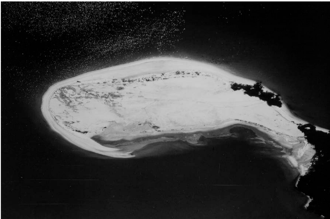
Figure 5-35. An Addition Built by the Jacksonville District, in Cooperation with the National Audubon Society, to Sunken Island in Hillsborough Bay, FL, During Maintenance Dredging Operations in the 1970s
