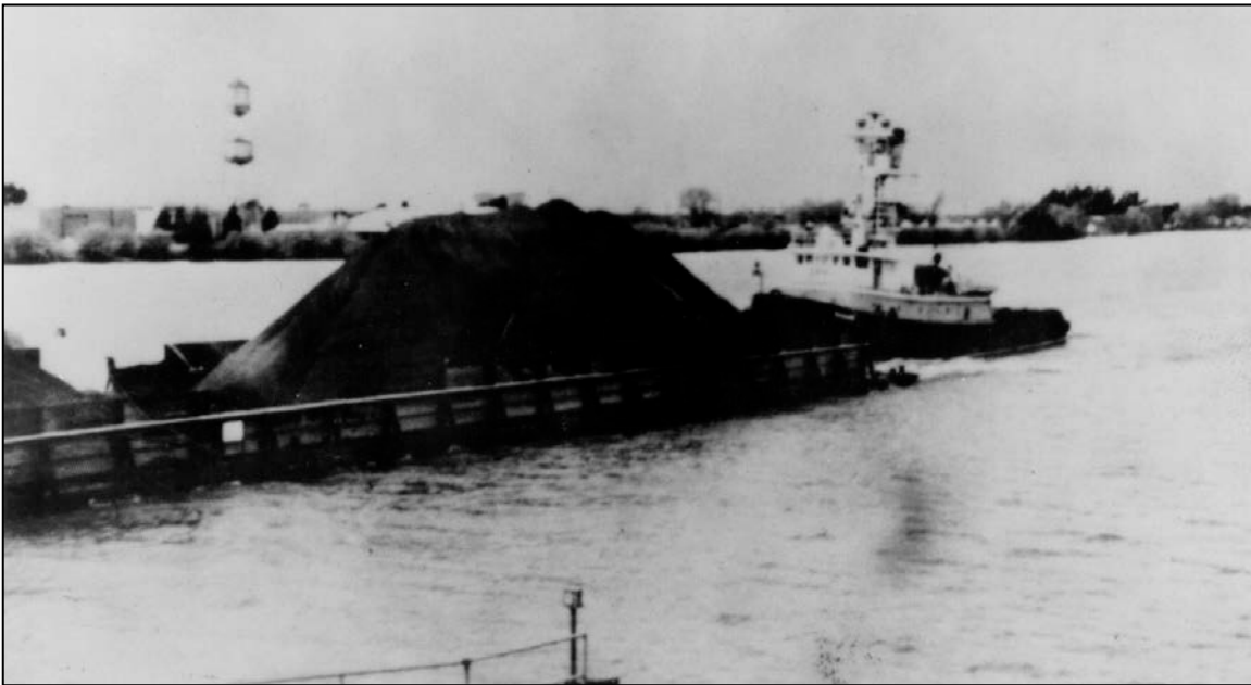
Figure 5-3. A Tugboat and Barge Transporting Dredged Material
