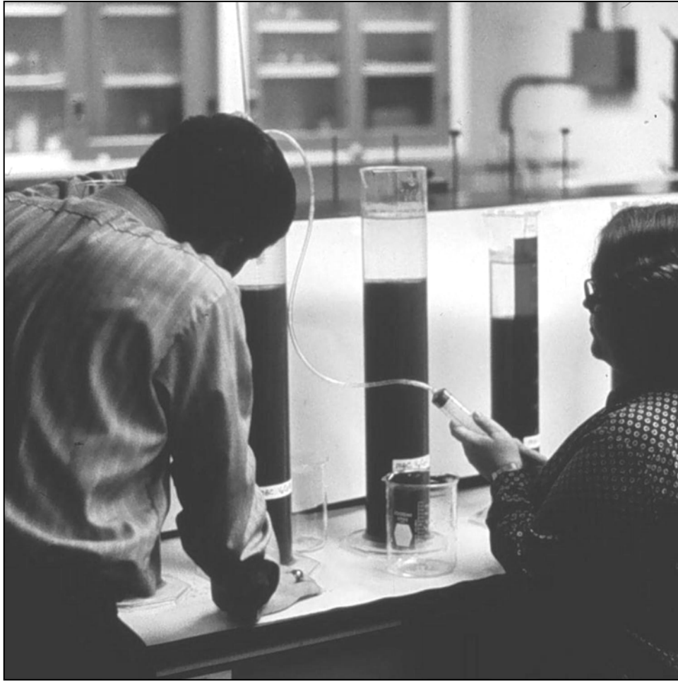
Figure 4-66. Modified Elutriate Test in Progress
