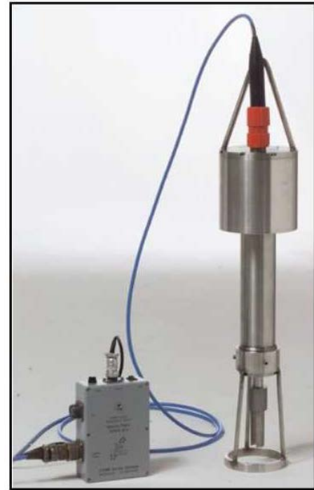
Figure 2-6. STEMA RheoTune Tuning Fork Shear Strength, Viscosity, and Density Probe
