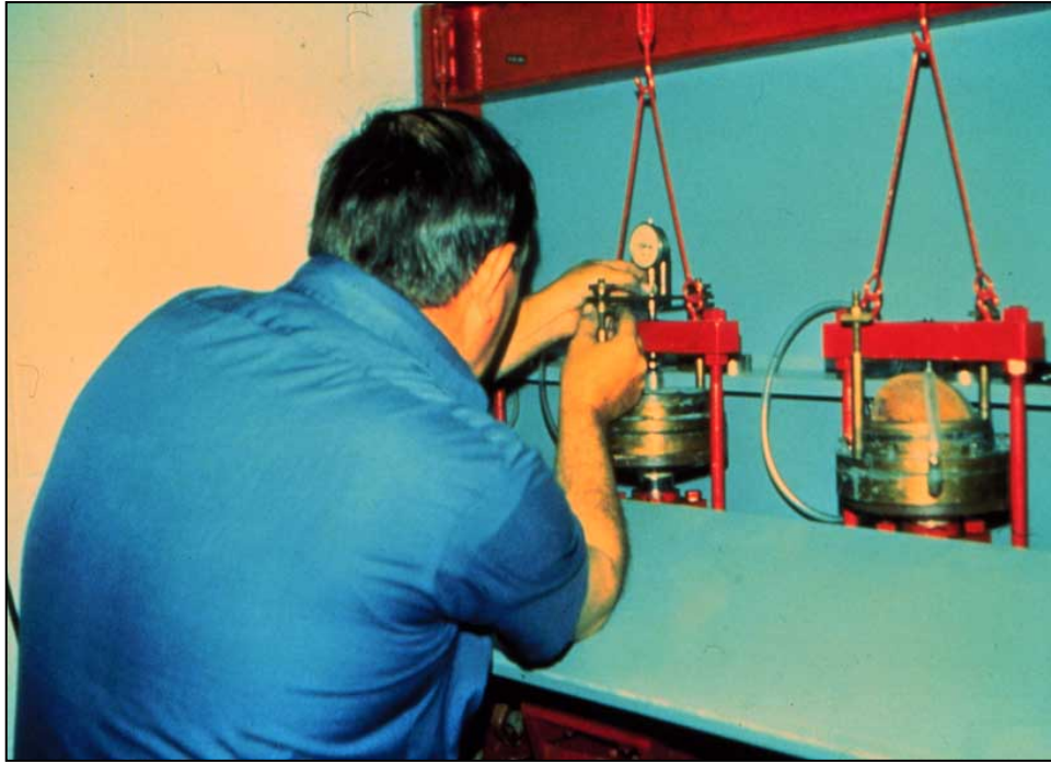
Figure J-3. Oedometer Testing Apparatus
