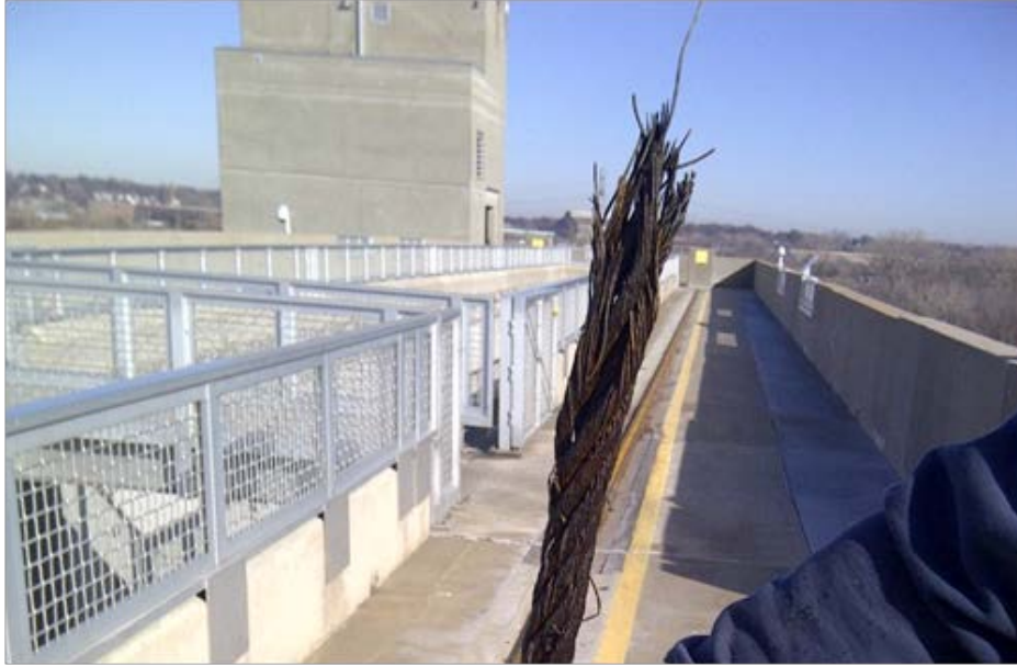
Figure B-2. Failed Cable – Failure Point Is Just above the Sockets. Must Dewater to Access.
