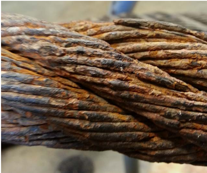
Figure 8-1. Severe Wire Rope Corrosion Including Pitting.
