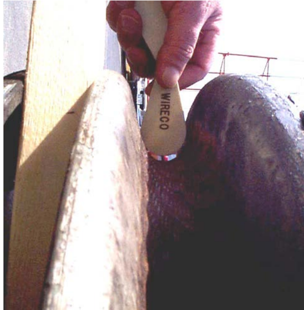
Figure 8-11. Sheave with Broken Flanges.
