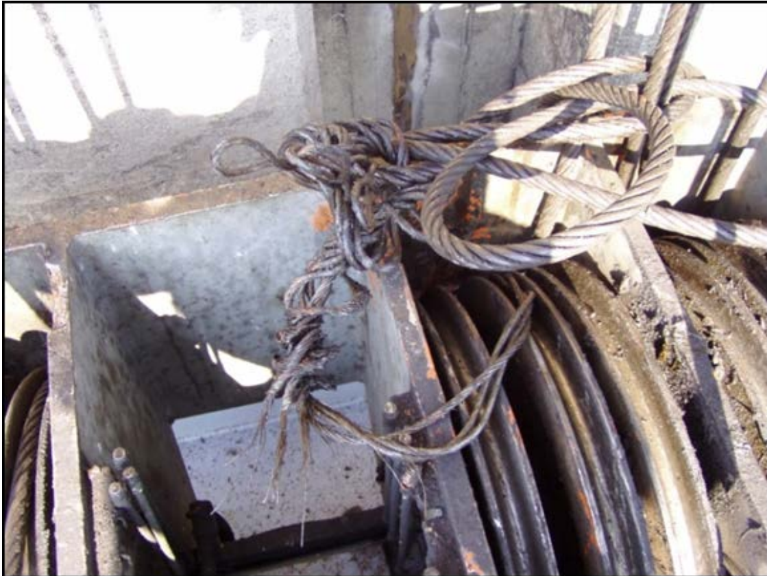
Figure B-9. Greenup Wire Rope Failure – Sheave Block.
