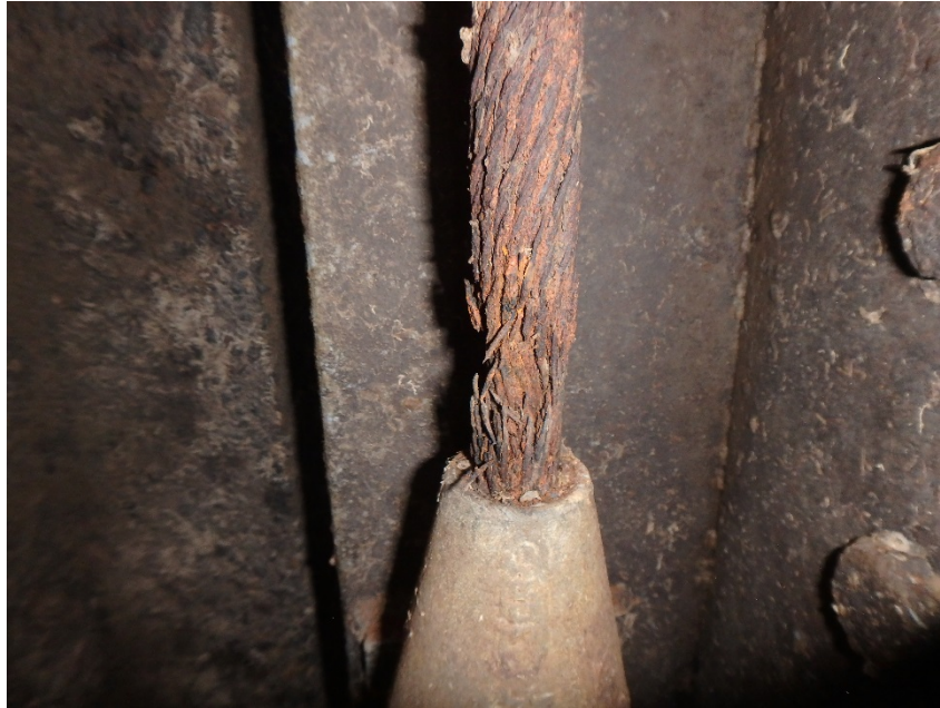
Figure 8-6. Pitting Corrosion (and Broken Wires) Lock 24 Culvert Valve
