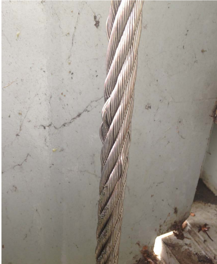
Figure 8-3. Lock 7 Tainter Valve - Wire Rope Showing Abrasion and Bird Caging.
