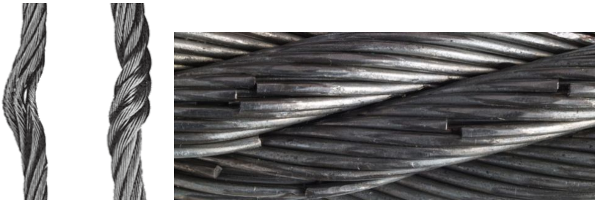
Figure 7-1. Wire Rope Kinks and Broken Wires.
