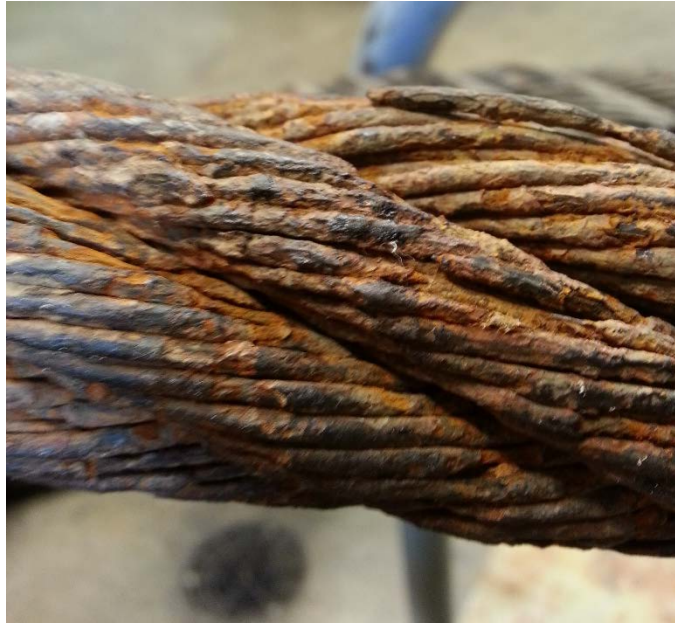
Figure B-4. Close up of Corroded Wire Rope.
