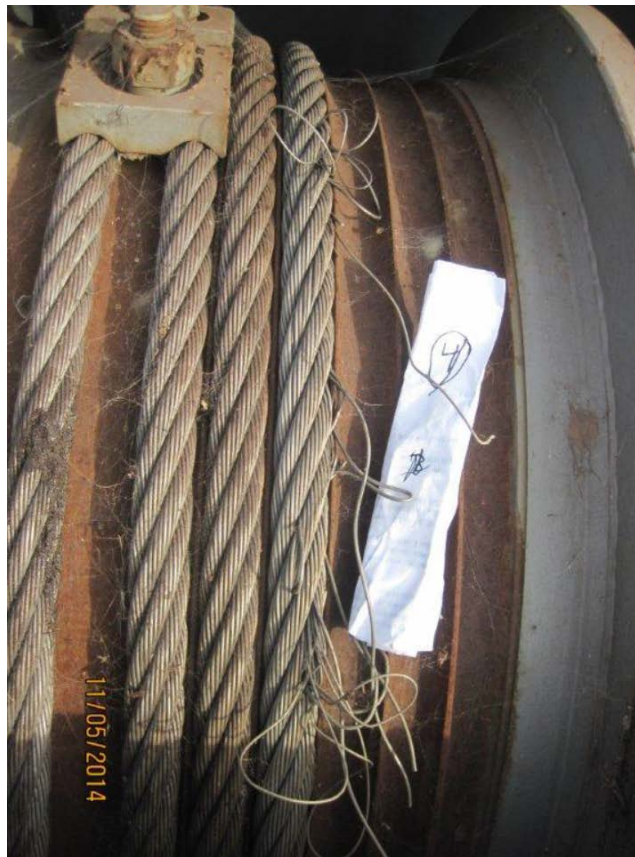
Figure 8-2. Wire Rope – Broken Rope Wires.
