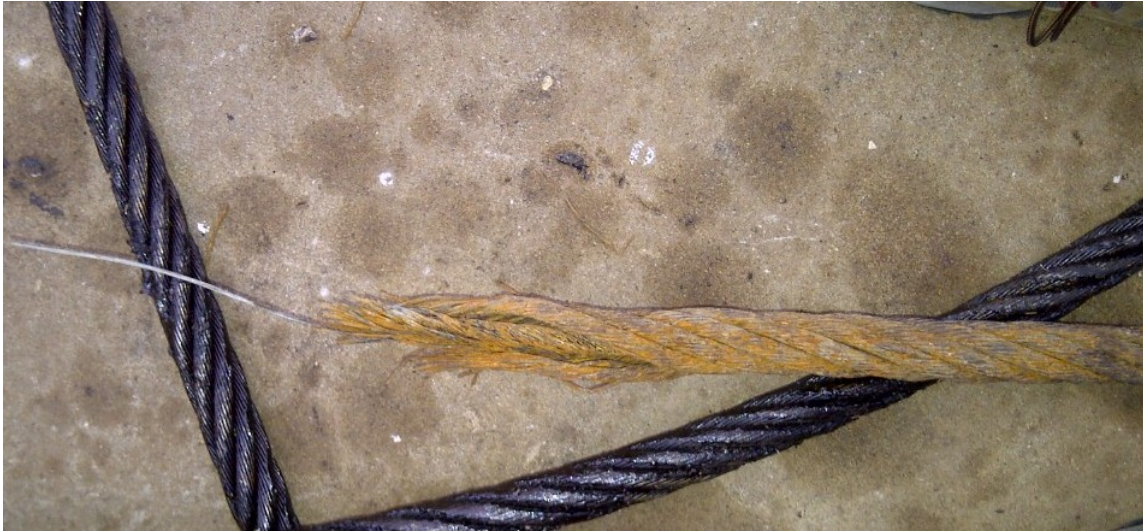
Figure 8-5. Mel Price Vertical Lift Gate Wire Rope Cable Breakage – Note Corrosion.
