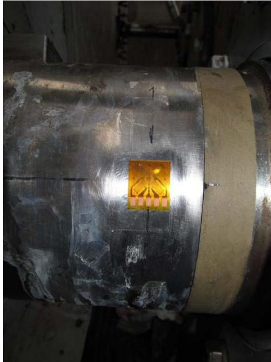
Figure 7-9. Strain Gauge on Rotating Shaft.
