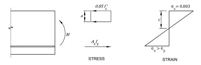
Figure C-4. Stress and Strain under Pure Flexure.
