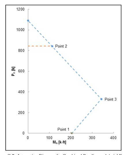
Figure C-7. Interaction Diagram for Combined Bending and Axial Forces.
