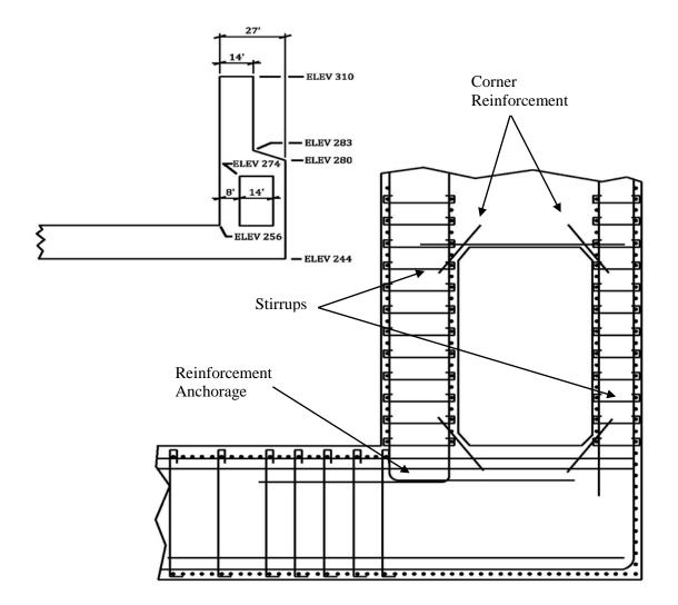
Figure 2-2. Typical Seismic Reinforcement Details – Olmsted L&D.
