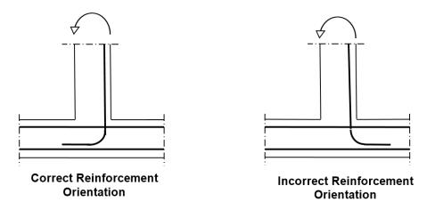
Figure 2-1. Reinforcement Detailing at Moment Connections.
