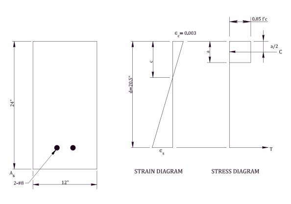
Figure C-1. Diagram of Singly Reinforced Beam Cross Section, Strain, and Stress.
