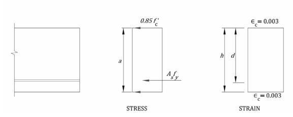
Figure C-5. Stress and Strain under Maximum Axial Load.
