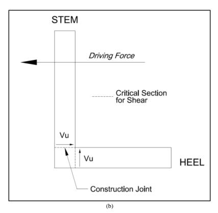
Figure 5-1. Critical Sections for Shear in Cantilever L-Type Walls.
