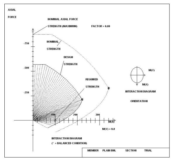
Figure C-8. Interaction Diagram produced in CGSI.
