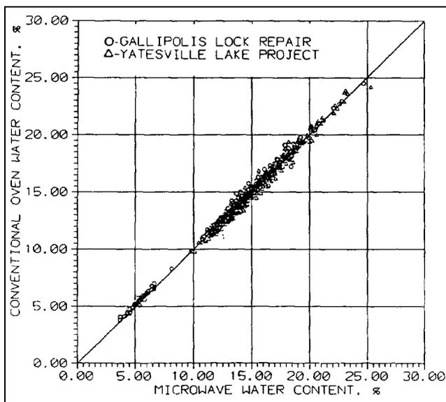
Figure 5-9. Conventional oven versus CCMOS water content data
