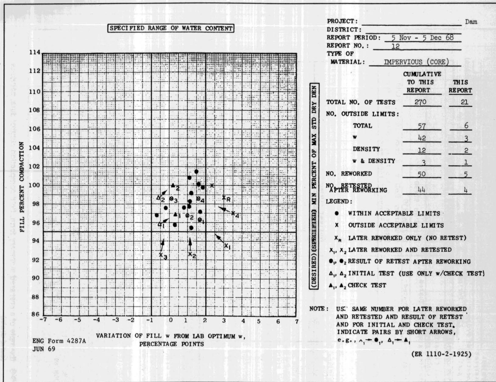
Figure D-2. Example of a prepared summary plot for materials requiring water content and density control
