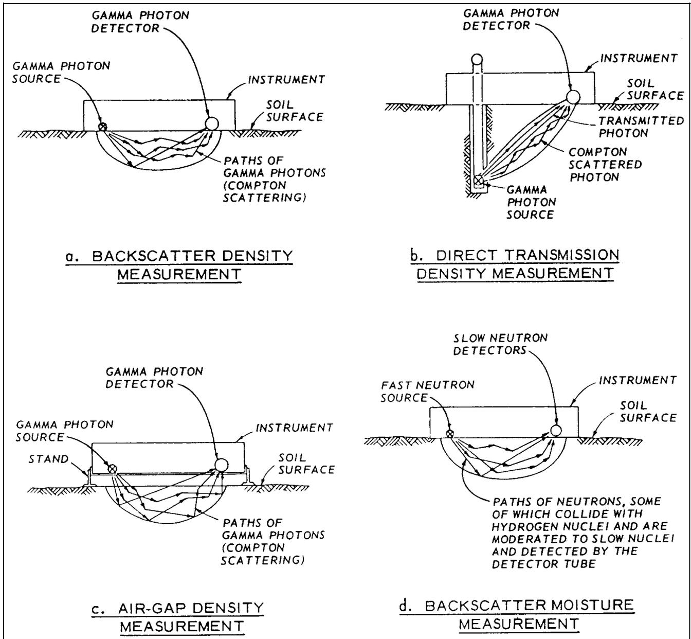
Figure 5-11. Schematic diagrams of density and moisture measurements
