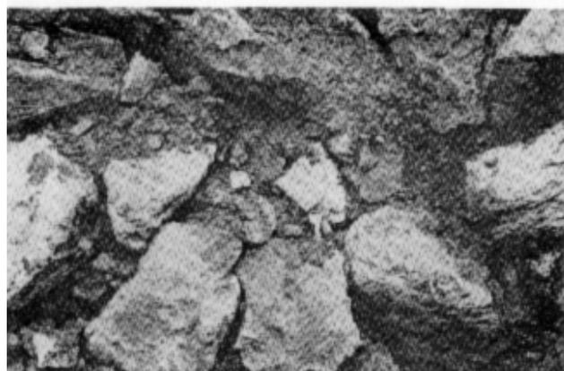
**Figure 5-5. Test trench through portion of rock test fill at New Melones Dam, California. General view of trench (top); closeup view of trench wall (bottom)**
