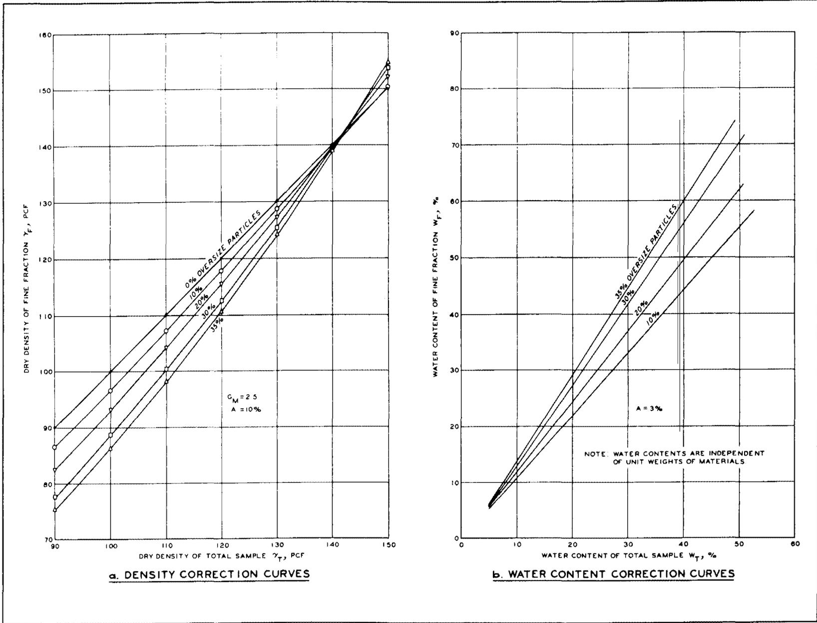
Figure B-6. Density and water content correction curves
