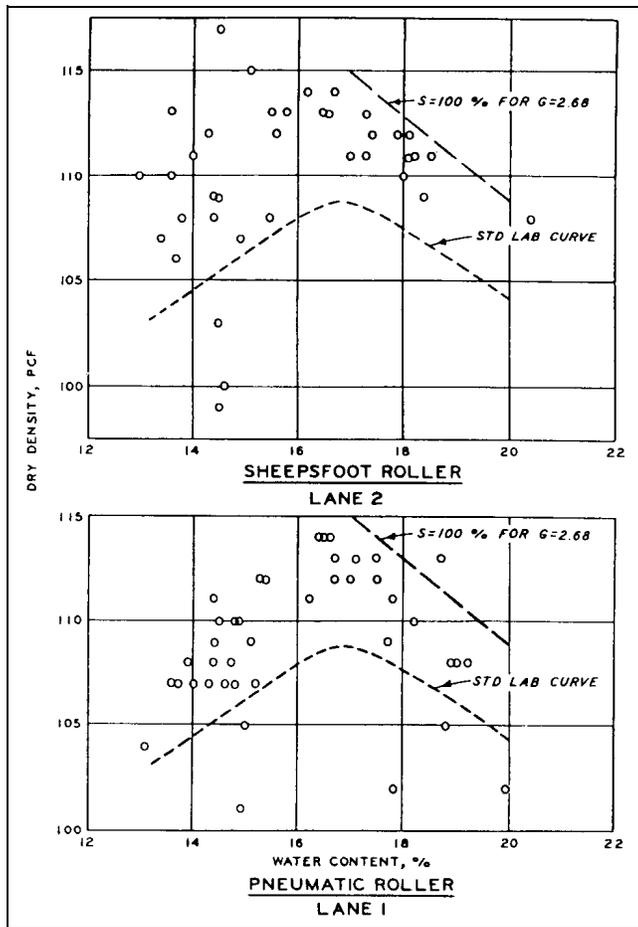
Figure 5-6. Test fill data from Canyon Dam, Texas
