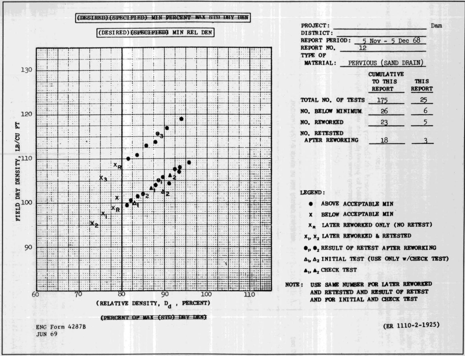
Figure D-4. Example of a summary plot for material requiring only density control
