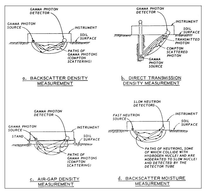
Figure 5-11. Schematic diagrams of density and moisture measurements
