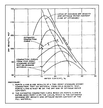
Figure B-3. Illustration of two-point compaction method
