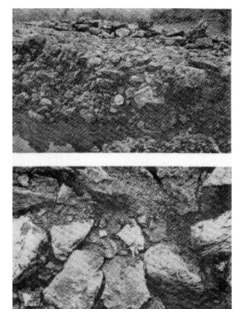
Figure 5-5. Test trench through portion of rock test fill at New Melones Dam, California. General view of trench (top); closeup view of trench wall (bottom)
