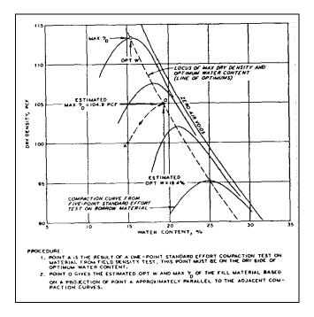
Figure B-1. Illustration of one-point compaction method
