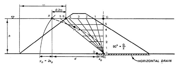
Figure 6-5. Construction of basic parabola and seepage line for  $\alpha$  = 180° Kozeny (courtesy of New England Waterways Association  $^{151})$
