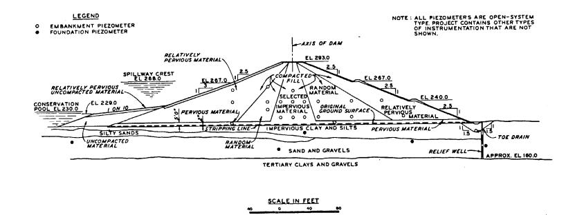
Figure 13-3. Piezometer installation with a thin impervious topstratum and relief well systems, Enid Dam (from EM 1110-2-1908)
