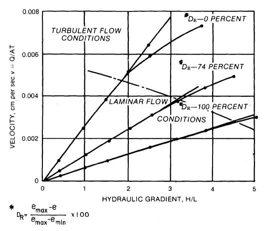
Figure 2-8. Determination of maximum hydraulic gradient for which laminar flow occurs for a fine sand (courtesy of American Society for Testing and Materials  $^{147}$ )
