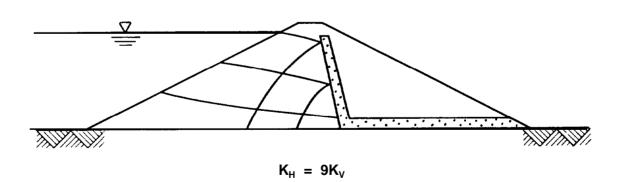
Figure 8-8. Effect of anisotropy of permeability on seepage through earth dam with and without an inclined drain (courtesy of John Wiley and  $\mathsf{Sons}^{\mathsf{155}}$ )
