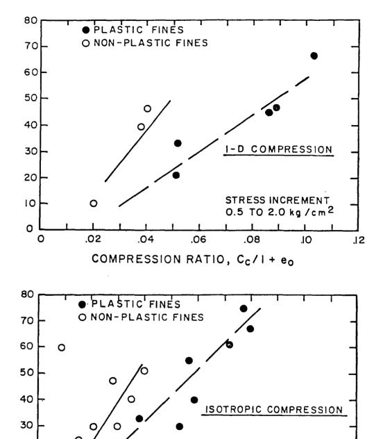
Figure 9-11. Relationship between fines content and compressibility of a soil-bentonite slurry trench backfill (courtesy of American Society of Civil Engineers $^{163}$ )
