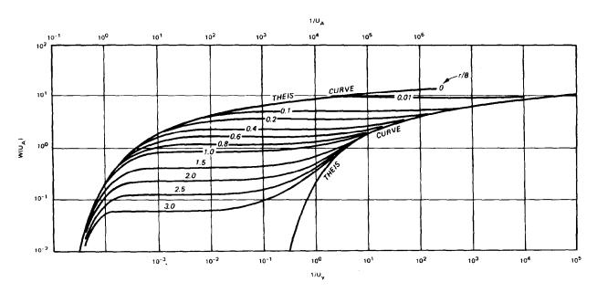
a FAMILY OF BOULTON TYPE CURVES: W (U\_A, r/B) VERSUS 1/U\_A AND W (U\_y, r/b) VERSUS 1/U\_y FOR DIFFERENT VALUES OF r/B.
