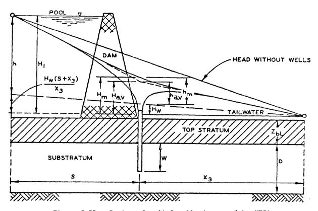
Figure 9-25. Design of relief wells (prepared by WES)
