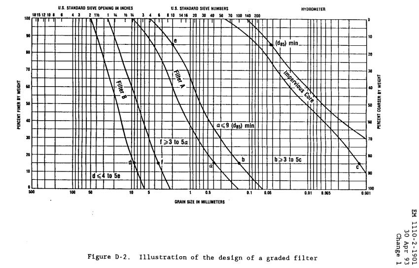
Figure D-2. Illustration of the design of a graded filter
