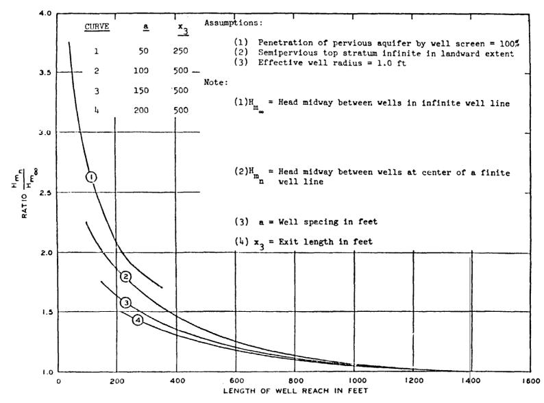
Figure 9-31. Ratio of head midway between relief wells at center of a finite well system to head midway between wells in an infinite system (from U.S. Army Engineer Waterways Experiment Station  $^{120}$ )
