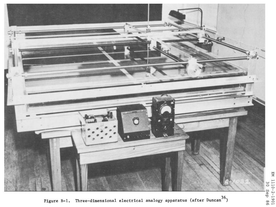
Figure B-1. Three-dimensional electrical analogy apparatus (after Duncan 36)
