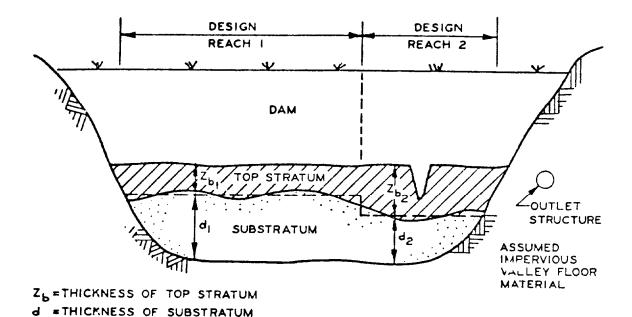
Figure 9-24. Profile of typical design reaches for relief well analysis (prepared by WES)
