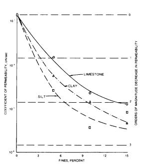
Effect of fines on permeability of concrete sand (from Barber and Sawyer<sup>137</sup>)
