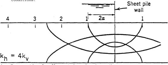
True section for flow net in a for  $k_h = 4k_v$
