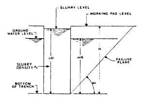
a. Slurry trench typical section
