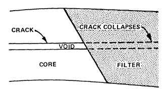
a. Self-healing (by collapse) of filter
