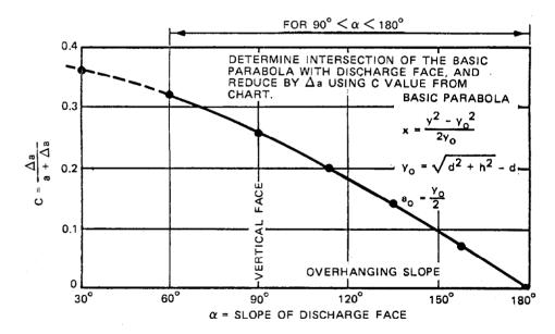
NOTE: POINTS WERE FOUND BY GRAPHICAL DETERMINATION OF FLOW NET. Figure 6-6. c vs  $\alpha$  (courtesy of New England Waterworks Association 151)
