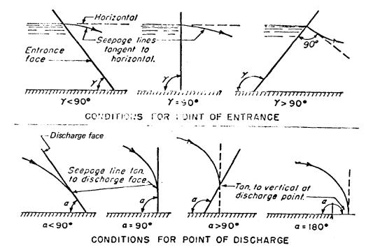
Figure 4-7. Entrance and discharge (exit) conditions for a line of seepage (courtesy of New England Waterworks Association  $^{151}$ )
