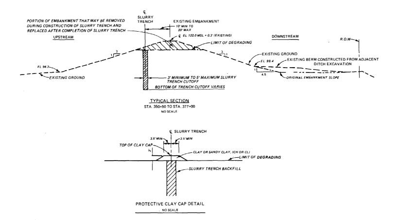
Figure 12-2. Addicks Dams remedial slurry trench for embankment and foundation seepage control (from U.S. Army Engineer District, Galveston<sup>83</sup>)
