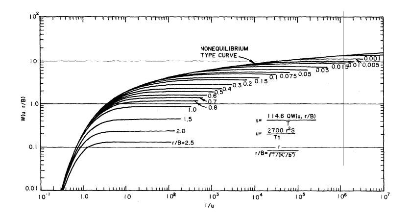
Figure 7-12. Type curve for nonsteady flow in a semiconfined aquifer (courtesy of John Wiley and  $\mathsf{Sons}^{164}$ )
