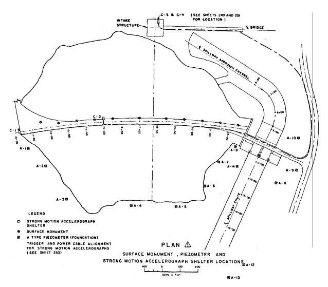
Figure 13-4. Piezometer installation for dam abutments having grout curtains or cut-slope drains, Applegate Lake Dam (from U. S. Army Engineer District, Portland  $^{104}$ )
