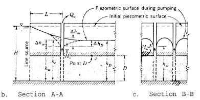
Figure 9-28. Flow to an infinite line of fully penetrating relief wells from an infinite line source of seepage (after Leonards $^{205}$ )
