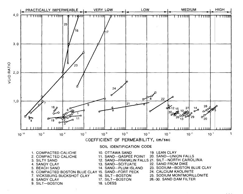
Figure 2-11. Relationship between void ratio and log of permeability (courtesy of Wiley 201)
