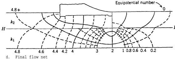
Figure 4-12. Flow net construction for a composite section (courtesy of John Wiley and  $Sons^{155}$ )
