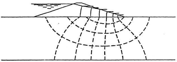
b. External equipotential lines into foundation without adjusting lines of net in dam.
