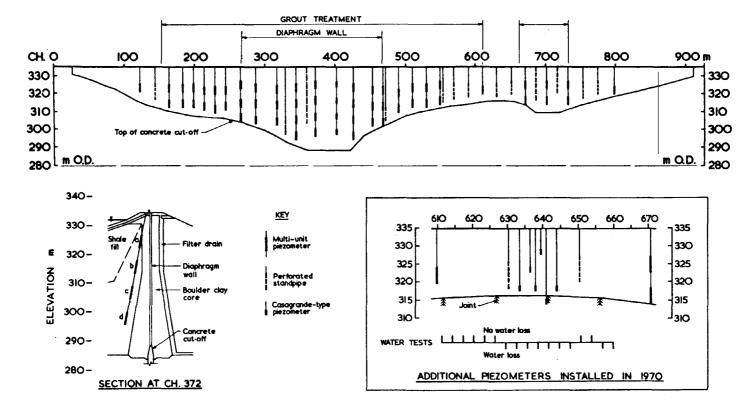
Figure 13-6. Layout of Baldershead Dam piezometer installation in upstream shale fill (courtesy of British Geotechnical Society 212)
