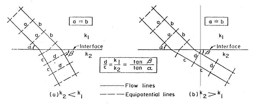
Figure 4-11. Deflections of flow lines at interfaces of soils having different permeabilities (courtesy of New England Waterworks Association  $^{151}$ )
