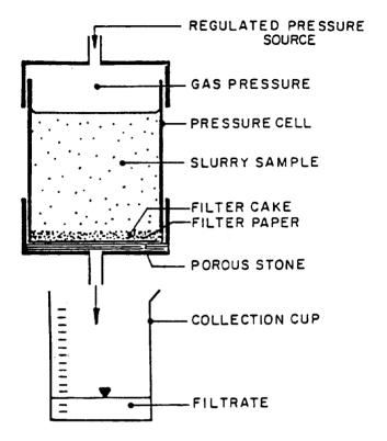
a. Schematic of filter press test apparatus
