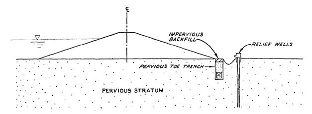
c. Trench drain used in conjunction with relief wells Figure 9-32. Trench drains to control underseepage (from EM 1110-2-1913)
