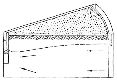
PARTIALLY PENETRATING WELL WITH A CIRCULAR SOURCE
