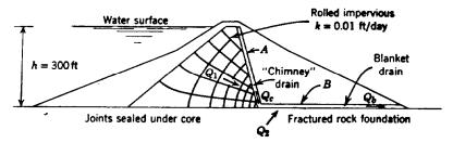
a. Cross section and flow net
