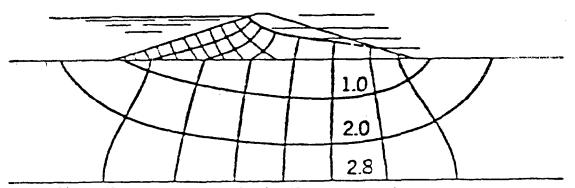
c. Adjust flow net to meet basic flow net requirements.
