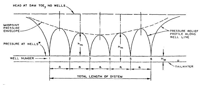
\*PRESSURE AT WELLS EQUALS TAILWATER EL + Hw.
