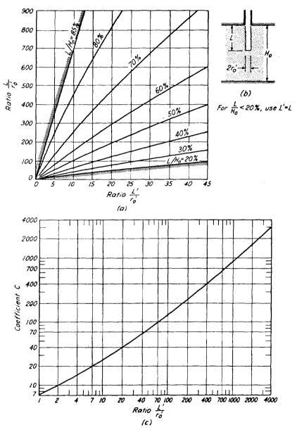
Figure 2-18. Field permeability test in bore hole (courtesy of John Wiley and  $\mathrm{Sons}^{175}$ )
