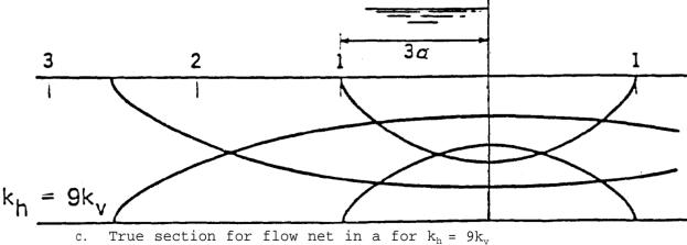
Figure 4-9. Flow nets constructed on transformed section and redrawn on true section (courtesy of John Wiley and Sons  $^{155}$ )
