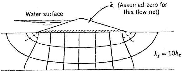
a. Construct flow net assuming impermeable embankment
