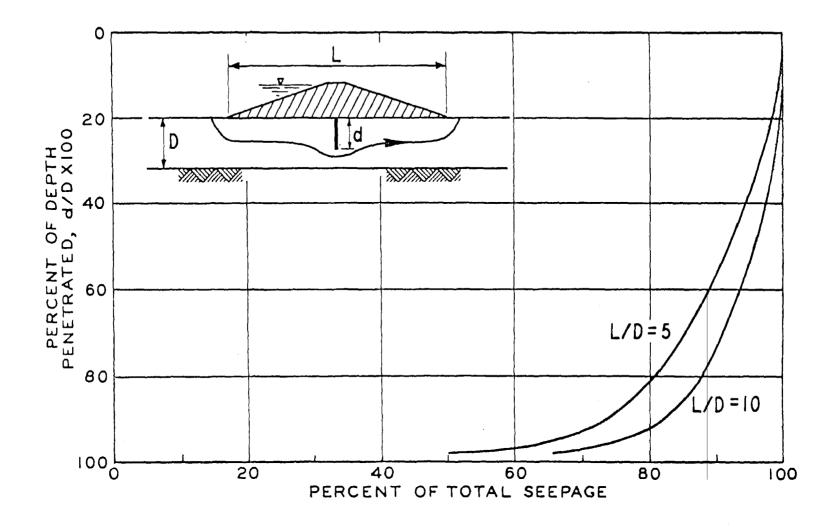
Figure 9-2. Effect of depth of penetration of partial cutoff on seepage reduction for a homogeneous isotropic foundation (prepared by WES)
