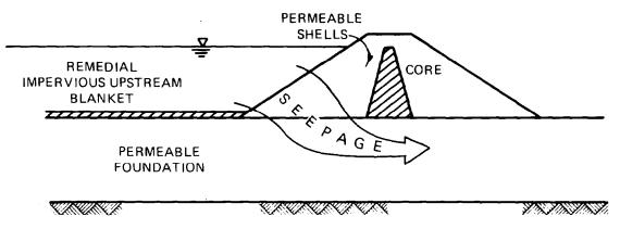
Figure 12-1. Possible problem if existing and remedial seepage control measures are not properly coordinated (prepared by WES)
