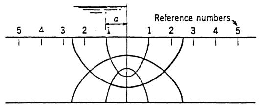
True section for  $k_{h}$  =  $k_{v}$  and transformed section for anisotropic conditions.
