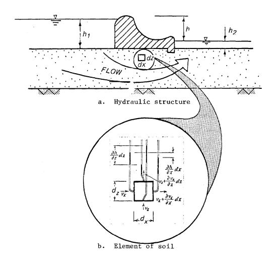
Figure 4-2. Flow of water through saturated pervious soil beneath a hydraulic structure (courtesy of John Wiley and  $\mathsf{Sons}^{274}$ )
