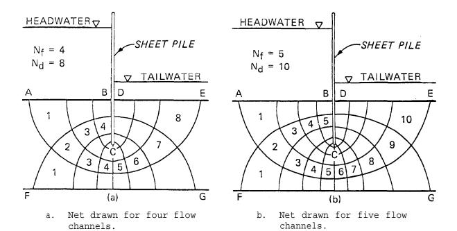
Figure 4-5. Flow net for a sheetpile wall in a permeable foundation (from U. S. Army Engineer District, Little  $Rock^{92}$ )
