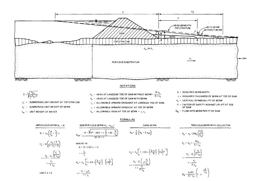
Figure 9-22. Design of downstream seepage berms where a downstream natural blanket is present (from U.S. Army Engineer Waterways Experiment Station  $^{120}$ )
