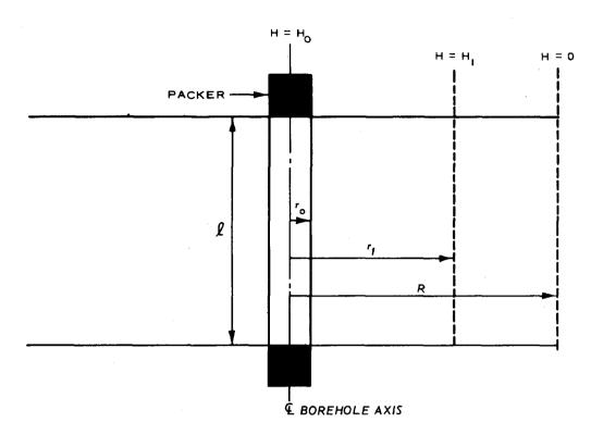
Figure C-2. Homogeneous isotropic material--radial flow (prepared by WES)
