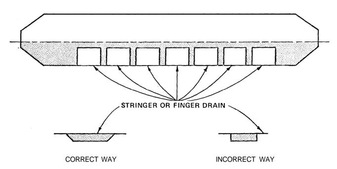
Figure 8-11. Use of stringers or finger drains as an alternative to a continuous horizontal drain (prepared by WES)
