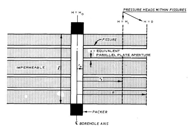
Figure C-3. Fissured-medium--radial flow (prepared by WES) and the permeability of each fissure is
