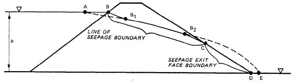
Figure 6-1. Line of seepage, BC, and seepage exit face, CD, for a homogeneous earth dam on an impermeable foundation (prepared by WES)
