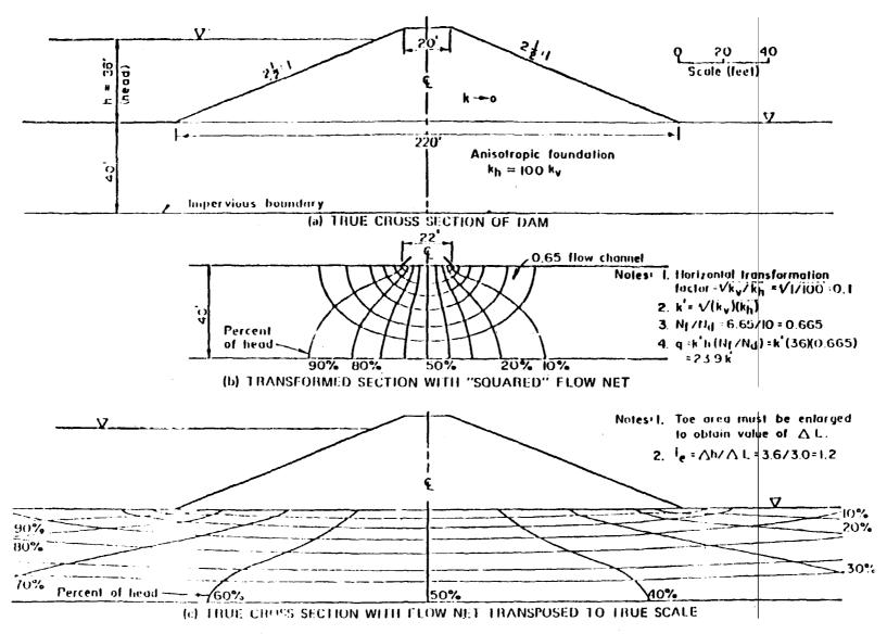
Figure 4-10. Example of technique for developing a flow net for an anisotropic foundation (from U. S. Department of Agriculture  $^{123}$ )
