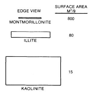
a. Edge view sketch to show relative size and shape of clay particles (dimension not shown in length)
