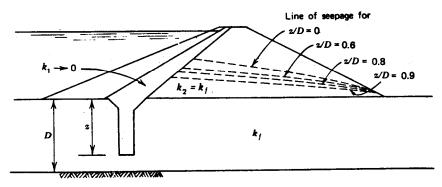
c. Position of line of seepage for various values of penetration  $% \left( 1\right) =\left( 1\right) \left( 1\right) +\left( 1\right) \left( 1\right) \left( 1\right) +\left( 1\right) \left( 1\right)$
