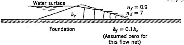
a. Construct flow net assuming an impermeable foundation.
