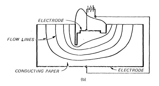
Figure 4-4. Use of two-dimensional conducting paper to find flow lines and equipotential lines (courtesy of John Wiley and Sons  $^{\rm 279)}$
