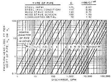
BASED ON HAZEN-WILLIAMS EQUATION WITH C = 100; MULTIPLY LOSSES BY (100/C) 1.85 FOR VALUES OF C OTHER THAN 100 (b)
