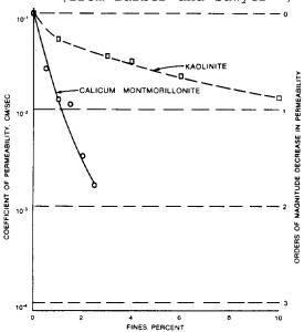
c. Effect of fines on permeability of uniform fine sand (from Fenn<sup>171</sup>)
