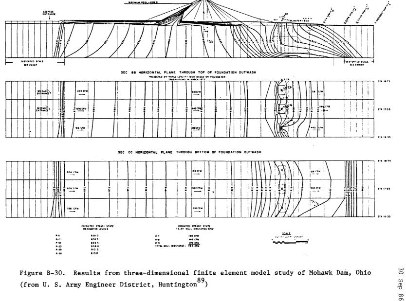
Figure B-30. Results from three-dimensional finite element model study of Mohawk Dam, Ohio (from U. S. Army Engineer District, Huntington 89)
