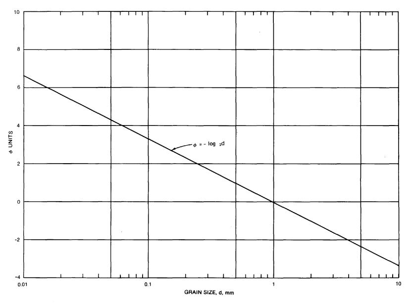
Figure 2-13. Conversion chart for  $\phi$  and grain size in mm, for the range 0.01 to 10 mm (prepared by WES)
