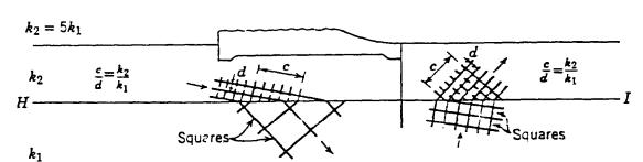
b. Determine deflection of flow net at interface between soils with different permeabilities.
