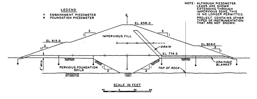
Figure 13-2. Piezometer installation for dams on pervious foundations, Deer Creek Dam (from EM 1110-2-1908)
