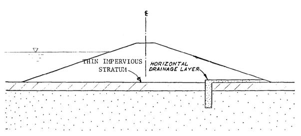
b. Trench drain under downstream slope of dam
