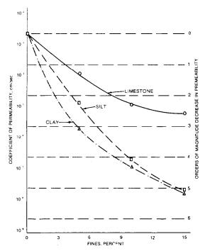
Effect of fines on permeability of sand-gravel mixture (from Barber and Sawyer<sup>137</sup>)
