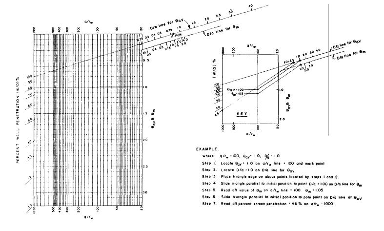
Figure 9-29. Nomograph for obtaining uplift factors for design of partially penetrating relief wells (from U.S. Army Engineer Waterways Experiment Station 120)
