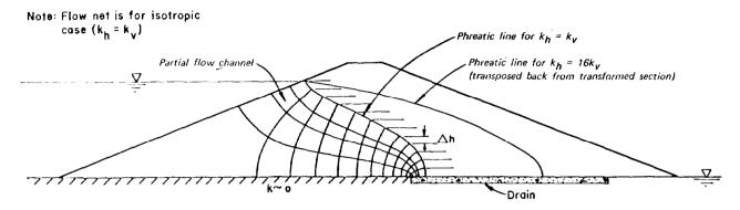
Figure 6-10. Effect of difference in horizontal and vertical permeability (anisotropy) on location of line of seepage within an embankment with a horizontal drain (after U. S. Department of Agriculture $^{123}$ )
