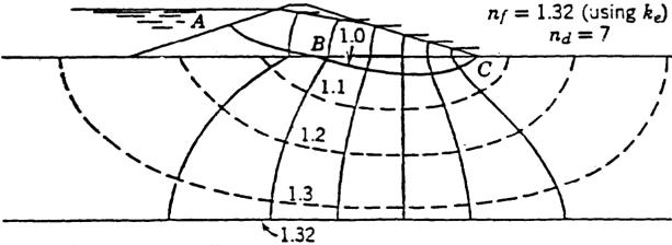
c. Adjust flow net until balanced.
