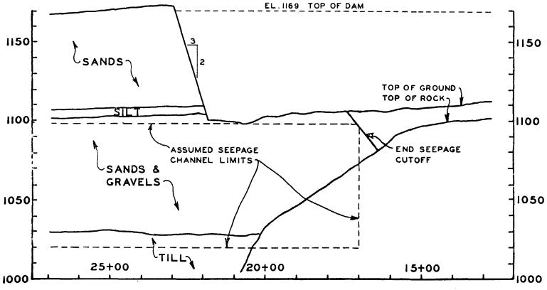
Figure 10-1. Profile of left pervious abutment at North Branch of Kokosing Dam, Ohio (from U. S. Army Engineer District, Huntington  $^{87}$ )
