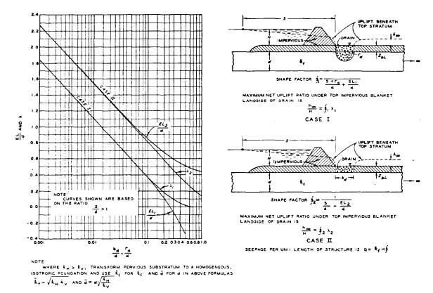
Figure 9-33. Design of toe trench drains for homogeneous, isotropic, pervious foundation, and for an impervious downstream top stratum (from U. S. Army Engineer Waterways Experiment Station  $^{120}$ )
