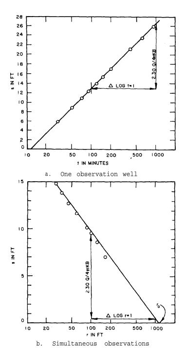
Figure 7-10. Use of Jacob approximation for nonsteady state flow (courtesy of John Wiley and Sons  $^{164}$ )
