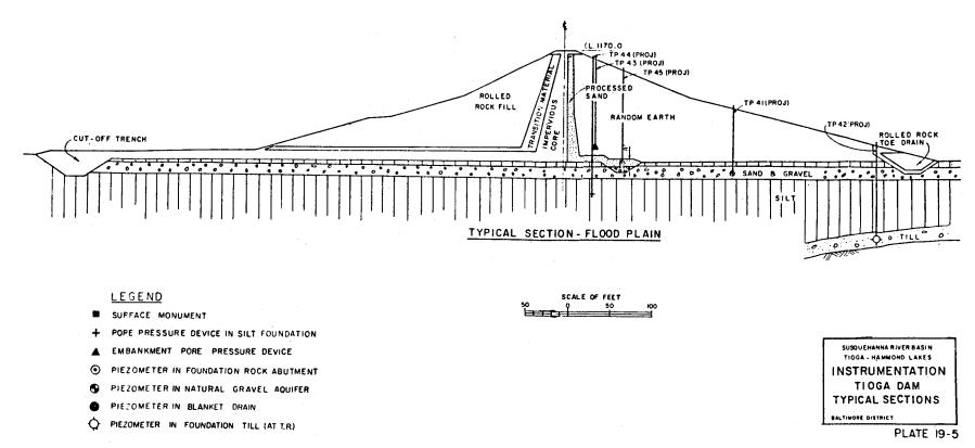
Figure 13-7. Piezometer installation for dams with through seepage and underseepage (from U. S. Army Engineer District, Baltimore  $^{79}$ )
