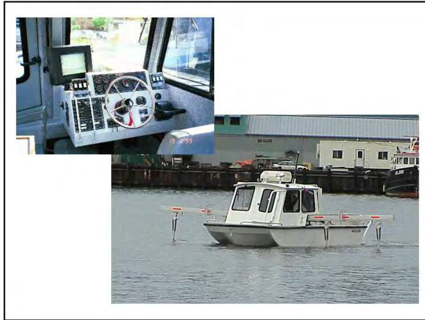
Figure 5-9. St. Paul District Five-Channel Ross Mini Sweep System on a 24-ft boat.
