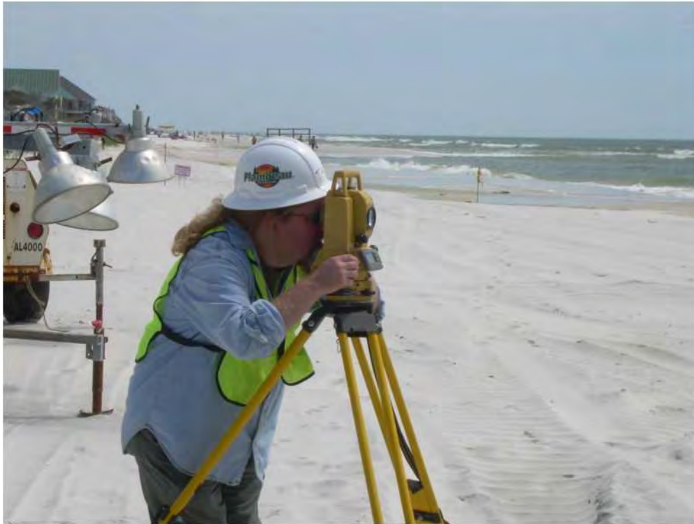
Figure 11-6. Total station control of topographic beach profiles.
