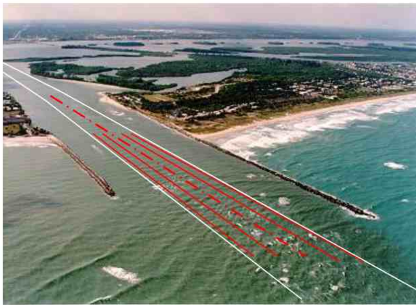
Figure 2-2. Multibeam survey line coverage on a 40x300 ft wide deep-draft navigation project.
