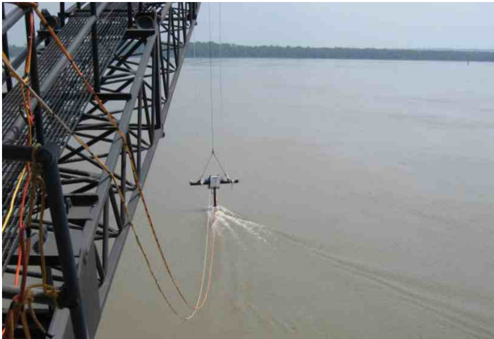
Figure N-19. Multibeam transducer deployed from crane on Low Sill Structure.
