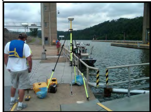
RTK GPS base station on lock wall @ Barkley
