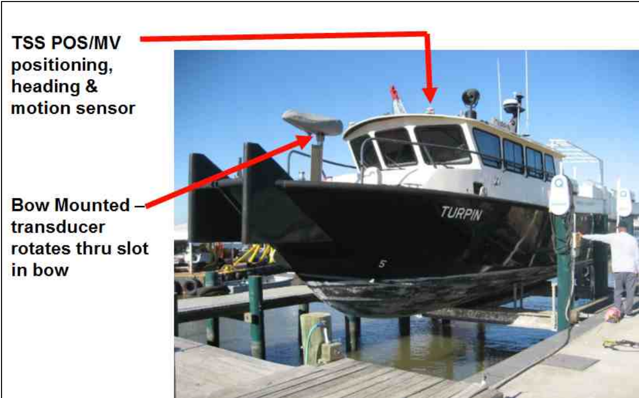
Figure 6-9. S/V Turpin with bow-mounted transducer.
