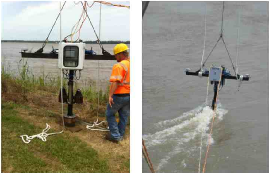
Figure N-18. Weighted multibeam transducer with DGPS positioning (POS/MV).
