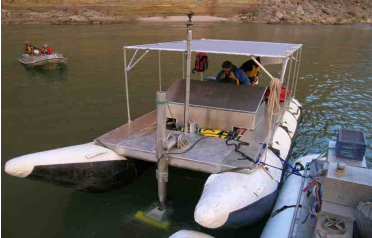
Figure 6-11. Bow-mounted transducer on an inflatable raft. This portable vessel is used for US Geological Survey multibeam surveys of the Colorado River in the Grand Canyon. It is manually deployed.
