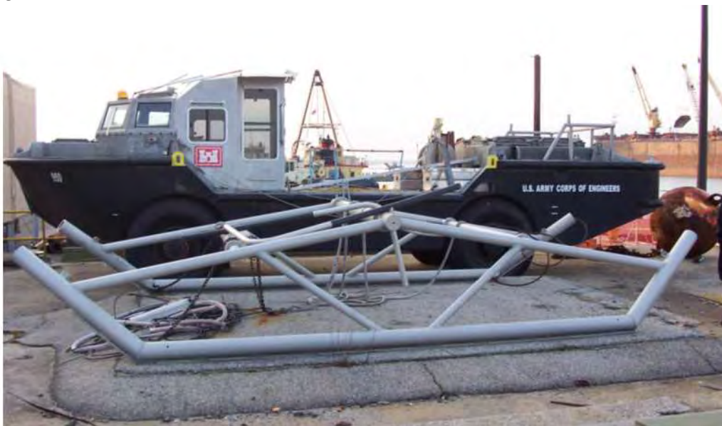
Figure 11-9. Sled profiling system—LARC ("Lighter, Amphibious, Re-Supply, Cargo") with towed sled. Used to collect profile data through the surf zone and into the nearshore areas. (New York District)
