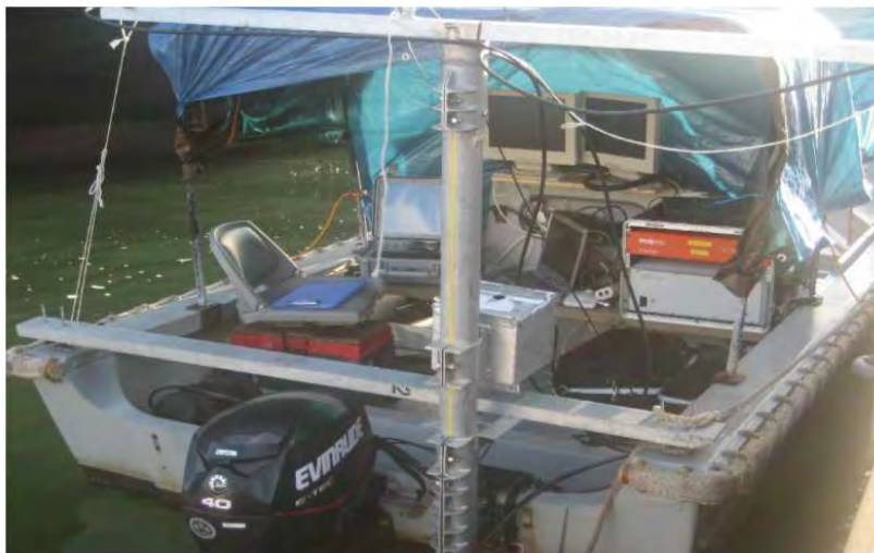
Figure 6-17. Temporary stern-mounted multibeam transducer on a small skiff. In this case, engine propeller noise did not appear to affect the data quality. (Portland and St. Louis District)
