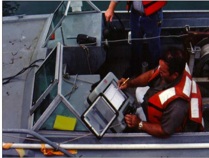
Figure 4-6. Raytheon DE 719 analog-recording portable echo sounder ca 1978. (Jacksonville District)
