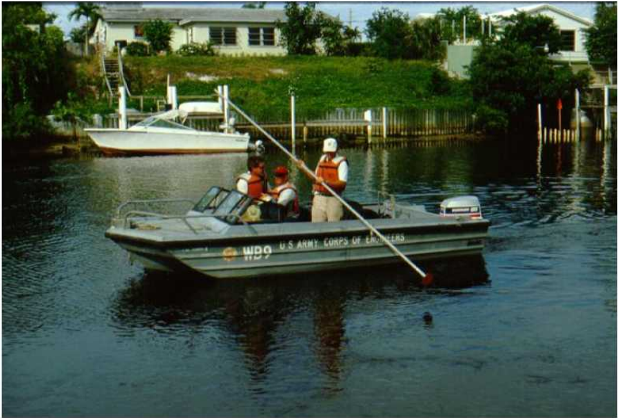
Figure B-5. Sounding pole measurement from a small work boat (Jacksonville District)
