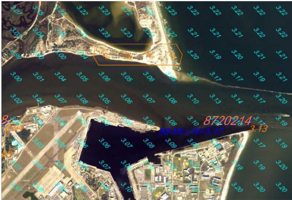
Figure 7-6. Example of a KTD file generated from VDatum. (Ocean entrance to Mayport Naval Base, St. Johns River, FL). “K” values are “NAVD88 – MLLW.” Note incorrect VDatum and KTD interpolation on north side of entrance, between the river and tidal pool. This region required manual edits to the KTD file to correct. Published NOAA gage 8720214 “K” at South Jetty agrees closely with VDatum “K.”
