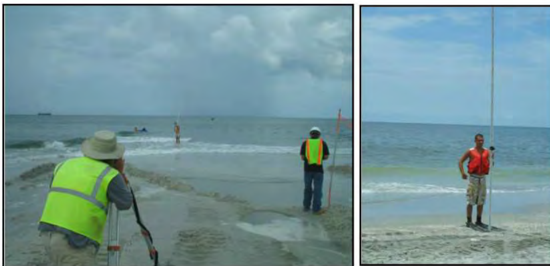
Figure 11-4. Beach profiles using a level and tagline for control. On left photo, fixed end of tag line is held at TBM next to grade stake. Range poles or grade stakes are used for visual alignment. Rodman on right photo is shown with 25-ft level rod.
