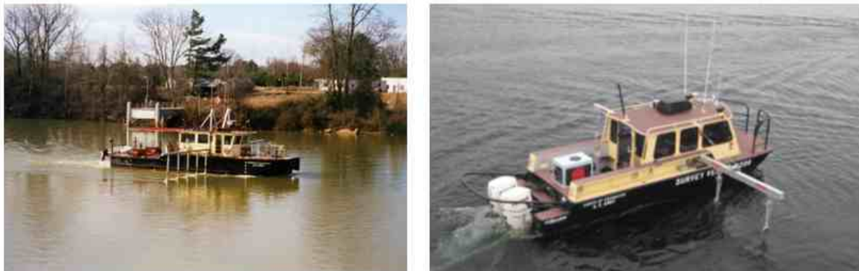
Figure 5-5. Tuscaloosa Multi-transducer sweep boats. E.B. WALLACE on left and one of three 24-ft vessels on right. (Mobile District)
