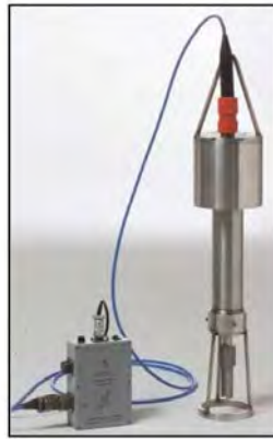
Figure P-19. Stema RheoTune tuning fork shear strength, viscosity, and density probe.
