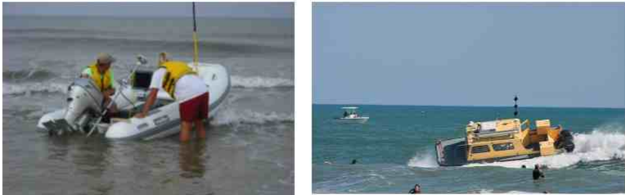
Figure 11-10. Inflatable raft on left is used on near-shore beach profile surveys. Water-proofed shallow-water depth sounder, RTK, and a laptop running HYPACK are installed aboard the raft. The Corps survey vessel on right must have sufficient engine power to maneuver through surf zones during turns at the inshore end of each profile line.
