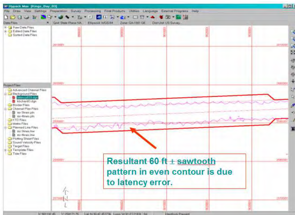
Figure 4-13. Effect of latency error in data contours as shown in plan view of channel.
