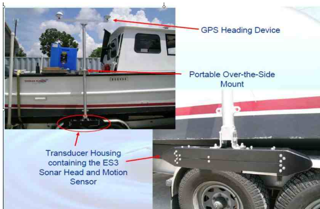
Figure 6-15. Side/aft mount of an Odom ES-3 transducer and inertial motion sensor. Mounting the GPS antenna directly above the transducer and motion sensor minimizes lever arm measurements and corrections.
