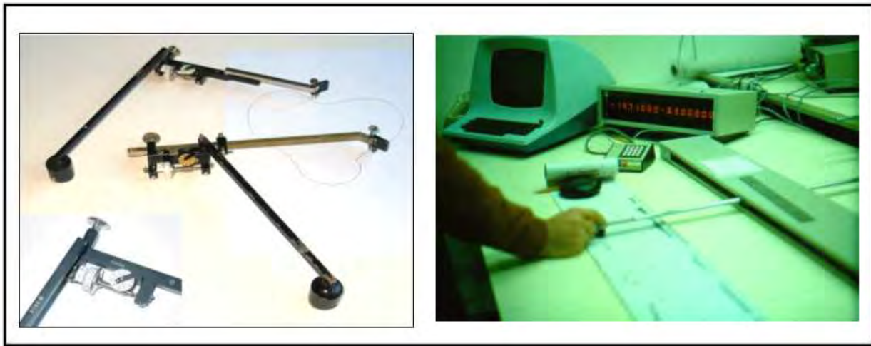
Figure 10-15. Quantity take-offs from polar planimeters (on left) and a digitizing tablet. The echo sounder analog record is directly digitized. (ca 1976 Jacksonville District)
