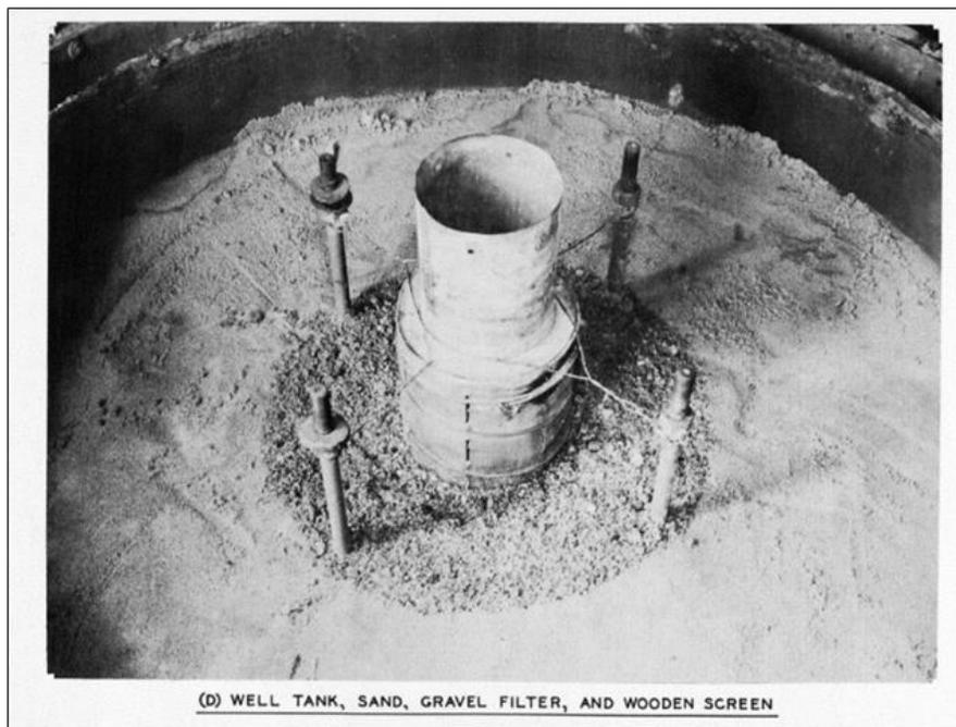
**Figure K-2. Tank used for relief well tests per Technical Memorandum TM 3-341 (USACE 1952)**
