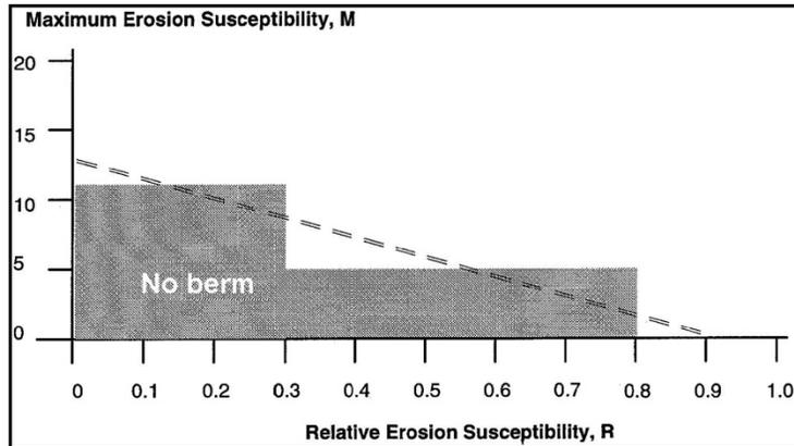
Figure 31. Rock Island District berm criteria and linear approximation of limit state
