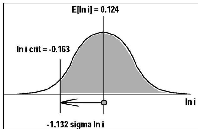
Figure 6. Calculation of probability of failure for underseepage
