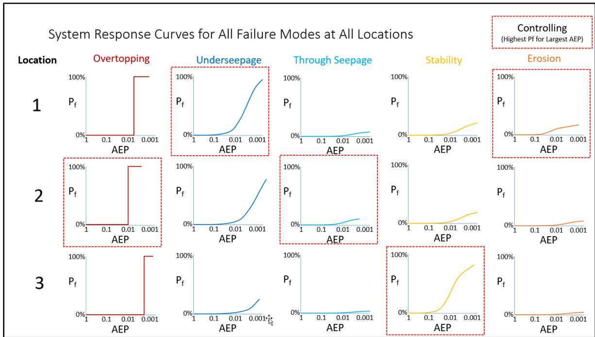
Figure 2. Development of Failure Mode System Response Curves and Selection of Controlling Curve for Index Location Station
