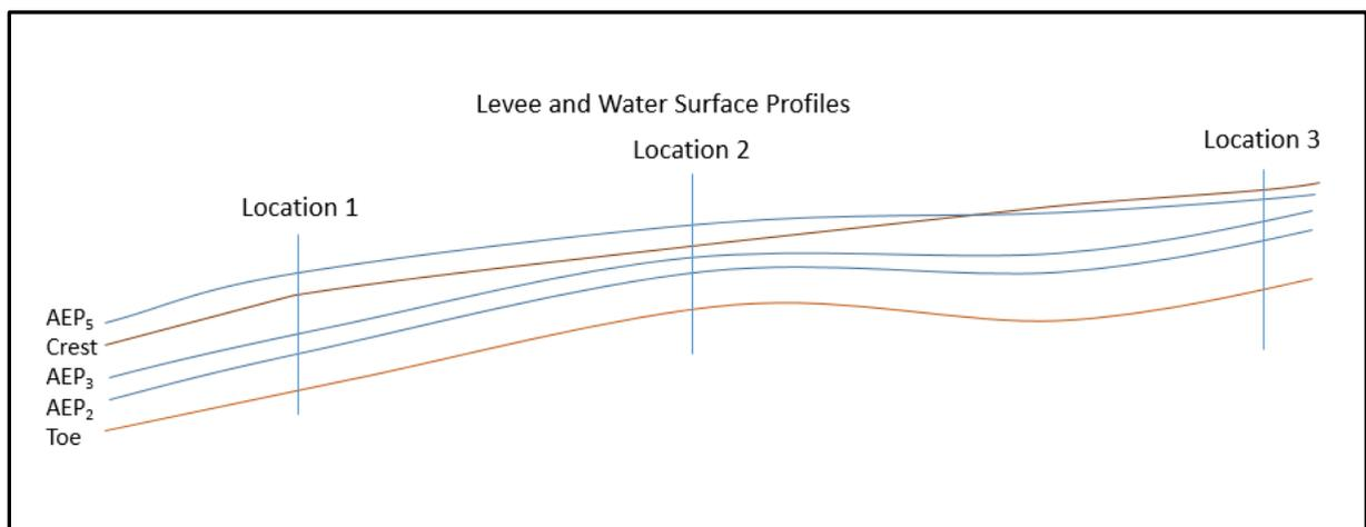
Figure 1. Levee Reach with Different Expected Performance at Varying Locations
