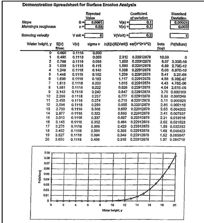
Figure 40. Example spreadsheet for surface erosion analysis
