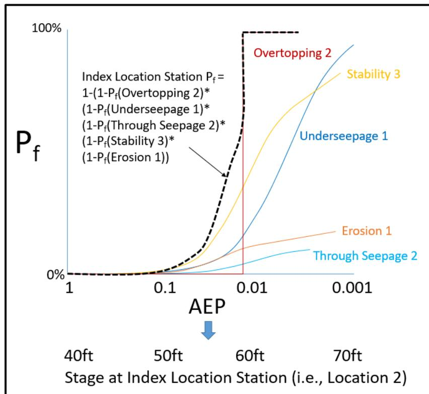
Figure 3. Upper Bound of Uni-Modal Bounds Theorem for Combination of Controlling System Response Curves and Conversion of AEP to Stage ( $P_f$  = Probability of Failure)
