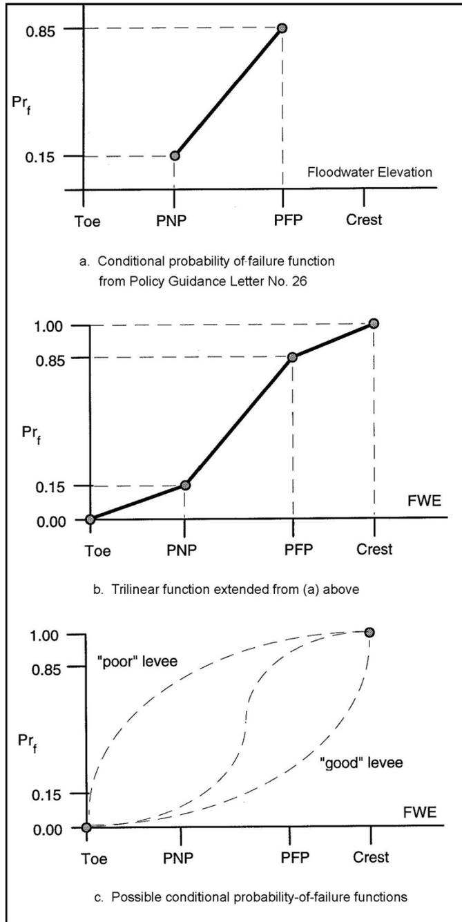
Figure 2. Alternative conditional probability-of-failure functions
