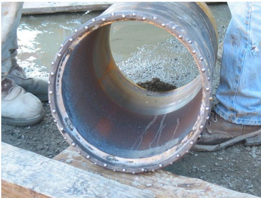
Figure 68. Carbide-studded shoe for 12-inch diameter dual rotary casing (Courtesy of AECOM)
