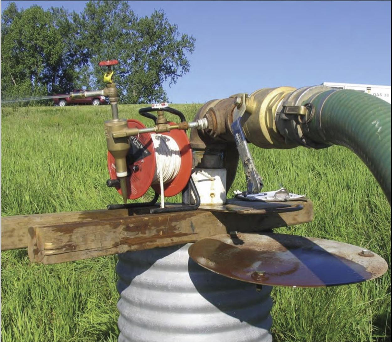
Figure B.15. Rossum sand tester (on left side) equipped with tee valve and Dole orifice to regulate flow through tester (Courtesy of AECOM)
