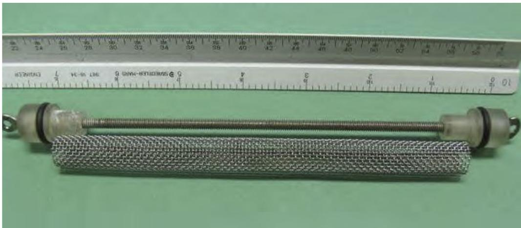
Figure 72. Stainless steel coupon (Courtesy of AECOM)
