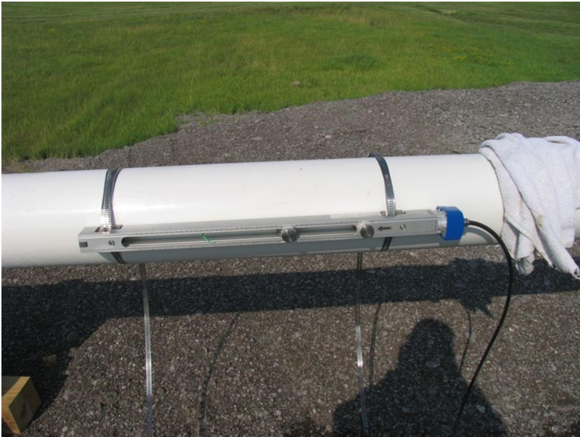
Figure D.3. Portable Krohne Optisonic 6300 medium ultrasonic flow meter strapped to 12-inch diameter discharge pipe; this model is rated for measuring flow in 2- through 16-inch diameter pipes (Courtesy of AECOM)
