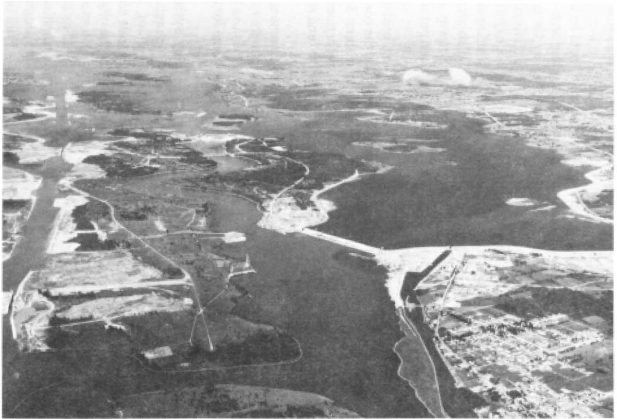
The completed project. At far left is the Wiley-Dondero Canal with the Eisenhower Lock at the upper left and the Snell Lock below. At the bottom of the picture is the tip of Cornwall Island. At right is the town of Cornwall, Ontario, and the Cornwall Canal. The St. Lawrence Power Dam is at the center, the Long Sault Dam to the left.
