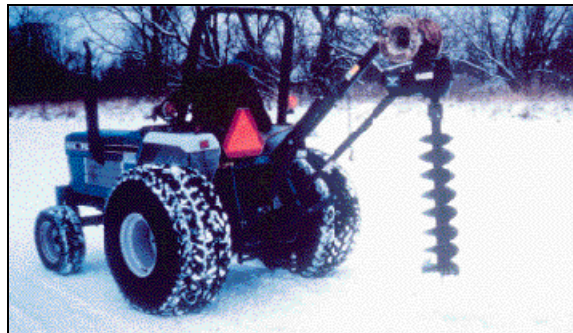
a. Posthole digger mounted on tractor.
