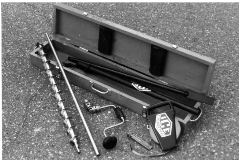
Figure 16-8. Standard CRREL ice thickness measuring kit.
