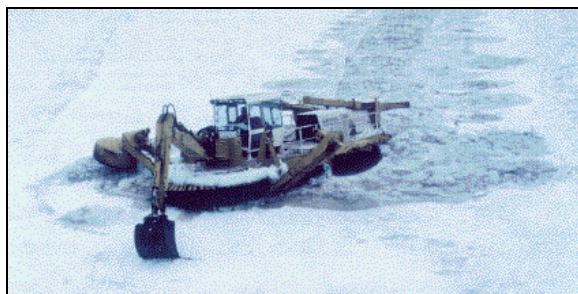
Figure 3-11. Breaking ice with an amphibious excavator on the Aroostook River, Ft. Fairfield, Maine.
