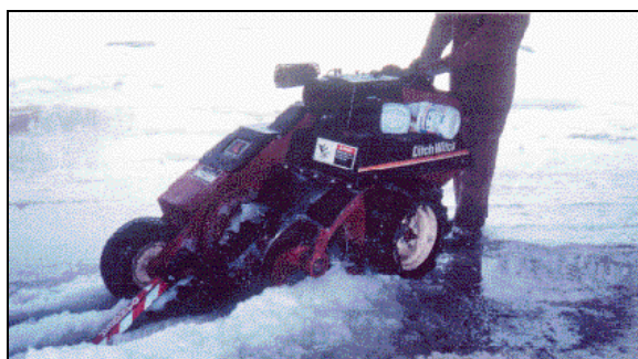
b. Ditchwitch 1260 cutting ice in Montpelier, Vermont.
