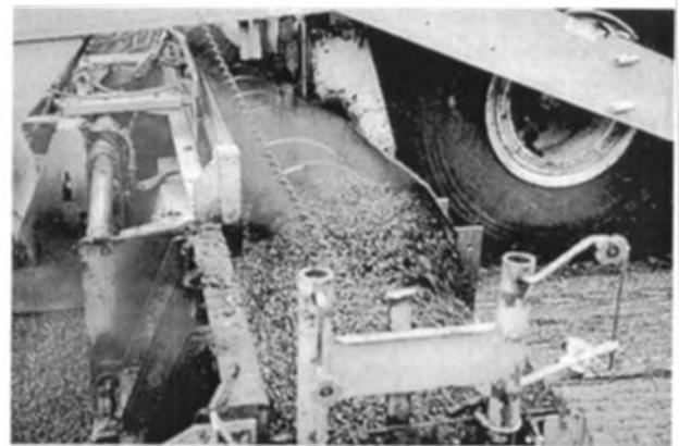
**FIGURE 15-8** Paver auger.
