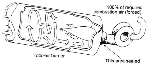
**FIGURE 9-4** Forced-draft, total-air, or 100 percent burner.
