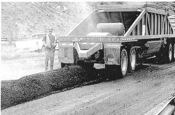
**FIGURE 13-2** Typical bottom- or belly-dump truck.
