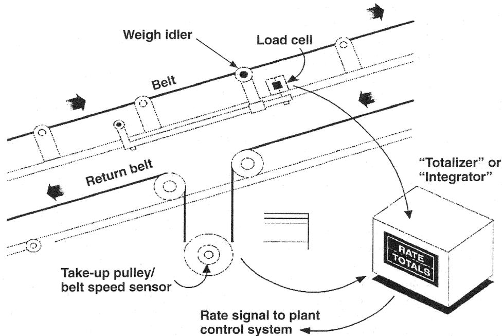
FIGURE 6-10 How a weigh bridge works.
