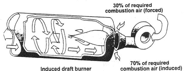
**FIGURE 9-3** Combined induced- and forced-draft burner.
