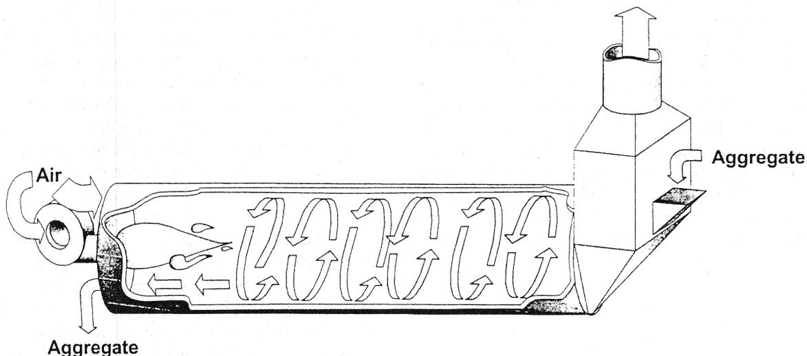
FIGURE 8-1 Typical counter-flow dryer.
