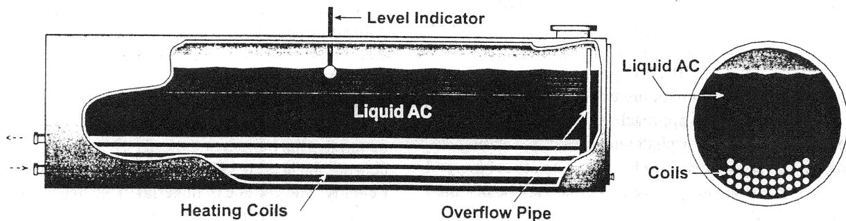
**FIGURE 7-2** Heating of horizontal storage tank.
