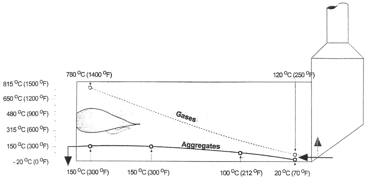
FIGURE 9-6 Temperature profile of counter-flow drum drying aggregate.
