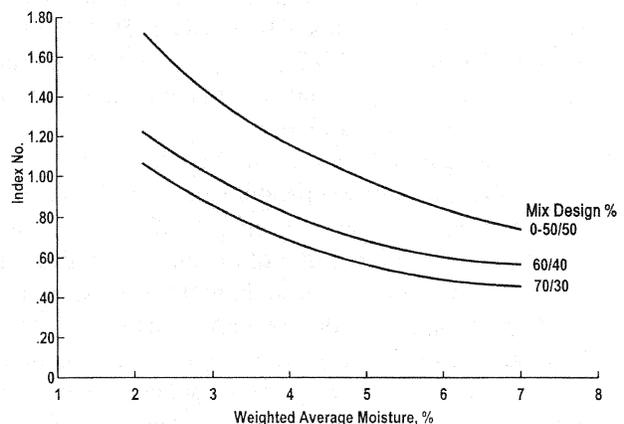
FIGURE 9-10 Effect of amount of RAP on drum-mix plant production.
