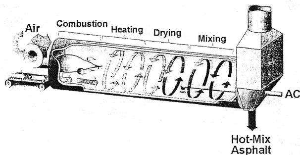
FIGURE 9-7 Parallel-flow drum-mixer zones.
