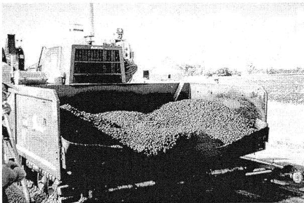
FIGURE 15-2 Loaded HMA paver hopper.
