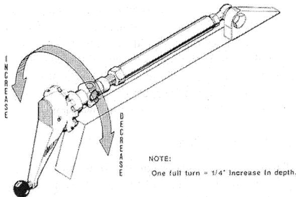
FIGURE 16-1 Thickness control crank.
