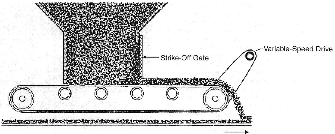
FIGURE 6-5 Continuous feeder belt.
