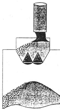
**FIGURE 11-6** Segregation caused by feeding batcher off center.
