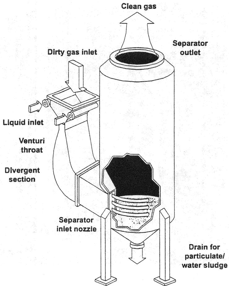
FIGURE 12-5 Flow through typical venturi scrubber.
