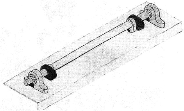
FIGURE 15-16 Screed vibration shaft with weights.
