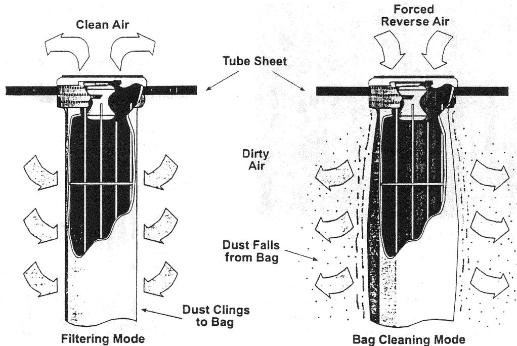
FIGURE 12-10 Bags filtering air and being cleaned.
