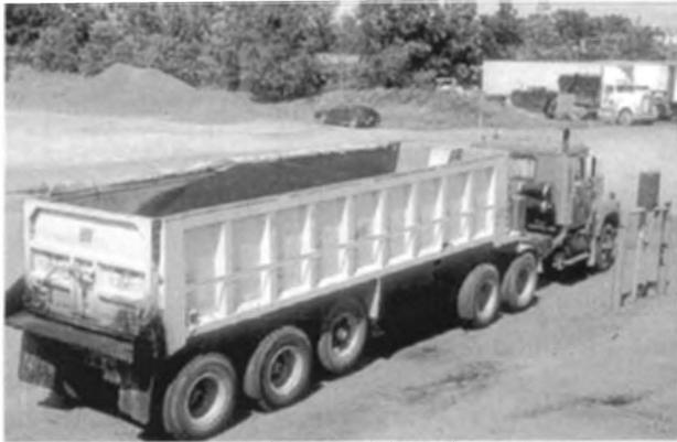
**FIGURE 13-1** Typical end-dump truck.
