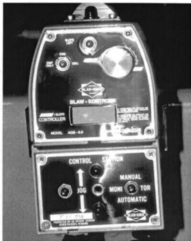
FIGURE 16-10 Slope-control device.
