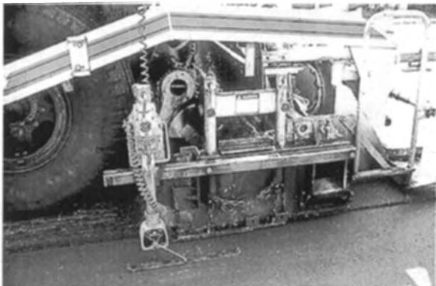
**FIGURE 16-9** Operation of joint-matching shoe.
