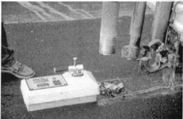
**FIGURE 18-7 Nuclear gauge for monitoring density.**
