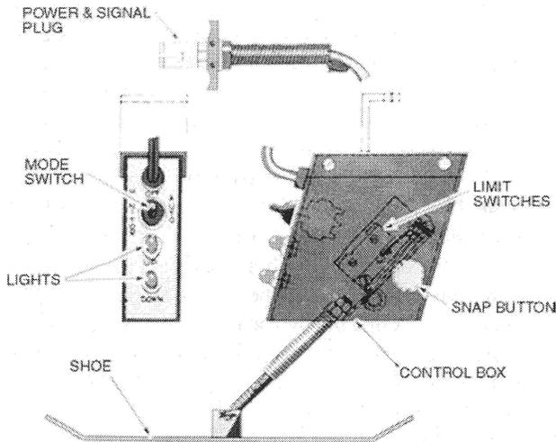
**FIGURE 16-8** Shoe for matching joints.
