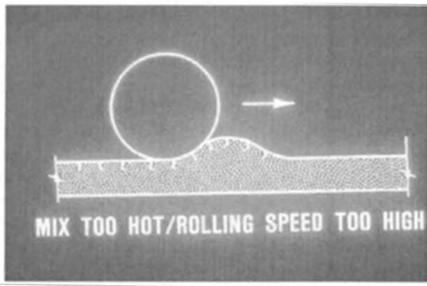
FIGURE 19-3 Roller checking during compaction.
