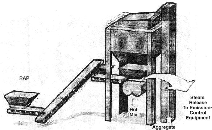
**FIGURE 8-6** Weigh-box method of batch plant recycling.
