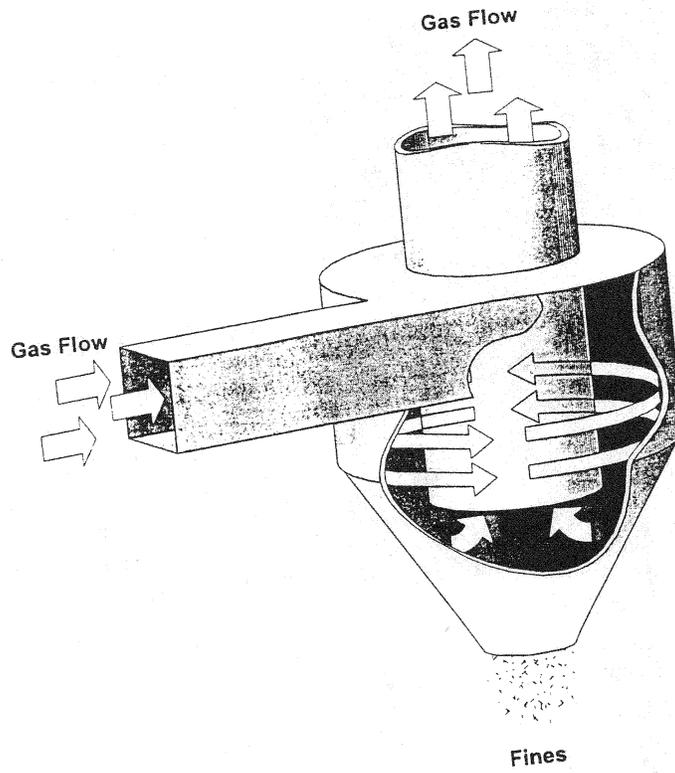
FIGURE 12-2 Flow through a typical cyclone dry collector.
