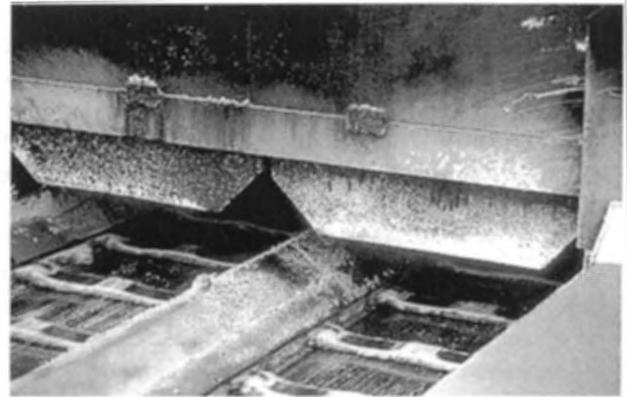
**FIGURE 15-7** Flow gates at back of paver hopper.
