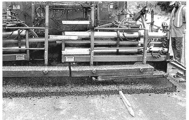
**FIGURE 15-21** Hydraulically extendable screed.
