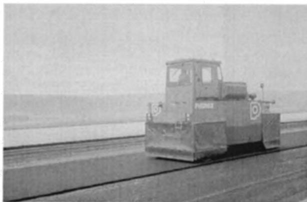
FIGURE 18-5 Pneumatic tire roller with skirts.
