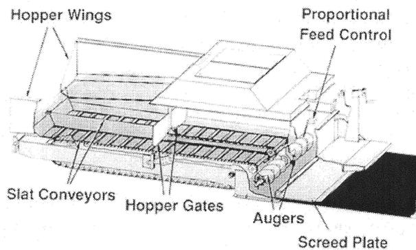
**FIGURE 15-6** Material flow through paver.
