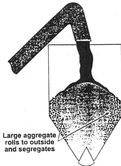
**FIGURE 11-4** Segregation at top of silo without batcher.
