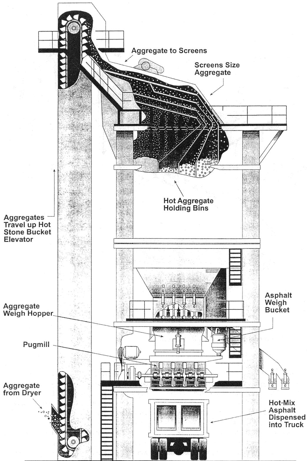
FIGURE 5-3 Flow of materials in batch tower.
