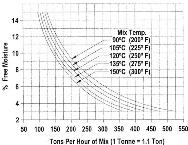
FIGURE 9-9 Effect of moisture content and mix discharge temperature on drum-mix plant production rate.
