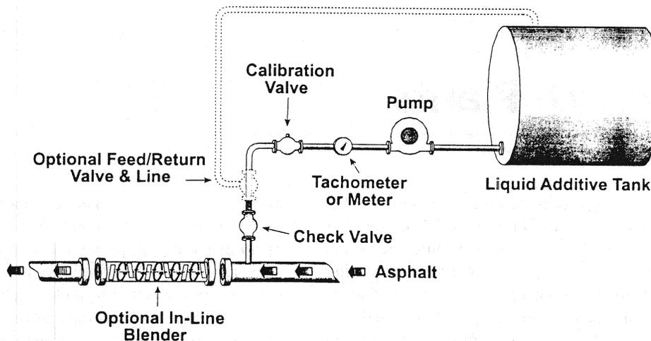
FIGURE 7-4 Typical asphalt additive tank system.
