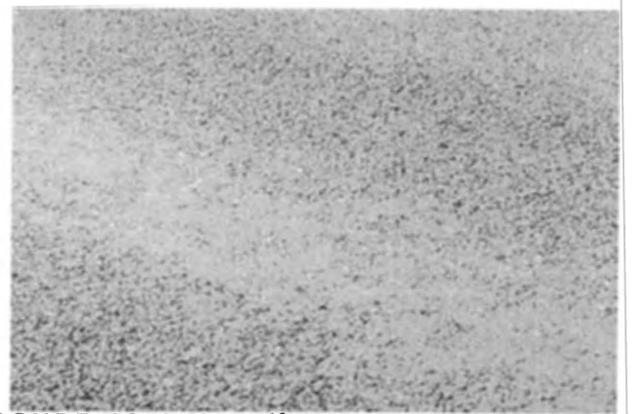
FIGURE 19-1 Nonuniform mat texture after compaction.
