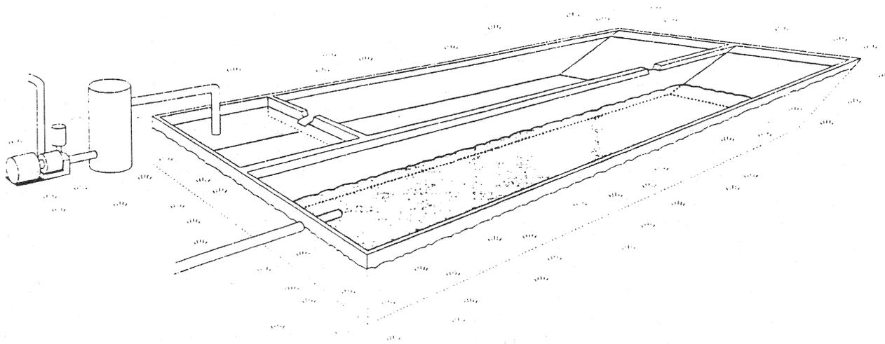
FIGURE 12-6 Typical settling pond.
