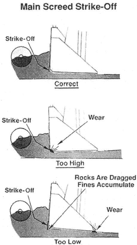
**FIGURE 15-15** Proper positioning of strike-off assembly.
