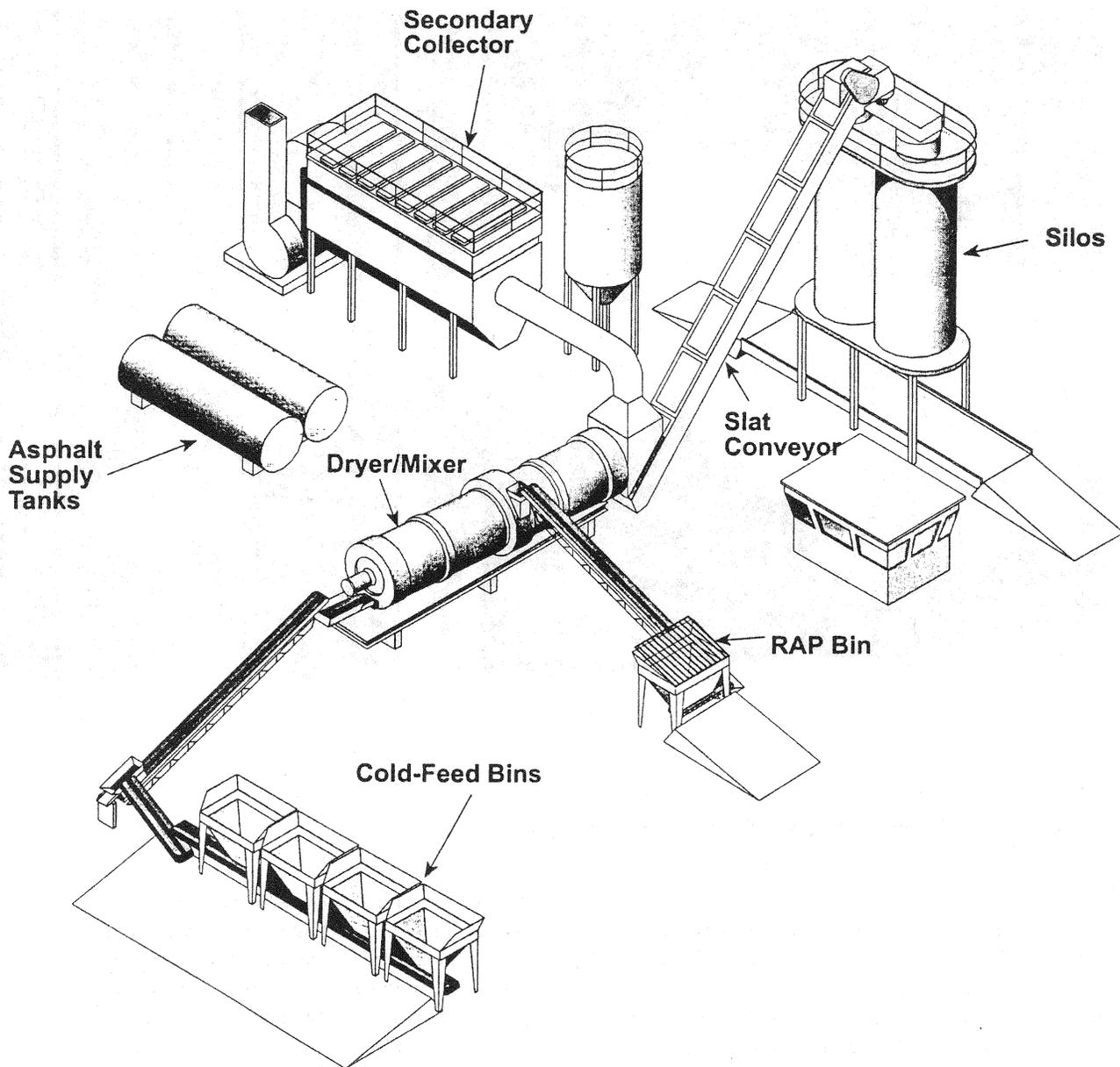
**FIGURE 5-5 Major components of a parallel-flow drum-mix plant.**
