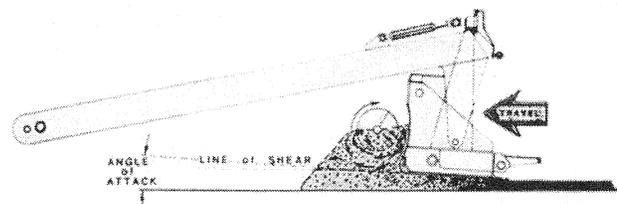
FIGURE 15-13 Angle of attack for paver screed.
