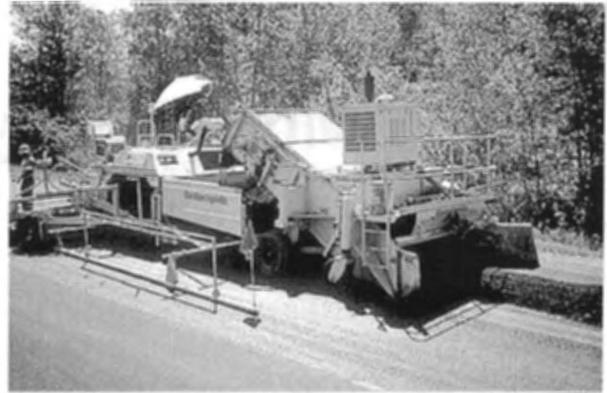
**FIGURE 13-3** Material pickup machine.
