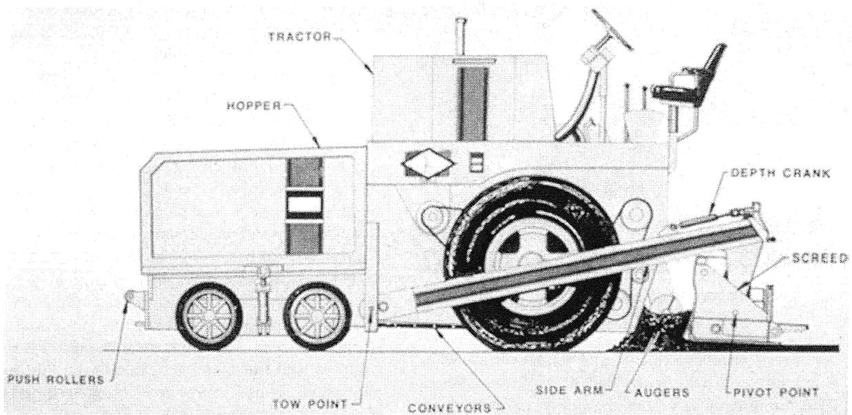
FIGURE 15-1 Schematic of HMA paver.
