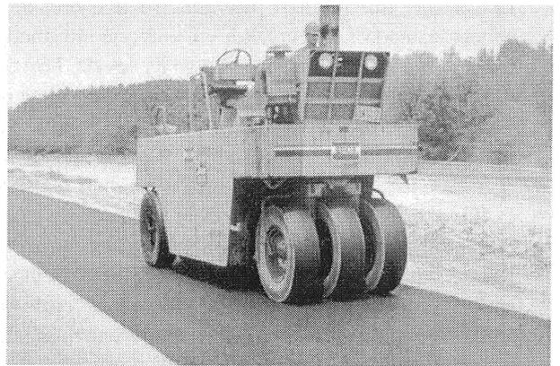
FIGURE 18-4 Pneumatic tire roller.
