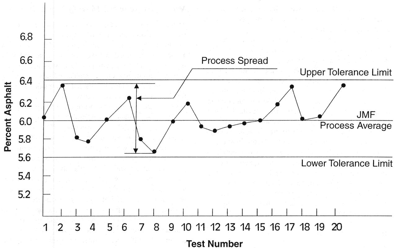
FIGURE 4-2 Asphalt content of paving mixture.
