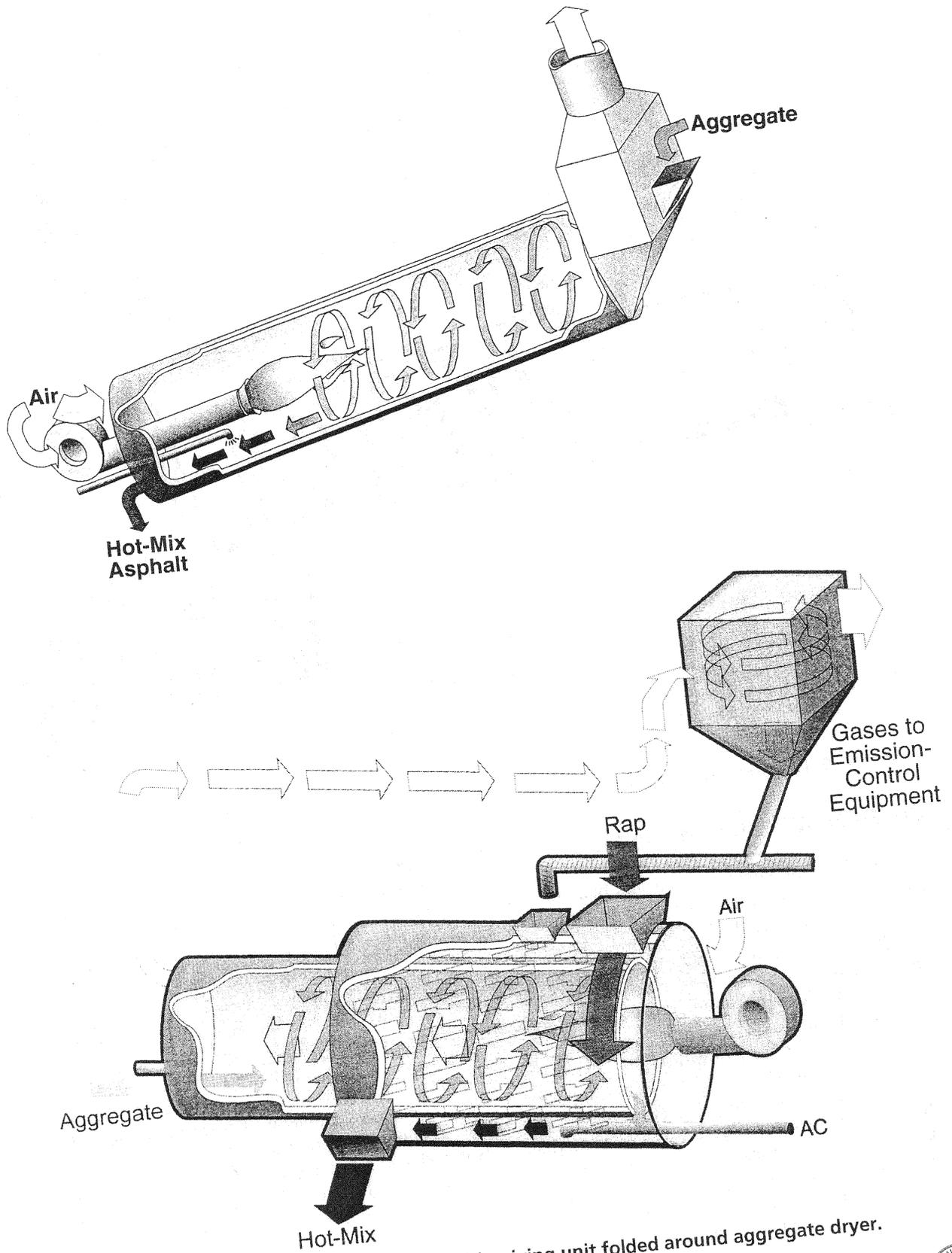
FIGURE 5-8 Counter-flow drum mixer with mixing unit folded around aggregate dryer.
