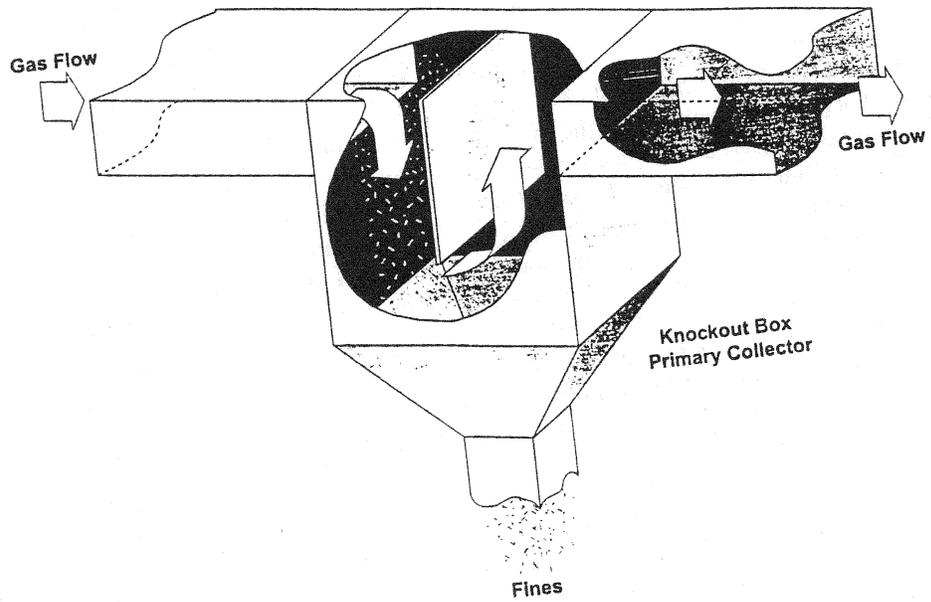
FIGURE 12-3 Flow through a typical knockout box.
