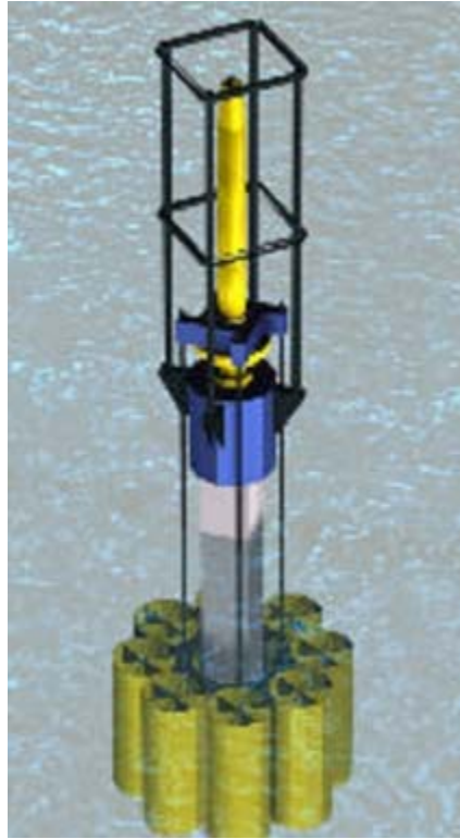
Figure A-53. How water can be used as a counterweight for an over-water statnamics test.
