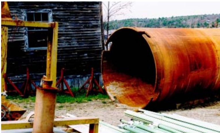
Figure A-2. Mono-directional casing disconnect for underwater termination of casing—Bath-Woolwich Bridge.
