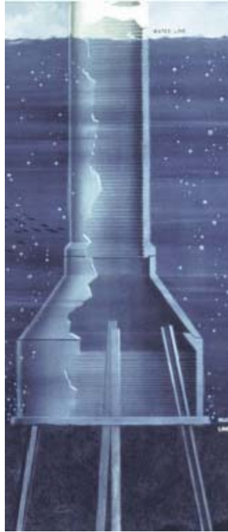
Figure A-12. Use of a precast concrete element as a template for battered H-pile on bridge pier for the Richmond–San Rafael Bridge, California.
