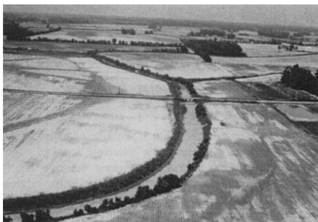
Figure 3-5. Realigned channel without serious instability problems
