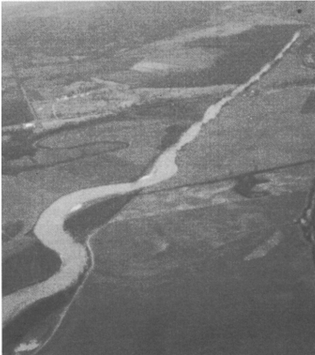
Figure 6-21. Redevelopment of meanders in straightened channel following side bar development
