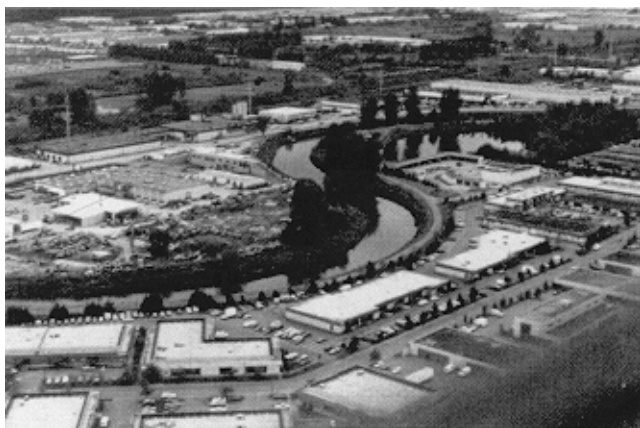
Figure 6-1. Regulated river with levees on meandering alignment
