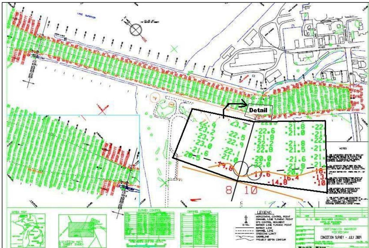
Figure K-6. Hydrographic condition survey of federal navigation channel with soundings referenced to IGLD85 (601.1 ft) Datum.
