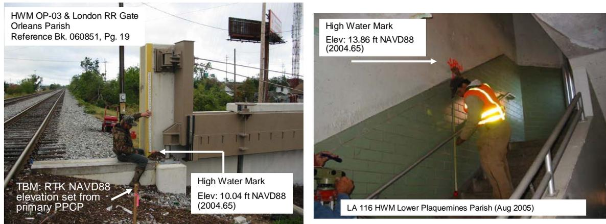
Figure 5-9. High water mark survey procedures and datum documentation.
