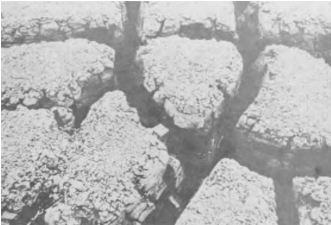
Figure 5-14. Desiccation crust achieved in highly plastic clay dredged material 200 yards into disposal area by perimeter trenching over 12-month period
