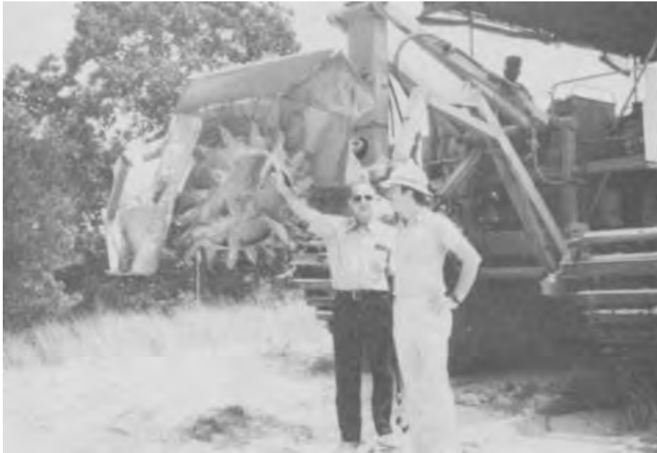
Figure 5-17. View of hemispherical rotary trenching implement
