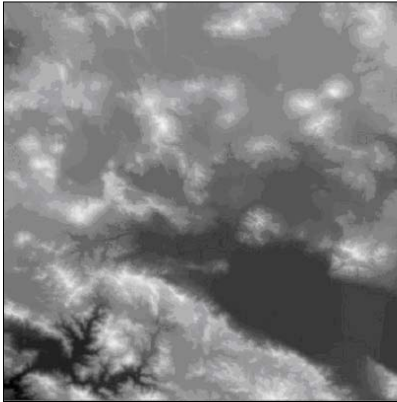
Figure 5-24. Digital elevation model (DEM). The brightness values in this image represent elevation data. Dark pixels correspond to low elevations while the brightest pixels represent higher elevations. Taken from the NASA tutorial at http://rst.gsfc.nasa.gov/Sect11/Sect11_5.html .
