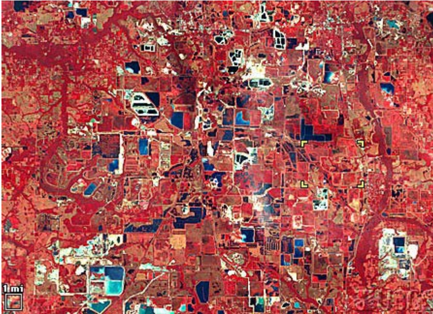
Figure 5-33. Orlando, Florida, imaged in 2000 by Landsat 7 ETM+ bands 4, 3, 2 (RGB). The small circular water bodies in this image denote the location of karst features. Karst topography presents a challenge to development in the Orlando area. Taken from http://edcwww.cr.usgs.gov/earthshots/slow/Orlando/Orlando
