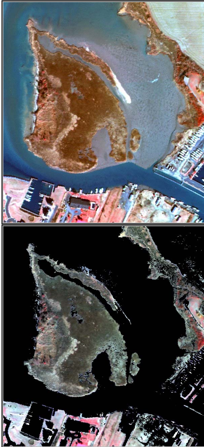
Figure 5-12. Top: True color CAMIS image. Bottom: NDVI mask isolating vegetated pixels. This mask will be useful during the classification process, which will subsequently classify only the vegetation in the scene while disregarding water and urban features. Taken from Campbell (2003).
