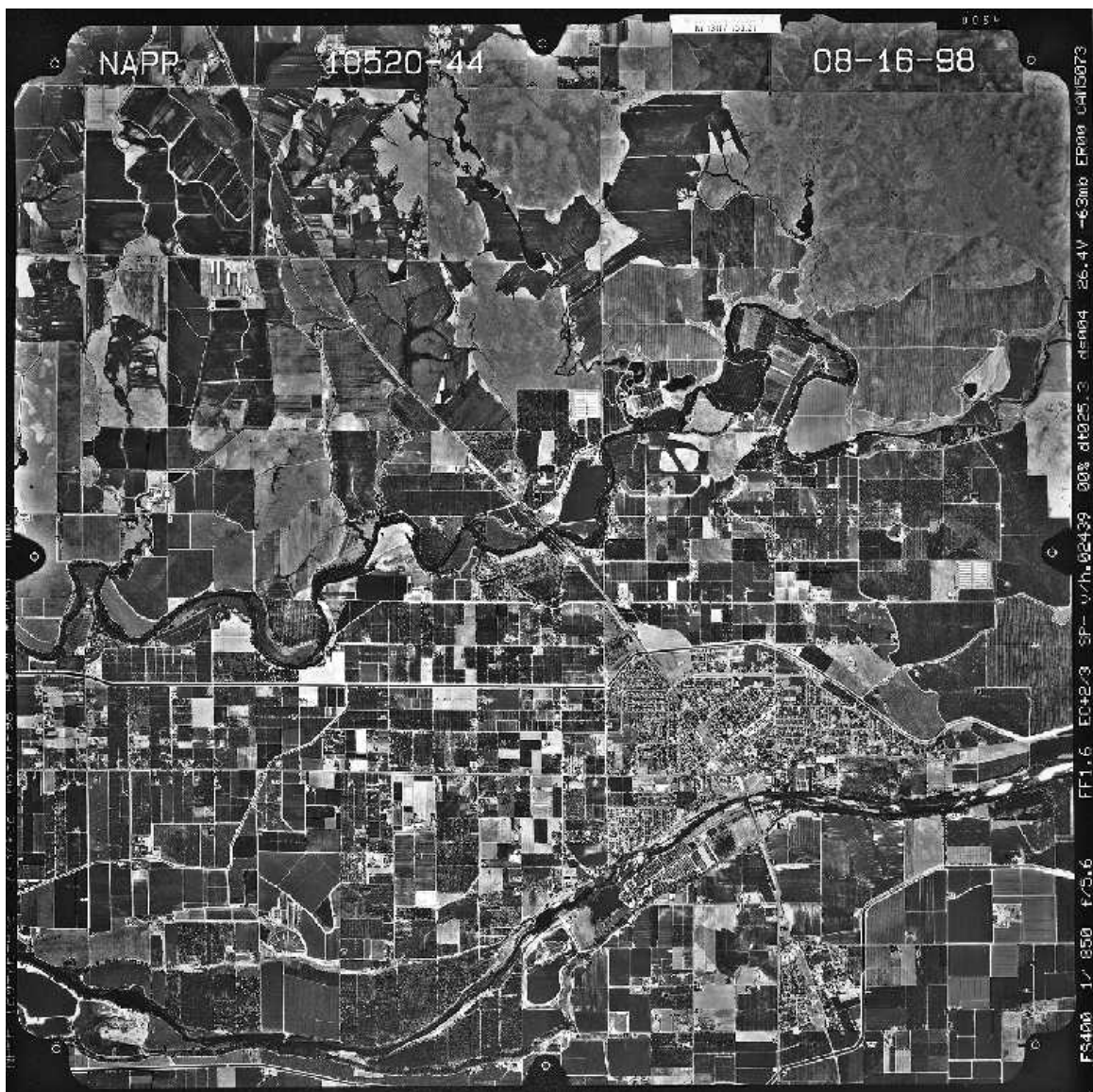
Figure 2-34. Aerial photograph of a predominately agricultural area near Modesto, California. Notice the ancillary data located on the upper and right side margins. These data provide information regarding the location and acquisition of the photo.
