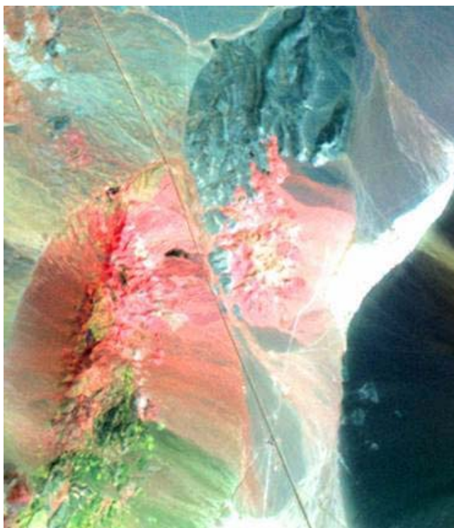
Figure 5-29. Landsat scene bands 5, 4, 2 (RGB). This composite highlights healthy vegetation, which is indicated in the scene with bright red pixels. Taken from http://imagers.gsfc.nasa.gov/ems/infrared.html .
