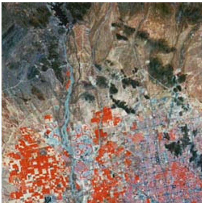
Figure 5-29. Landsat scene bands 5, 4, 2 (RGB). This composite highlights healthy vegetation, which is indicated in the scene with bright red pixels. Taken from http://imagers.gsfc.nasa.gov/ems/infrared.html .
