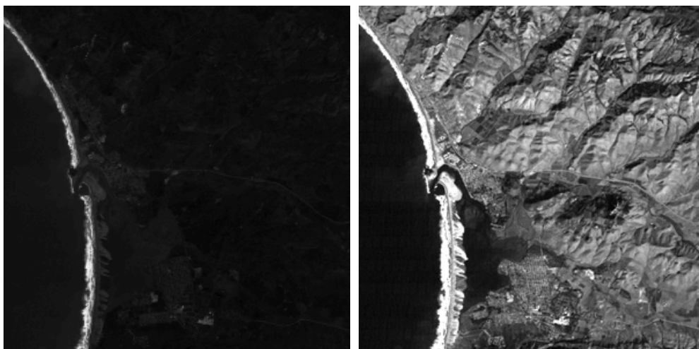
Figure 5-6. Contrast in an image before (left) and after (right) a linear contrast stretch. Taken from http://rst.gsfc.nasa.gov/Sect1/Sect1_12a.html .
