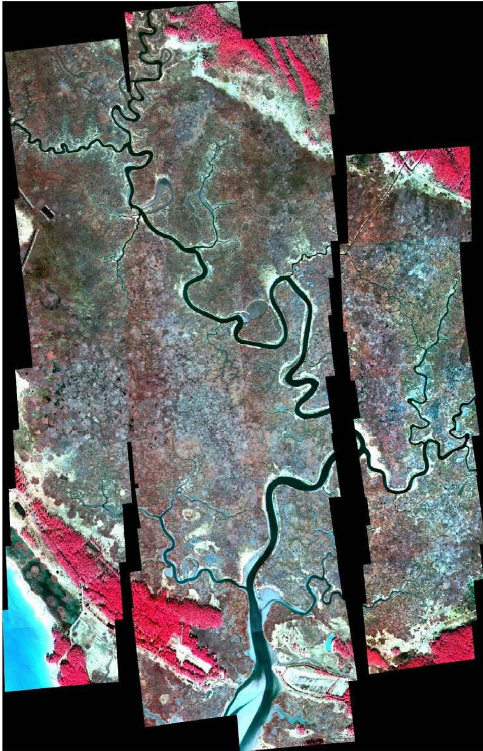
Figure 3-1. In this CAMIS image a decrease in aircraft altitude (due to circumstances beyond the operators control) reduced the pixel size and subsequently decreased the image scene. After mosaicing the individual scenes the side overlaps created “holidays” or gaps in the data. Taken from Campbell (2003).
