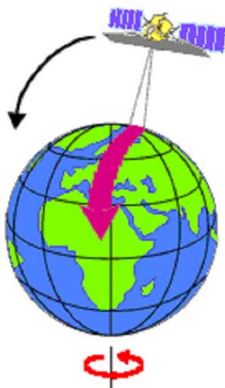
Figure 3-3. Satellite Near Polar Orbit, Courtesy of the Natural Resources Canada.
