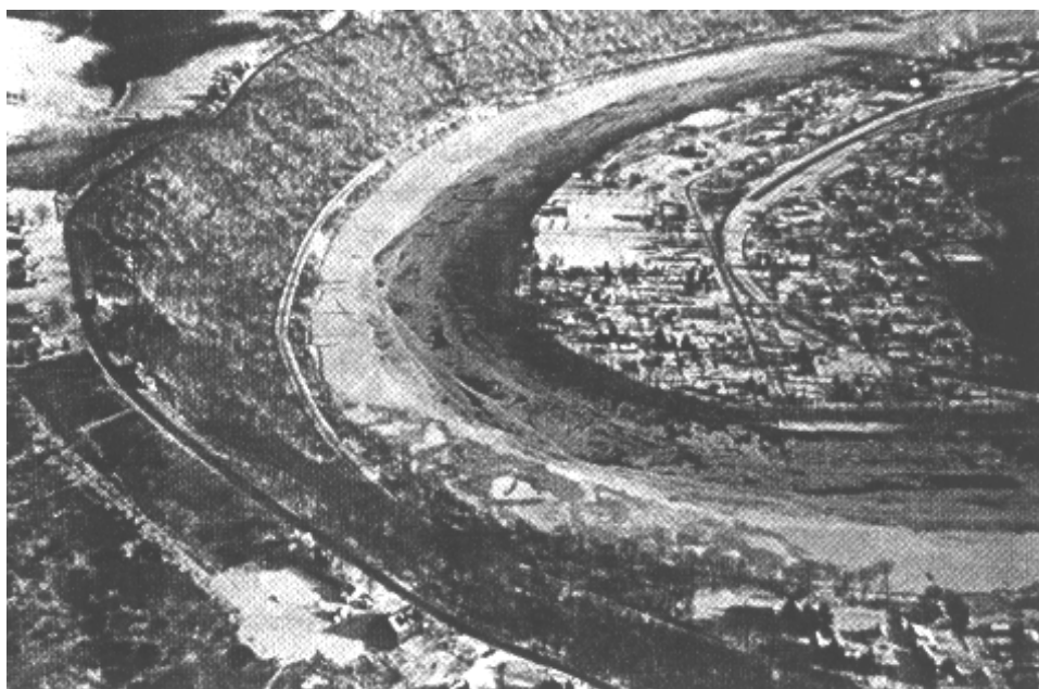
Figure 14-11. Broken, irregular vessel track around a sharp river bend, indicating difficulties in navigating through the ice
