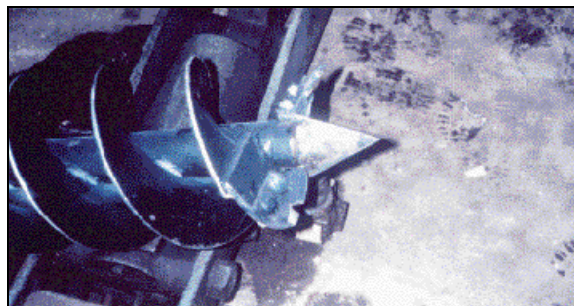
b. Close-up of the modified auger tip.
