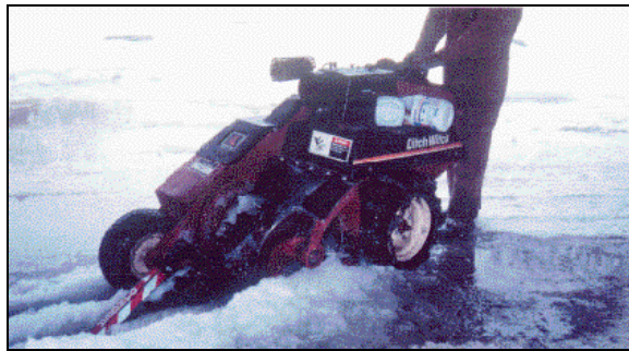
b. Ditchwitch 1260 cutting ice in Montpelier, Vermont.
