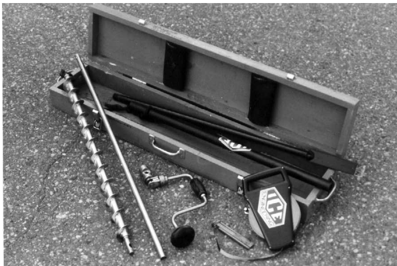
Figure 16-8. Standard CRREL ice thickness measuring kit.
