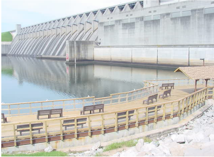
Photo N-17. Fishing pier, Example 5. Below dam, J. Strom Thurmond Lake, SC. This shows recommended amenities including lowered section in railing for UA, rod holders, and benches. Visible at right edge is shade shelter roof. A picnic table is just outside the photo (Tables 5.9 and 5.10 )
