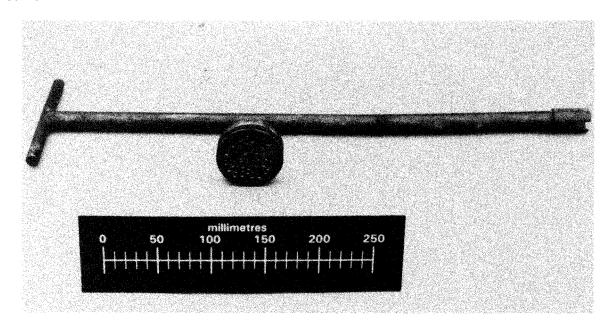
Figure 6-5. Photograph of a perforated, expandable packer
