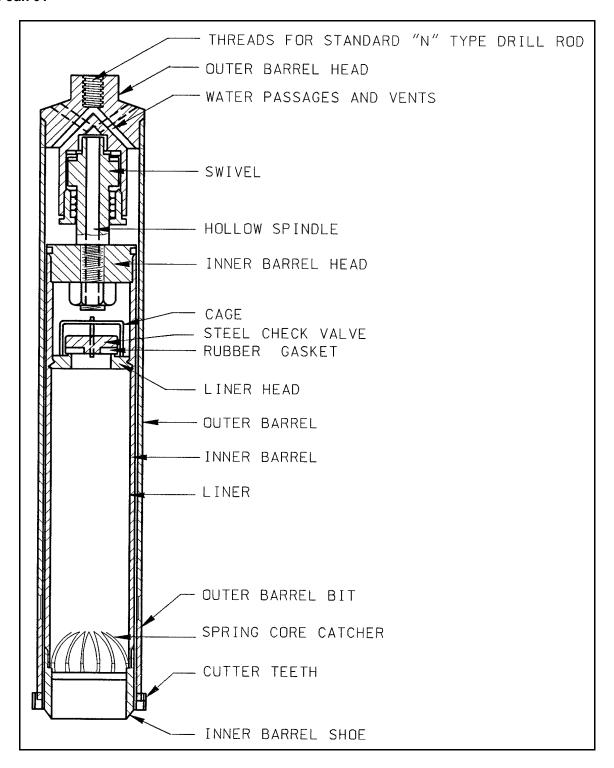
Figure 5-12. Schematic diagram of the Denison sampler (after Hvorslev 1949)
