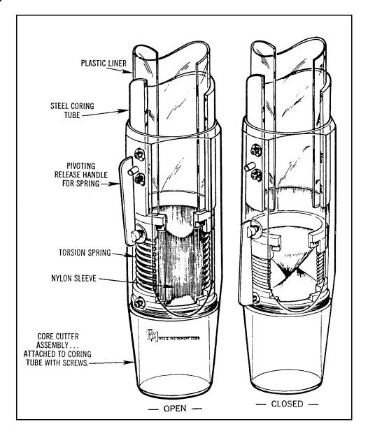
Figure 10-20. Isometric drawing of a core catcher with a sphincter closure to retain the core. (Figure provided by the U.S. Naval Facilities Engineering Service Center)
