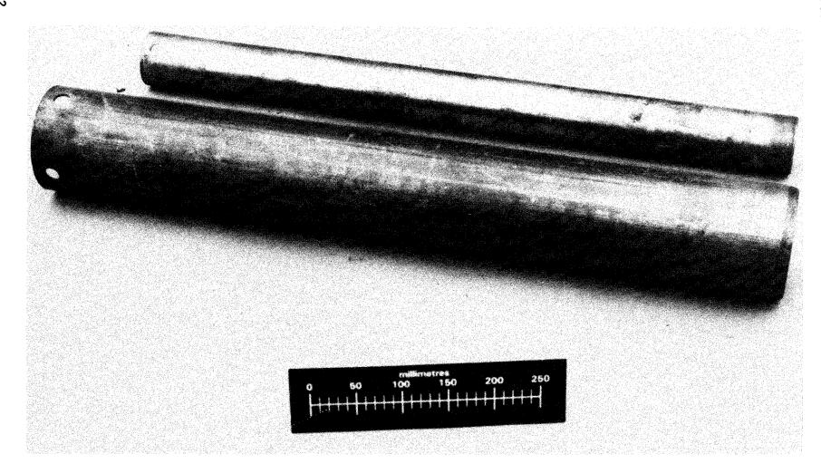
Figure 5-20. Photograph of 75-mm- (3-in.-) and 125-mm- (5-in.-) diam sampling tubes
