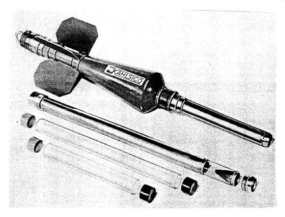
Figure 10-11. Photograph of the Phleger gravity corer. (Figure provided by the U.S. Naval Facilities Engineering Service Center
