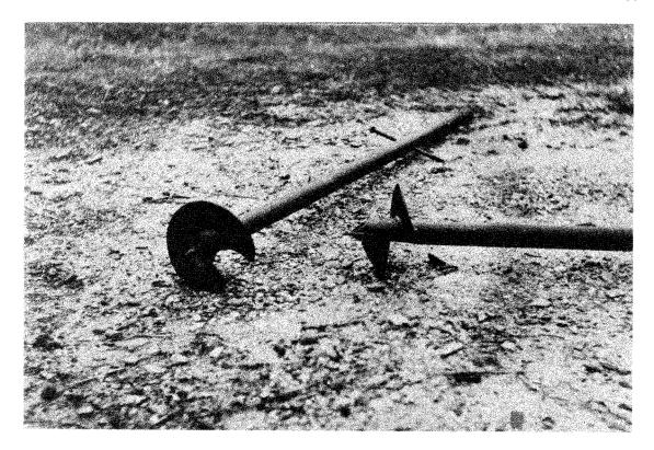
Figure 6-1. Photograph of a screw-type earth anchors
