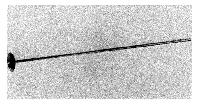
Figure 6-6. Photograph of a sampling tube wall scraper
