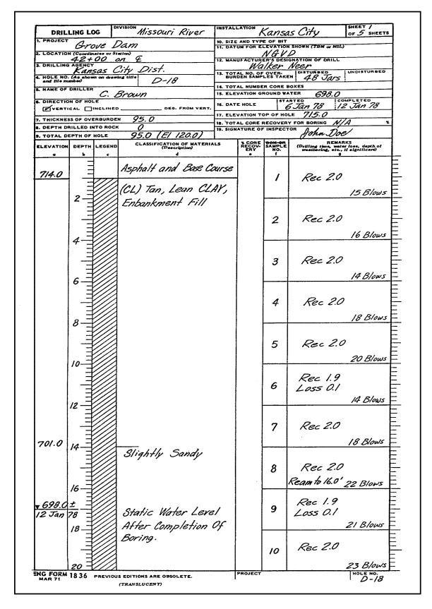
Figure D-2. Example of Form 1836 for overburden, disturbed, and drive data
