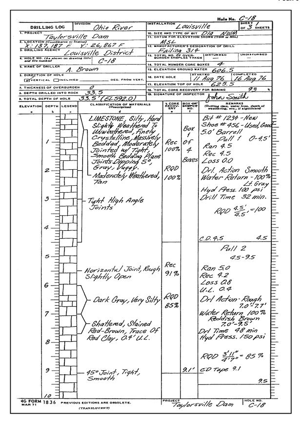
Figure D-7. Example of Form 1836 for bedrock and core data (Sheet 1 of 3)
