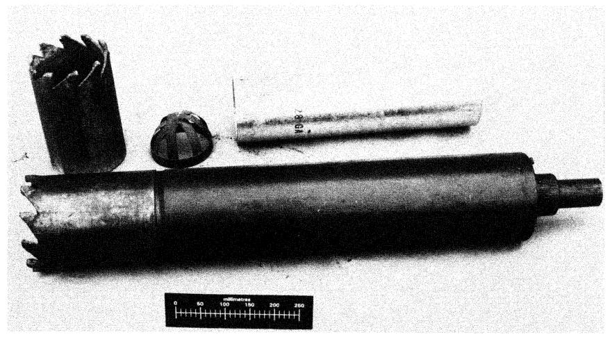
Figure 5-11. Photograph of the Denison sampler
