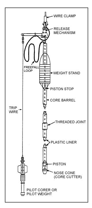
Figure 10-14. Schematic diagram of a typical piston-type gravity corer. (Figure provided by the U.S. Naval Facilities Engineer Service Center)
