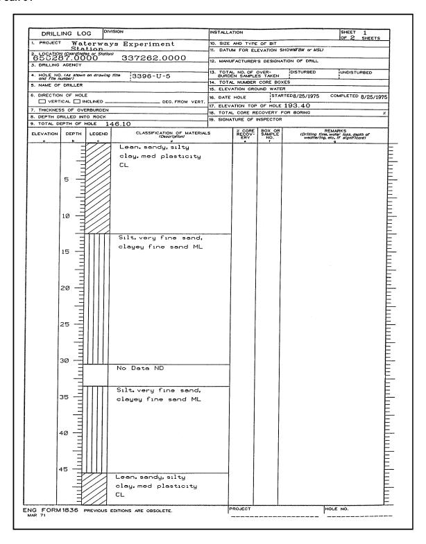
Figure D-8. Foundation boring in which geotechnical data were entered into the BLDM, exported to Intergraph Insight, and printed in the ENG FORM 1836 format (Continued)
