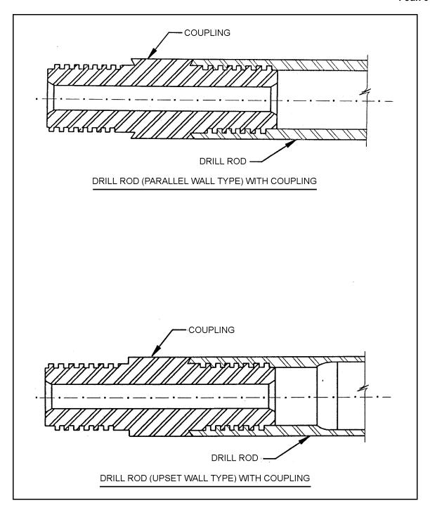
Figure 3-11. Cross sections of drill rods which illustrate upset and parallel wall tubing (after Hvorslev 1949)
