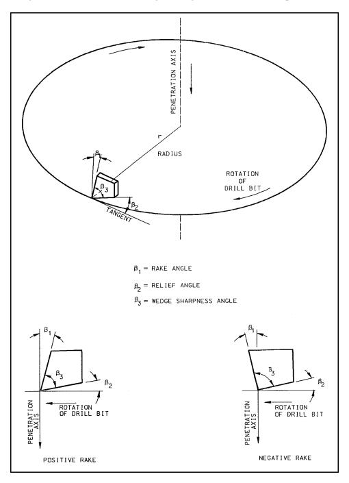
Figure 9-1. Schematic of a cutting tooth which defines the shape and orientation of the tooth (after Mellor 1976)
