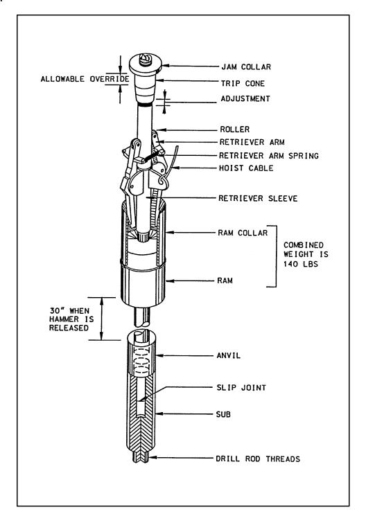
Figure G-2. Schematic drawing of the automatic trip hammer
