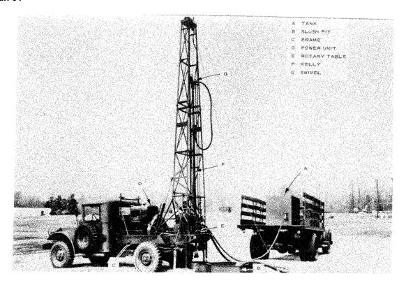
Figure 3-3. Truck-mounted rotary drill rig with a chain feed drive system
