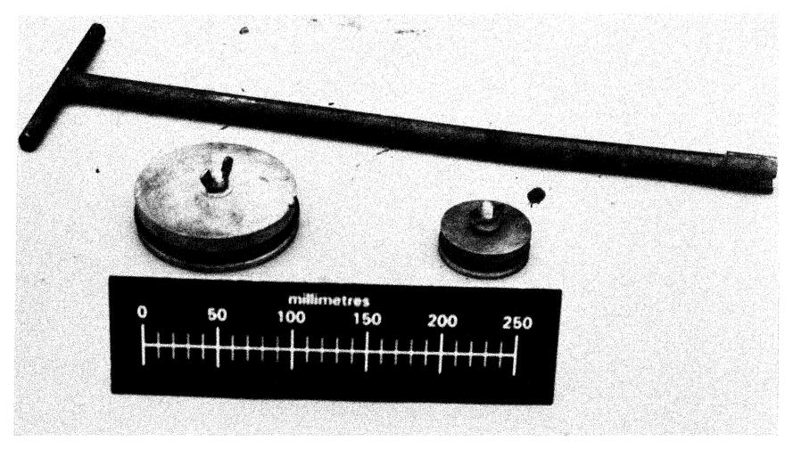
Figure 6-3. Photograph of an expandable packer
