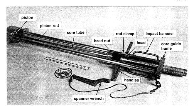
a. Diver-operated corer with parts identified
