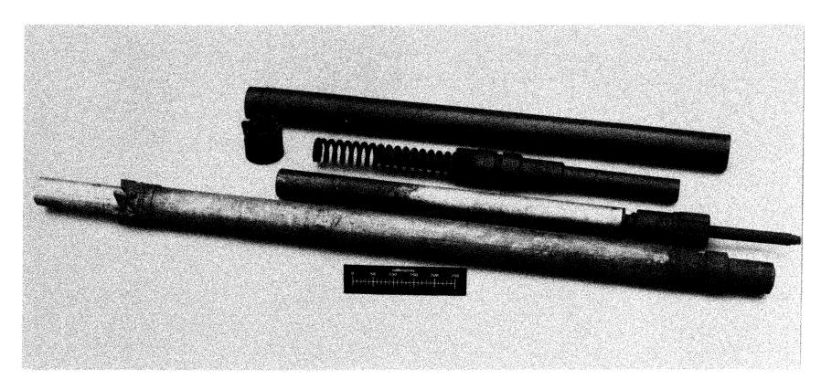
Figure 5-13. Photograph of the Pitcher double-tube core barrel sampler
