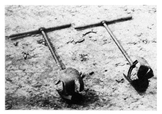
Figure 7-1. Photograph of an Iwan auger
