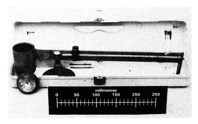
Figure 4-2. Mud balance for determining the density of drilling mud
