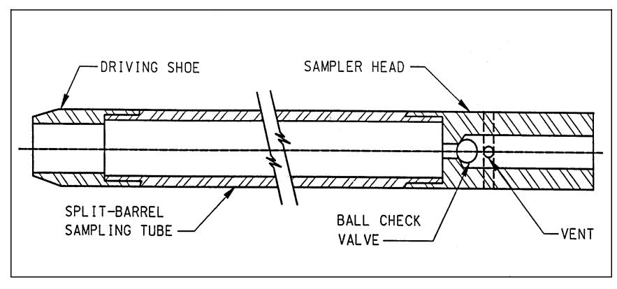
Figure G-4. Schematic drawing of the split-barrel sampler
