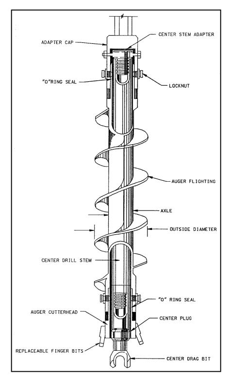
Figure 5-17. Isometric drawing of the hollow-stem auger with the center drag bit which can be used with soil sampling devices (after Acker 1974)
