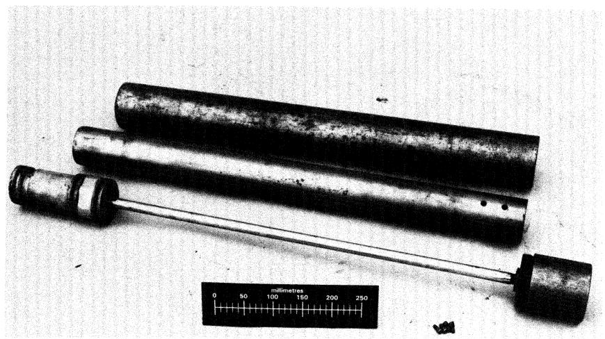
Figure 5-7. Photograph of the Osterberg sampler
