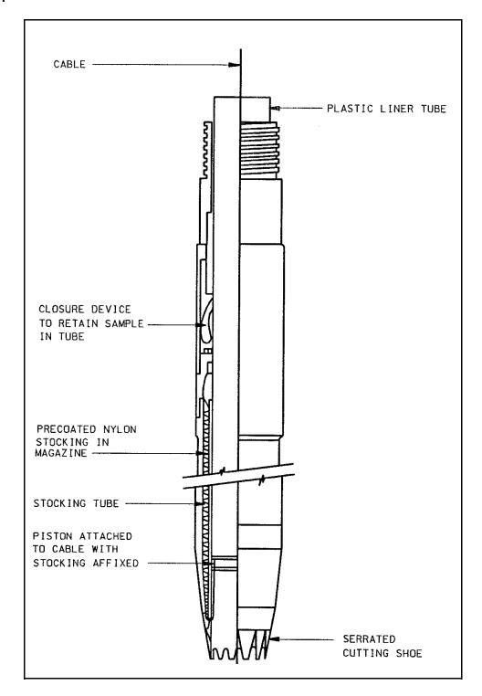
Figure 5-10. Schematic diagram of the Delft continuous soil sampler
