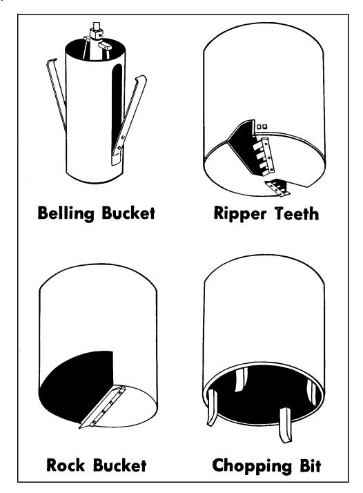
Figure 7-6. Isometric drawing of several types of bucket augers
