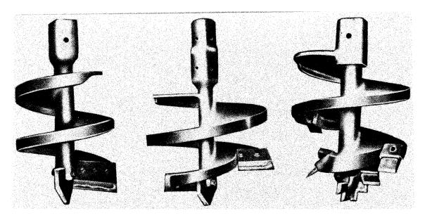
Figure 7-4. Photograph of short-flight solid-stem augers
