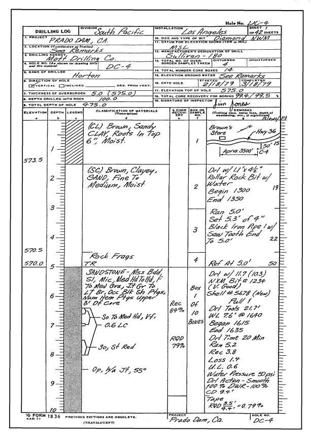
Figure D-6. Example of Form 1836 for bedrock, disturbed, SPT, and core data (Continued)
