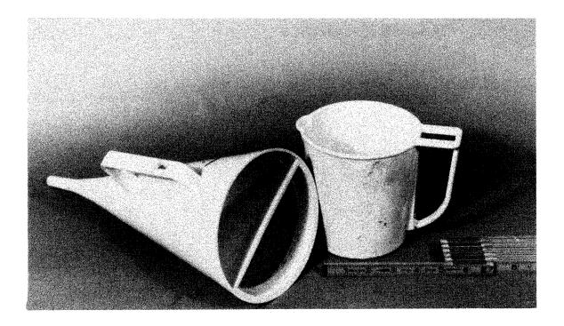
Figure 4-1. Photograph of a Marsh funnel and a one quart (0.95 dm³) measuring cup for determining the viscosity of drilling mud
