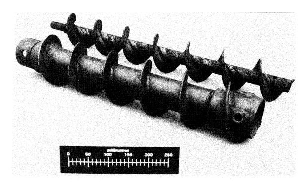
Figure 7-5. Photograph of segments of a continuous-flight solid-stem auger and a continuous-flight hollow-stem auger
