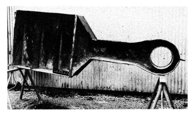
Figure 4-6. Photograph of a portable mud pit
