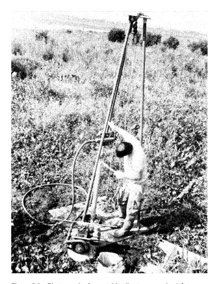
Figure 7-9. Photograph of a portable vibratory sampler (after Smith, Dunbar, and Britsch 1986). Note: Safety is a very important consideration for Corps of Engineers projects. Safety items, including hardhats, gloves, safety shoes, protective clothing, and dust or vapor masks, should be worn, as appropriate, for the particular drilling and sampling operation
