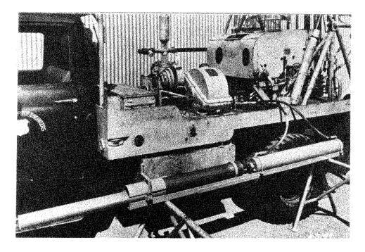
Figure 6-7. Photograph of a hydraulic sample jack which is operated by the hydraulic system of the drill rig
