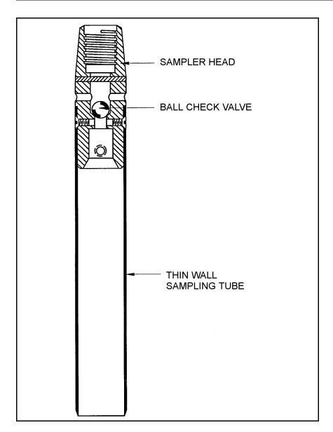
Figure 5-1. Schematic drawing of an open-tube sampler
