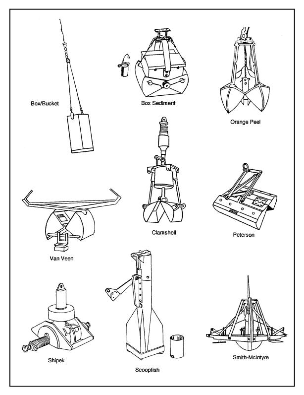
Figure 10-9. Schematic diagrams of several dredges and grab samplers that can be used to obtain disturbed, surficial sediment samples of the seafloor from almost any depth of water. (Figure provided by the U.S. Naval Facilities Engineering Service Center)
