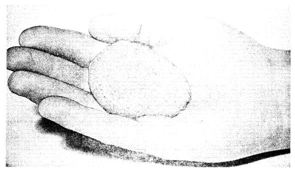
Figure E-5. Livery appearance of a sample of moist, fine-grained soil which occurred as a result of shaking during the dilatancy test
