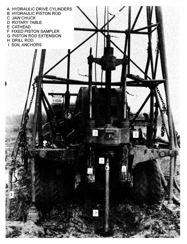
Figure 3-2. Photograph of a truck-mounted rotary drill rig with specific features of the drill rig identified
