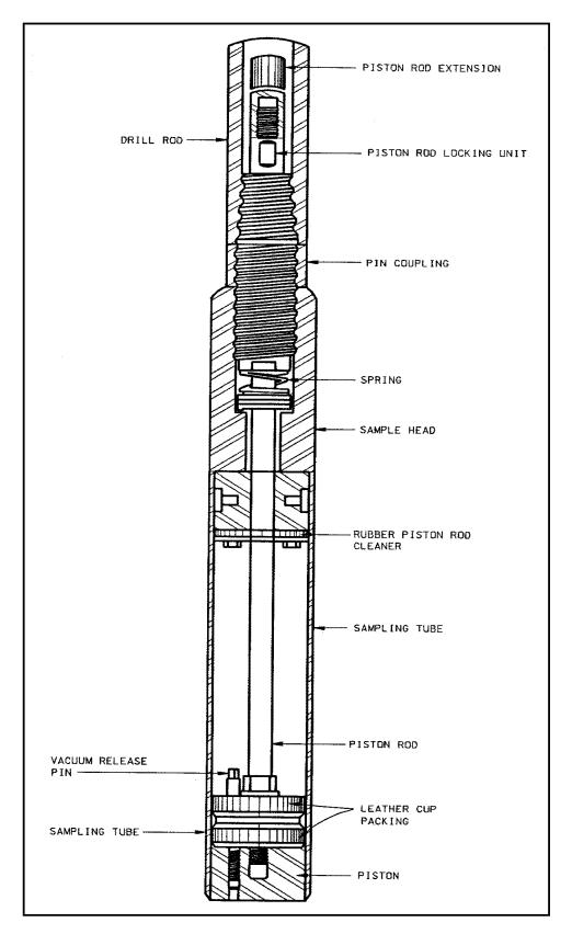
Figure 5-6. Cross-sectional diagram of the Butters samplers (after U.S. Department of the Interior 1974)
