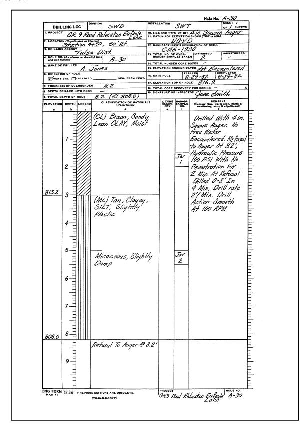
Figure D-3. Example of Form 1836 for overburden, disturbed, and auger data
