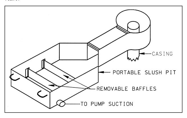
Figure 4-5. Sketch of a portable mud pit
