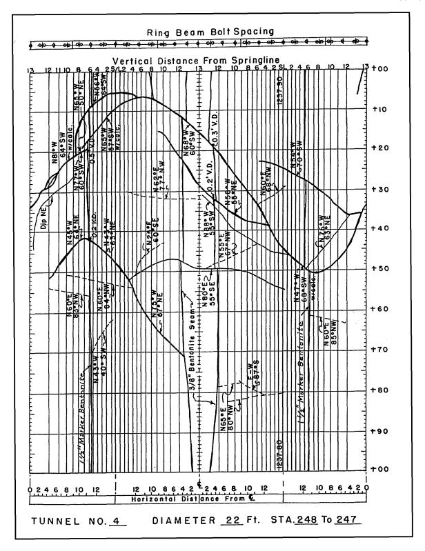
Figure C-2. Developed plan of cylindrical tunnel section Fort Randall Dam, South Dakota (note: 1 ft = 0.3 m approx.)
