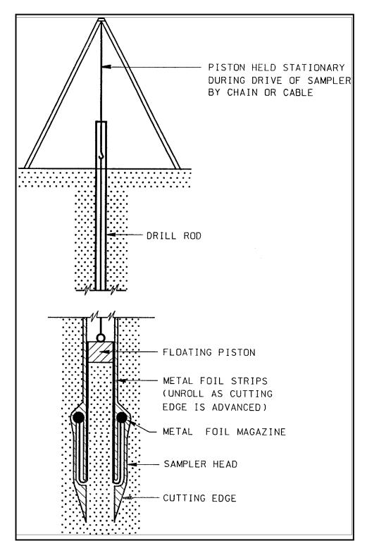
Figure 5-9. Schematic diagram of the Swedish foil sampler
