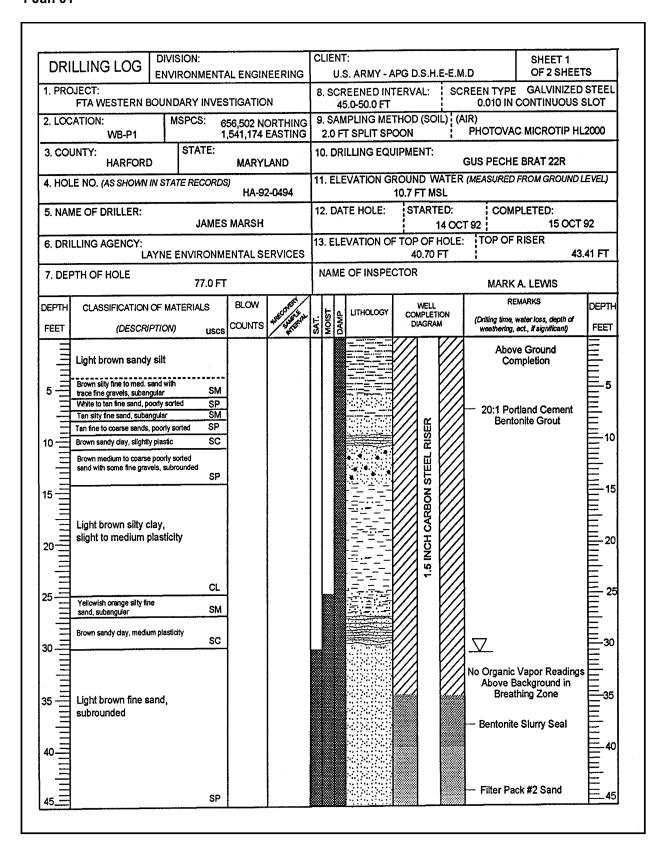
Figure 5-2. Example of a report-quality log with lithologic, blow count, moisture, and well completion information. Note that the header contains a variety of details concerning this monitoring well (Continued)
