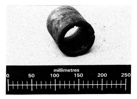
Figure 3-16. Photograph of a typical diamond coring bit
