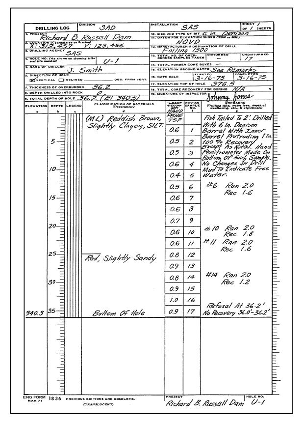
Figure D-4. Example of Form 1836 for overburden, undisturbed, and Denison data
