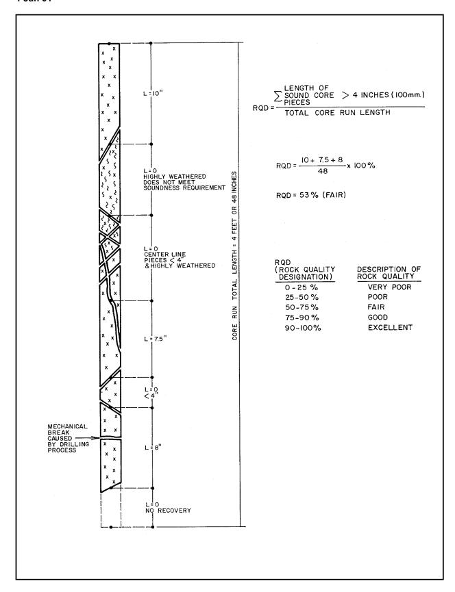
Figure 5-1. Illustration of Deere and Deere (1989) modified procedure for calculating RQD
