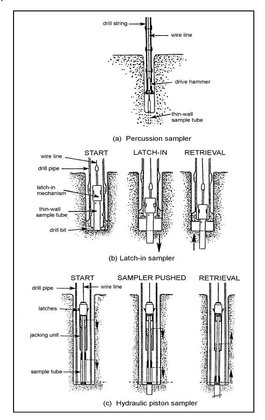
Figure 10-18. Wireline sampling tools which can be used if a motion compensation system is not available. (Figure provided by the U.S. Naval Facilities Engineering Service Center)
