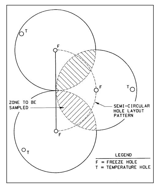
Figure D-2. Semicircular layout of freeze holes and temperature holes
