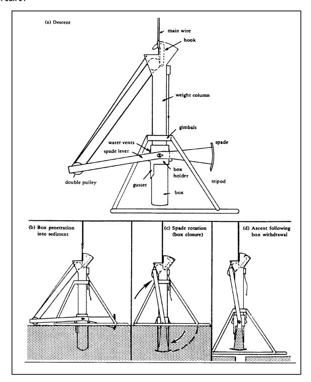
Figure 10-10. Conceptual presentation of the operating sequence of the box corer. (Figure provided by the U.S. Naval Engineering Service Center)
