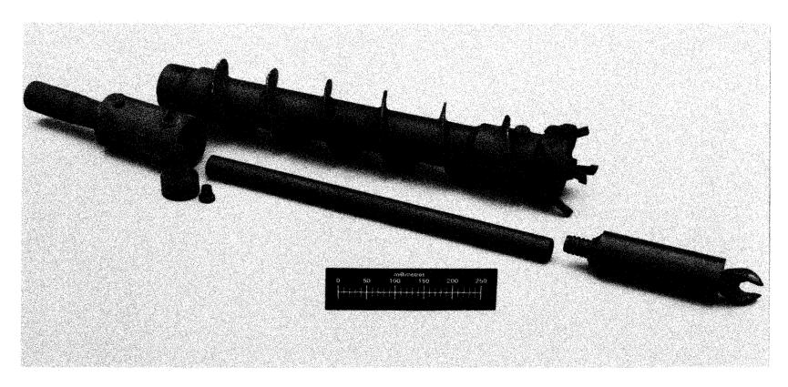
Figure 5-16. Photograph of a hollow-stem auger with a center drag bit
