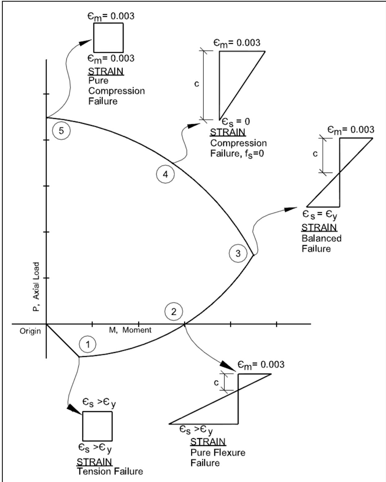
Figure 4-2. Interaction Diagram with Strain Conditions Illustrated.
