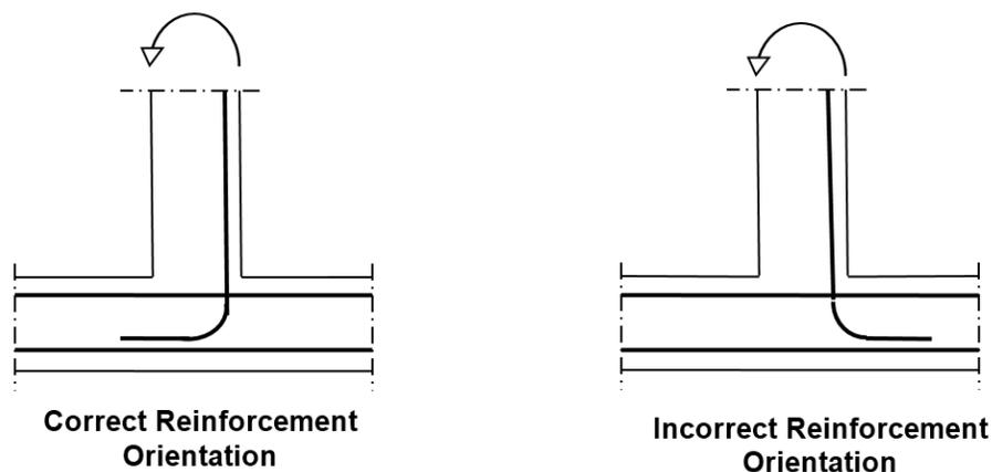
Figure 2-1. Reinforcement Detailing at Moment Connections.
