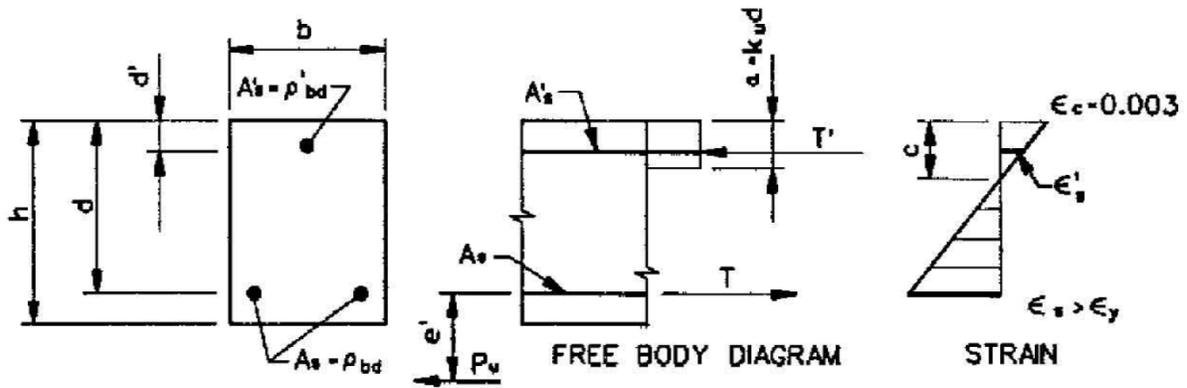
AXIAL TENSION, CONCRETE AT COMPRESSION FACE AT ULTIMATE STRAIN OF 0.003
