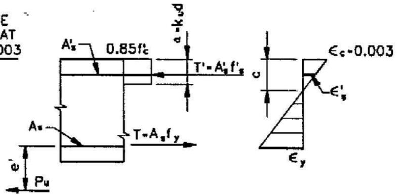
AXIAL TENSION, BOTH LAYERS OF STEEL IN TENSION
