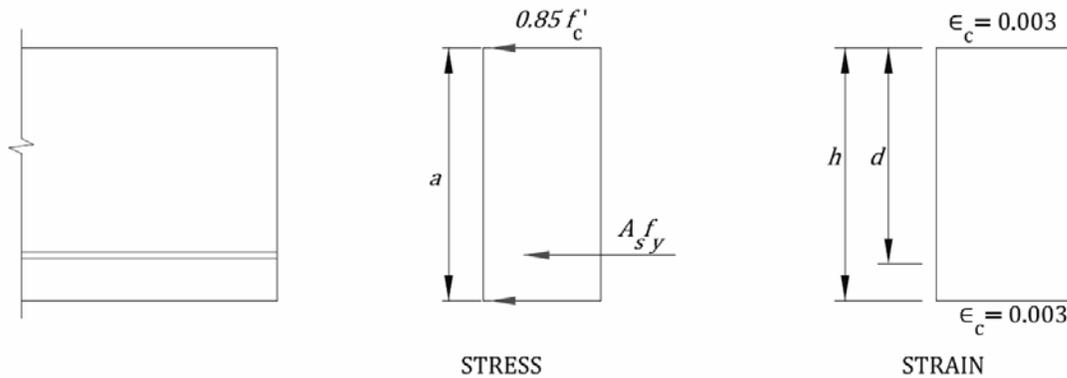
Figure C-5. Stress and Strain under Maximum Axial Load.
